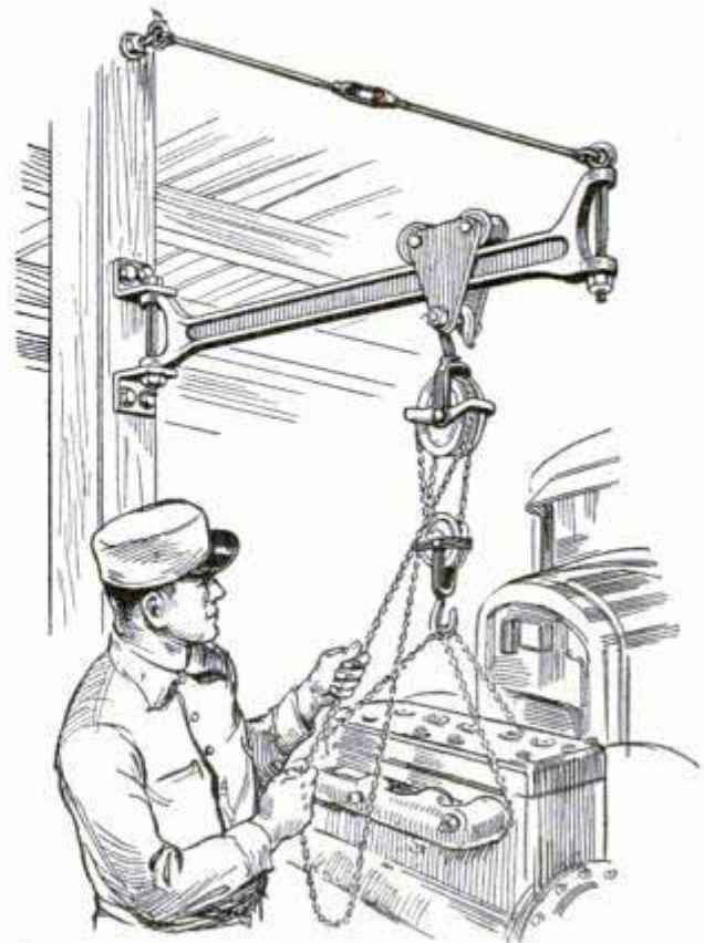
Discarded Auto Axle Can Be Used to Make a Crane for the Small Garage
