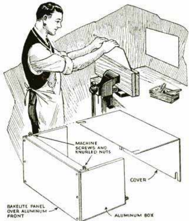
Above, Bending the Aluminum Sheet; Below, Diagram Showing Construction of Removable Top and Back
