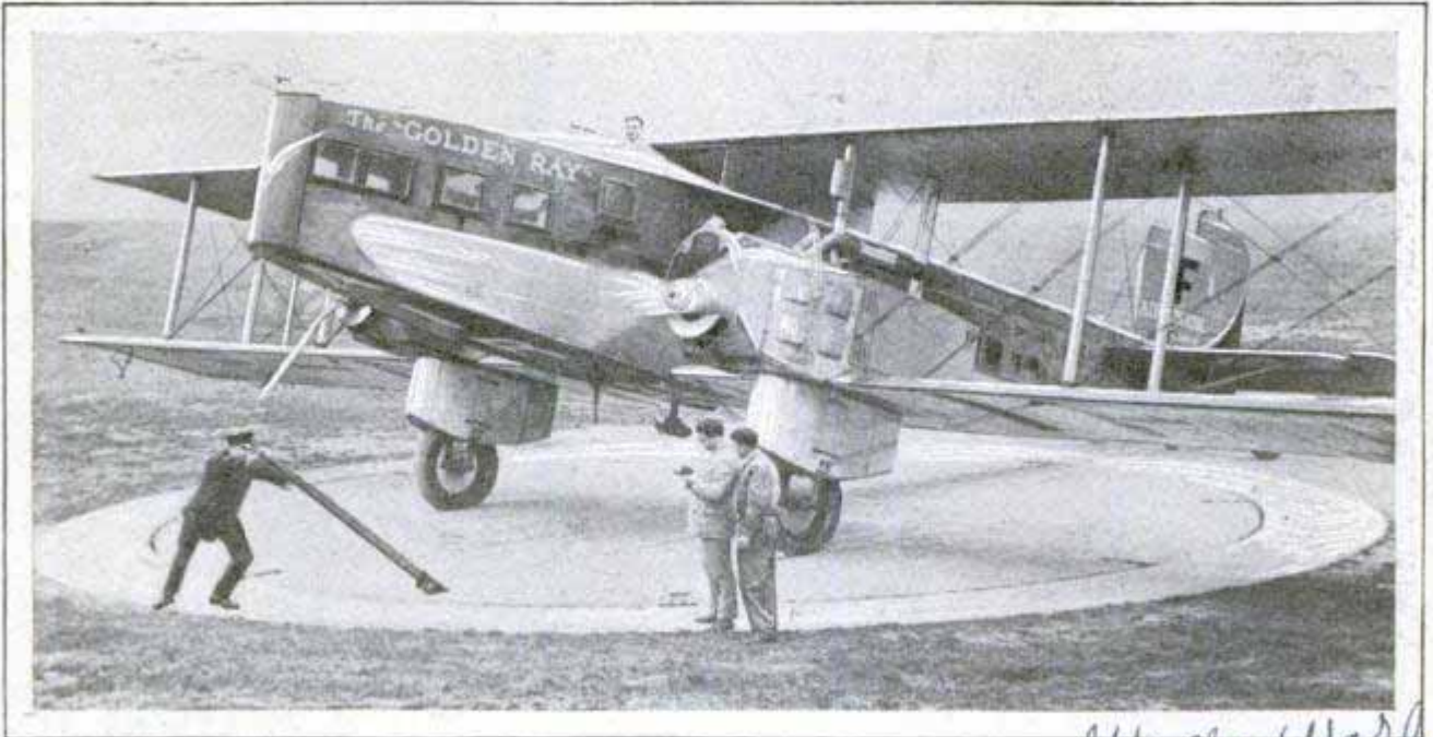
Turntable for Airplanes at Croydon Airdrome in London; It Is Not Used like the Ordinary Turntable to Wheel the Ships End for End, but as an Aid in Adjusting the Plane's Compass
