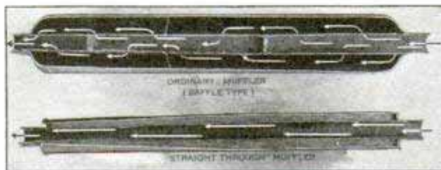
Above, Ordinary Baffle-Type Muffler, and, Below, a Type in Which Exhaust Gases Pass Straight Through
