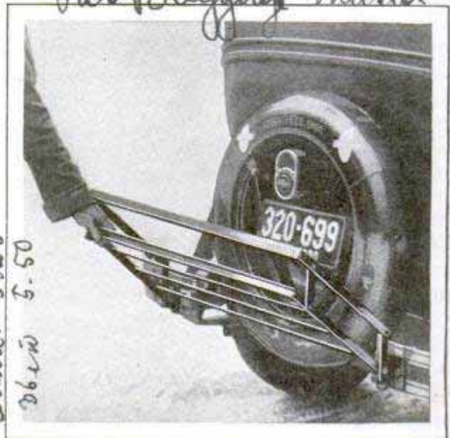
Auto Luggage Carrier Attached to Rear Bumpers, Thus Affording Easy Access to the Spare Tire
