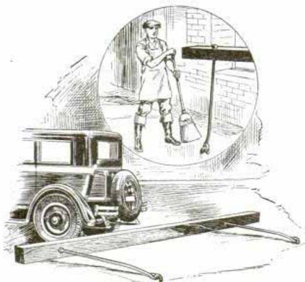
Wooden Beams Installed on Garage Floor Stop Cars from Hitting the Wall
