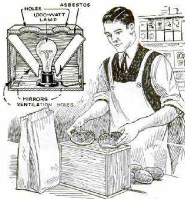
Candler Fitted with a 1,000-Watt Lamp, Shows Up Hollow Spots in Potatoes
