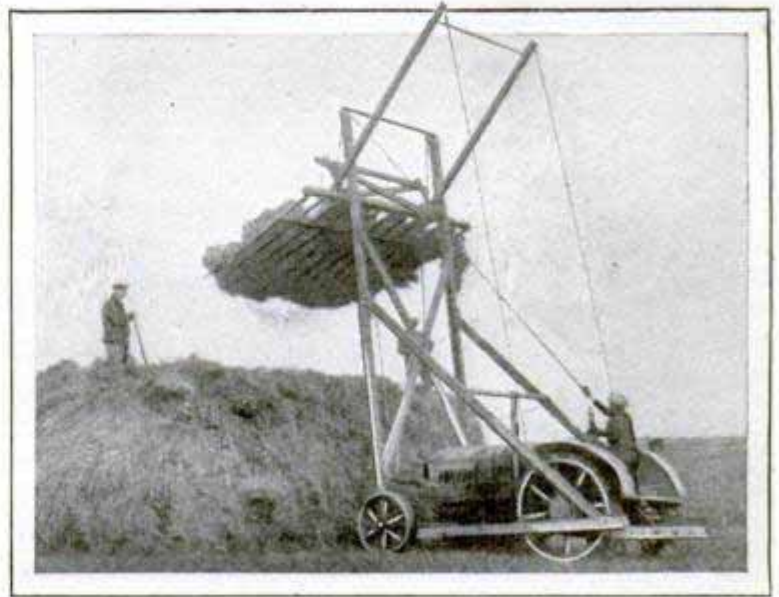
Hay Stacker Mounted in Front of Tractor; It Gathers and Piles the Hay in a Stack and Also Loads Grain Shocks
