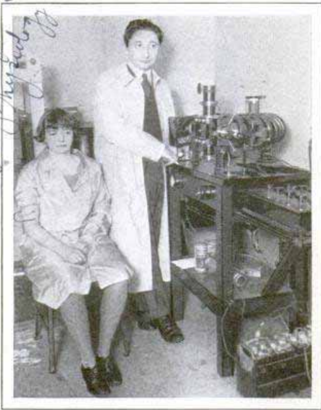
Subject Undergoing Test with Galvanometer, so Sensitive It Records One-Millionth Volt of Electricity
