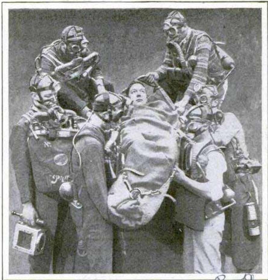
Rope-Stretcher Sled Which Has Demonstrated Its Usefulness in Carrying or Pulling the Victims of Mine Disasters to the Surface
