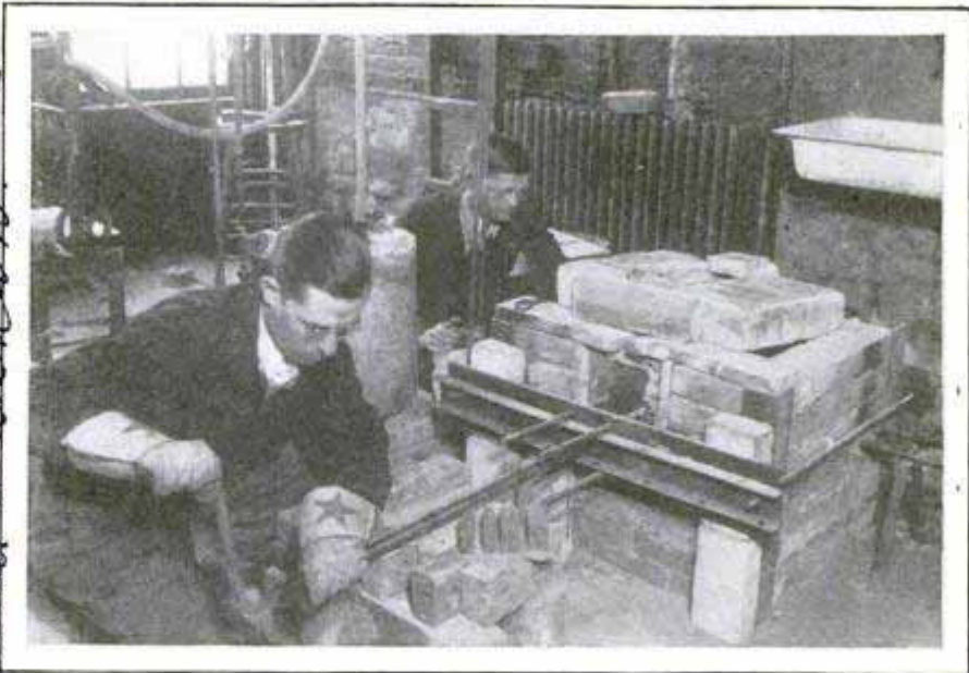
Preparing the Bricks in Experimental Furnace; Samples of the Product Are Seen in Center Foreground
