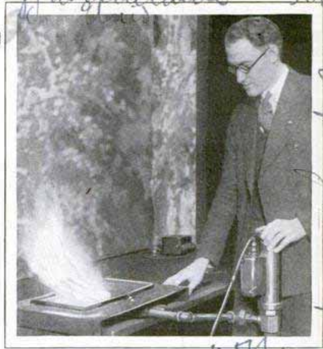
Using Electric Eye as Fire Extinguisher; the Sensitive Photoelectric Cell Detects the Smoke
