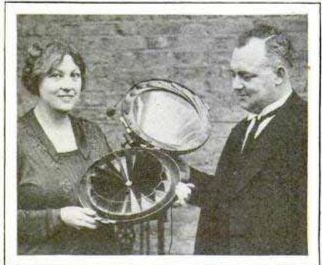
Anti-Glare Auto-Light Shutter in Open and Closed Positions; It Operates from Steering Wheel
