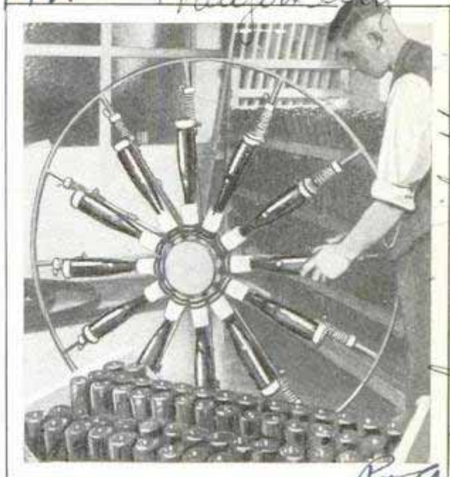
Bottling Machine Which Fills Containers with Fresh Liquid Fruits for Future Consumption
