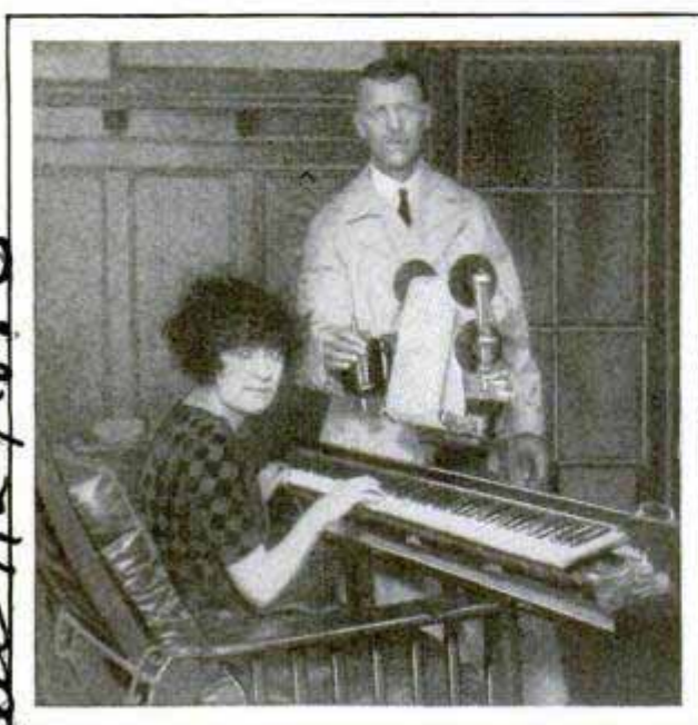
Superimposed Keyboard for Transposing Music, and a Music Writer for Recording Improvisations
