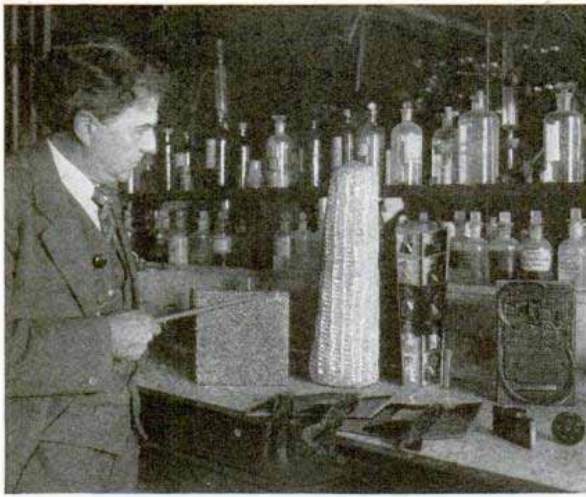
Samples of By-Products Made from Corncobs, Including Insulating Material, Furfural, Lignin, Ethyl, Alcohol, Cellulose and Oxylose
