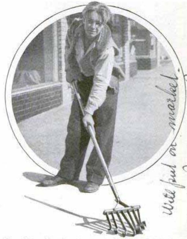
Gang-Plow Hoe for the Truck Garden, Which Cultivates and Weeds in the Same Operation
