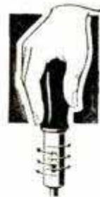
Working on ratchet, the handle moves to and fro with your hand. Finger-touch gives right or left ratchet, for driving or drawing screws; or makes it a rigid driver.
