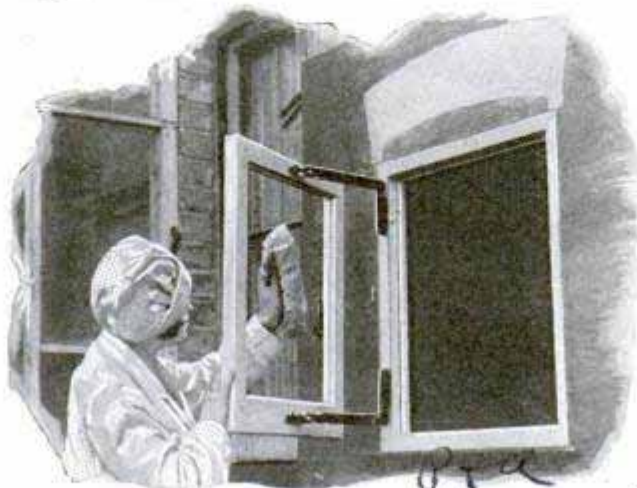
Reversible Casement Window Which Is Easily Cleaned
