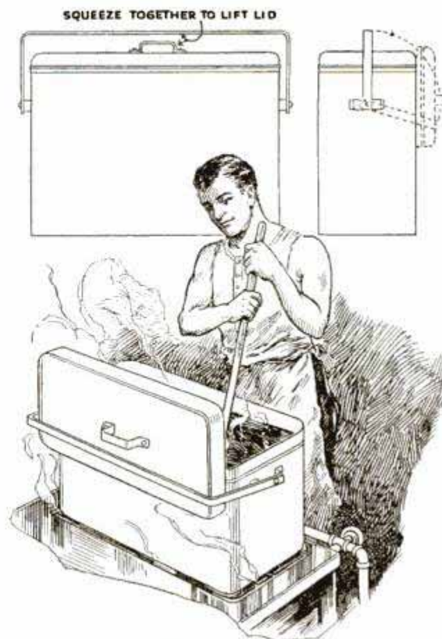
Rod Attached to Wash Boiler Helps to Remove Lid and Serves as a Holder for It
