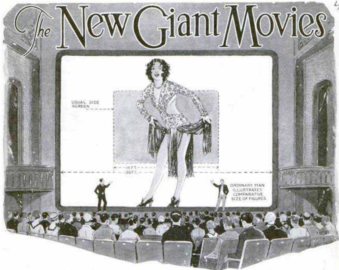
Artist's Drawing of "Magnafilm," as Presented at the Pantheon Theater in Chicago; the Effect Is Produced by Magnifying Standard Thirty-Five Millimeter Film through Lenses in the Projector
