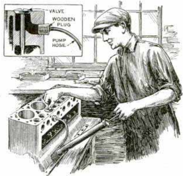
Air Pressure Applied to Valve Port Shows Whether Valves Are Leaky
