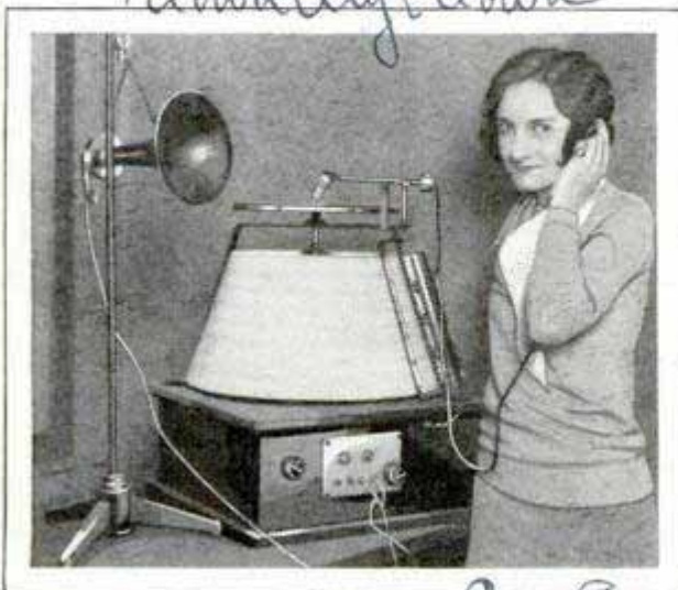
Instrument Which Tests a Singer's Voice by Registering Tone Waves as They Are Produced
