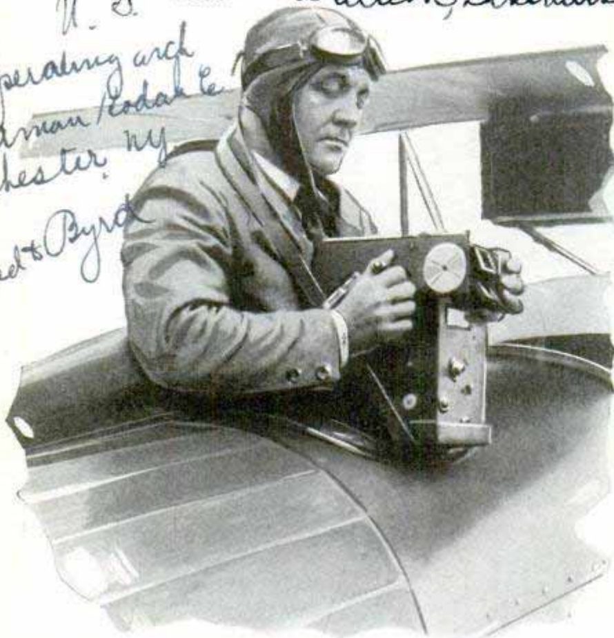
Sextant Camera That Photographs a Complete Reading of the Sun to Show the Observer's Exact Position; This Instrument Has Been a Great Aid to the Byrd Expedition
