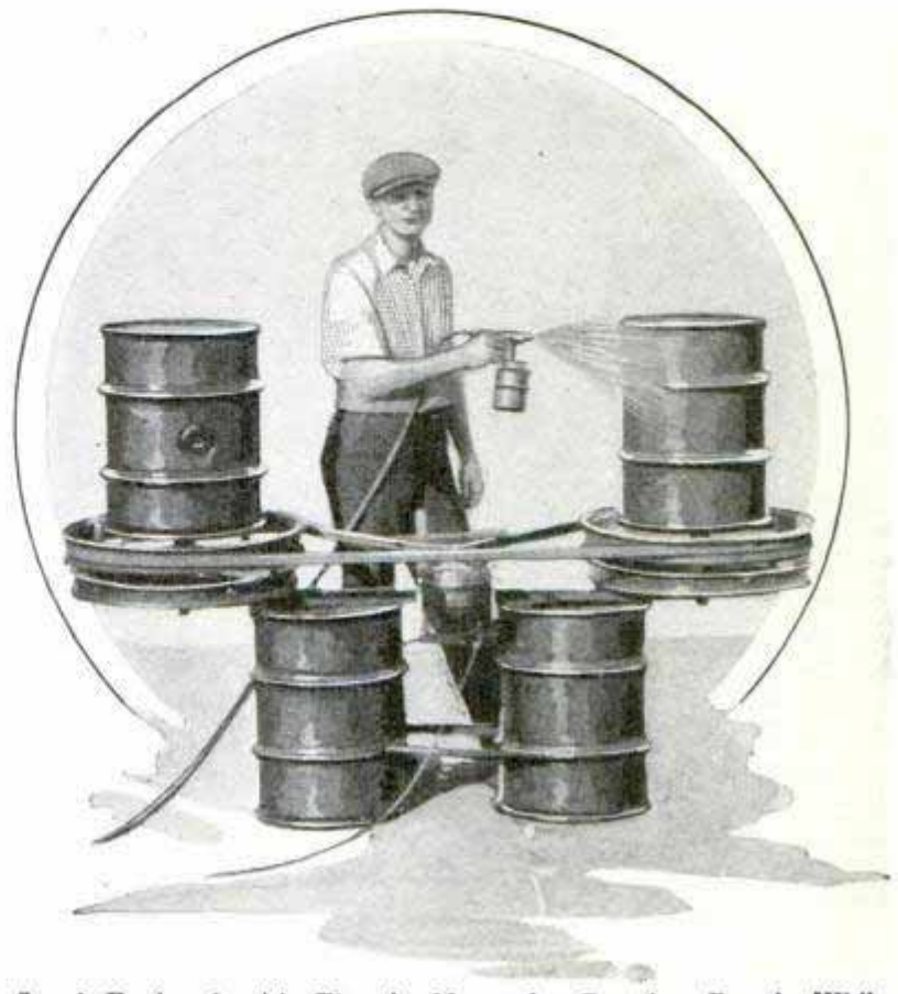
Stand Equipped with Electric Motor for Rotating Barrels While Spray-Painting Them
