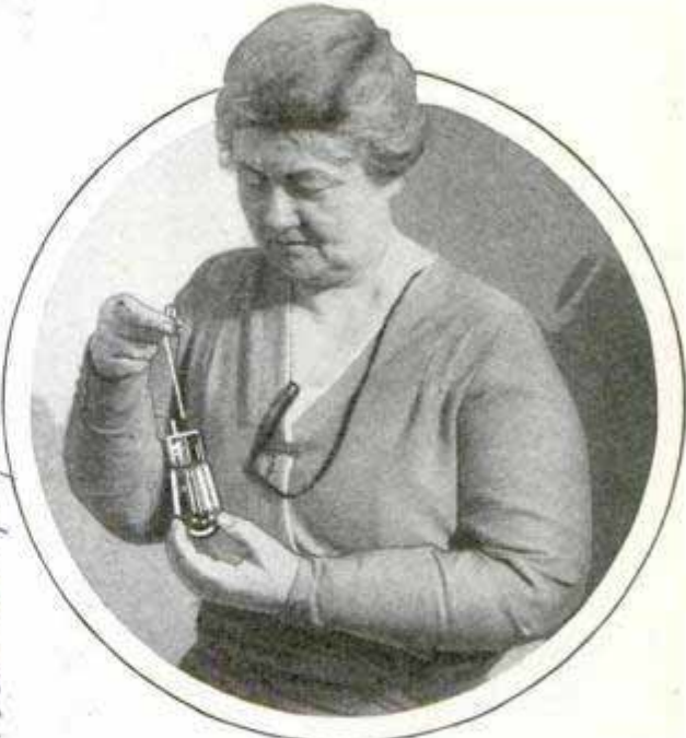
Radio Tube with Removable Heating Element, Which May Be Replaced When a Tube Fails
