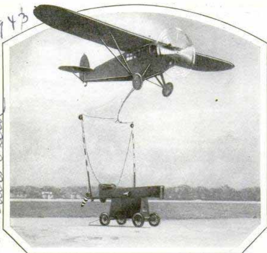
Mail Plane with Hook Attachment, Snatching Mail from Truck by Hooking Line between Upright Posts to Which Bag Is Fastened
