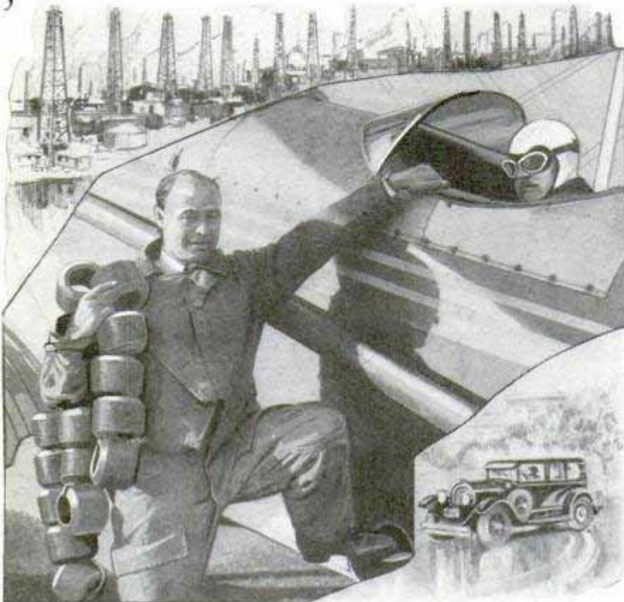
Rubber "Doughnuts" Which Eliminate Friction between Casing and Tools in Drilling Oil Wells; a Spinning Auto Tire Furnished the Idea
