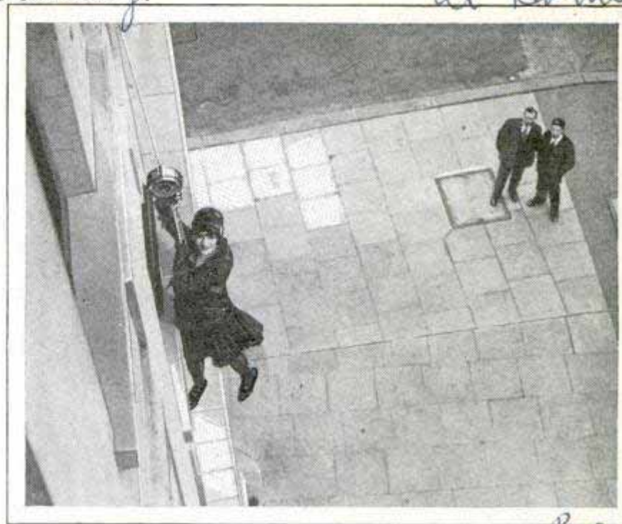
Self-Operated Lifeline to Escape from Fire, the Person Clinging to the Line Governing the Speed of Descent to the Ground
