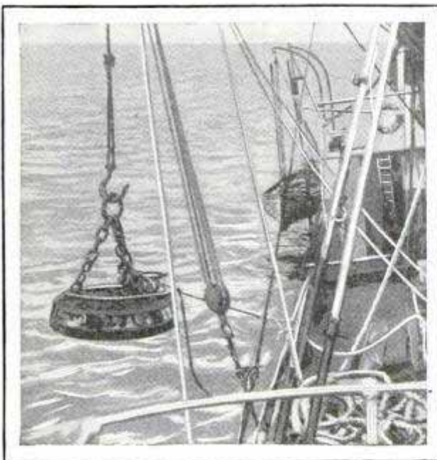
Electromagnet Able to Raise Many Tons, Employed in the Salvaging of Sunken Treasure Ships
