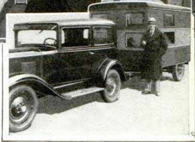
Auto Trailer Which at Night May Be Expanded to Provide Sleeping Quarters for Four Persons
