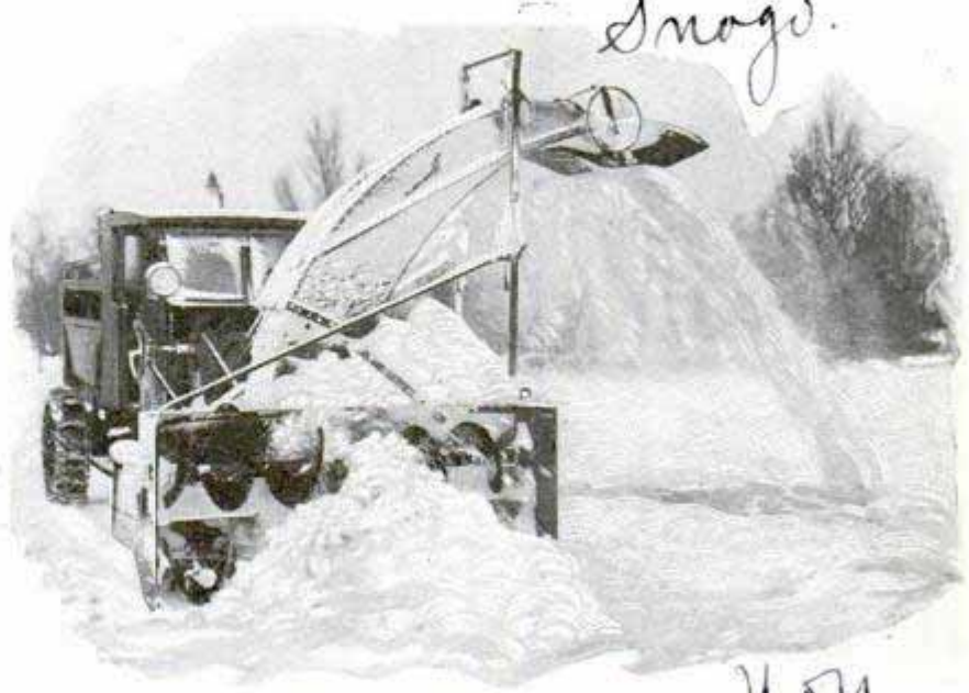
Rotary Plow That Eats Up a Snow Bank at Twenty Miles an Hour, Picking Up the Snow and Tossing It Far beyond the Curbing
