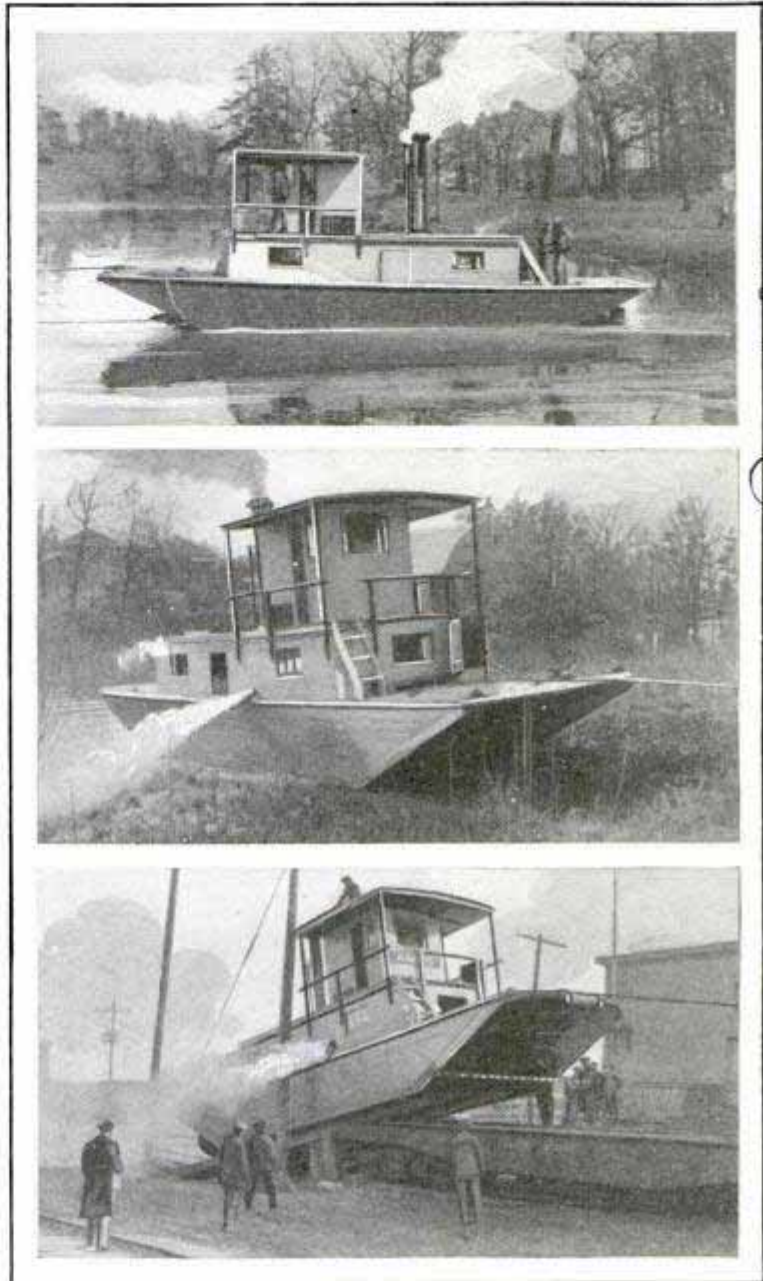
"Alligator" Boat That Navigates Land as Well as Water by a System of Skids and Cables Attached to It
