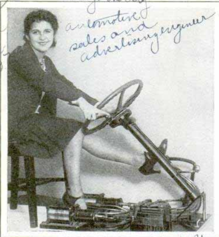
Vacuum Gear Shift for Auto Is Operated by a Throttle on the Wheel Instead of by a Lever
