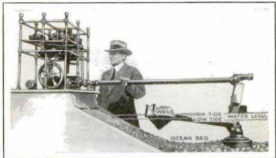
Model of Ocean-Wave Motor Intended to Convert Wave Energy into Electric Power for Commercial Purposes
