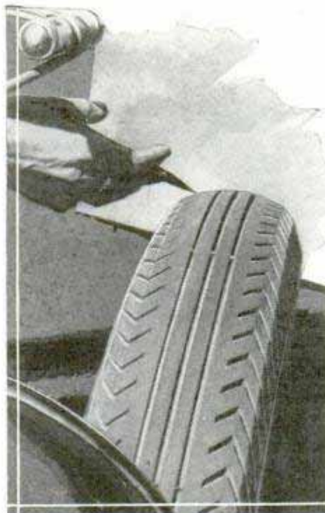
Uneven Wear on Front Tire Due to Insufficient Camber of Wheel
