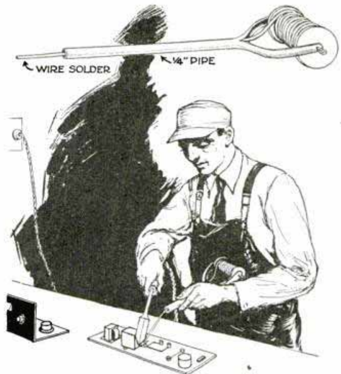
Handle for Wire Solder Is Made of Pipe, and Remains Cool While Soldering
