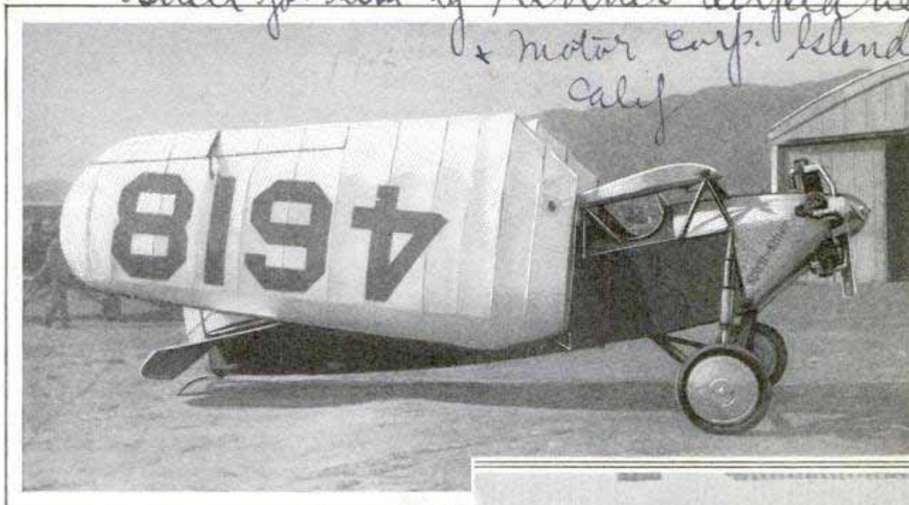
Monoplane Whose Wings Can Be Folded for Parking in a Garage; Below, Rear View with Wings Folded
