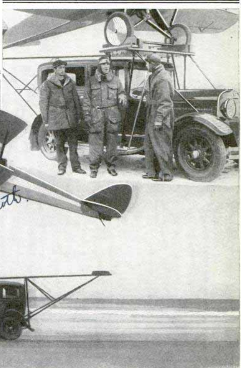
Upper Right, Airplane Resting on Frame on Top of Automobile from Which It Hopped, as Shown Below, When the Car Had Attained a Speed of Fifty-Two Miles an Hour
