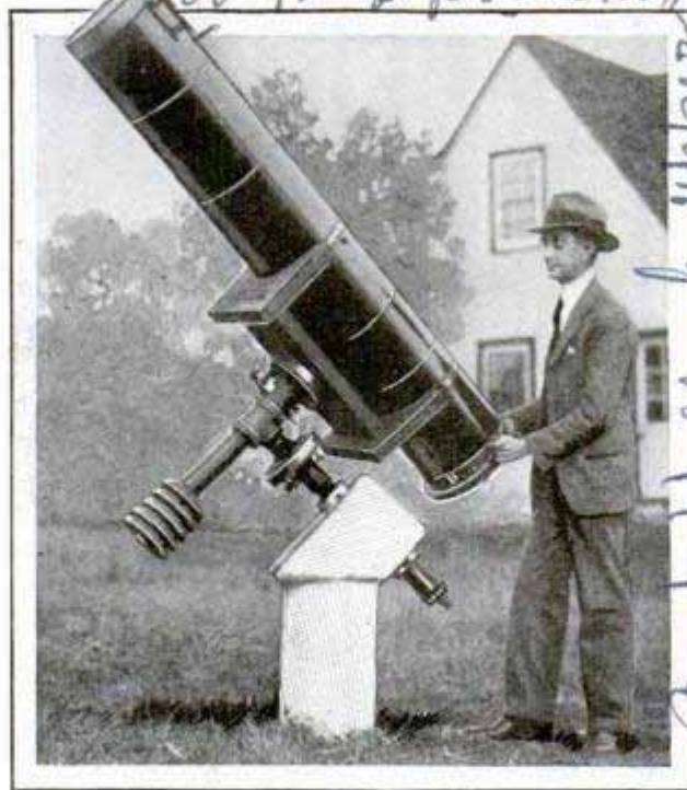
Homemade Telescope Constructed of Part of an Automobile Axle and Galvanized Sheet Iron
