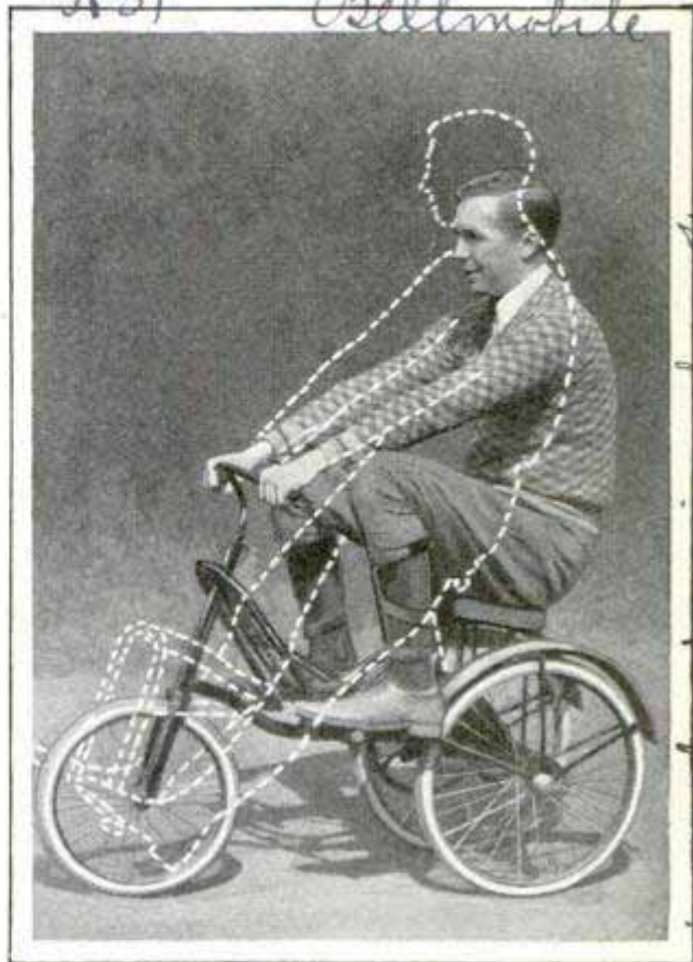
Exercising Machine, Resembling a Tricycle, Which Gives Effect of Rowing When Propelled
