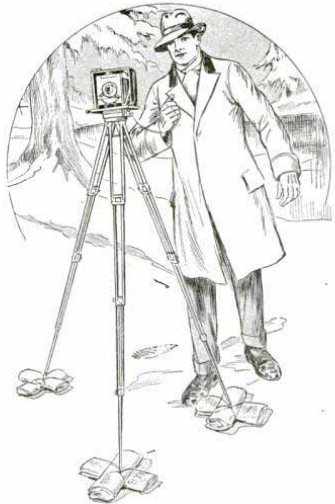
Satisfactory Support for the Camera Tripod on Snow Is Provided with Newspapers
