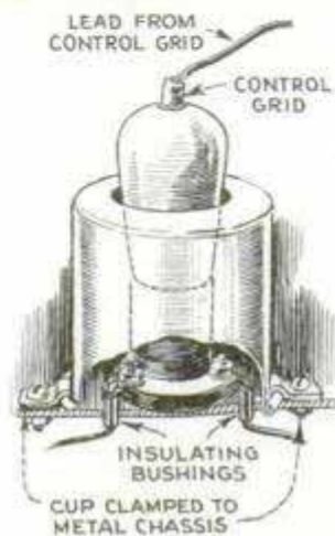
Left, for a Good Antenna Joint, Wrap Lead-In Wire as Shown, Leaving 2 In. Parallel to Horizontal Wire and Solder Together; Right, Aluminum Drinking Cup Makes Good Tube Shield
