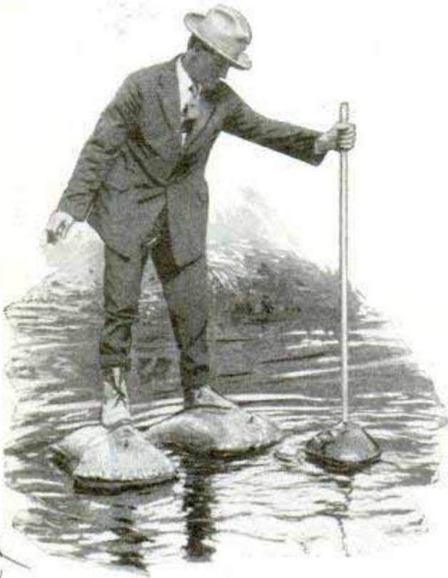
Shoes Attached to Inflated Cushions and an Inflated Staff Form Water-Walking Apparatus
