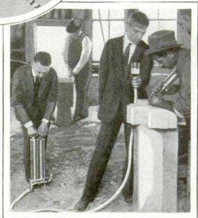
Direct-Vision Dust Counter; Dust Particles Magnified 100 Diameters, and Measuring Dustiness in Stone-Cutting Plant
