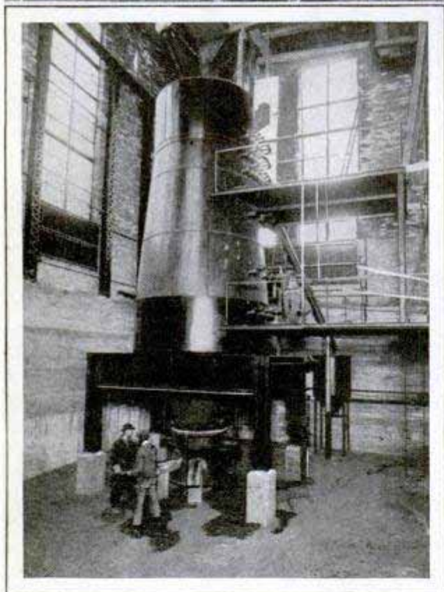
Mining Coal with the Latest Electrical Diggers, and Experimental Blast Furnace at the Bureau of Mines
