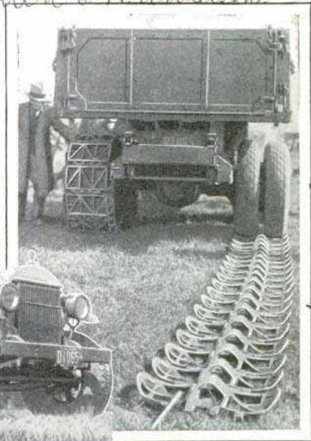
A Heavy-Duty Truck with Two Sets of Rear Wheels Transformed into a Tractor for Rough Traveling by Adding Chain Treads, Allowing the Wheels to Travel on a Track
