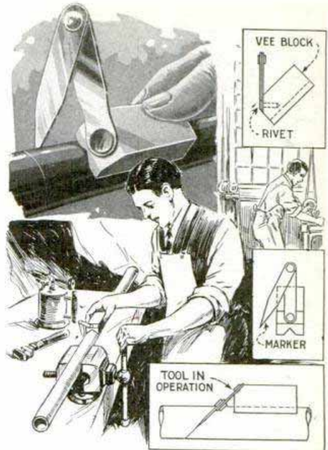
Block with Two Pivoted Arms Marks Pipes at 45-Degree Angle
