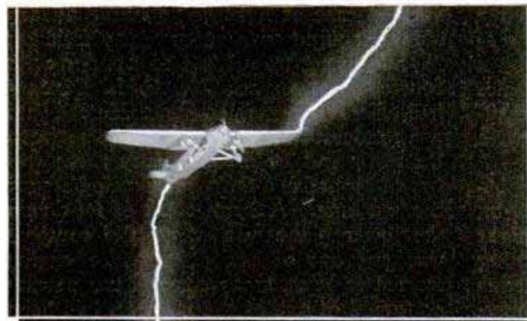
Remarkable Night Photos of Model Metal Plane Being Struck by Artificial Lightning Bolts; Note How the Charges Always Enter and Pass Out at the Tips
