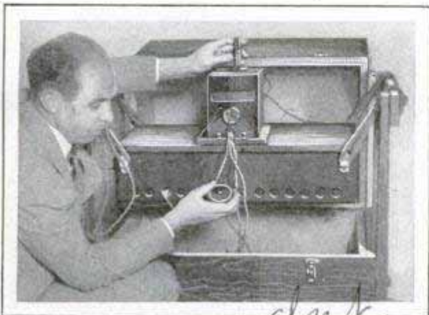
Hunting for a Sound Whose Echo Will Indicate a Plane's Actual Height above the Ground
