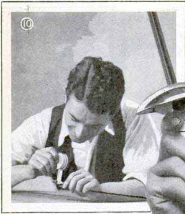
Fig 10, Fitting the Tip, a Rubber Eraser, to the Foil with Glue and Tape; Fig. 11, Showing the Handle Wrapping and Also How the Foil Should Be Held
