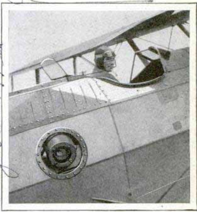
Courtesy Army Air Corps Special Mounting for an Aerial Camera, Which Enables a Pilot to Snap His Own Pictures
