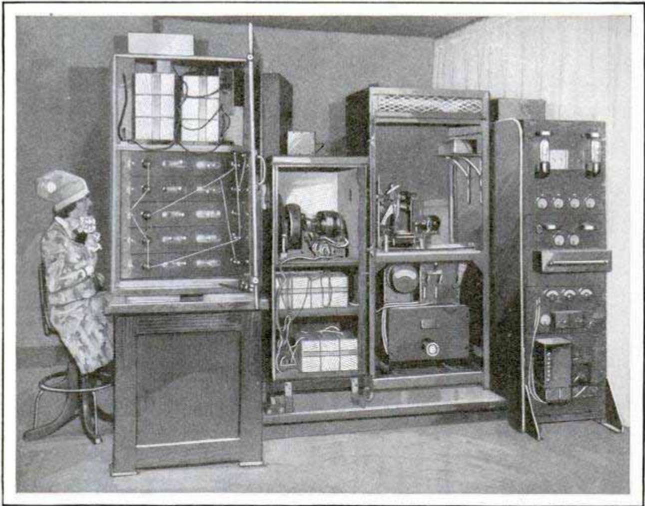
Side View of Sending Apparatus, Which Constitutes the Mechanical Telephone Operator; Except for the Photoelectric Cell at Left, It Is Similar to Ordinary Television Equipment
