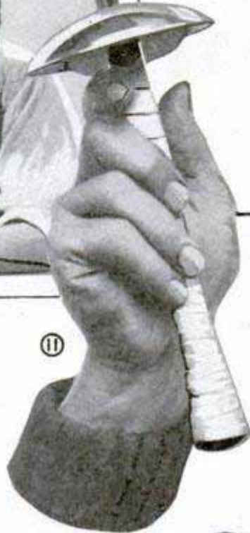
Fig 10, Fitting the Tip, a Rubber Eraser, to the Foil with Glue and Tape; Fig. 11, Showing the Handle Wrapping and Also How the Foil Should Be Held
