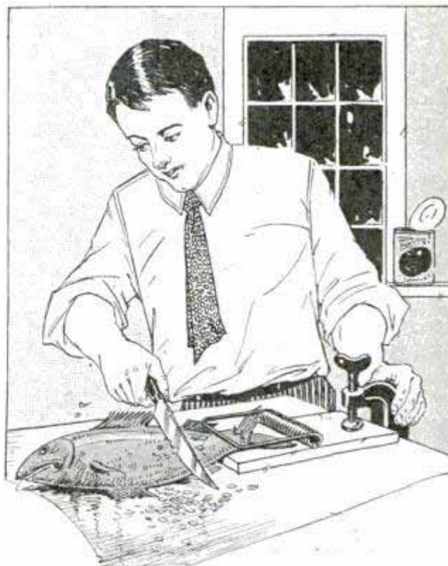
Ordinary C-Clamp and Mousetrap Arranged to Hold Fish Securely While Scaling Them
