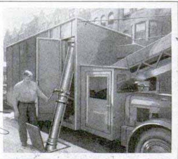
Ash Cans Are Being Replaced by This Truck, Which Sucks the Ashes through Pneumatic Tubes
