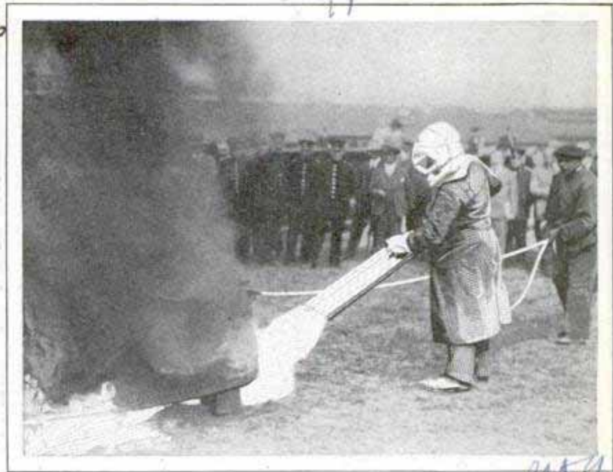
Extinguishing a Fire with Powder under Pressure; This Method Eliminates Danger of Damage by Water or Chemicals
