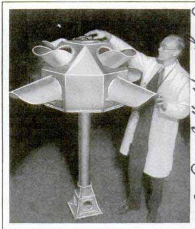
Model of Traffic Signal for Planes: When Downward Lights Are Green, Opposite Ones Are Red
