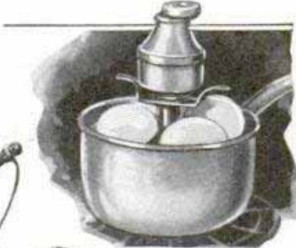
Boiling Eggs Exactly the Desired Time Is Easy in This Aluminum Kettle; a Simple Device at Top Is Set, and at the End of the Period, the Eggs Automatically Are Lifted Out of the Water
