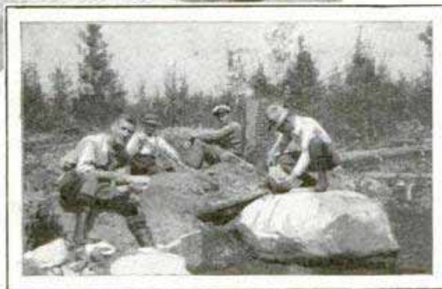
Examining Rock Specimens from a Trench Cut across the Face of a Silver Vein, at Lorrain, Northern Ontario
