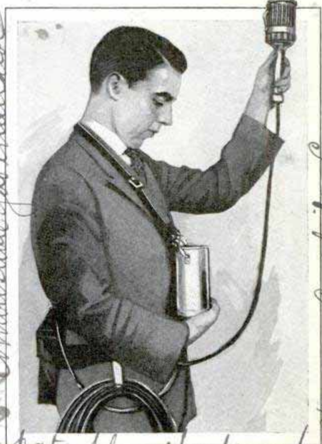
This Apparatus Detects the Amount of Combustible Gases in the Air of Mines and Factories
