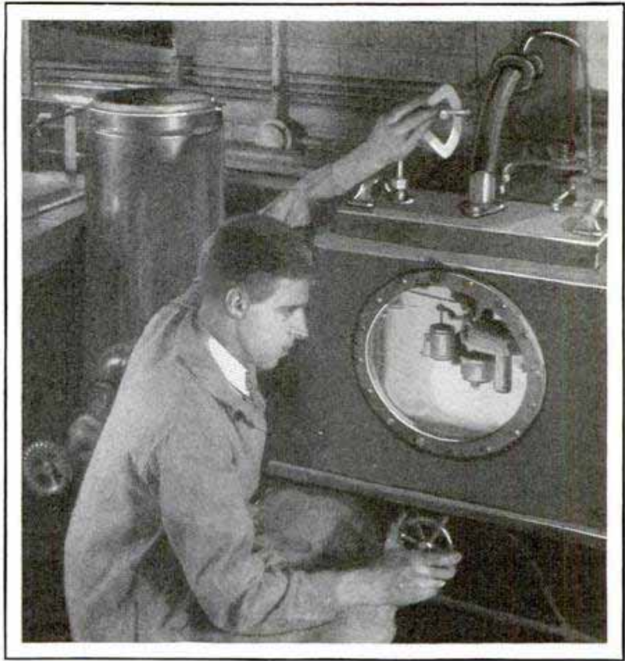
Determining Exact Carburetor Performance by Placing It in a Mercury-Sealed Box and Observing Data from Instruments
