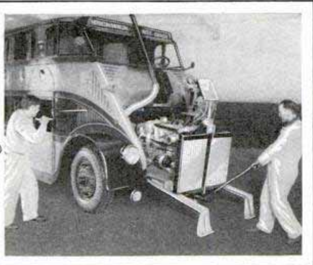
Motor Coach with Detachable Engine, the Motor Being Changed at Division Headquarters
