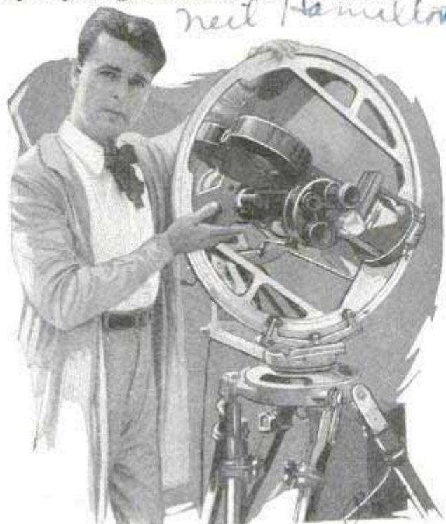
A Motion-Picture Camera That May Be Revolved to Shoot from Any Position or Angle
