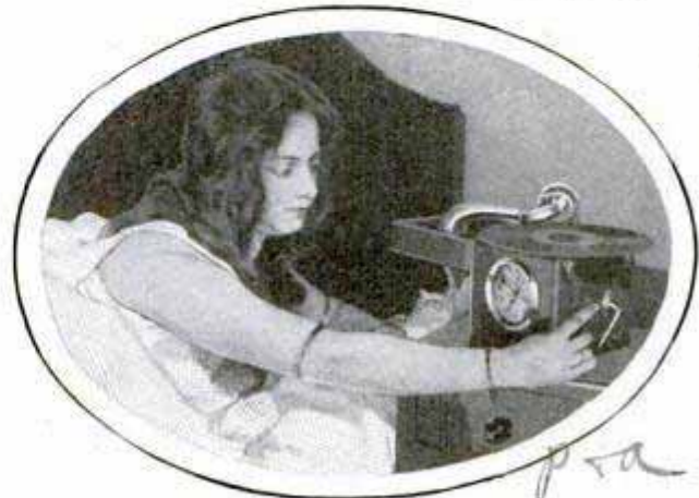
Alarm Clock Attached to a Phonograph Awakens You with Your Favorite Record
