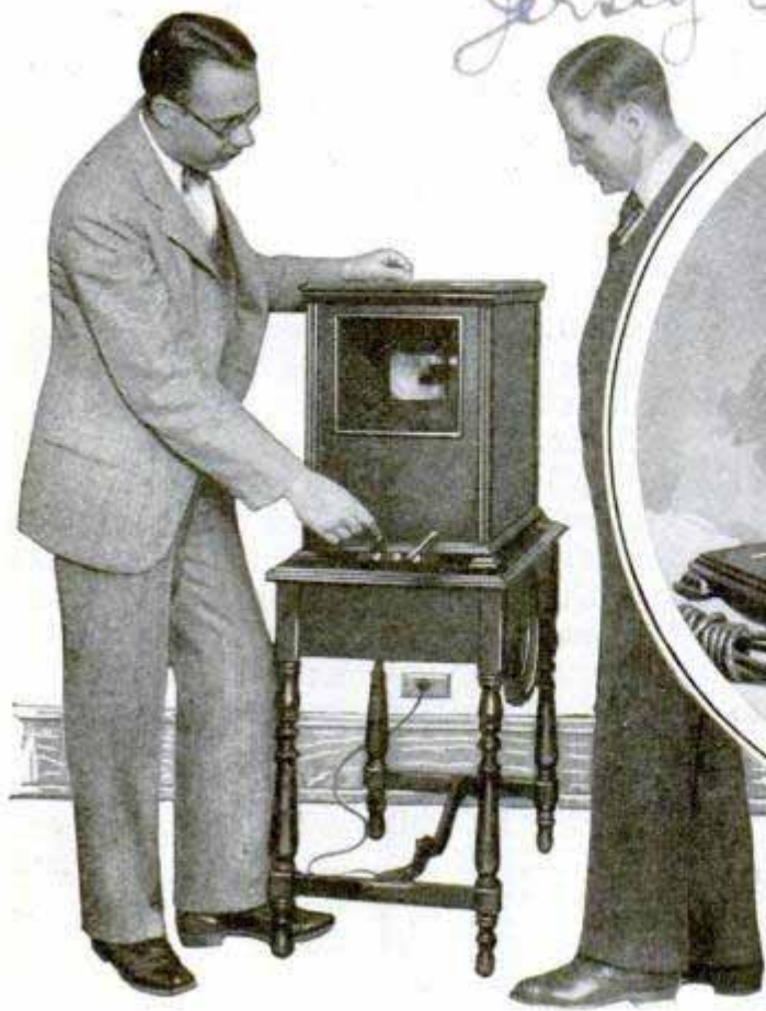
Televisor for Home Use, Showing the Toggle Switches and Framing Crank; Above, the Instrument Removed from the Cabinet, Showing the Simple Mechanism for Rotating the Entire Motor and Scanning Drum to Bring the Pictures in Phase with the Signals
