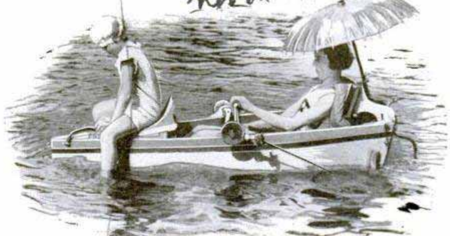
A Rowboat without Oars, Run by Turning the Cranks in Front of the Passenger, Thus Revolving Two Propellers in the Rear
