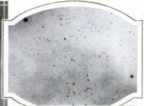
Profusion of Air Bubbles Reveals That This Is a Synthetic Sapphire
