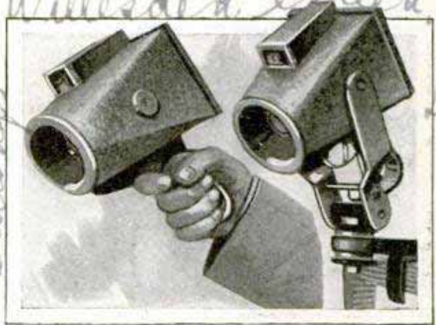
One Hand Only Is Required to Operate This Aerial Camera with Its Pistol Grip and Trigger
