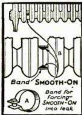
Leak at radiator joint stopped with Smooth-On
