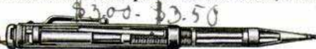
Sectional View of the "Magazine" Pencil That Holds Leads of Different Colors
