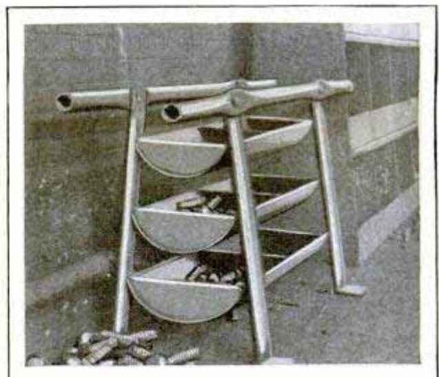
Rack of Sheet-Metal Trays on Pipe Frame Used for Holding Bolts in Machine Shop
