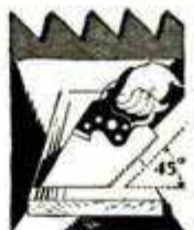
Teeth of cross-cut saw and proper sawing angle
