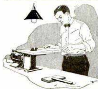
Fig. 1 Shows the Three Parts of Setter Used for Circular Saws; Photos Show, Left, Holder for Saws While Filing; Right, a Setter in Use
