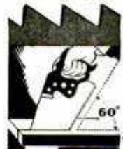
Teeth of rip saw and proper sawing angle
