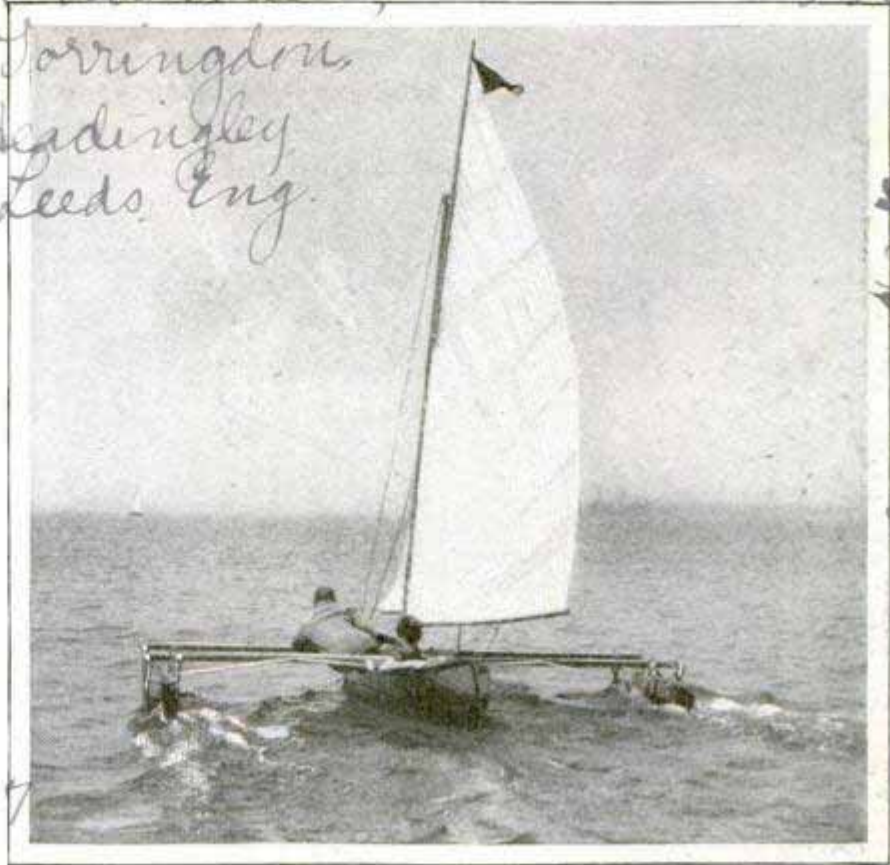
A Canoe Made into a Sailboat by Adding Outrigger Beams and Stabilizers; an Engine Also May Be Attached
