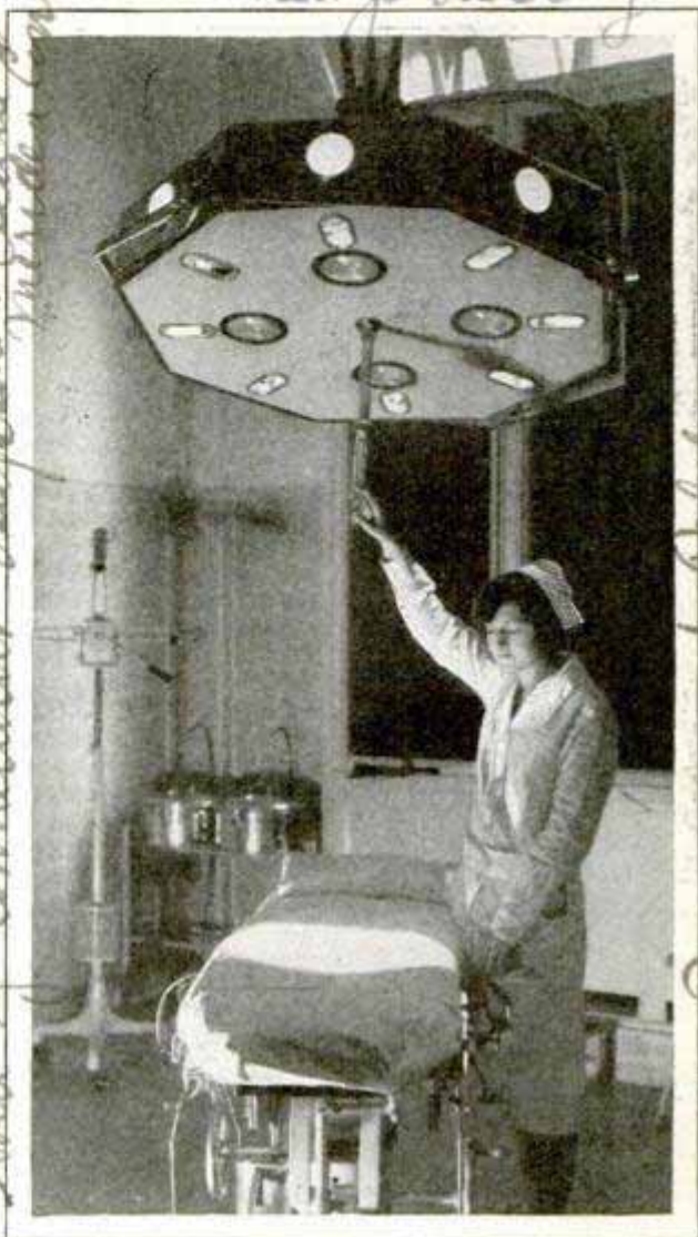
A Shadowless Light for the Operating Table Formed by Focusing Eight Beams from Various Angles
