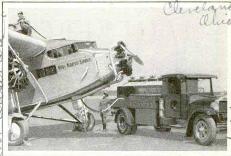
Servicing Tri-Motor Plane from the Special Truck Equipped with Electric Pump and Air Compressor for Inflating Tires
