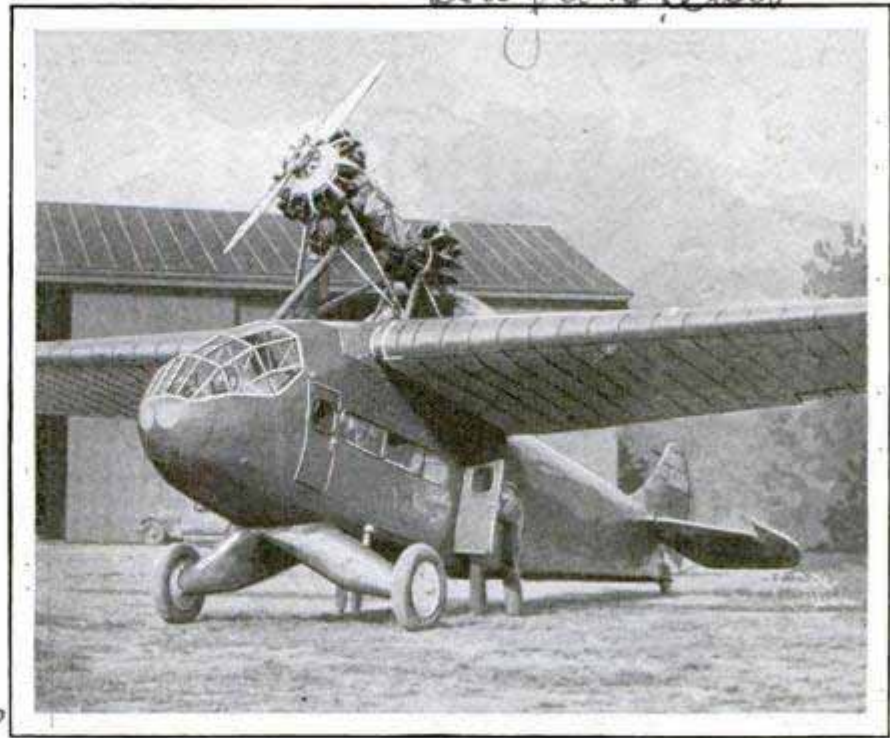
Tandem Motors on This Plane Are Mounted above the Wings to Give an Unobstructed View and Add to the Power
