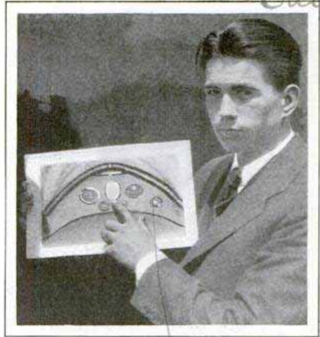
The Instrument Indicated Is an "Hourometer," Which Shows a Plane's Actual Time in the Air
