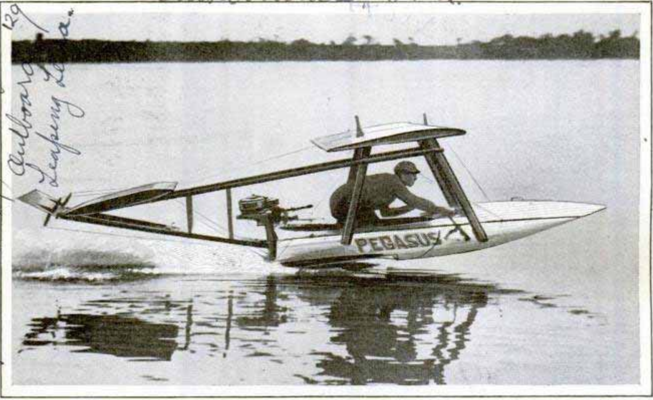
Motorboating and Flying Are Combined in This Racing Craft Equipped with an Outboard Motor Which at Times Causes the Craft to Leap into the Air and Fly Short Distances
