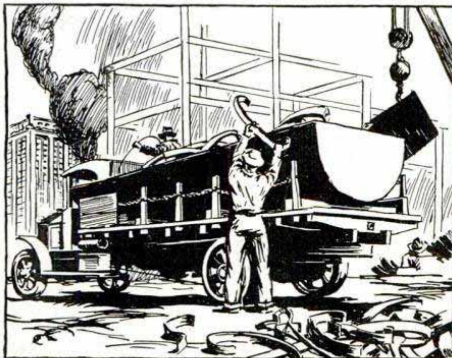
Useful Truck Body for Odd-Shaped Iron Pieces Can Be Made from Half of Discarded Tank
