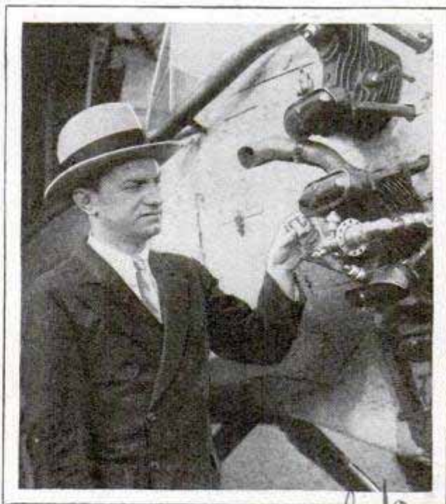
Here Is a Self-Starter for an Airplane, Using a Shotgun Shell to Supply the Force
