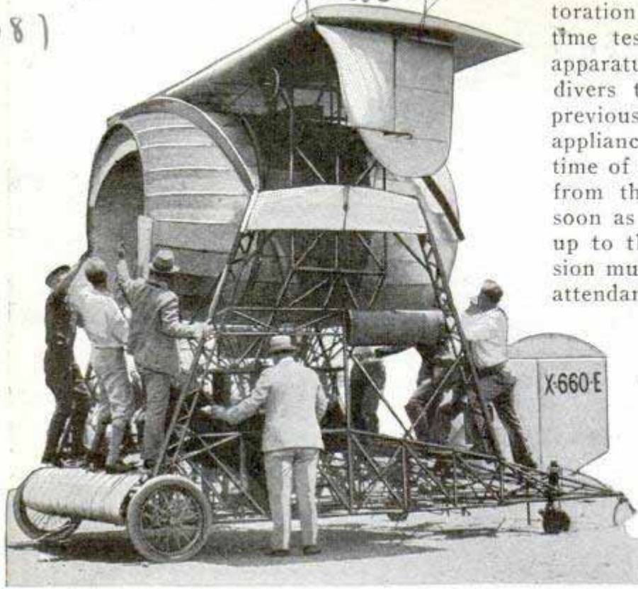
Contrasting in Appearance with the Ordinary Plane is This 'Ship' with a Flanged Cylinder for a Propeller
