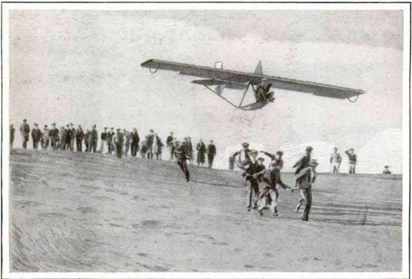
Vance Breese, San Francisco Aviator, at the Controls of a Ferguson Glider Which Is Being Launched by Men with Aid of Tow Rope, Dropped Free as Glider Rises
