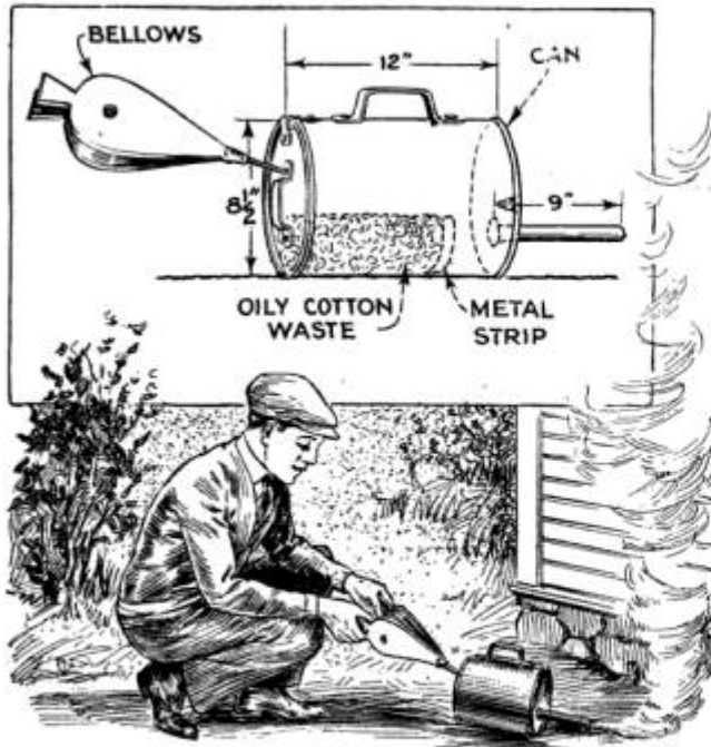
Simple Device for Gassing Rodents in Their Burrows Has Been Found Effective
