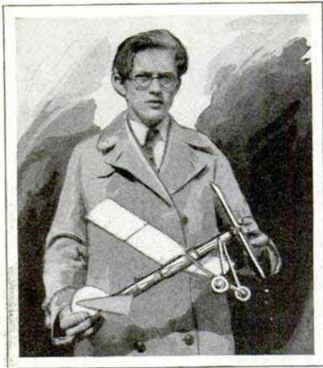
Cornstalk Fuselage for Model Airplane Is Strong and Durable
