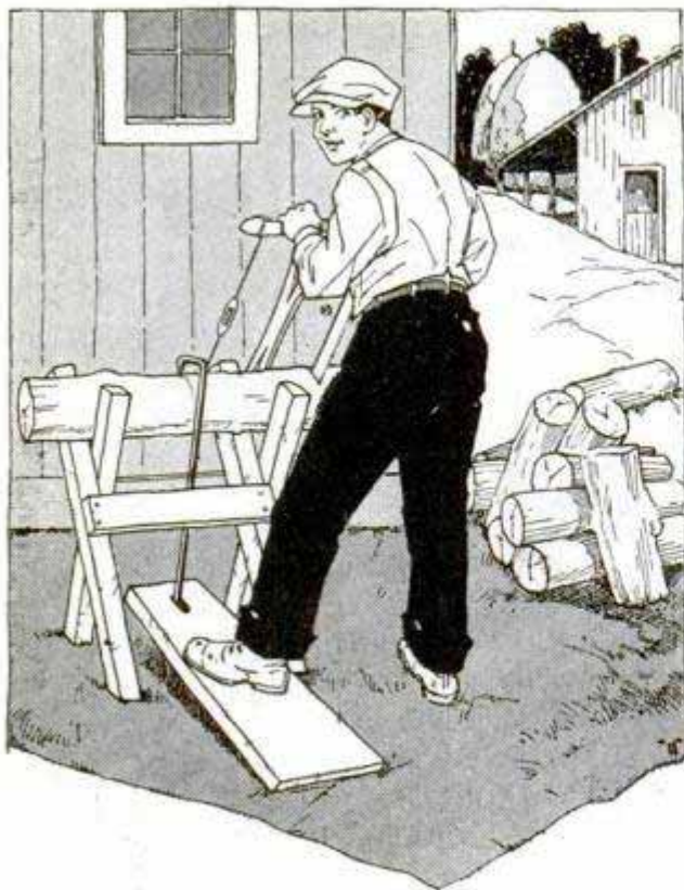
Footboard or Treadle with Pivoted Hook Holds Work Firmly in Sawbuck
