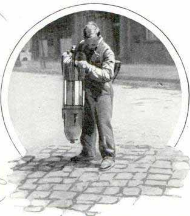
Machine for Tamping Paving Blocks Contains a Cylinder Like an Auto Motor, to Operate It
