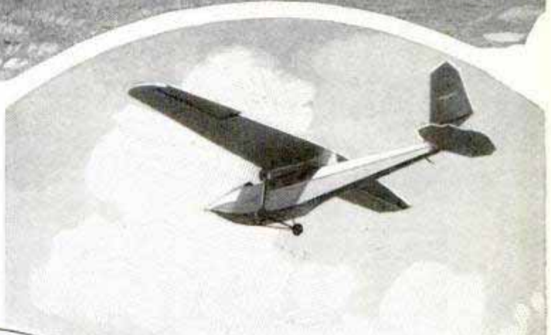
Drake in Glider Which Was Towed by Plane 200 Miles during Recent Exhibition by the Long Beach Glider Club; at Right, Glider, Designed by Hawley Bowlus of San Diego, in the Air; It Has a Wing Spread of Forty-Six Feet and Has Been Built to Enable the Pilot to Take Quick Advantage of Favorable Currents, Which Often Rise Several Times Higher than the Take-Off Hill
