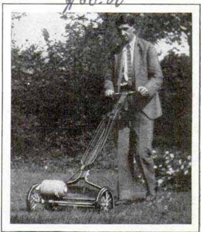
A Hand Lawn Mower with Electric Motor Eliminates Some of the Work of Cutting the Grass
