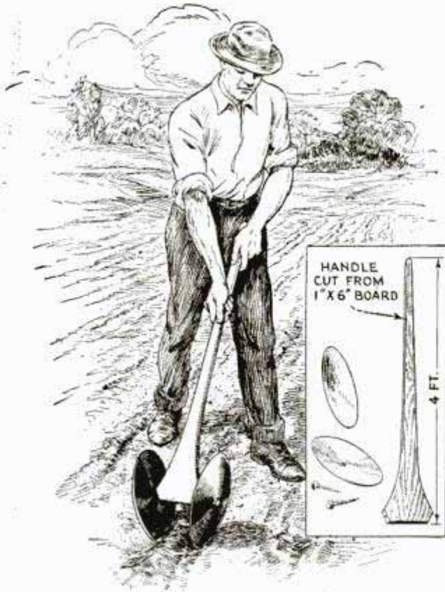
Two Harrow Disks on a Wooden Handle Make a Good Tool for Covering Freshly Seeded Rows
