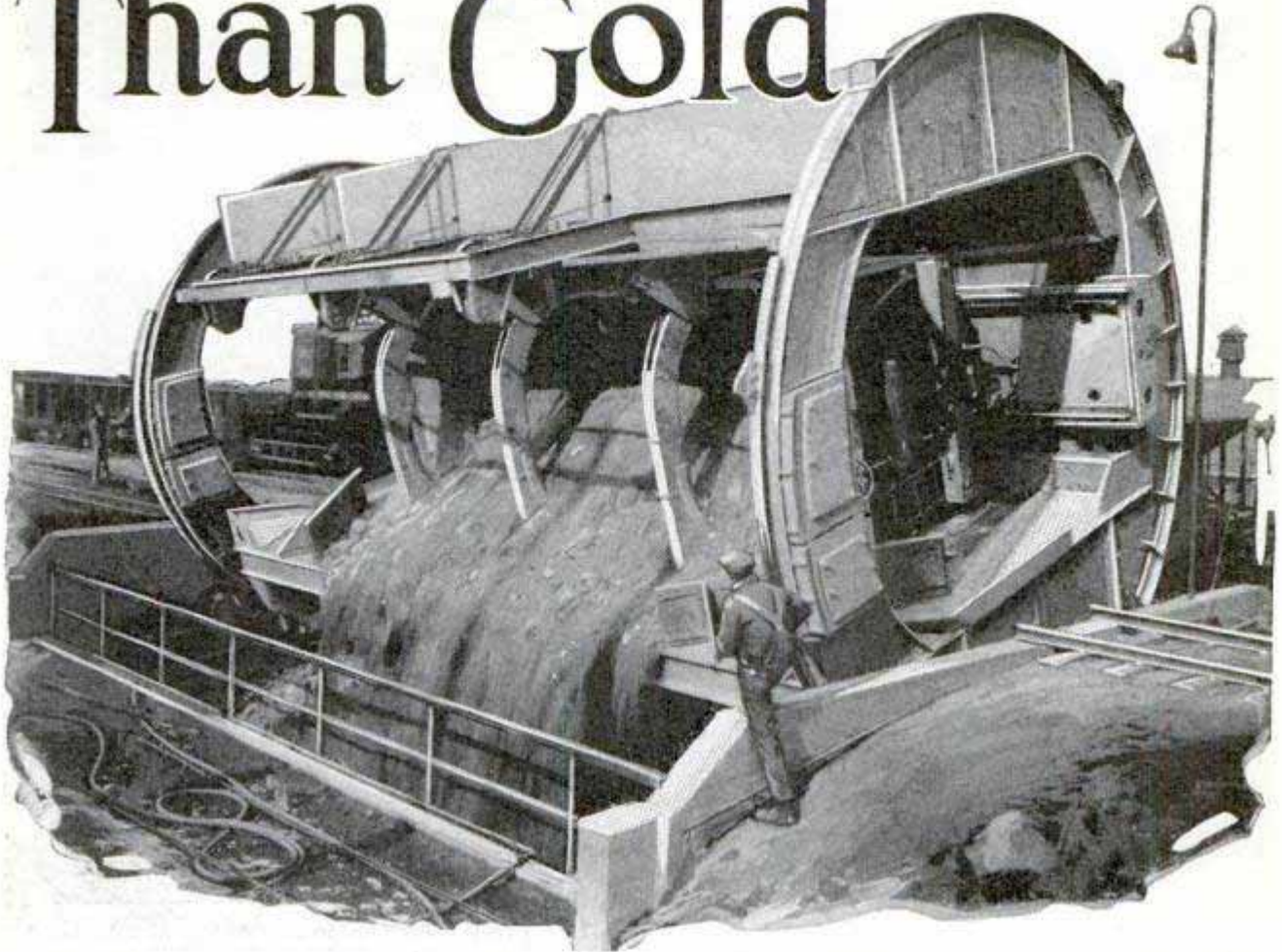
Rotary Car Dumper to Speed the Unloading of Ore; by This Method About Five Times as Much Material Can Be Handled in a Day as Was Possible with the Drop-Gate Cars
