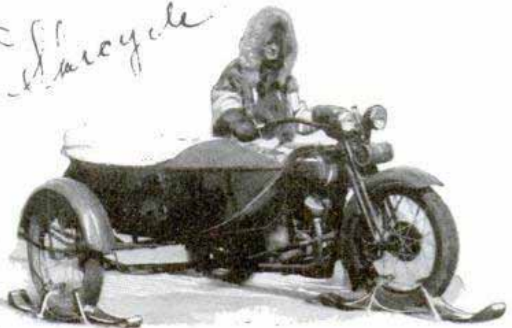
Alaskan Dog Teams Mushed for Three Weeks over a Trail Covered by This Motorcycle on Skis in Two Days
