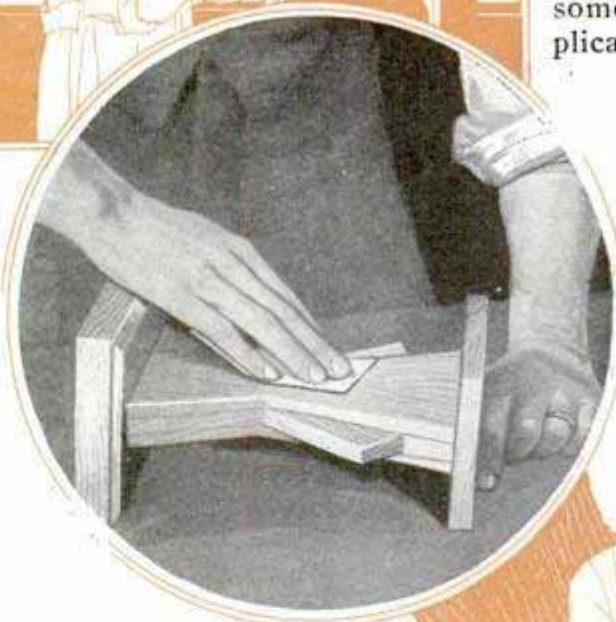
New Wood Must Be Sanded with the Grain to Make the Surface Ready for the Finish
