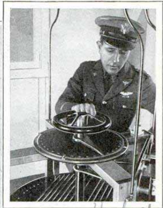
This Appliance, the Goniometer, Causes Directional Radio Signals to Be Sent to the Point toward Which the Arrow Points
