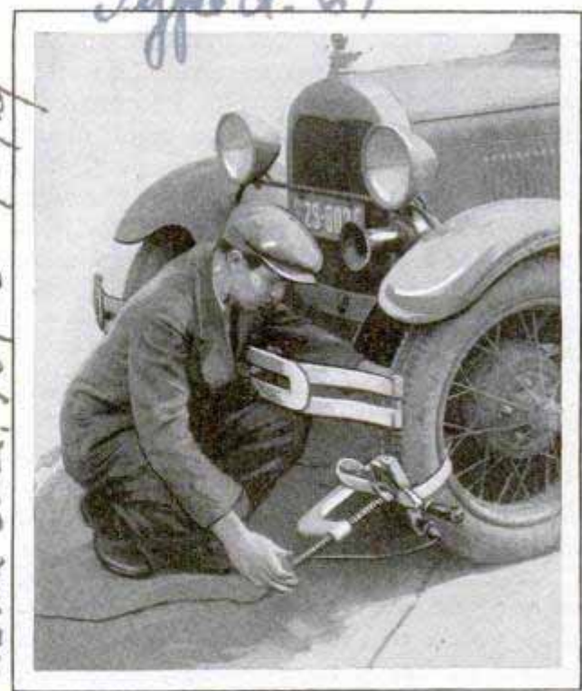
This Vulcanizer Repairs a Surface Cut without Removing or Deflating the Tire
