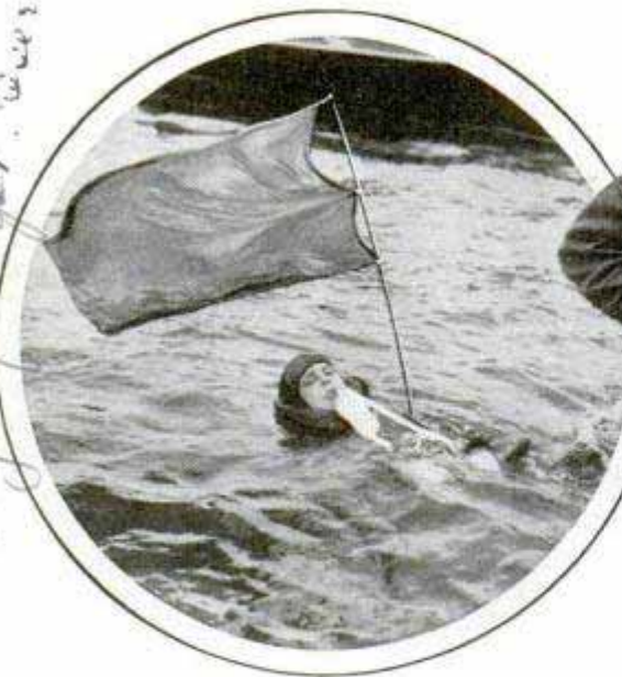
Non-Sinkable Suit Enabling Flyers to Remain Afloat Three Days; Oval Shows Suit in Use, with Flag to Attract Attention and Breath Condenser Supplying Drinking Water
