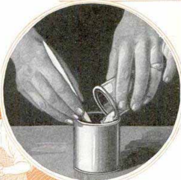
In Enameling New Wood, Some Turpentine Should Always Be Added to the First Coat, to Aid It in Penetrating the Wood
