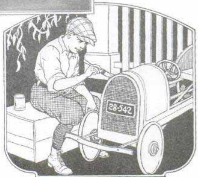
A First Coat of Shellac on Work to Be Lacquered Seals the Surface and Saves an Extra Coat of Lacquer
