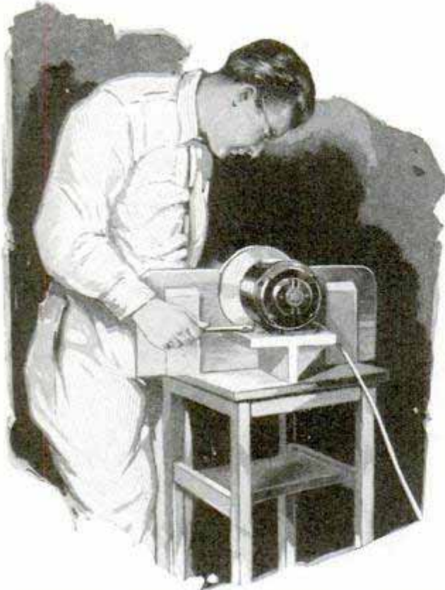
Adjusting the Sand Disk to the Fence or Guide by Shifting the Motor on the Table
