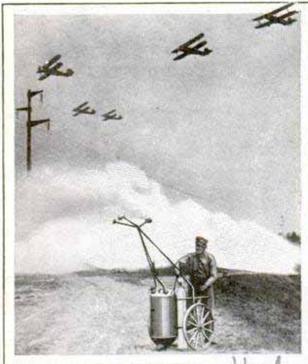
Operator Using a Smoke Tank to Conceal Important Buildings from View of Aerial Enemy
