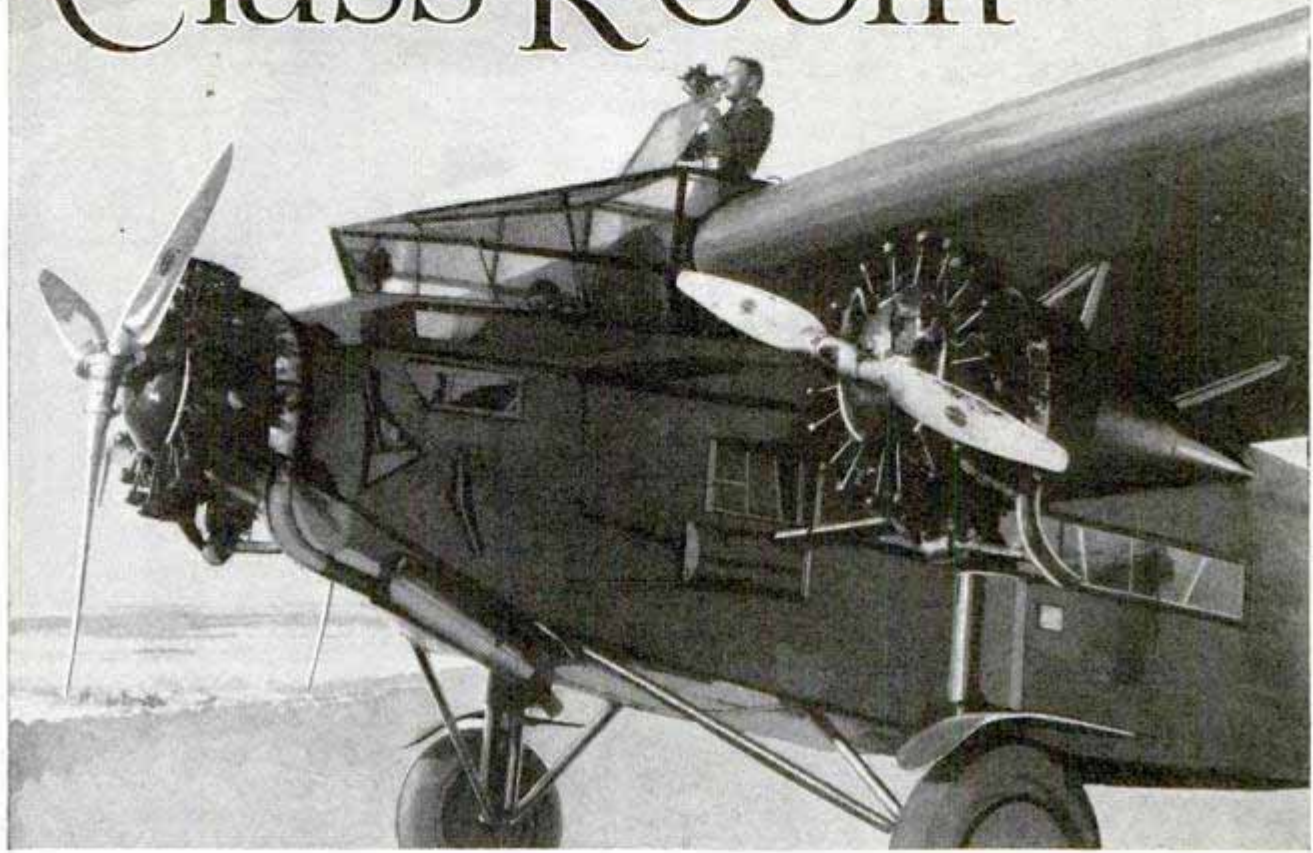
Through the Trapdoor on Top of the Navigation Ship's Forward Cockpit, the Observer Can Rise with His Instruments to Take the Plane's Bearings
