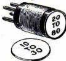
Left, a High-Resistance Unit, Provided with a Shunting Button and Designed for Controlling the Speed of a Television Motor, May Be Connected in One Side of the Line Supplying an Electric Soldering Iron to Prevent Overheating; for Quick Start, the Device May Be Turned On Full and the Button Pressed Down, after Which a Suitable Temperature May Be Maintained by Adjusting the Resistance; Right, a Drawing Triangle, Drilled and Cut to Be of Aid in the Drawing of Radio Circuits; Many Other Symbols besides Those Shown May Be Drawn by the Same Method
