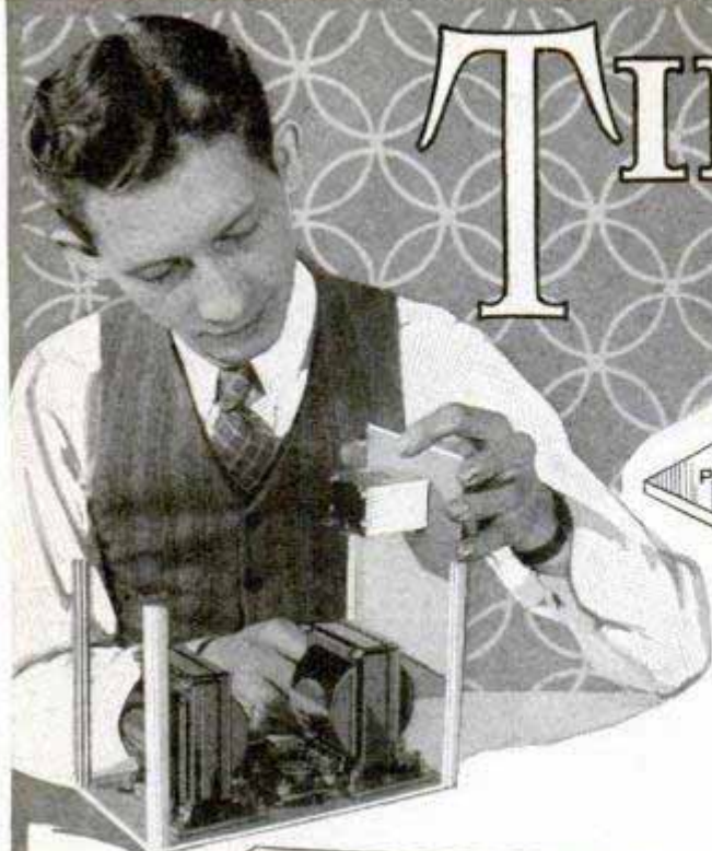
Left, Standard Aluminum Shield Employed to House a Push-Pull Stage Complete with Tubes, Resistors and By-Pass Condensers; Above, a Simple Method of Mounting Inductance Coils So That They May Be Turned at the Necessary Angle to Prevent Field Coupling
