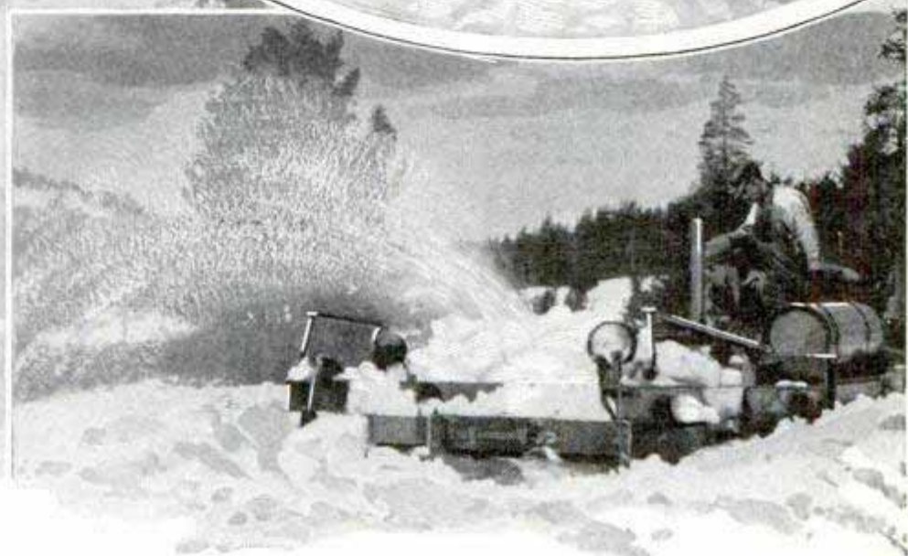
Rotary Snowplow Keeps Mountain Roads Clear; Left, a Road Freed of Snow; Upper Right, the Plow, Showing Large Blades, and, Below, the Machine Bucking a Drift
