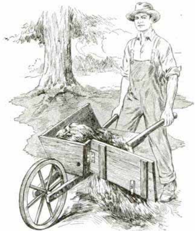
Hinged Side Boards on Wheelbarrow Permit Load to Be Dumped Quickly
