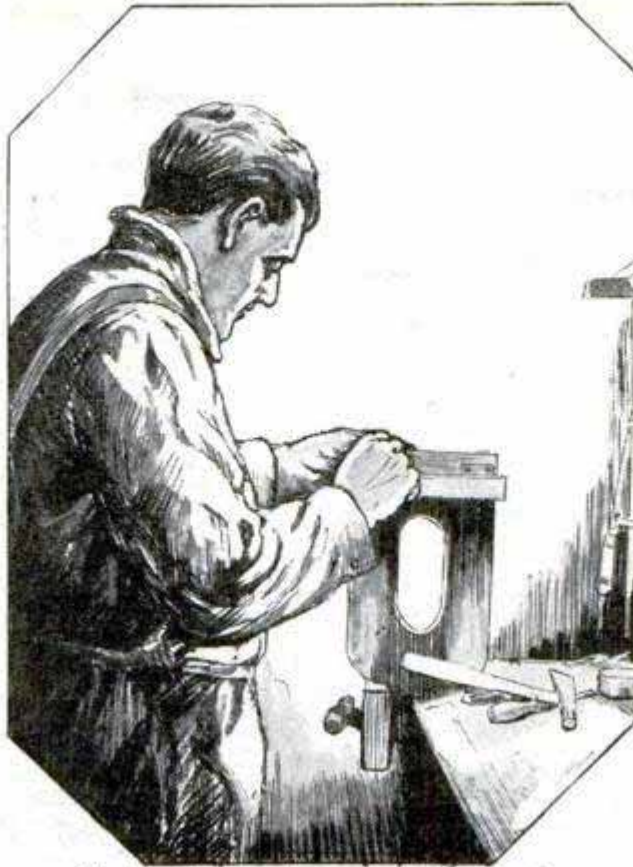
Hinging the Saw Support to Its Crosspiece
