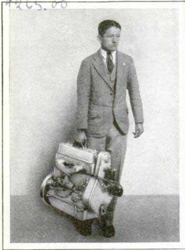
A Portable Four-Cycle Inboard Motor for Small Boats Weighs But 100 Pounds
