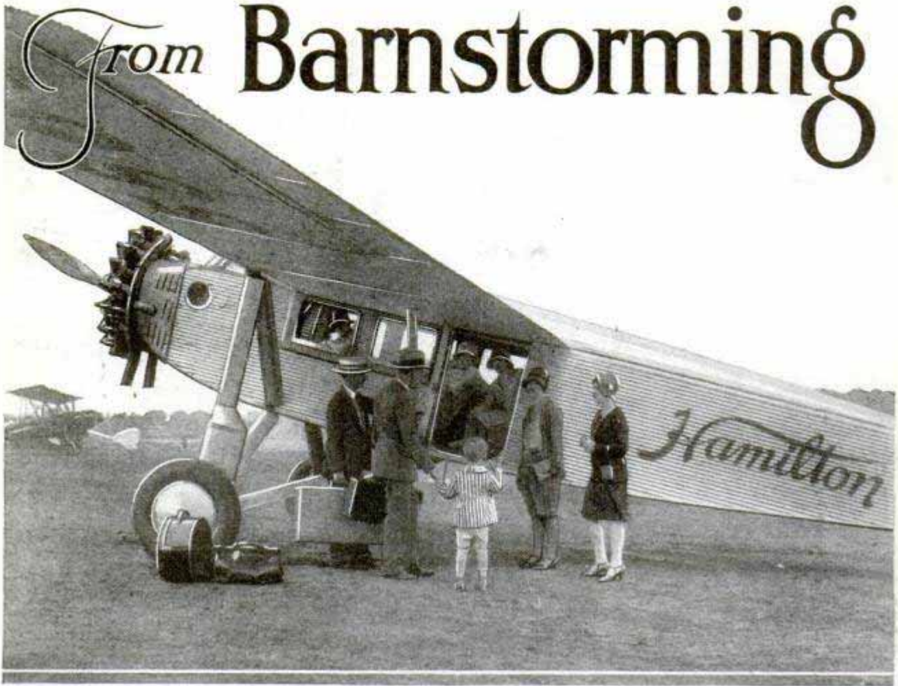
Loading Passengers into One of the Single-Engined All-Metal Planes Used by Northwest Airways on Its "Local" Run between Chicago and the Twin Cities of Minneapolis and St. Paul
