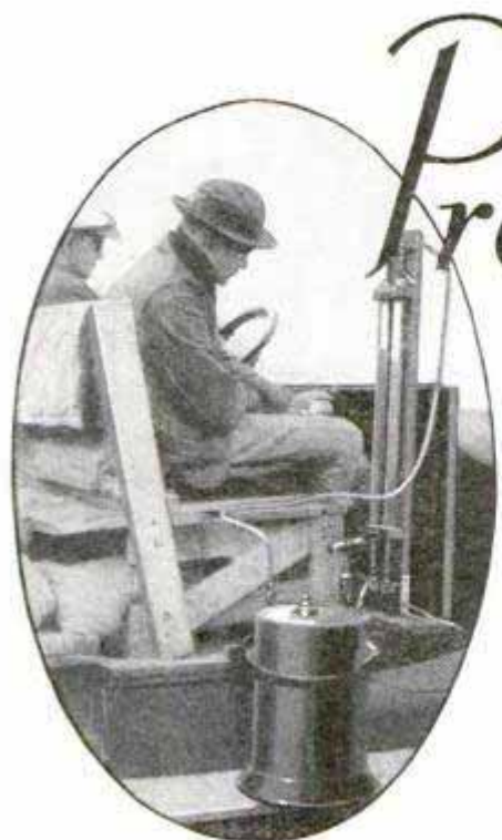
Device used at the Proving Ground for measuring gasoline economy. The gasoline consumed over any given distance is measured so carefully that the record can be read to a fraction of a drop.
