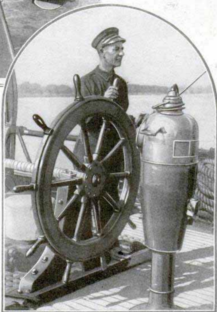
The Anchors, Top, Are of Bronze, and the Steering Wheel of Wood, to Avoid Magnetic Interference with the Ship's Work
