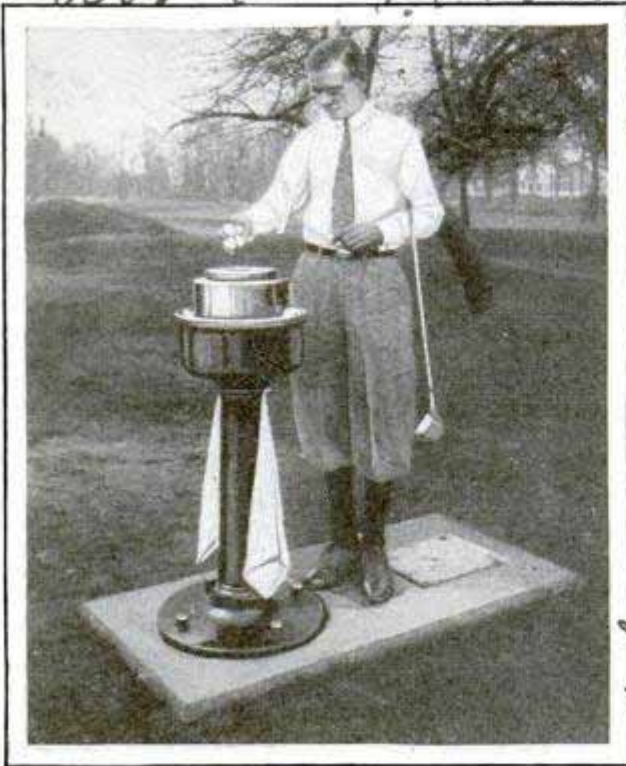
Reconditioning Golf Balls on the Links with the Aid of the Motor or Water-Driven Cleaner
