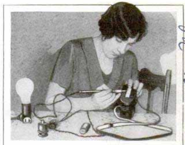
Using the Electric Pen for Lettering on Leather Case; It Operates on House Current
