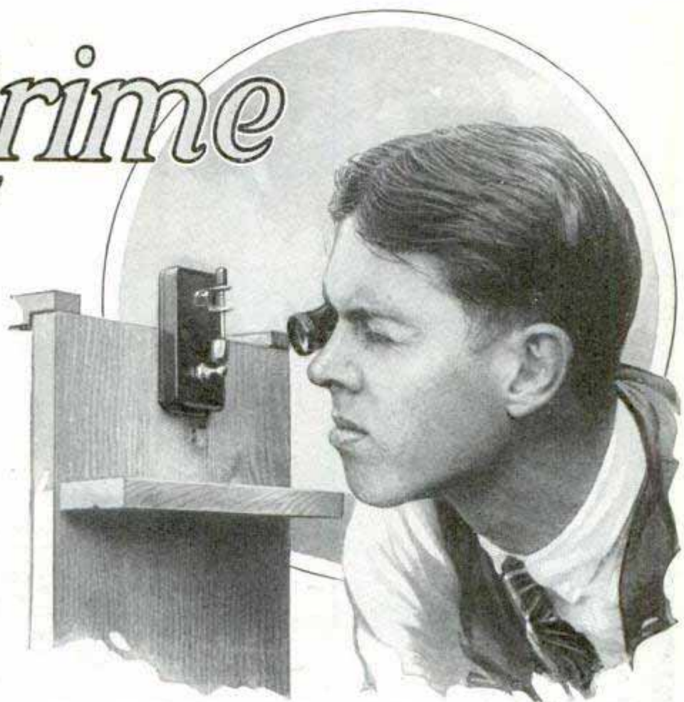
Examining a Fired Bullet through a Powerful Microscope in an Effort to Identify Its "Autograph," the Markings Caused by the Gun
