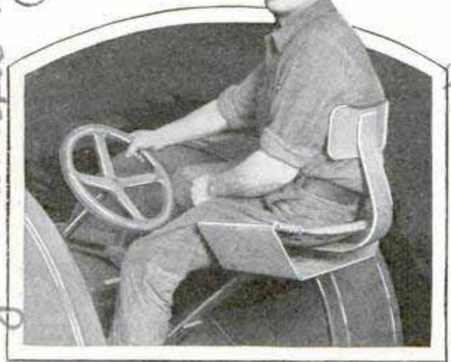
Spring-Mounted Seat with Office-Chair Back to Make Riding on Farm Implements Less Uncomfortable
