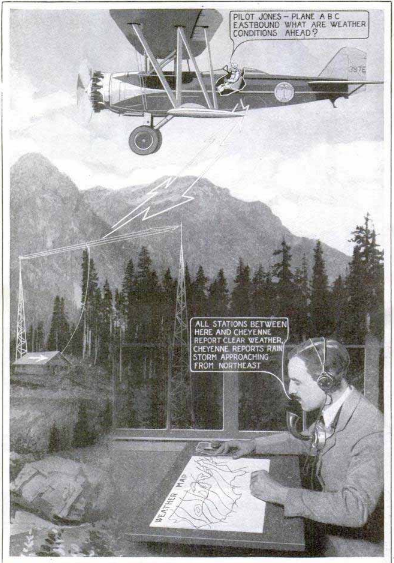
How the Air-Mail Radiophone Works; the Pilot Is in Constant Communication with Ground Stations at 200-Mile Intervals and Knows the Weather Conditions Ahead at All Times
