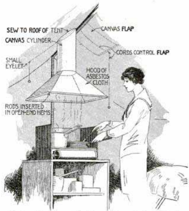
Asbestos Hood over the Camp Stove in the Tent Carries Off the Fumes
