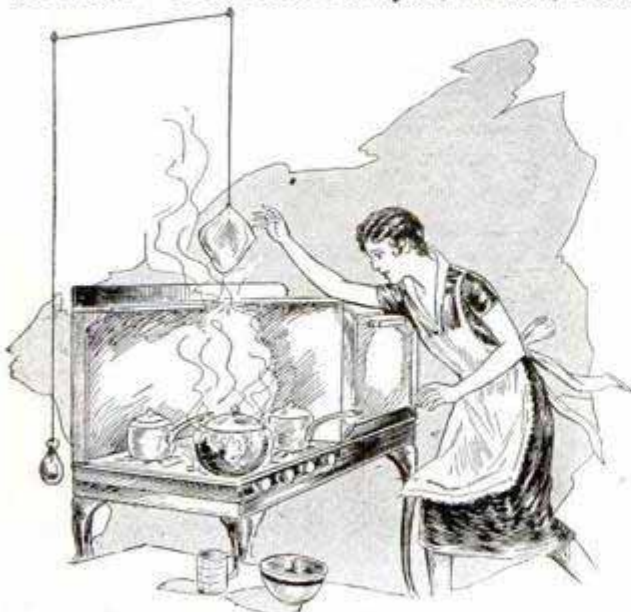
This Counterbalanced Pot Holder Is Always at Hand When Needed
