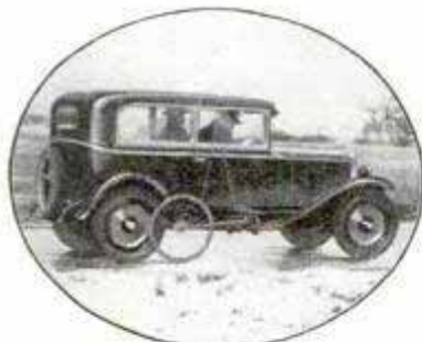
A fifth wheel speedometer scientifically measures speed and mileage.
