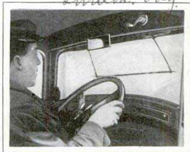
Wide Windshield Wiper Which Sweeps across the Top of the Glass, Clearing a Larger Space
