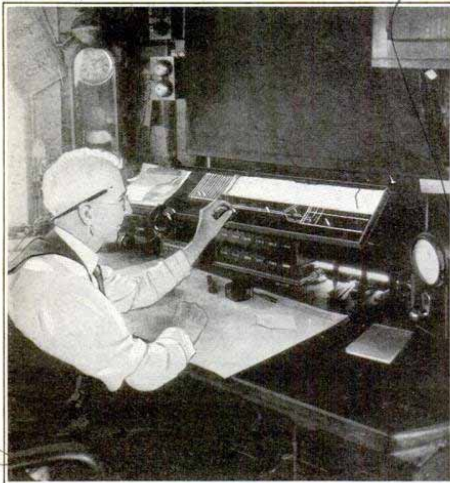
"Cribbage Board" Train Indicator, Used in Tower at Louisville, Ky., to Keep Track of Train and Engine Movements in Yards
