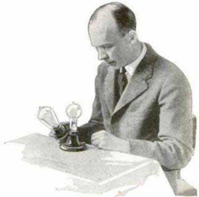
Model of Edison's First Incandescent Light in Holder, Being Compared with a Recent Bulb
