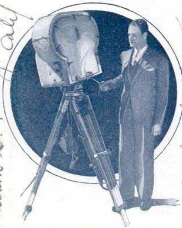
Soundproof Camera Cover Stops the Grinding of the Machine from Being Recorded on "Talkie" Film
