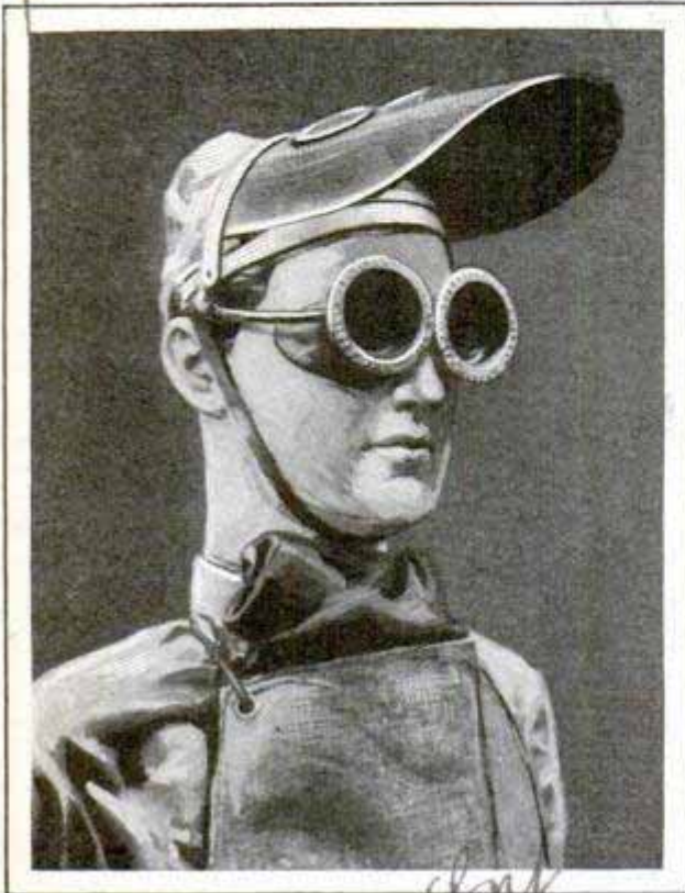
Face Mask Raised over the Goggles; It Can Be Lowered Quickly to Protect the Wearer
