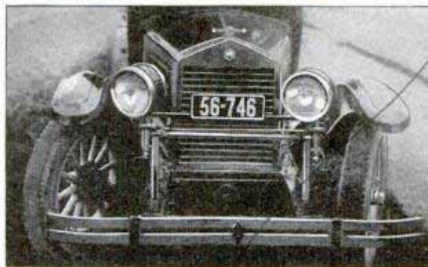
When the Front Wheels Turn, the Headlights Turn with Them, Directing Their Rays around Corners
