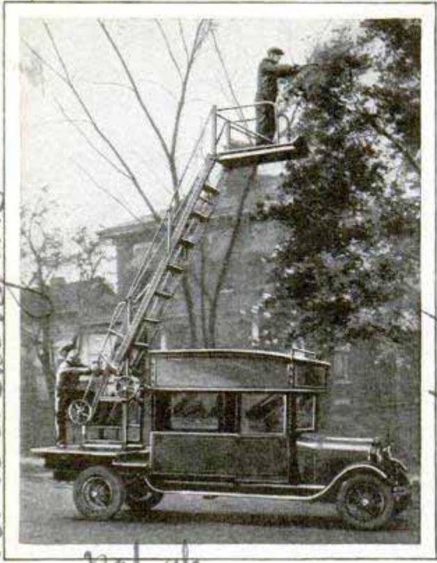
Trimming Trees with the Aid of the Ladder Truck; the Steps Swing on a Turntable
