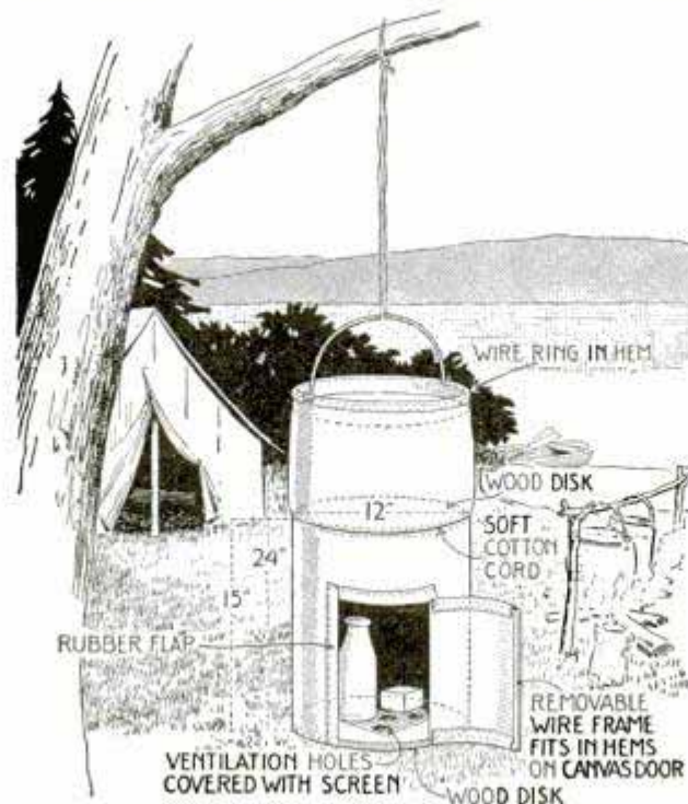
Collapsible, Iceless Refrigerator, Made of Canvas, Keeps Food Cool in Camp
