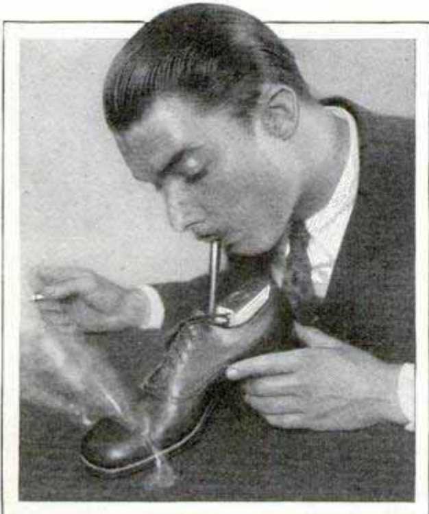
Blowing Smoke through the Openings in the Shoe to Show How Well the Article Is Ventilated
