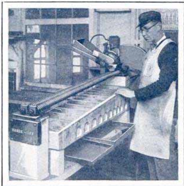
Sorter That Separates Nuts or Bolts of Different Sizes from Hopper
