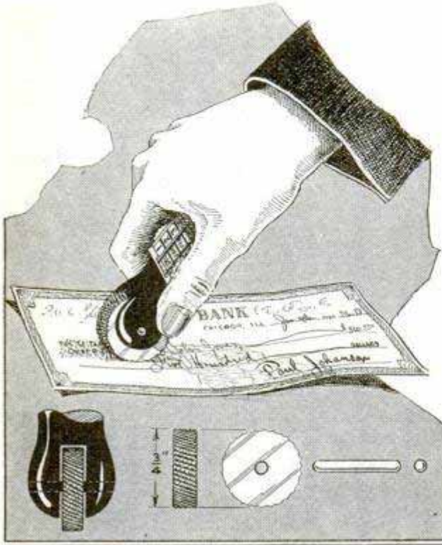
Deeply Knurled Steel Disk, Attached to Dating-Stamp Handle, Makes Good Check Protector
