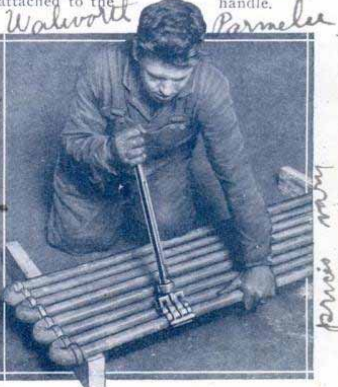
Even Soft Brass Pipe Is Not Injured by This Wrench, Which Grips like a Human Hand
