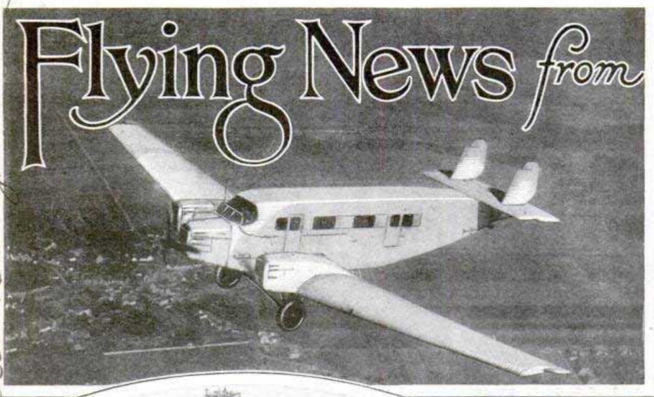
Inclosed Motors, a Larger Cabin and Improved Streamline Design Feature This Recent Passenger Air Liner; at Left, a Big Fuel and Service Truck to Supply the Planes and Landing-Field Tanks
