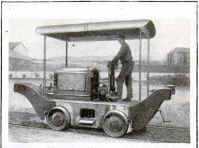
Railroad Tractor, Powered with Converted Ford Engine, for Use in Moving Cars in French Yards
