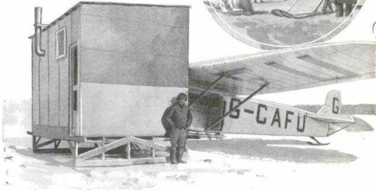
Keeping the Airplane's Engine Warm in Winter; the Top Picture Shows a Simple Canvas Covering Serving as a Flue for a Heater; the Bottom, a Portable Workshop for the Mechanic
