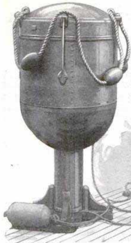
Close View of the Rescue Buoy; Cover Removed to Show the Reel for the Life Line and Space for Other Articles; Right, a Launching
