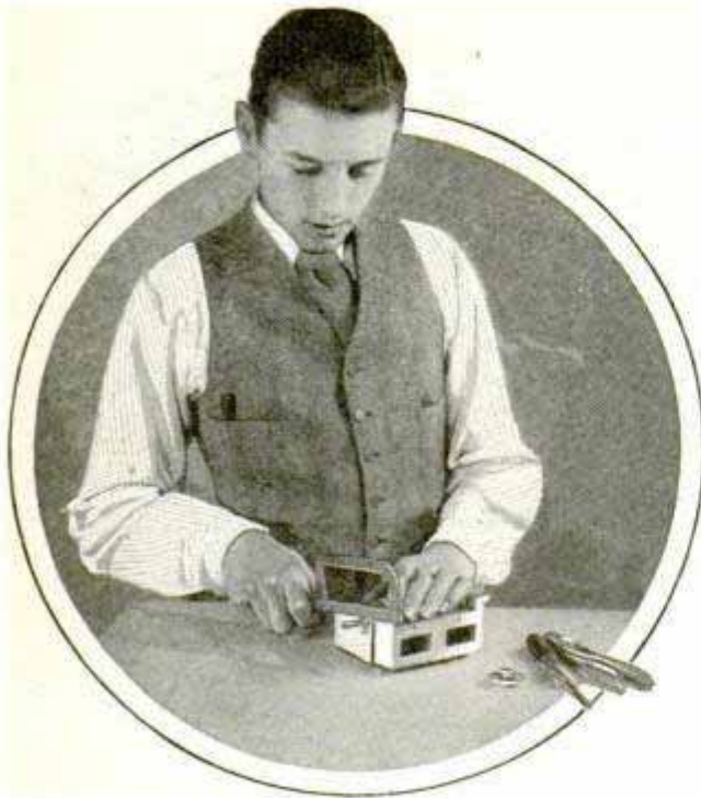
Top, Sawing Off Unused Length of Shaft at Rear of Ganged Condenser Unit; Above, Mounting Flexible Coupling for Shaft Extension
