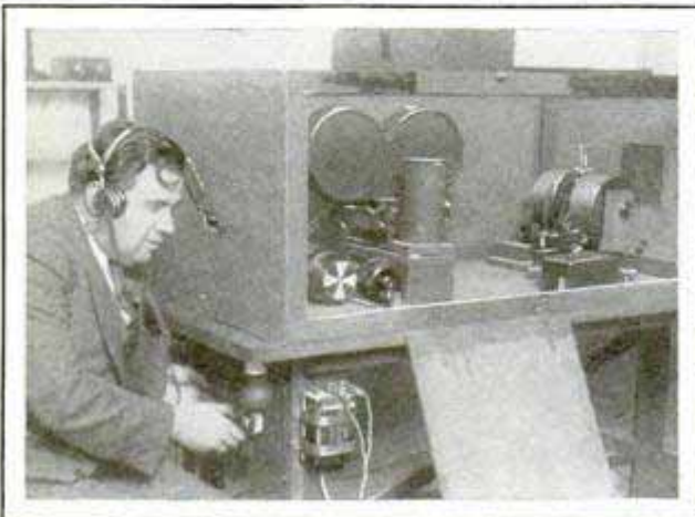
Machine Which Films the Beating of a Heart for the Movies as an Aid to Doctors Studying the Organ
