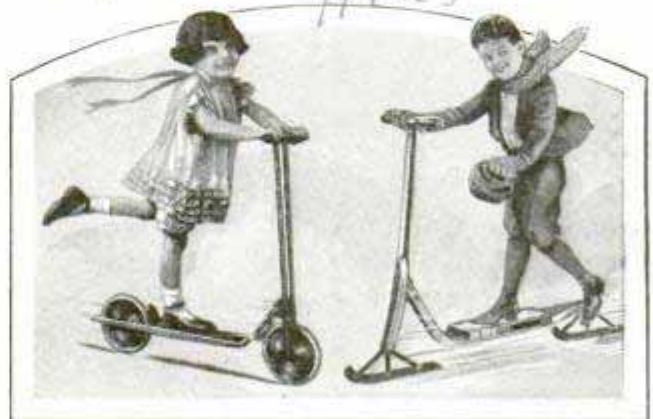
Adding a Pair of Special Skates to a Scooter, in Place of the Wheels, Turns It into a Sled
