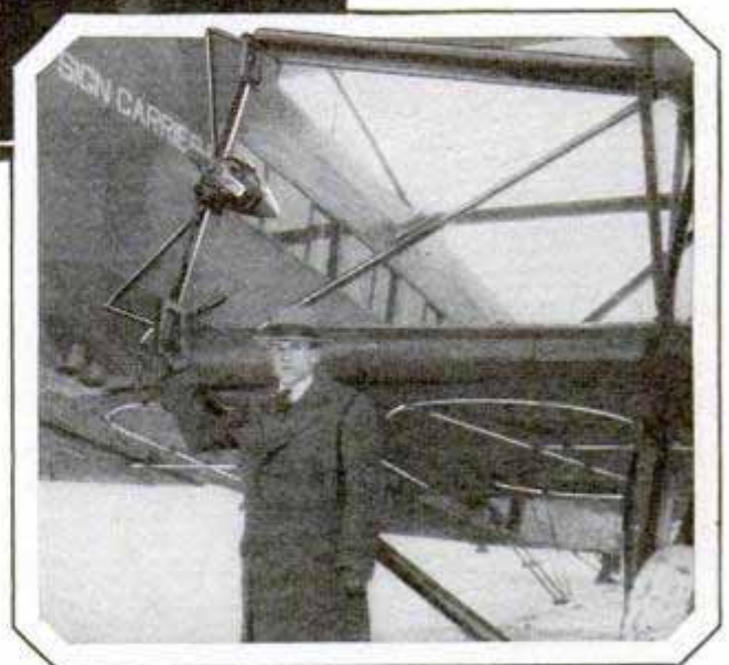
Close-Up of the Inspection Mirrors; the Control Cabin of the Neon-Light Plane, and the Light Tubes on the Lower Wing
