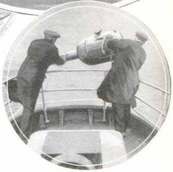
Close View of the Rescue Buoy; Cover Removed to Show the Reel for the Life Line and Space for Other Articles; Right, a Launching
