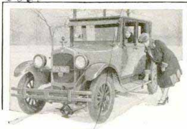
Jacking Up the Car by Turning Crank at Side of Running Board; Front and Rear Are Raised
