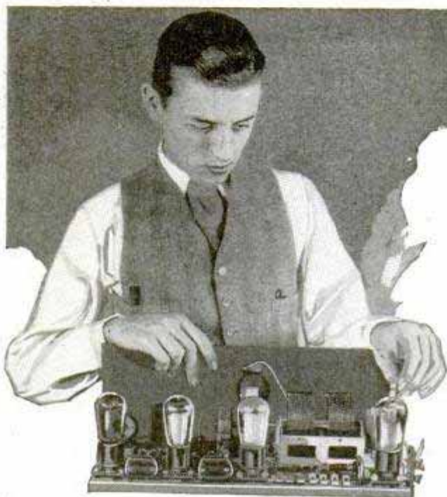
Rear View of Completed Receiver, Showing Tubes in Position
