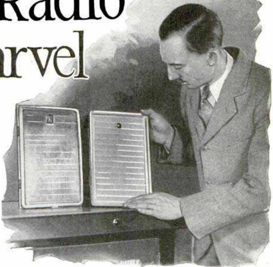
The Speaker Itself; in His Hands, Kyle Has the Thin Aluminum Plate; the Other One Is Completed with Foil Covering
