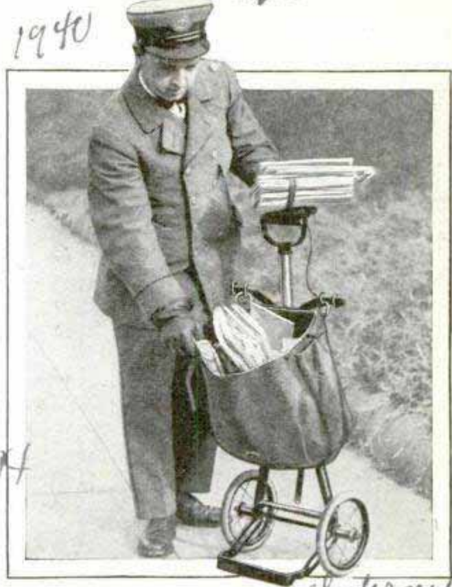
Wheeled Cart for Carrying Mail Bag; It Takes a Load from the Postman's Shoulders
