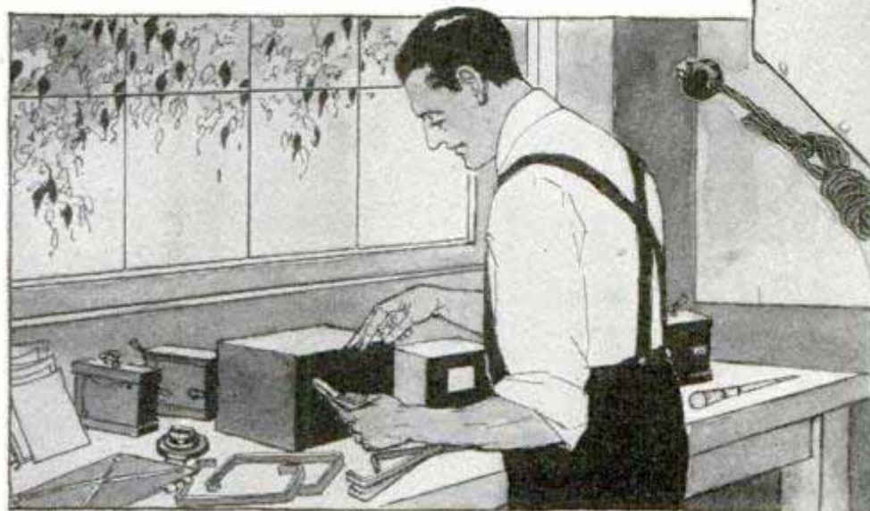
Left, Unit of Compact Design Provides Efficient Antenna and Ground Connections as Well as a Means of Controlling Line Voltage; Two Outlets Are Also Furnished for Set and Dynamic Speaker; the Unit Is Well Fused to Prevent Burn-Outs in the Receiver; Right, a Compact Short-Wave Adapter, Now Available for Use with Any Receiver, Covers All Short-Wave Bands without Changing Set Wiring
