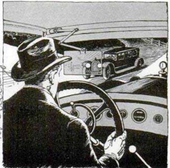
Glare Screen in Place on Windshield, Showing How It Protects the Eyes from Approaching Headlights
