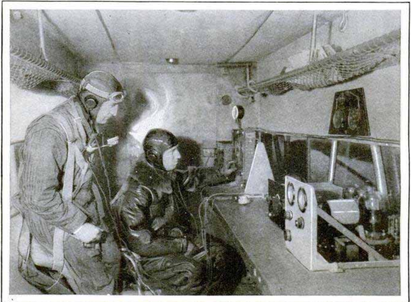
Lieut. Leroy M. Wolfe and Capt. P. S. Edwards in the Flying Laboratory at Wilbur Wright Field; Experimental Work Is Carried On While in Flight, to Test Radio Beacons, Two-Way Voice Conversations, Long and Short-Wave Code Transmitters and Receivers, and Various Types of Radio-Operated Signals
