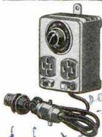
Left, Unit of Compact Design Provides Efficient Antenna and Ground Connections as Well as a Means of Controlling Line Voltage; Two Outlets Are Also Furnished for Set and Dynamic Speaker; the Unit Is Well Fused to Prevent Burn-Outs in the Receiver; Right, a Compact Short-Wave Adapter, Now Available for Use with Any Receiver, Covers All Short-Wave Bands without Changing Set Wiring
