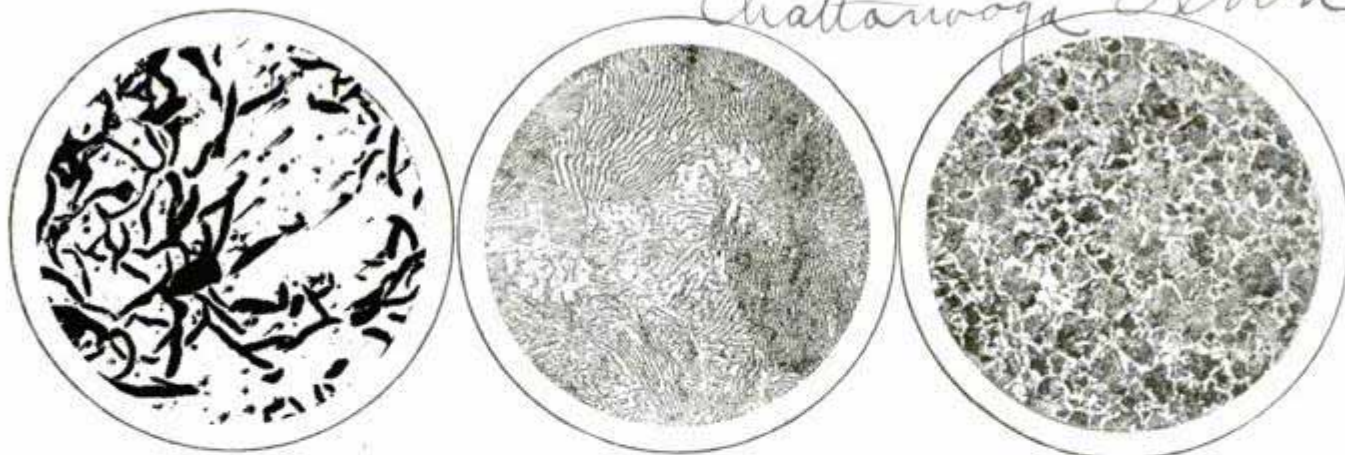
Three Kinds of Iron; Gray Cast Iron, with Coarse Graphite Flakes, at Left; Pure Iron and Carbide of Iron, Center, and, at Right, Crystals of Pure Iron Imbedded in Carbide
