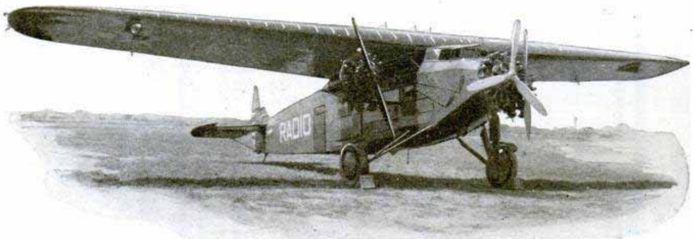
The Radio Plane at Wright Field; to Keep the Slipstream of the Nose Propeller from Interfering with the Wing Screws, It Has Three Blades, Thereby Making a Smaller Diameter Possible
