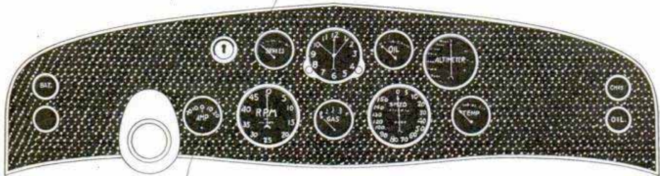
The New Duesenberg's Instrument Board Includes Brake-Pressure Gauge, Tachometer, Altimeter, and, in the Corners, Four Telltale Lights to Warn When Attention Is Needed
