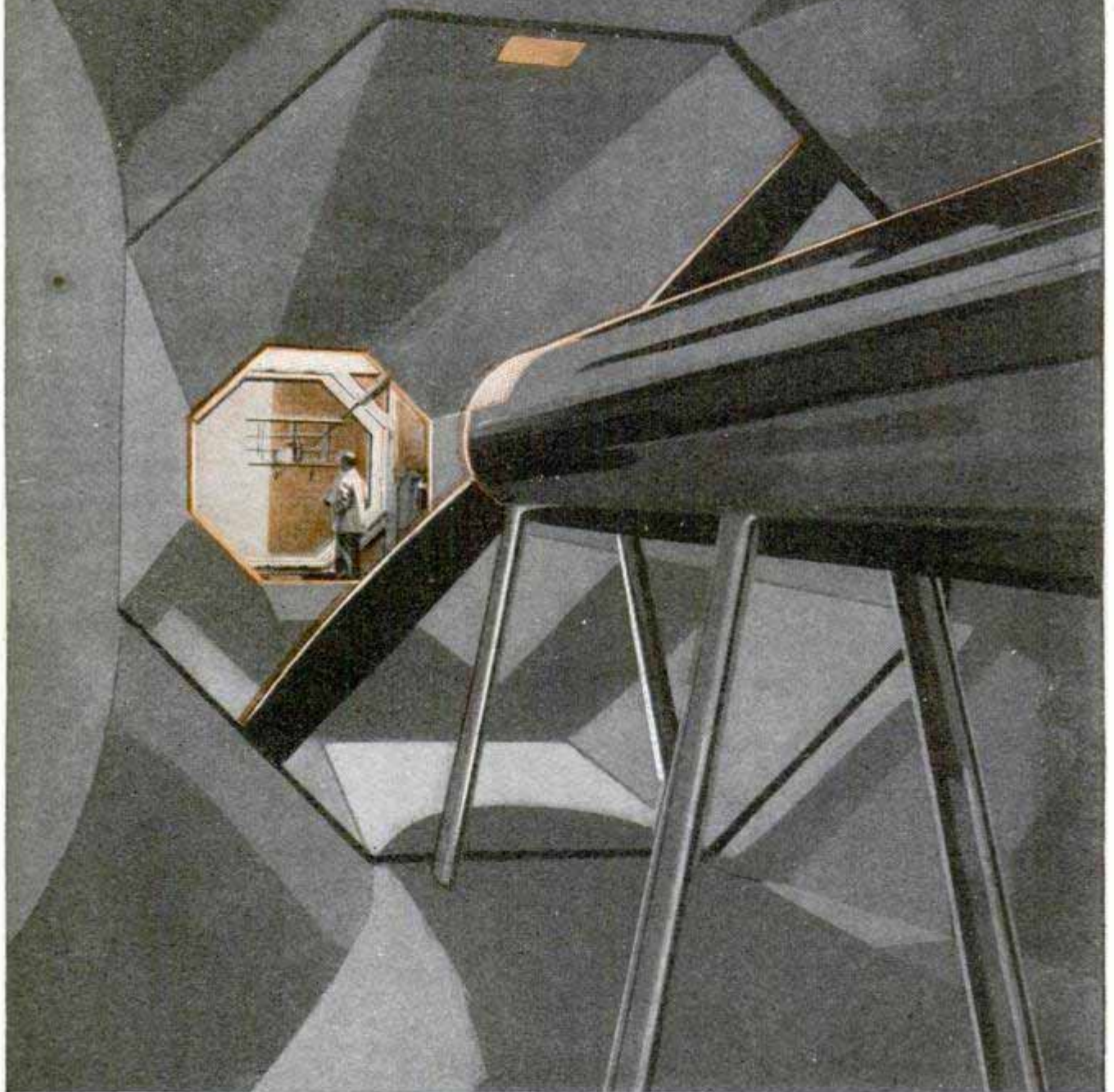
Looking through a Wind Tunnel; in the Background Is a Model Plane, Mounted in the Test Chamber Ready for Measurement, and in the Foreground the Propeller That Furnishes the Gale
