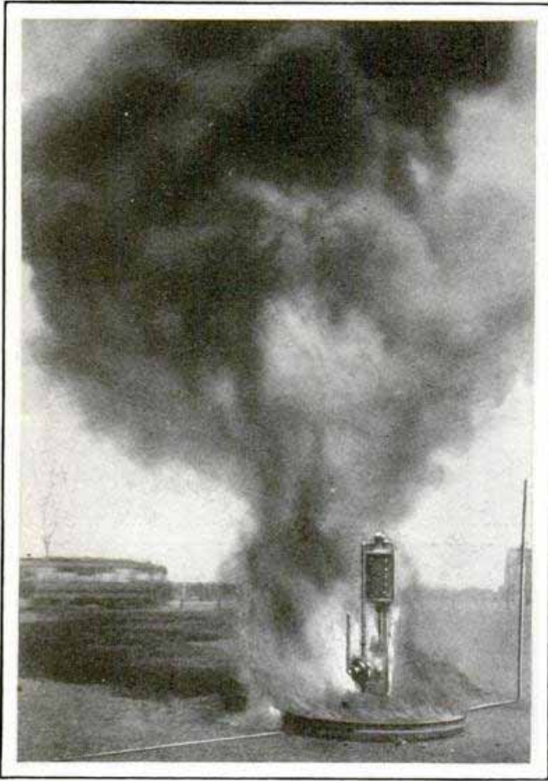
An Experiment to Find Whether the Gas Pump Is Safe from Cigaretts and Carelessly Tossed Matches
