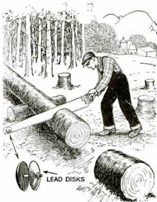
Weighting End of Saw Blade with Lead Disks Makes It Cut Faster
