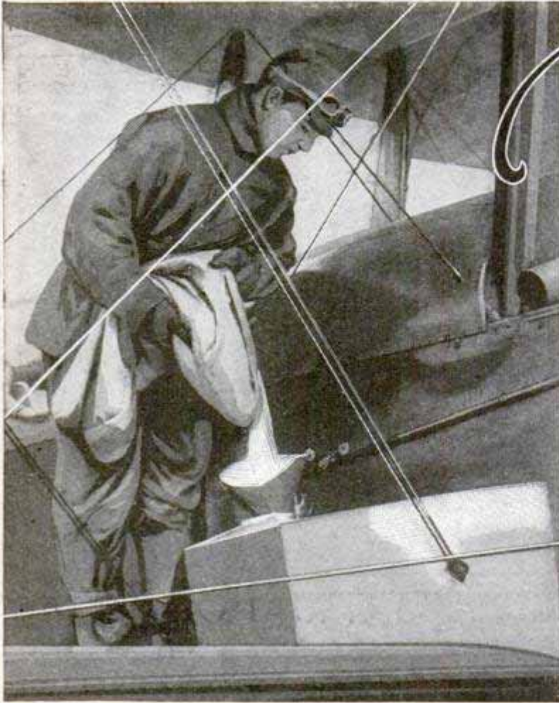
Capt. A. I. Eagle, Bolling Field, Filling the Sand Box before a Flight in an Attempt to Disperse Fog with Electrified Sand
