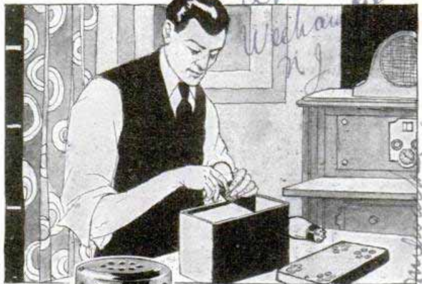
Left, Dry Rectifier Unit of Plug-In Type, Said to Have Extra-Long Life, Replaces Full-Wave Rectifier Tubes in B-Eliminators; Below, Handy Unit Combines Light-Socket Antenna and Supply Outlets for Dynamic Speaker, Eliminators or A. C. Receiving Sets
