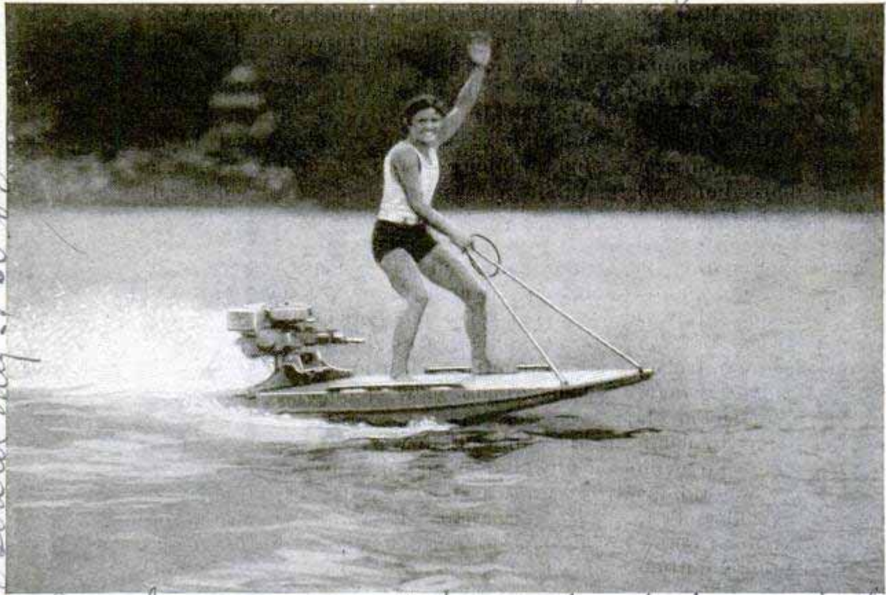
No Chicago - can be bought thru boat engine dealer Surfboards Pulled behind Fast Motorboats Are Common, but Here Is One That Is Pushed, and by an Outboard Motor - Leaning to the One Side or the Other Steers the Board
