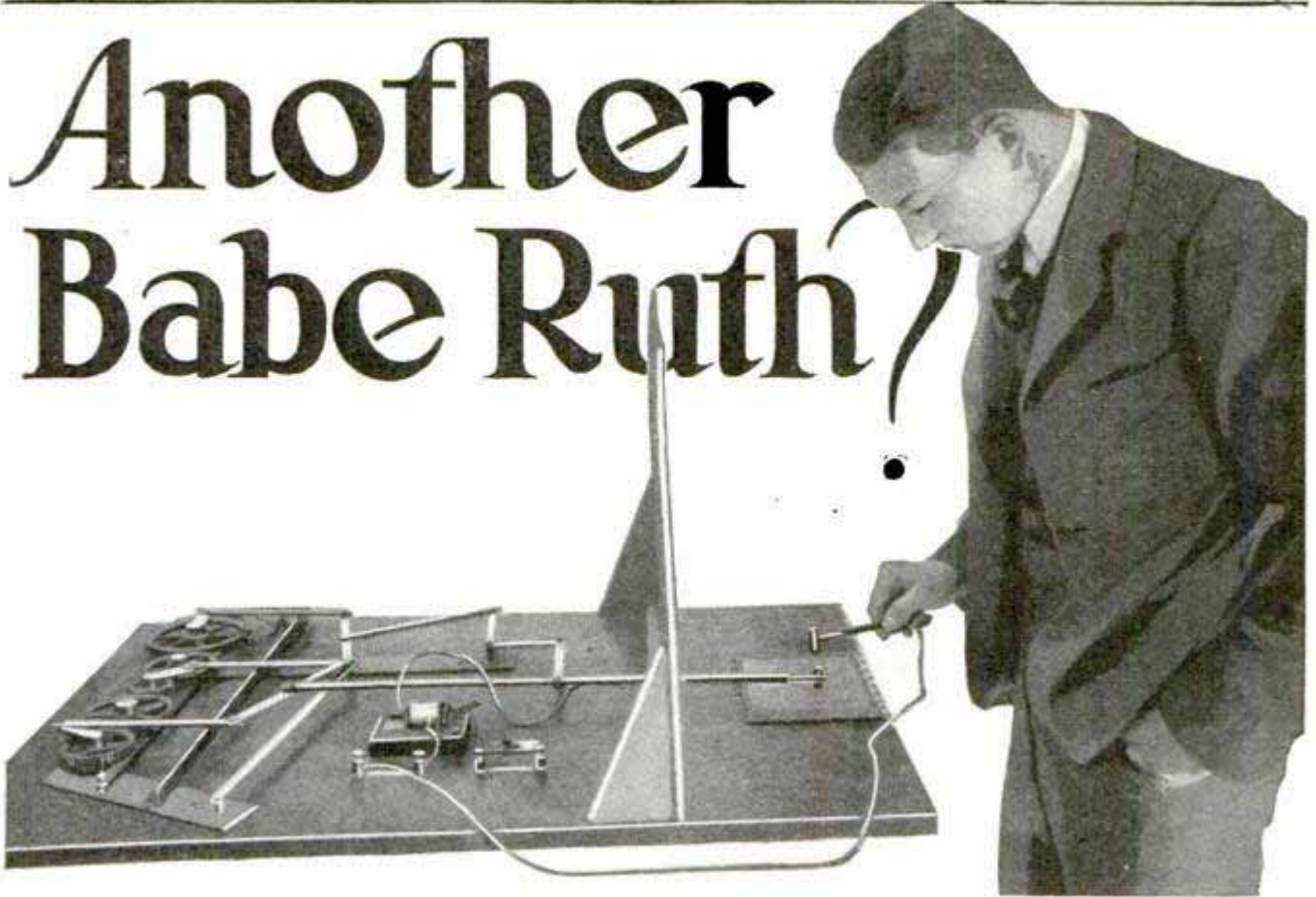
A Test for Mental and Muscular Co-ordination; the Athlete Attempts to Make Regular Contact with the Electrified Hammer as It Is Moved by the Hidden Mechanism
