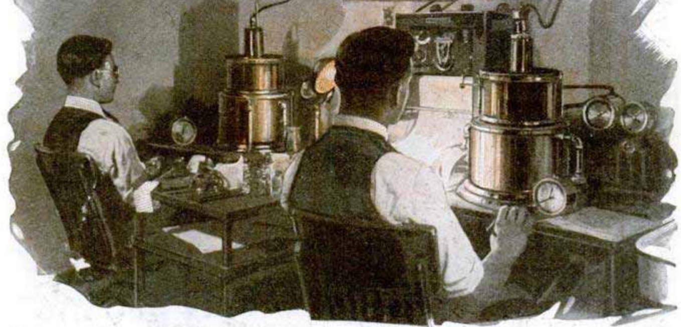
Testing Automatic Sprinkler Heads to Determine Whether Corrosion, Suffered during Use in Industrial Plants, Is Sufficient to Prevent Their "Popping" at the Correct Temperature
