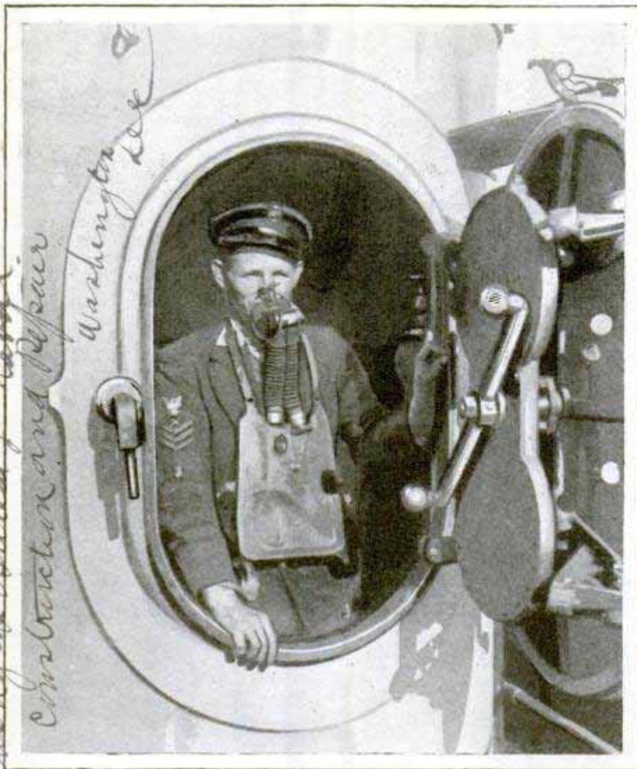
Diver in the Recompression Chamber, Preparing to Test an "Artificial Lung," Which Has Proved Practical at Depths of 155 Feet
