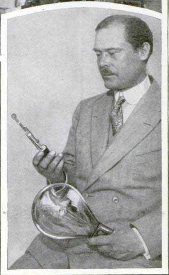
Laboratory Installation Showing the Projector and Disk at the Left and the Screen at the Right; Right, Doctor Alexanderson with the Filament and Tube Used in the Television Apparatus
