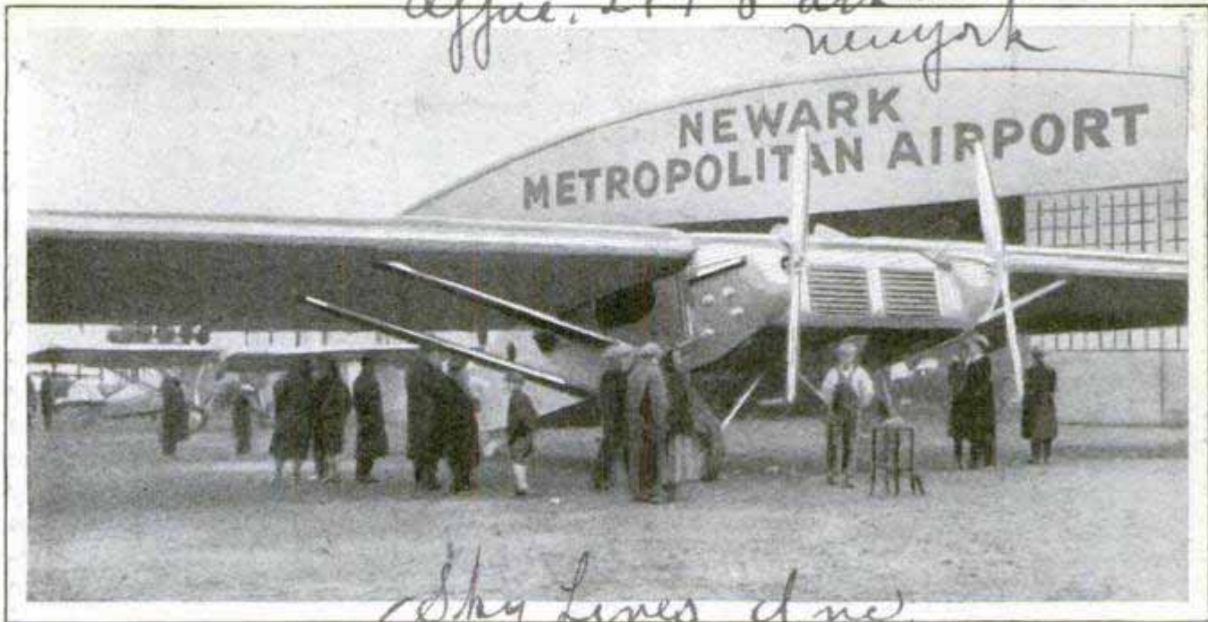
Twenty-Passenger Metal Monoplane with Its Wide Cabin, Shaped like the Wing Itself, to Afford More Room for the Occupants and Decrease Air Resistance
