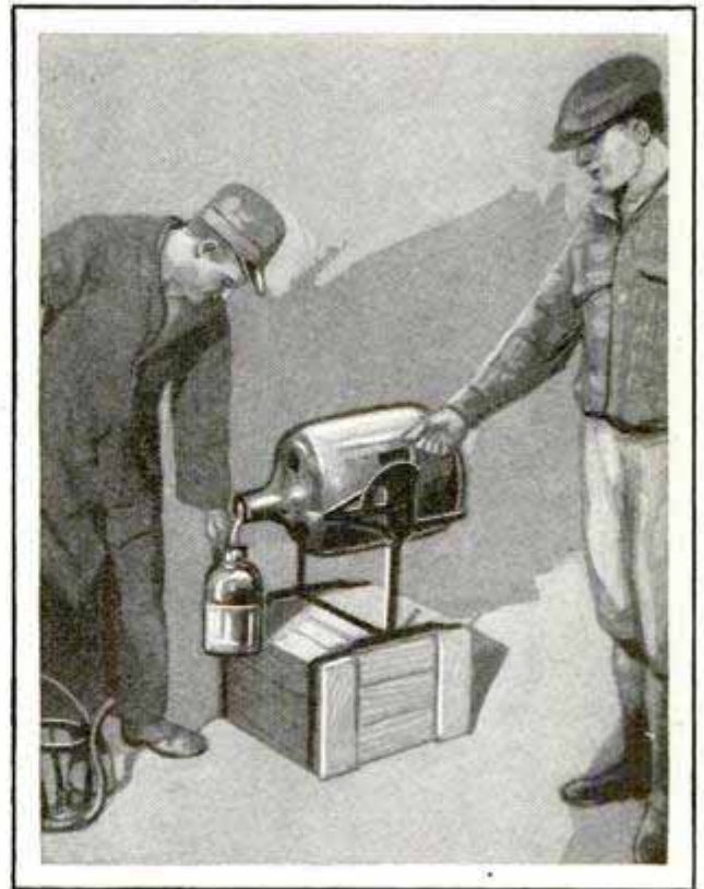
Window-Raising Mechanism Taken from Auto Door Makes Good Bottle Tipper
