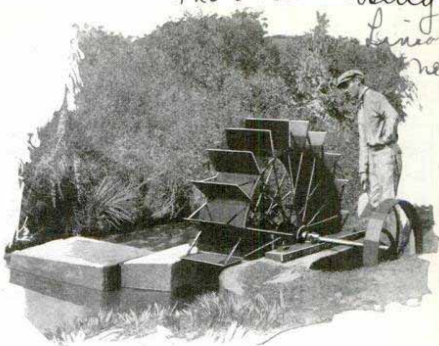
Old Tractor Wheel Belted to Small Generator Provides Electricity for the Farm House
