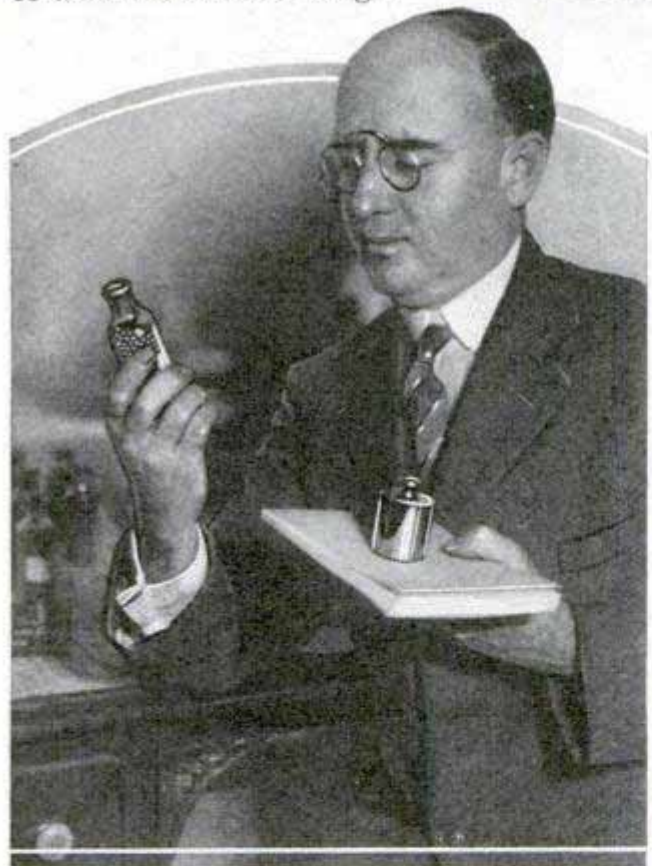
Comparing Home-Made Test Weight with Metal Standard, at Left, and, Above, the Final Accuracy Test
