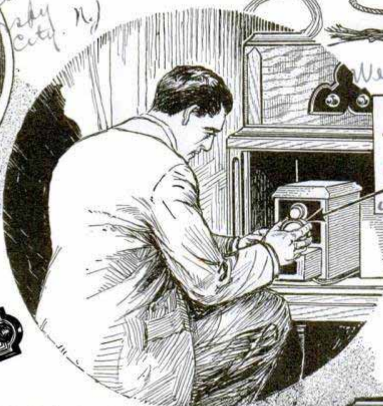
New Tuning Control Is Designed to Automatically Tune in the Station When the Correct Wavelength Number Is Turned Up in the Slot
