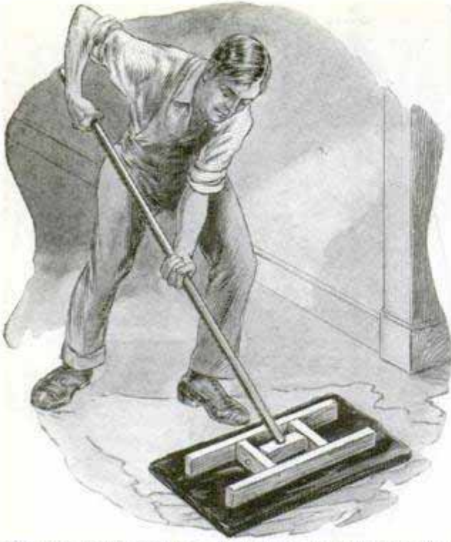
Homemade Floor Wiper Facilitates Janitor's Work of Cleaning Floors
