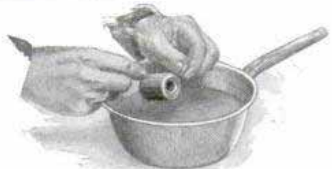
Above, to Separate the Coils, Hold in Boiling Water Until the Paraffin Softens, Then Remove the Primary by Pushing It Out with a Round Stick as Shown in the Photo Below
