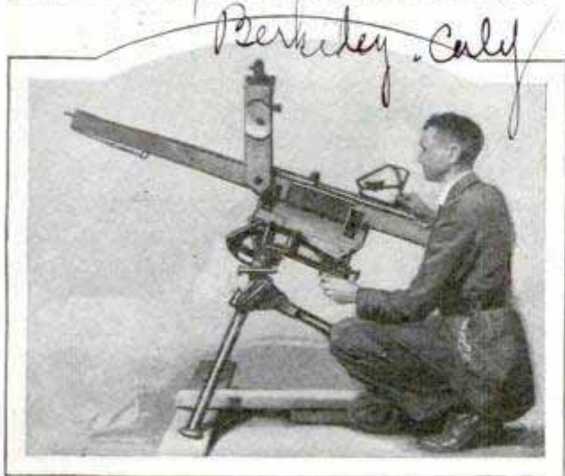
Wooden Gun That Fires Steel Bearing Balls, to Aid in Target Practice at Less Expense
