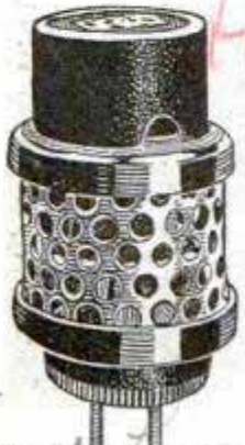
Left, Device Which Protects A. C. Tubes from Varying Line Voltage; Right, an Ingenious Assembly for Television Reception Permits Accurate Adjustment of the Neon Tube and Automatic Speed Control
