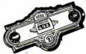
New Tuning Control Is Designed to Automatically Tune in the Station When the Correct Wavelength Number Is Turned Up in the Slot
