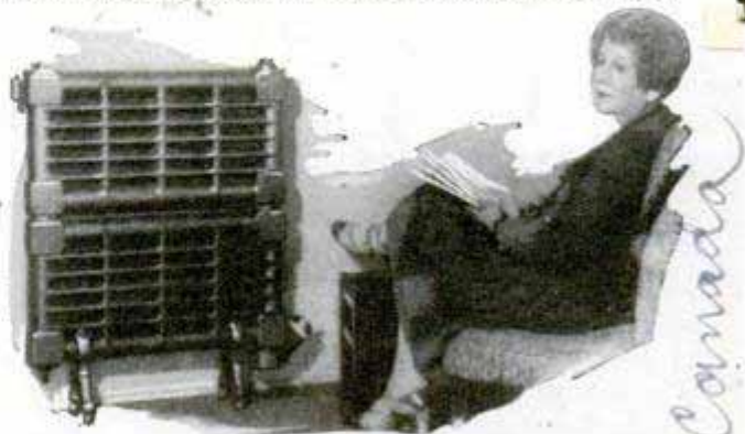
Electric Steam Radiator Which Requires No Piping; Water Is Vaporized between Two Electrodes
