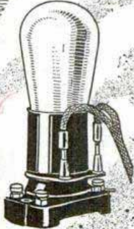
Right, Handy Adapter for Connecting Phonograph Pick-Up Is Available for Either Four or Five-Prong Tubes; Below, Resistance Unit for 32-Volt Systems Supplies Filament Current
