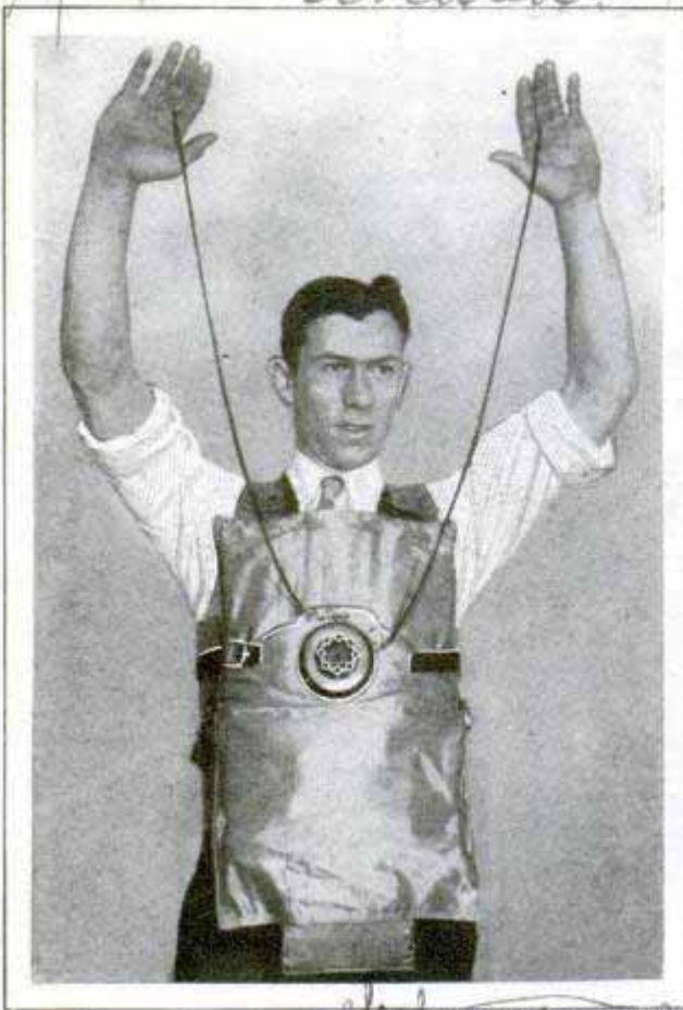
As Wearer Raises His Hands at Bandit's Order, a Stream of Bullets Issues from Gun in Center
