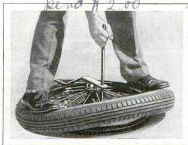
Tire Tool for Fords; It Is Hooked over the Rim and Leverage Applied from the Hub
