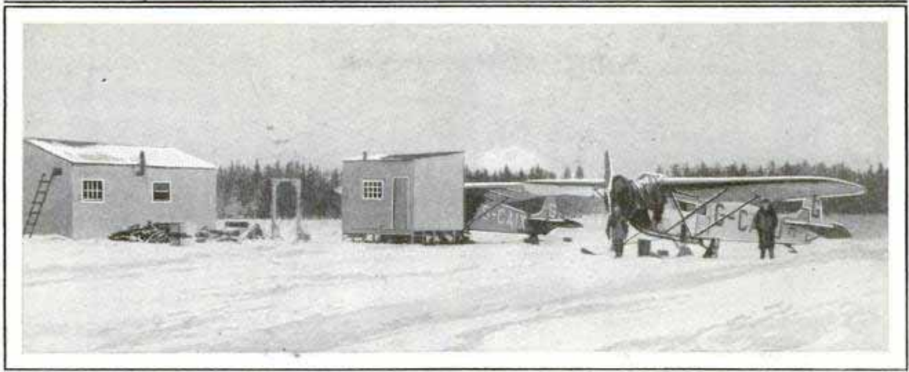
Freighting of the Railroad Is Largely Done by Air; in Winter, Portable Houses on Sled Runners Are Pulled over the Engines, to Keep Them Warm and Enable Mechanics to Work
