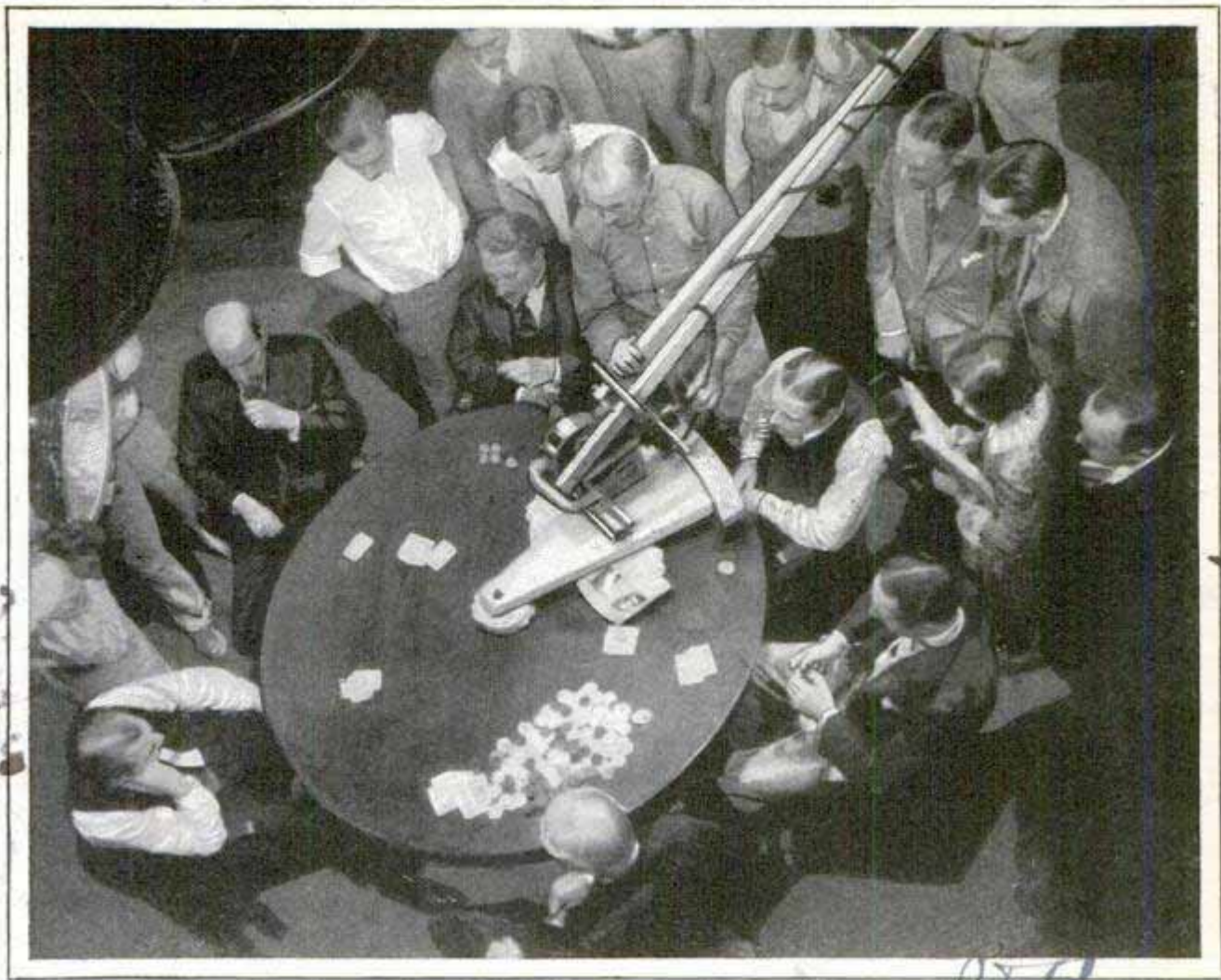
Photographing the Players' Faces in a Movie Poker Game; the Camera Turntable Was Operated by a Long Arm Extending over the Actors' Heads, and the Camera Was Motor-Driven
