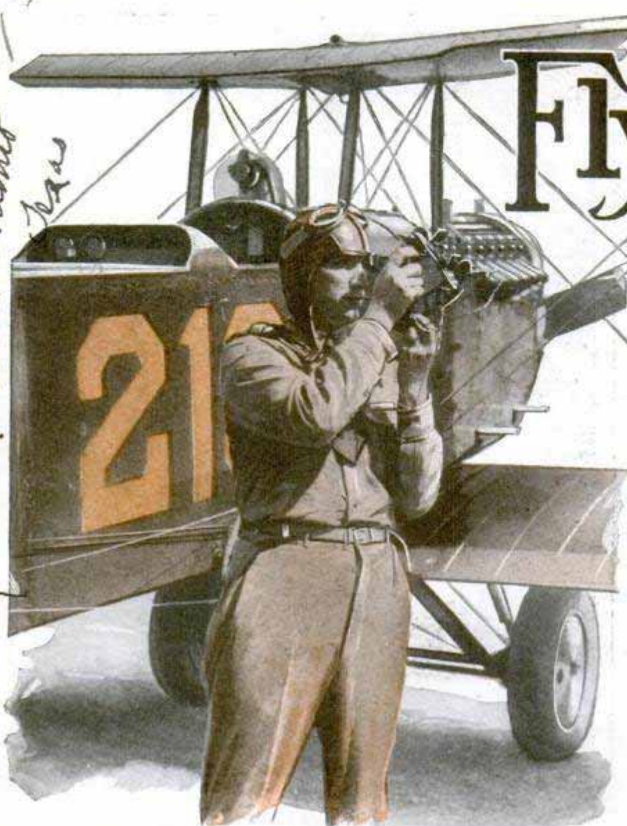
Shooting the Sun with a Special Sextant, Which Carries Its Own Horizon, for Aerial Work
