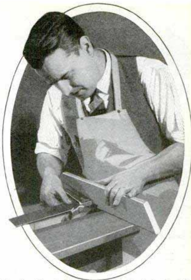
Squaring Up the Back Fence with the Dado Head before Screwing It Fast; This Is Important
