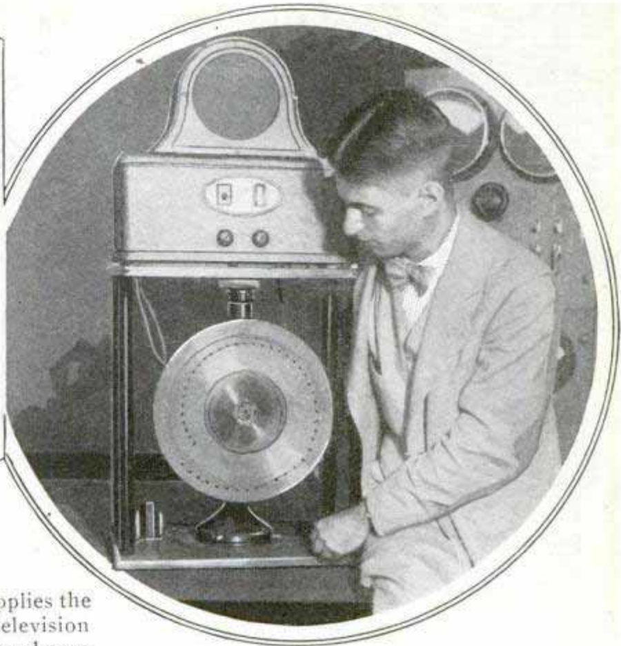
Left, Homemade Television Receiver Showing Fan Motor in Position; Right, Front View of the Apparatus Showing Radio Receiver and Loud Speaker Mounted Above
