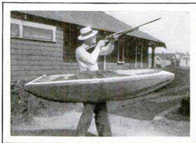
Rubber Boots and Boat in One Unit for the Duck Hunter, Who Can Propel Himself by Kicking
