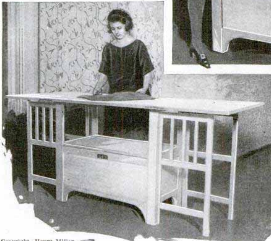
Space-Saving Combination of Seat, Cabinet and Workbench; the Upper Photo Shows It as a Cabinet and the Lower, as a Workbench
