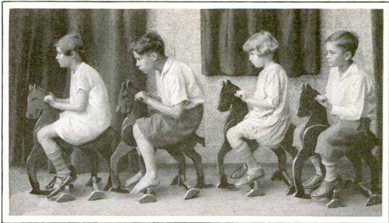
Walking Hobbyhorse Moves over the Floor as the Rider Swings His Weight Back and Forth, Alternately Advancing the Walking Legs and the Body of the Horse
