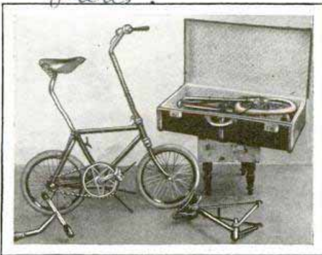
Folding Bicycle for Adults; the Machine Can Be Carried on Journeys Packed into an Ordinary Suitcase
