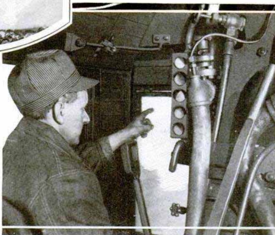
A Modern Semaphore Signal, and a Pennsylvania Fireman Pointing to the Five-Light Board Which Shows the Condition of the Track Ahead
