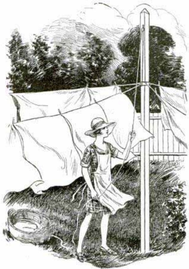
Convenient Arrangement for Hoisting Sagging Clotheslines Out of the Way
