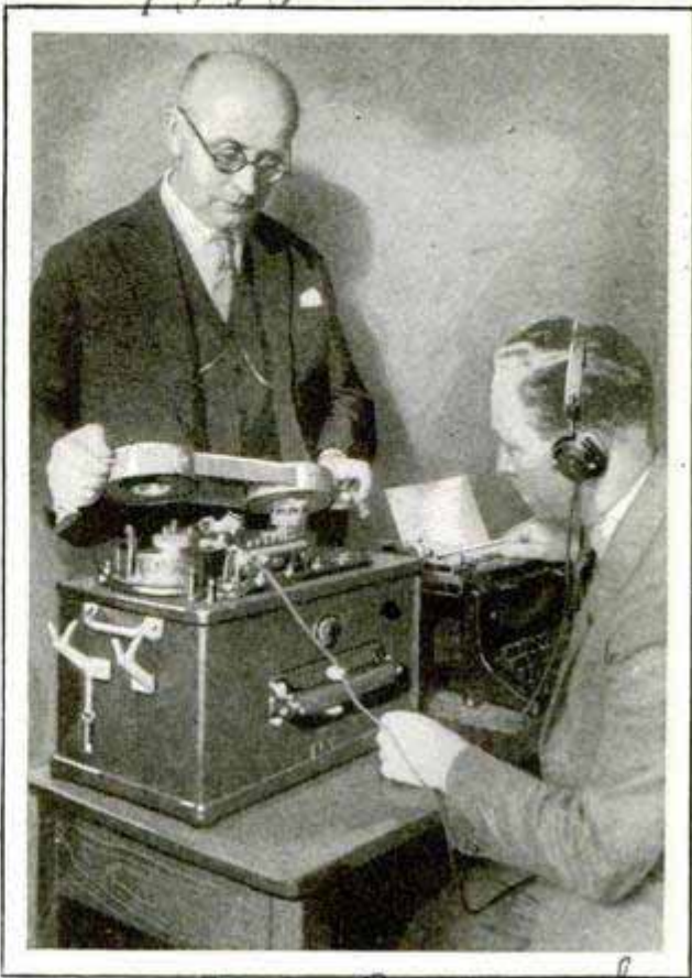
© Henry Miller News Picture Service Dictating Machine Which Records Messages on a Fine Steel Wire Instead of a Wax Record
