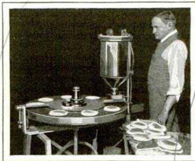
Automatic Pancake Machine; Batter Container at the Right, and the Cake-Turning Arm at the Left
