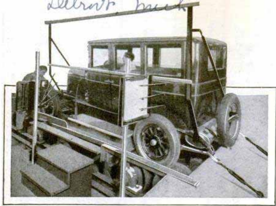
Shaking Table Which Gives an Automobile All Its Road Tests on One Platform, Taking the Place of Proving Grounds
