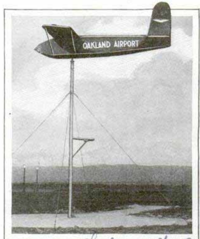
Dummy Airplane That Serves as Wind Vane; It Is Brilliantly Lighted at Night
