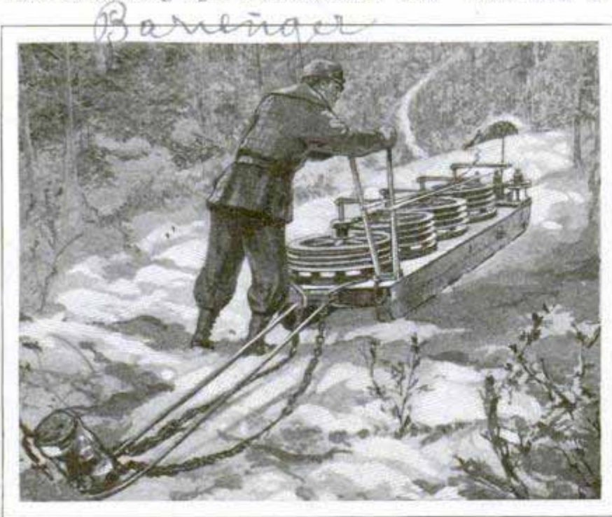
Controlling the Speed of Logs' Descent down Steep Grade with Braking Appliance at the Top of the Hill
