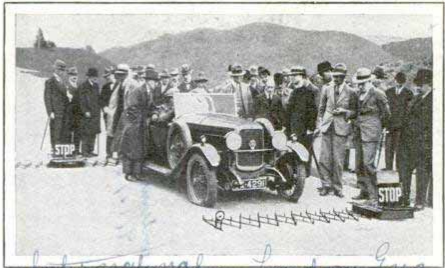
Puncture Trap That Can Be Quickly Extended across the Road to Halt Cars; Pressing a Button Releases the Rack
