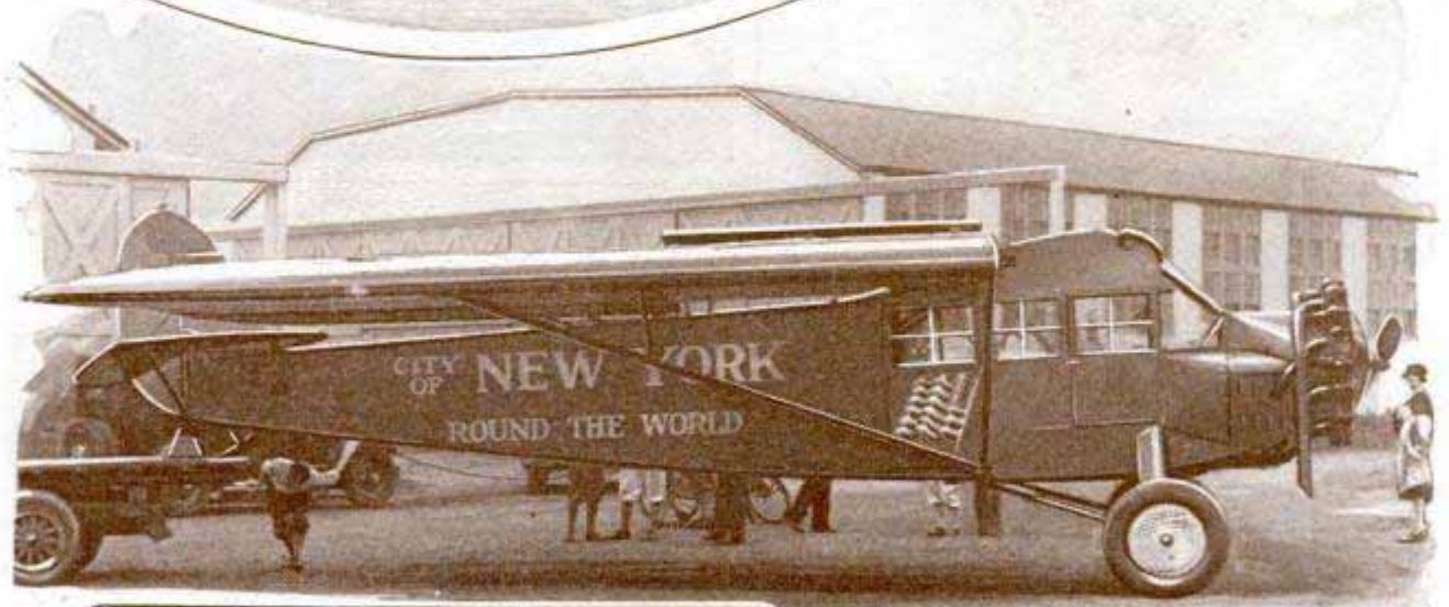
Modern Cabin Plane with Folding Wings; the Fairchild Monoplane John Henry Mears Used in Round-the-World Trip
