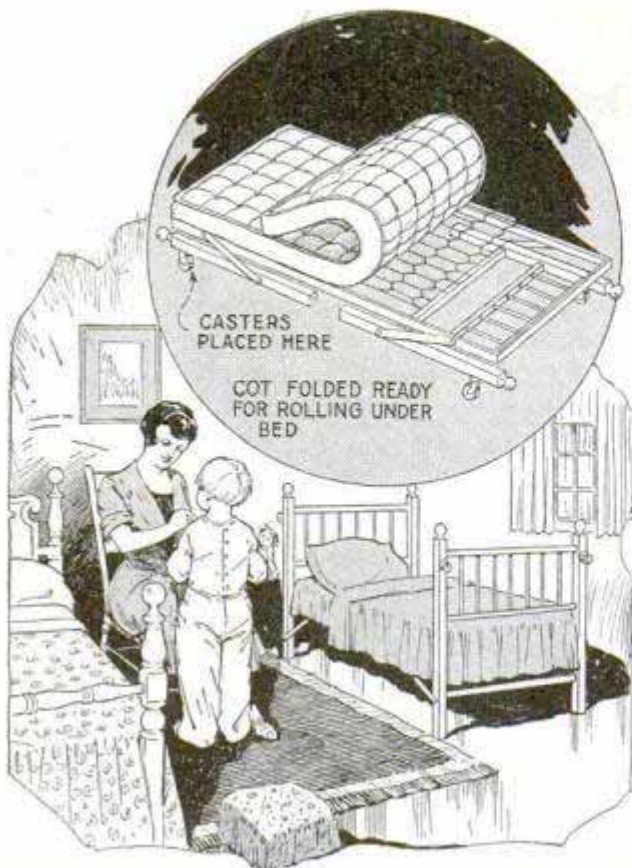
Folding Cot Equipped with Casters Is Stored Out of Sight under the Bed
