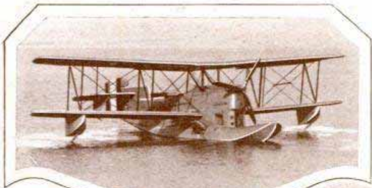
Loening Amphibian, with Three-Bladed Propeller; the Same Type Ship Is Being Produced as an Air Yacht, with Comfortable Cabin
