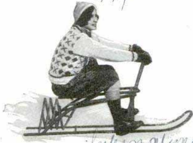
Foot and Hand-Propelled Sled with the "Pusher" Arm at the Rear; Note the Lightweight Construction
