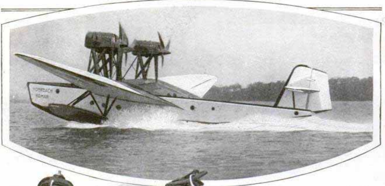
The Biggest Flying Boat Ever Built, the Triple-Engine Rohrbach "Romar," Was Successfully Flown on Its Initial Trials after Being Launched Recently at Travemuende, Germany. The Huge Craft Develops 2,160 Horsepower and Carries 2,114 Gallons of Gasoline in Its Wing Tanks. Owing to Its Boatlike Construction, It Can Ride Out a Storm at Sea If Forced to Alight; Three of the Boats Have Been Ordered by the German Air Lines for Service to South America, to Be Flown in Three Hops, the Longest Being from the Cape Verde Islands to Fernando Noronha, off the Coast of Brazil; the Planes Have a Wing Span of 121 Feet and a Length of Seventy-Two Feet Eight Inches, and Weigh 41,140 Pounds with Full Load
