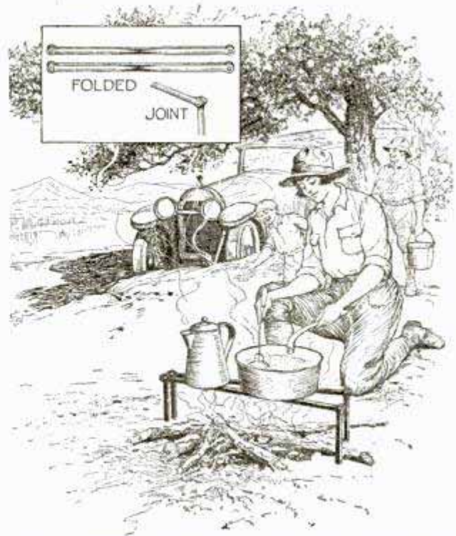
Handy Folding Camp-Fire Grate for the Tourist-Camper Takes Up Little Space in the Car
