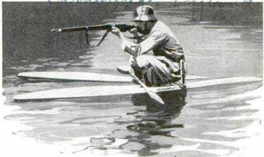
Foot Pontoons for the Soldiers Who Patrol the Danube River; Waterproof Sacks Inside Keep Their Feet Dry
