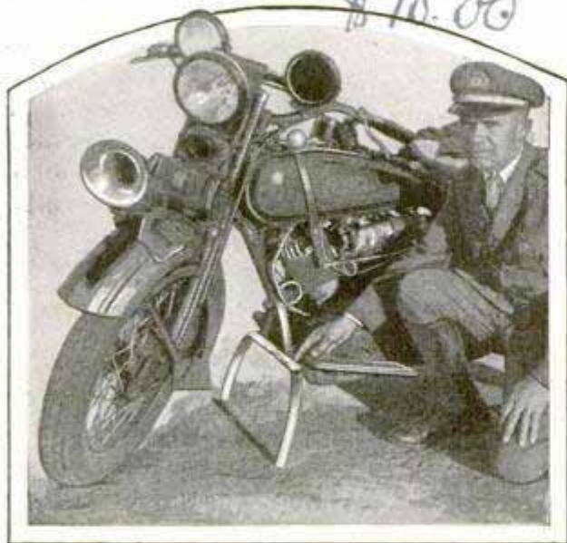
Support for Motorcycle Which Permits a Faster Get-Away and Is More Easily Lowered
