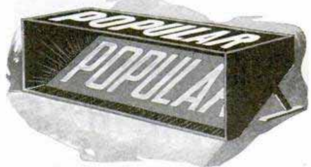
Drawing of the Lightless Sign, Showing How Letters Are Reflected by Mirror through Prism Glass
