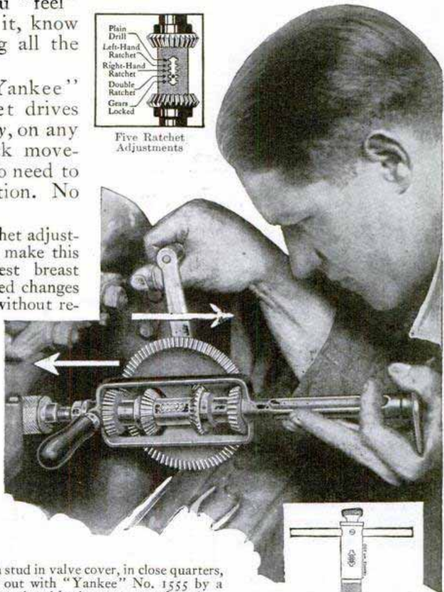
Tap the hole with the "Yankee" Tap Wrench, No. 250. Ratchet adjustments and sliding crossbar make awkward jobs easy. Price, $1.85.
