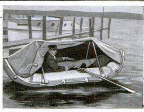
"Tire" Boat in Use; It Is of Fabric That Can Be Folded into Small Bundle When Deflated
