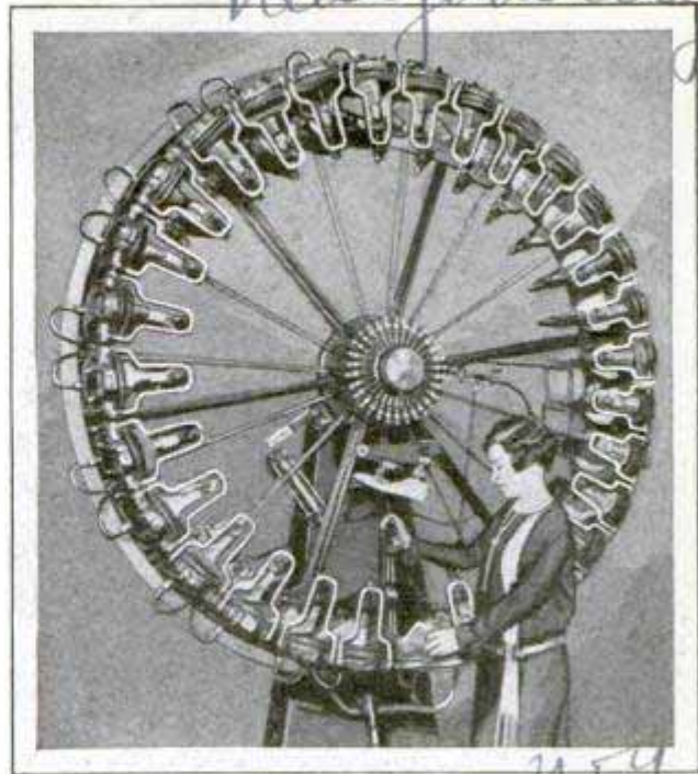
Wheel for Rapid Assembly of Shoes; It Makes 600 Pairs in Eight Hours
