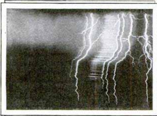
Photographing Electric Flashes with a Moving Camera; the Plate Separates the Discharges, Top Picture, into Many Separate Flashes
