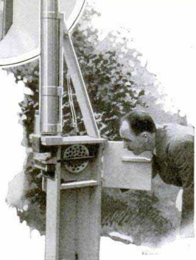
Studying the Effects of Weather on the Activities of Uncle Sam's Bees, and, Center, an Electric Flight Detector That Measures Their Trips
