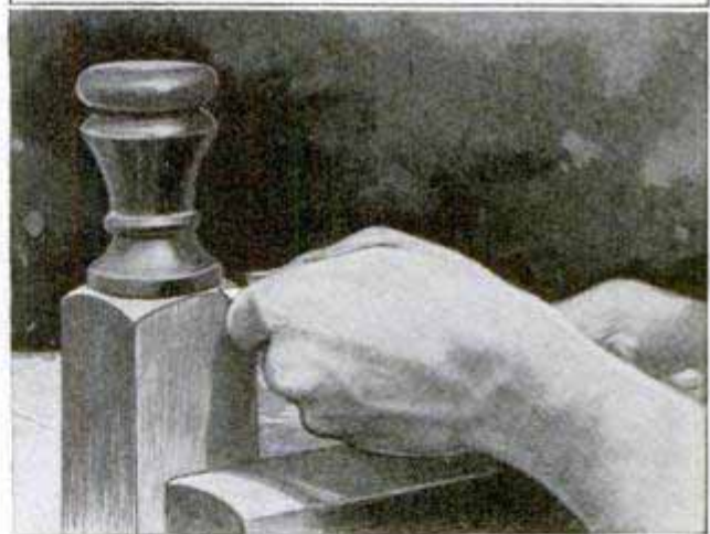
Left, Scribing the Centers of the Square Sections on the Center Spindles; Right, Rounding the Corners; Upper Right, End Elevation, Showing Rails, Corner and Center Spindles
