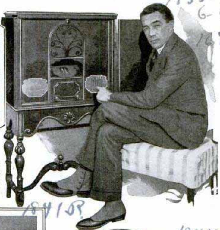
Right, Comm. E. F. McDonald, the Arctic Explorer, Demonstrating the New Automatic Radio Receiver Which Is Operated by Pressing One of a Series of Buttons That Automatically Tunes In the Particular Station Desired; Left, an Interior View, Showing the Tuning Mechanism
