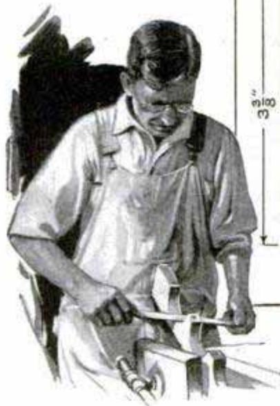
Above, End Veneer Clamped in Vise, Showing the Method of Lacing the Veneer to the Curves for Gluing; Below, Smoothing the Stretcher-Rail Arches with a Half-Round File; Right, Details of the Stop Blocks and the Carved Seashell Ornaments for the Stand Ends; Upper Right, Shaping the Lower Rail Ends, Chipping Out the Waste and Trimming Smooth with a Chisel
