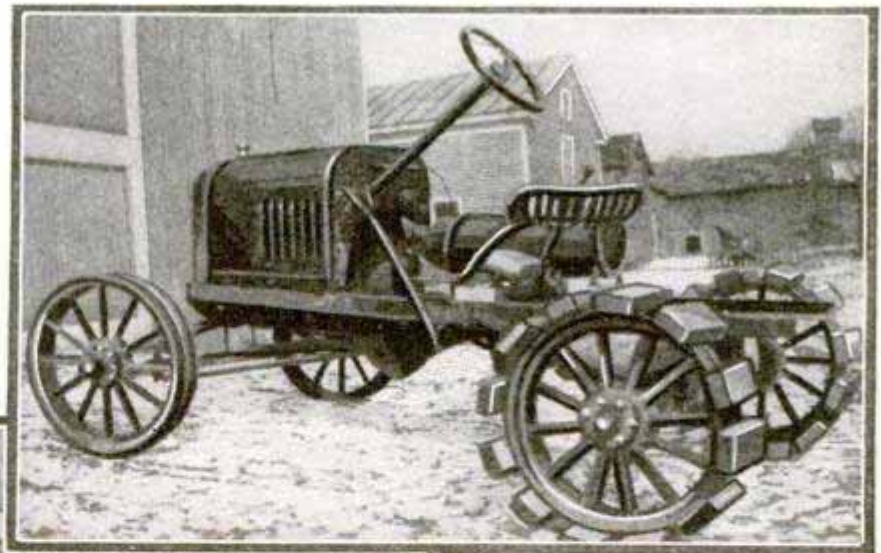
Two Views of a Light Farm Tractor, Consisting of a Ford Auto Chassis Equipped with an Extra Transmission of the Three-Speed Type; This Arrangement Gives a Wide Range of Power
