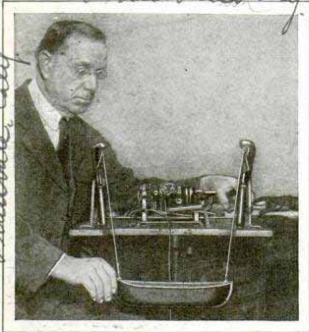
Model of the Lifeboat Which Can Be Launched in Few Seconds by Pressing a Button
