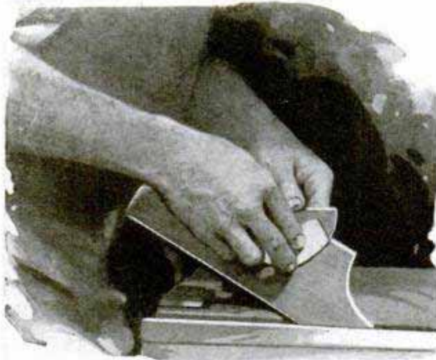
Sanding the Arches
