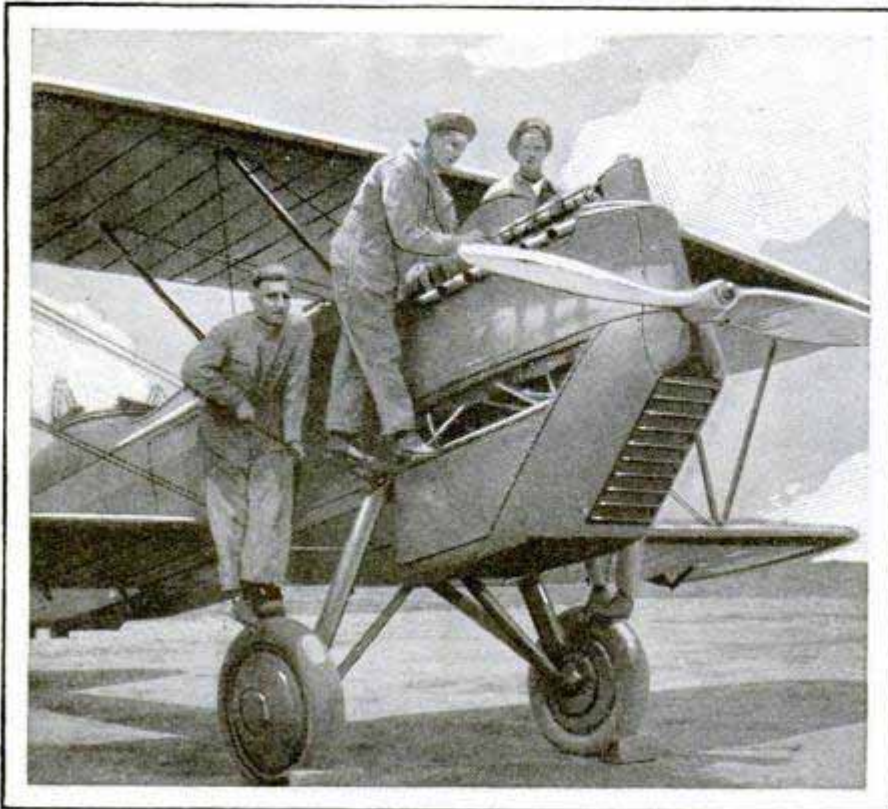
Mechanics Working on a Curtiss Observation Plane; This Type Has a High Speed of 140 Miles an Hour
