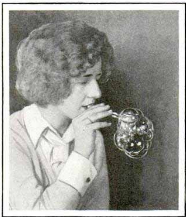
Demonstrating the Flotation Process with a Soap-Bubble Pipe and a Few Small Shavings of Lead
