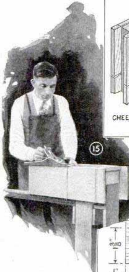
Fig. 14, Cutting a Tenon; Fig. 15, Planing Down the Sides of the Cabinet; Fig. 18, How the Saw Is Used in Cutting a Dado, and Fig. 19, Nailing In the Shelves
