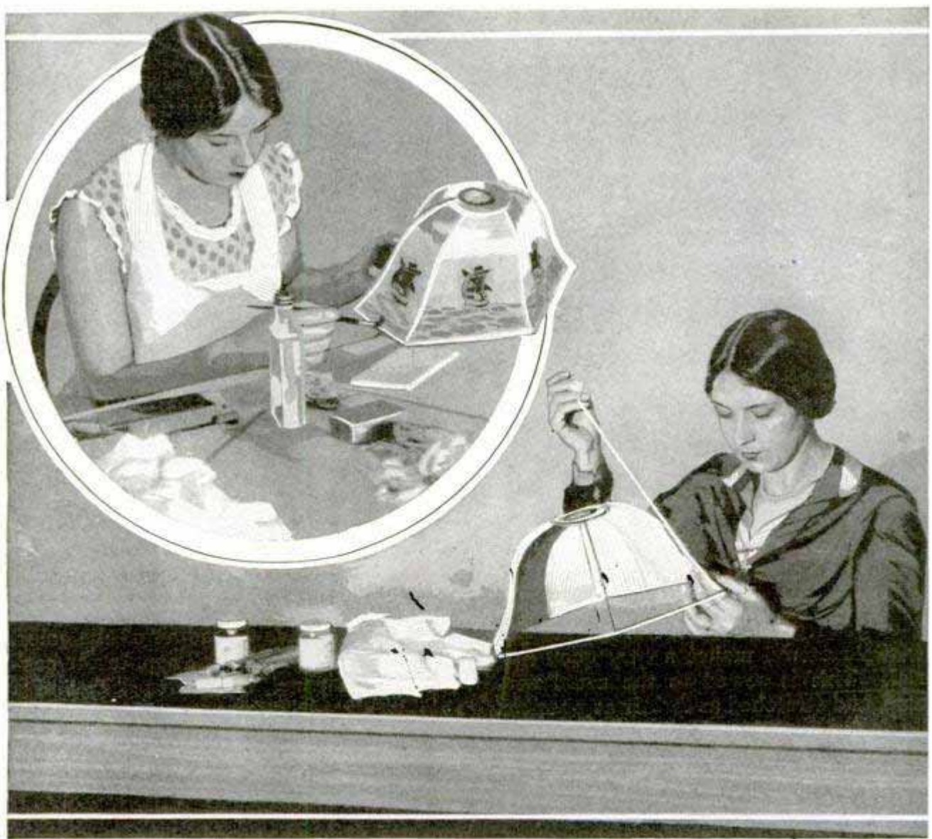
Two Steps in Making the "Ballotini" Shades: Sewing the Cotton Sheeting to the Shade Frame; Above, Painting the "Sea" to Meet the Transfer Pattern
