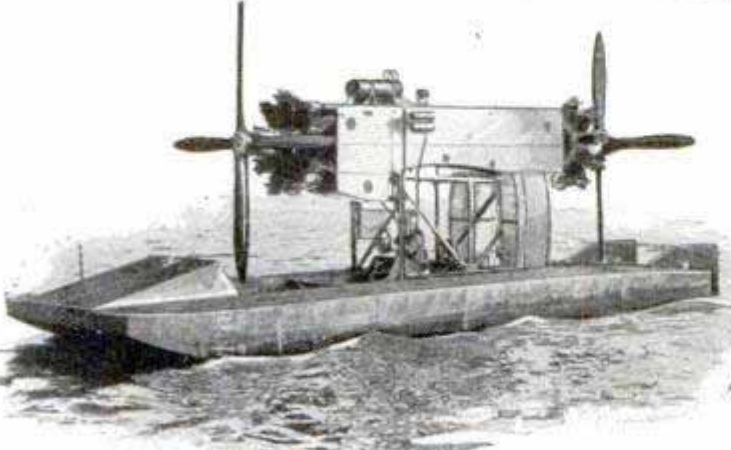
The Floating Testing Ground for Airplane Engines: Hydroplane with Motors Installed for Trial Run
