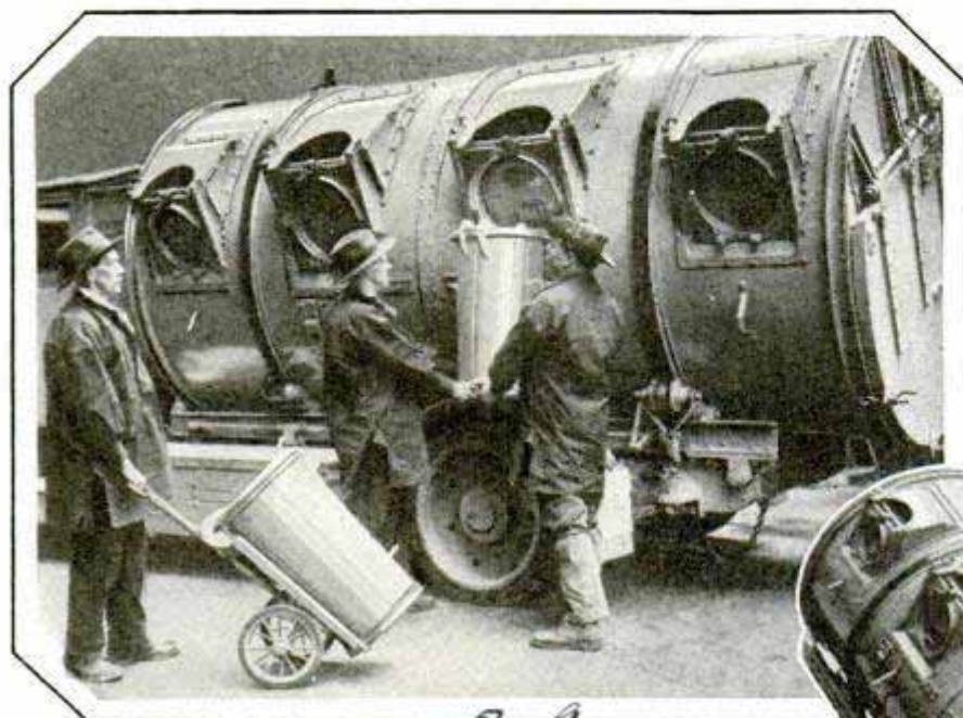
Filling the Garbage Truck through the Side Doors and Emptying a Load; the Tank Is Elevated by Hydraulic Mechanism
