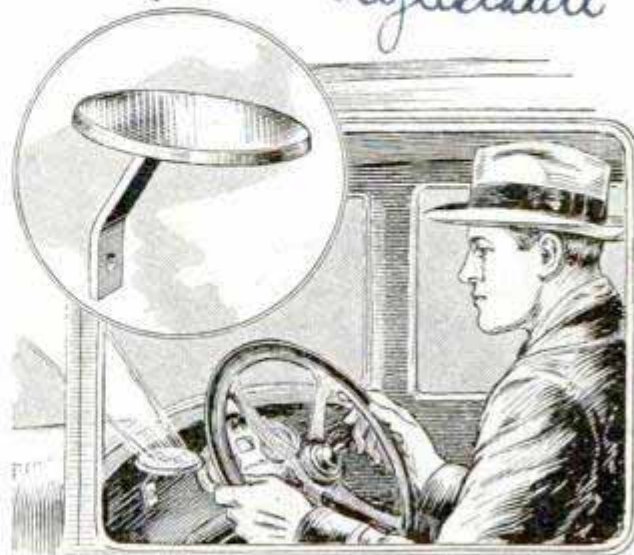
Drawing to Show Traffic-Light Mirror Installed for Reflecting Overhead Light Signals
