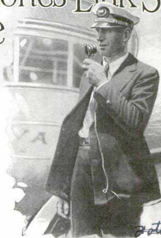
Tugboat Captain Receives Instructions from Shore While Towing a Ship, through Radio Telephone Installed on Deck
