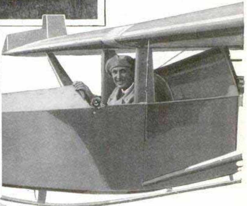
The Pilot's Cockpit of the Opel Rocket Plane; the Shield behind Him Covers the Rocket Compartment, While, in Front of Him, the Fuselage Is Carried Forward to Support the Stabilizer, and the Rudders, as Shown Below, Are Built above the Wing Tips; the Insert Shows the Machine in Flight, the Figure of the Watcher on the Ground Giving an Idea of Its Size; These Pictures of the Secret Tests of the Rocket Airplane Were Taken at the Trials Conducted by Herr Opel in the German Mountains, Following the Tryouts of the Rocket Idea on an Automobile and a Railway Car; the Former Developed a Speed of More Than 125 Miles an Hour, the Rail Car Being Even Faster
