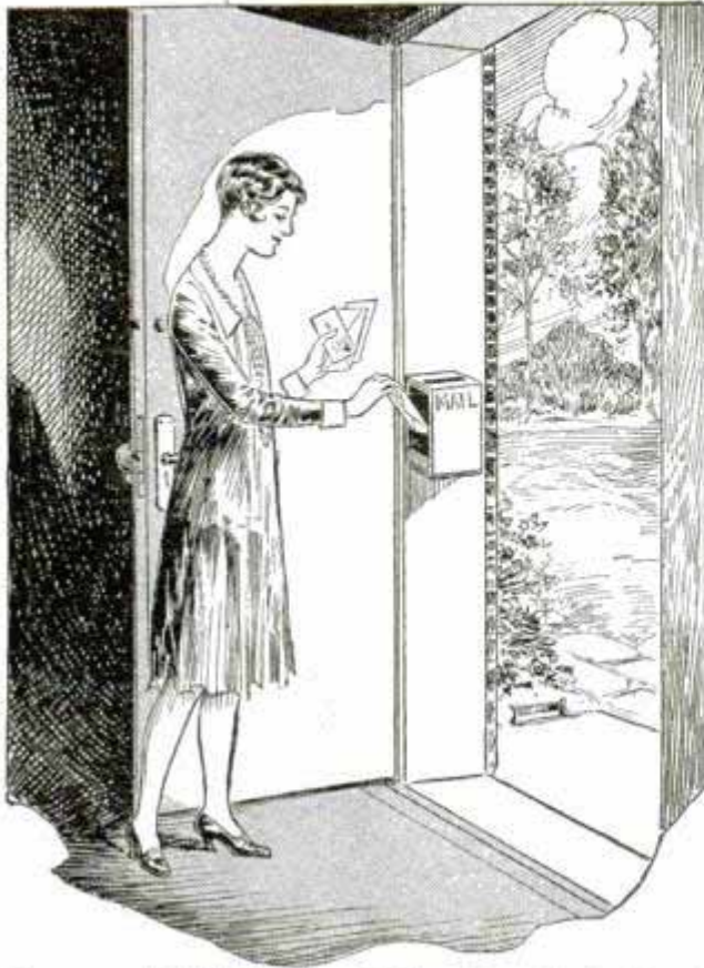
Contents of Mail Box Attached to Door Jamb Cannot Be Removed Unless the House Door Is Open
