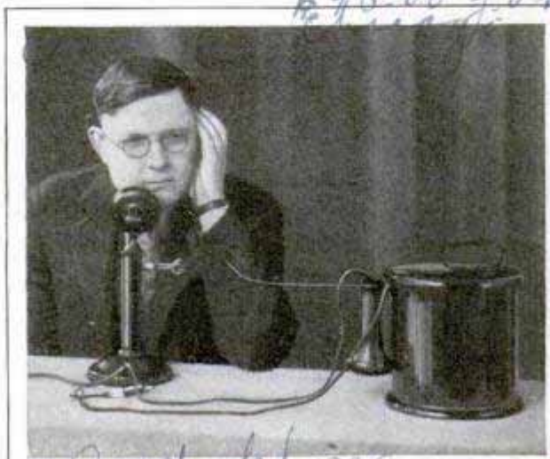
Radio Comes to the Aid of the Deaf in Telephoning; the Amplifying Unit in Use
