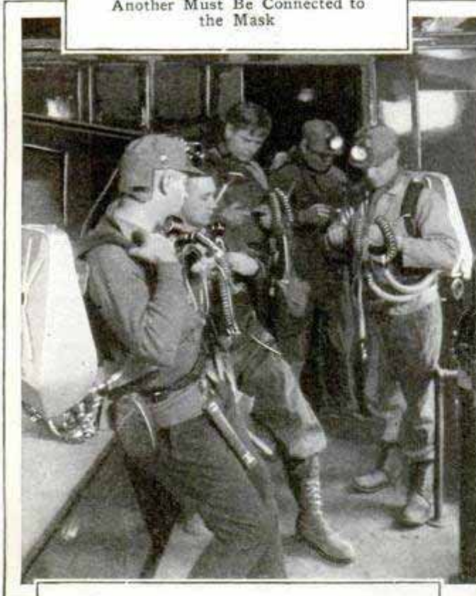
A Rescue Crew Adjusting Oxygen Masks and Tanks before Entering a Burning Mine; the Masks Render Them Immune to Every Form of Gas and Smoke for Two Hours
