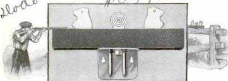
Small Shooting Gallery for Rifle Practice; the Figures Fall When Struck but Reappear if Center Target Is Hit
