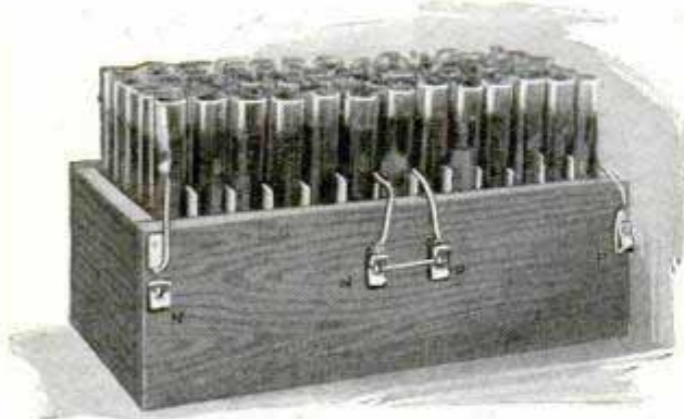
The Completed B-Battery Ready for Use
