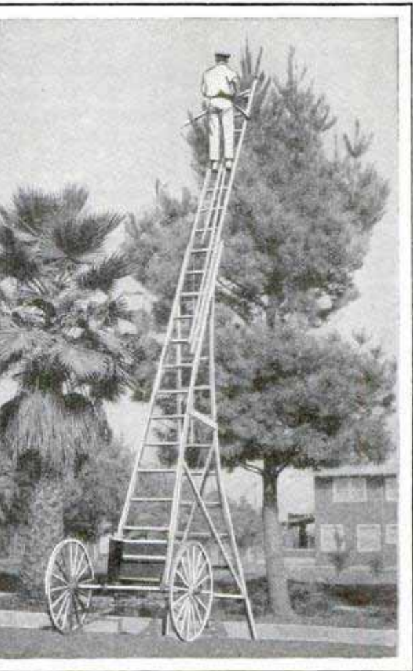
High Folding Ladder for the Tree Trimmer Is Attached to an Auto Trailer
