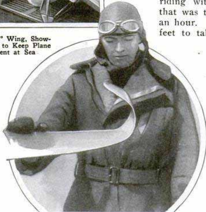
Here Is the Wing Tip of "Bremen's" Steel Propeller, Bent in Landing on the Ice of Greenly Island
