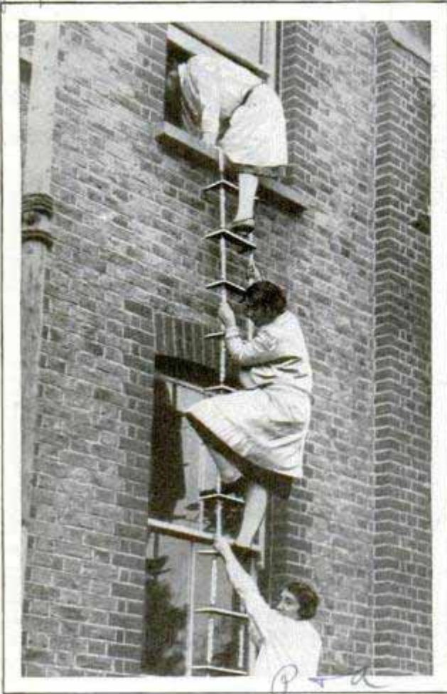
Testing Special Fire-Escape Ladder, Which Is Held to the Wall to Prevent Swaying
