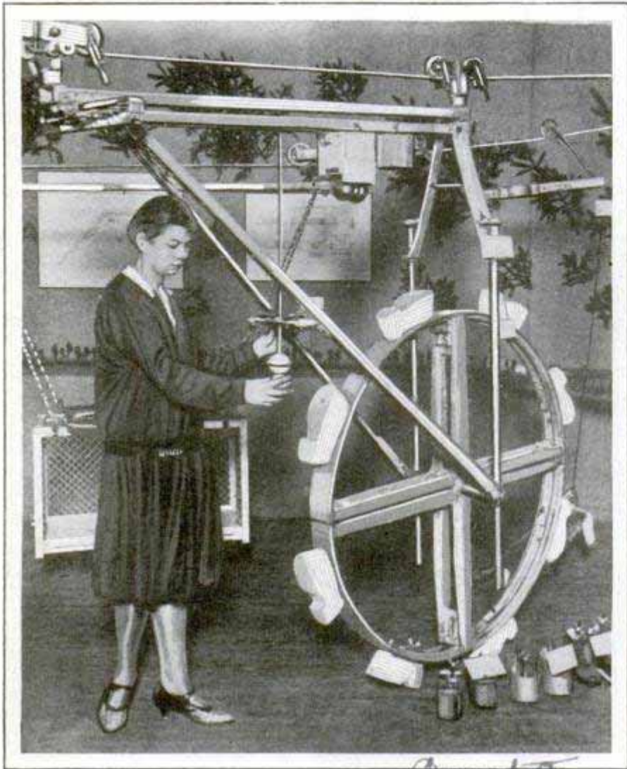
"Walking Wheel" for Testing Dogs' Manner of Following Trail; It Was Run on Cable to Eliminate a Human Attendant
