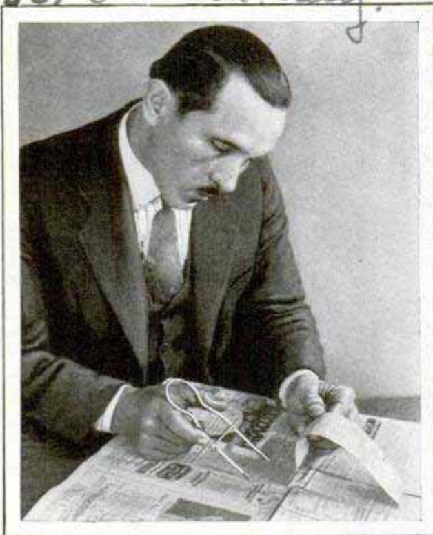
Both Sides of the Newspaper Column Are Cut at Once with This Timesaving Unit
