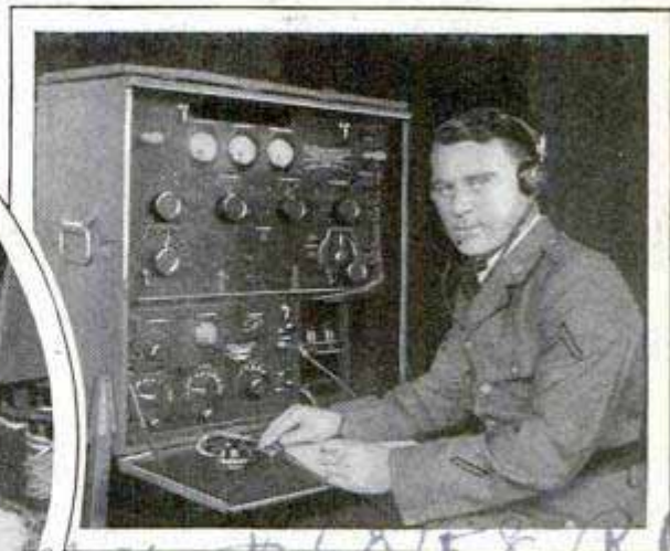
Portable Transmitter, Designed for Signal-Corps Communication with Aircraft. Is Suitable for Either Telegraph or Voice
