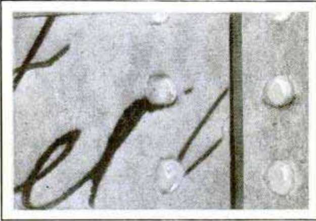
Ink Flowing around Edge of Perforation Showed That Writing Was Made After Paper Was Punched
