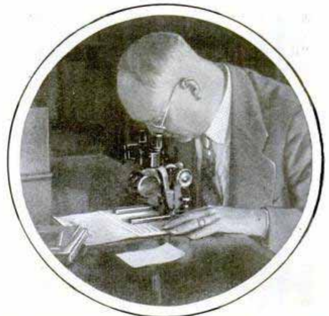
Mr. Wood at the Binocular Microscope That "Gets behind the Lines," Revealing a Surface in Three Dimensions Instead of the Usual Two
