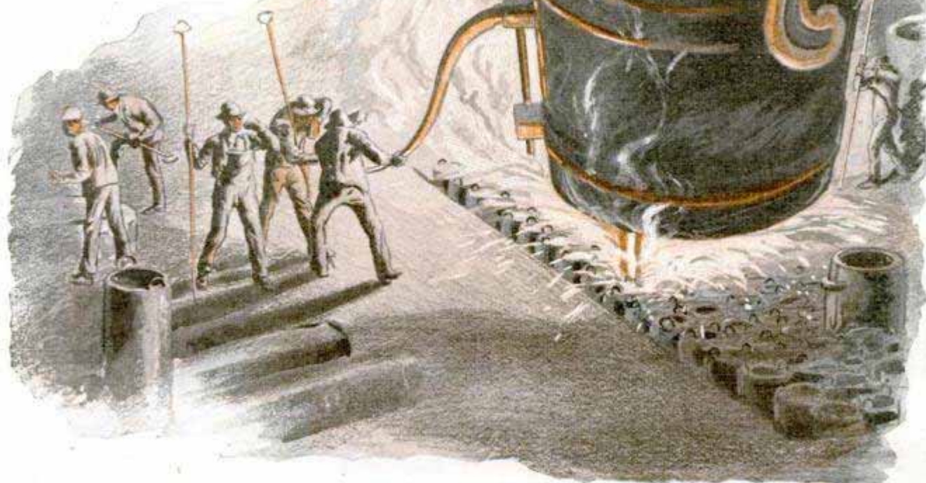
Pouring Castings from a Huge Ladle of Molten Iron in a German Foundry; the Big Pots Are Lined with Thick Walls of Fire Clay to Protect Them from the Intense Heat
