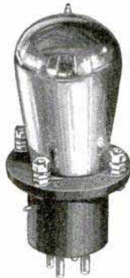
Left, Three-in-One Tube Showing Simple Arrangement of Binding Posts; Right, Diagram of Connections
