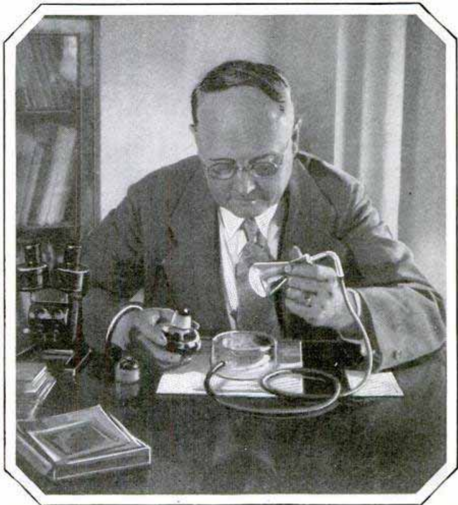
Fuming Operation in Progress; Fumes Pass from Heated Container through the Tube and Spread over the Page, to Restore Faded Ink So That It Can Be Photographed
