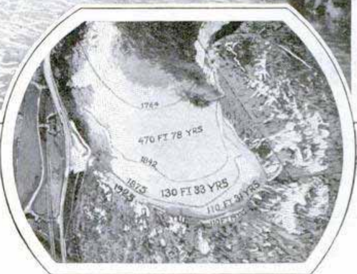
Miniature Niagara Falls Built to Study Conservation Problem, and Aerial Photo of Horseshoe Falls, Showing Crest Lines of Past Years
