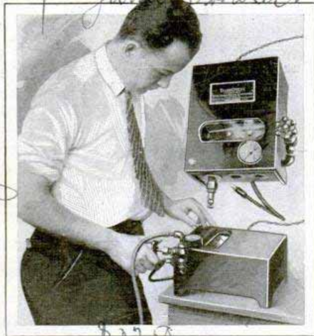
Testing Spark Plugs under Pressure, to Reveal Defects That Might Appear in Actual Operation.
