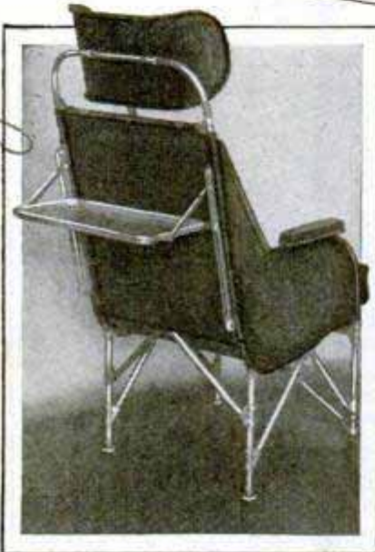
Passengers Who Ride on Air Cushions in New British Liners Can Wear the Seats as Life Preservers; at Left, Food Tray on Back of Seat; Other Views, the Life-Preserver Cushions
