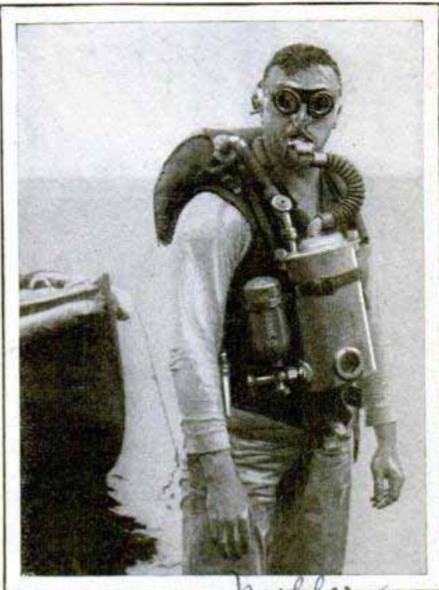
For Diving in Shallow Water; Suit with Air Supply Permits Wearer to Stay Under Ten Minutes
