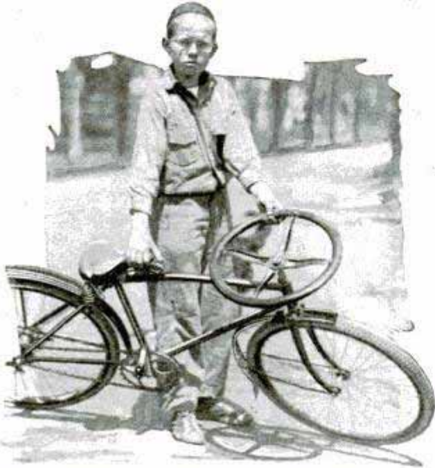
Old Automobile Steering Wheel Substituted for the Customary Handlebars on Bicycle
