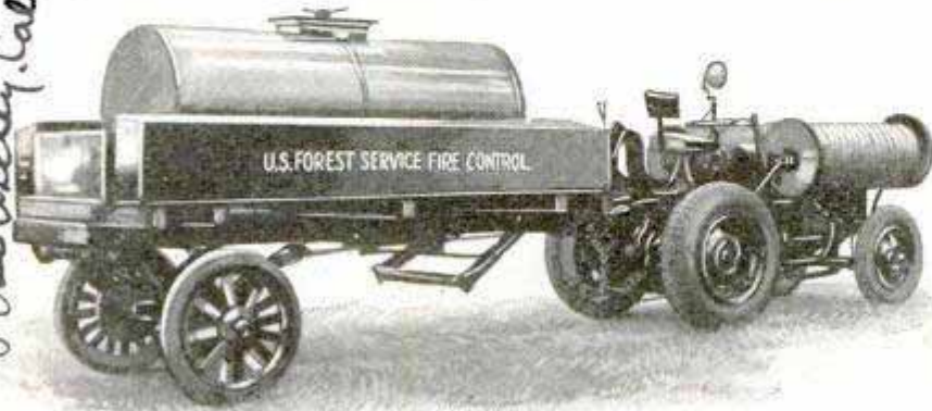
Forest-Fire Engine, Made from Tractor, with Trailer Carrying the Emergency Water-Supply Tank
