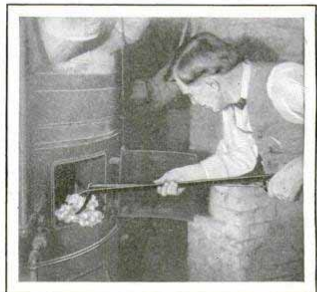
Gripping Tongs That Clutch the Stubborn Clinker, to Effect Its Removal without Shaking the Grates
