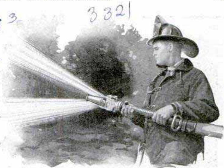
Nozzle Which Breaks the Force of the Fire Spray So That It Will Do Less Damage to Interiors
