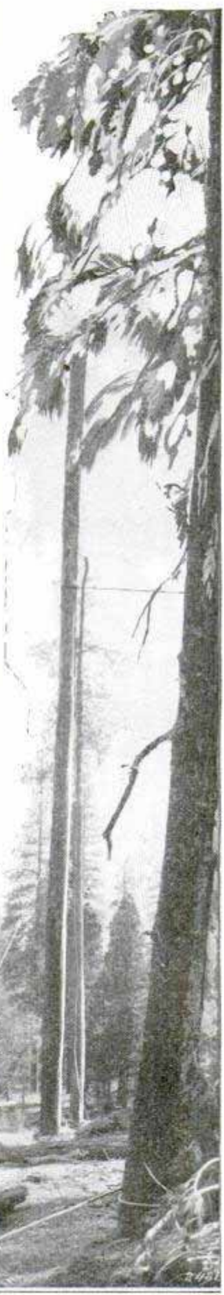
With the "Spar Tree" Set Up and Rigged, the Tractor Is Able to Handle All the Logs for 500 Feet Around, and Later Skyline Them to the Road or Railway
