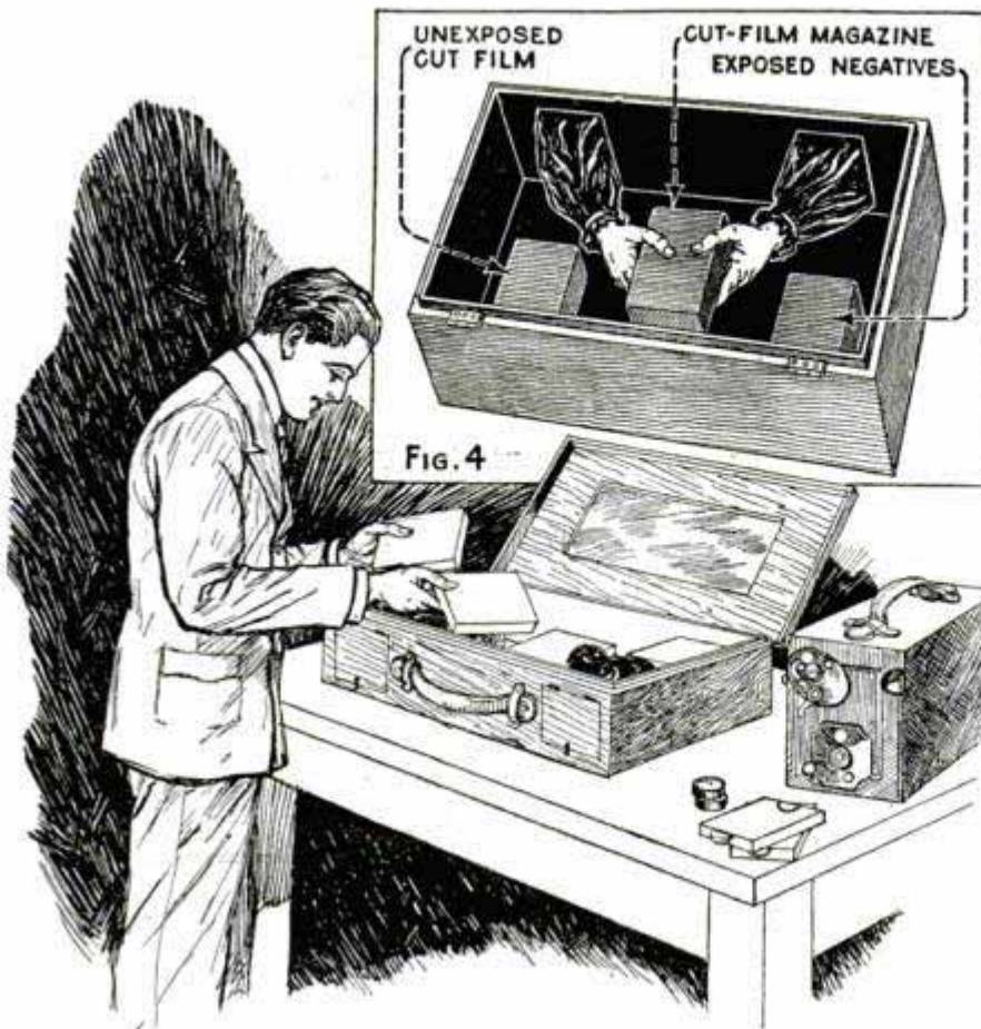
Above, Details of the Loading Box; Below, the Box Serves as a "Carryall," When Not in Use as a Dark Room
