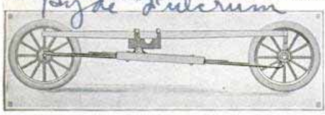
For Smoother Riding in the Small Auto; Drawing to Show the "Cantilever" Springs in Place
