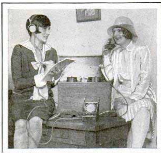
Speech Repeater in Use; Tones of the Voice Are Recorded and Amplified for Study of Defects
