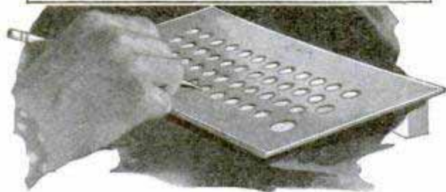
Chart in Use and Close View Showing Perforations That Take Place of Typewriter Keys
