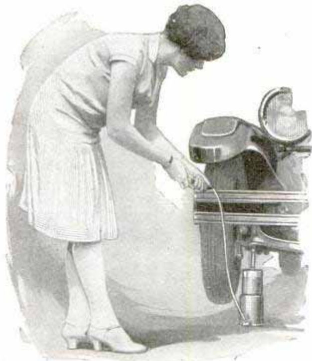
Jack in Place and About to Raise the Car When Compressed Air Is Released by Twisting Tube Handle
