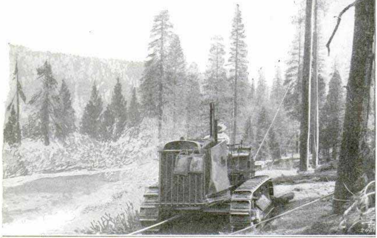
With the "Spar Tree" Set Up and Rigged, the Tractor Is Able to Handle All the Logs for 500 Feet Around, and Later Skyline Them to the Road or Railway
