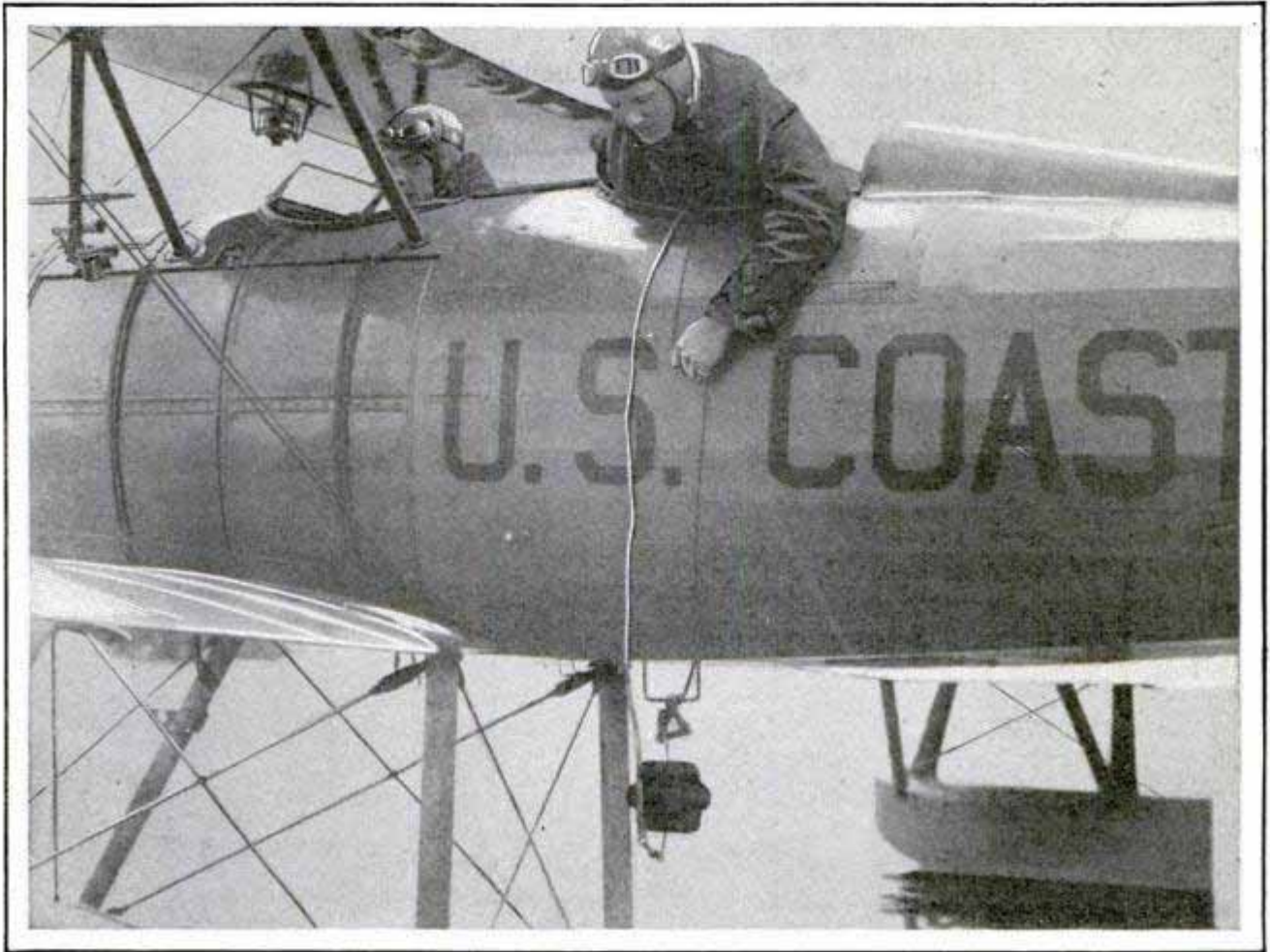
Coast-Guard Flyer Preparing to Drop the Trailing Gear to Pick Up the Life Line as His Plane Races Out to Sea above the Shore Masts Which Replace the Life-Saving Cannon
