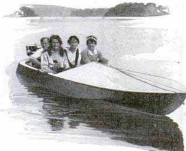
Rubber Speed Boat Carries Four Persons with Ease and Does Not Lose Its Buoyancy
