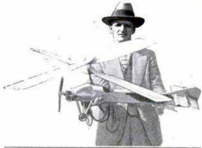
Model Helicopter Plane Which Flies Up or Down and Can Remain Stationary for a Time in Air
