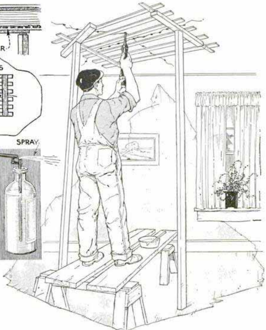
Patching and Re-Anchoring of a Cracked and Sagging Ceiling May Easily Be Done by This Simple Method without Dirt or Fuss
