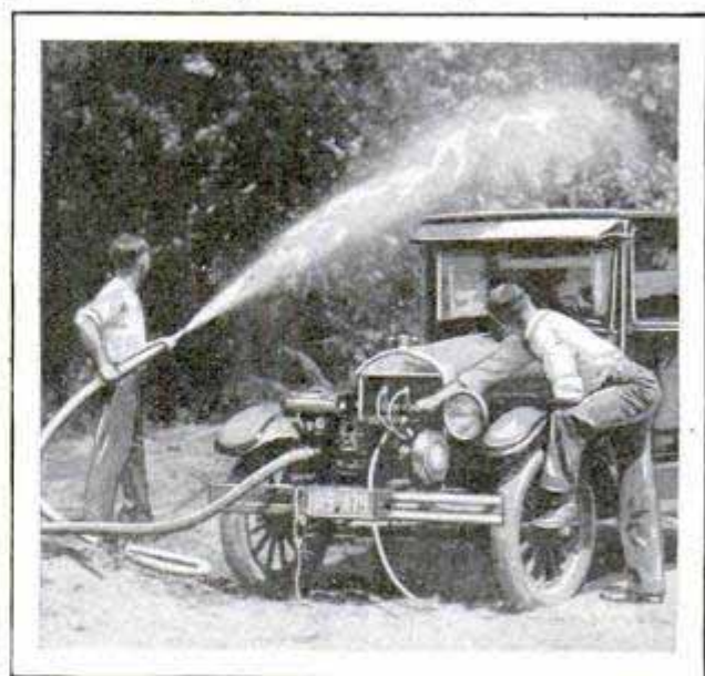
Pump in Action on Front of Auto, Which Has Been Converted into Fire Engine to Guard Forests
