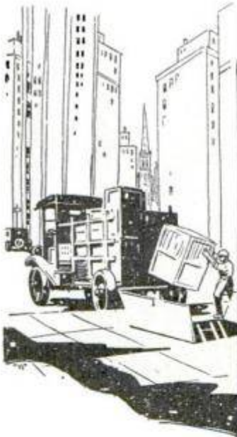
Strong Chute of Angle Iron for Advantageous Handling of Both Barrels and Boxes
