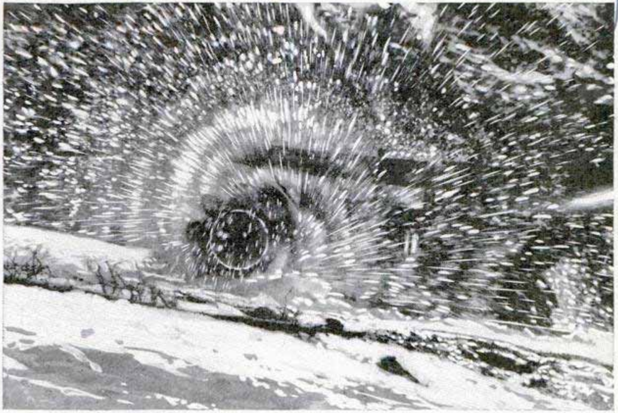
Pinwheels in Snow! Rotary Plow Cutting Its Way through Drifts up Pikes-Peak Motor Road; in Places Surveys Had to Be Made to Find the Hidden Highway
