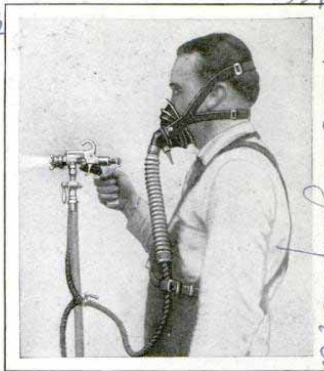
Painter Wearing Mask While Spraying; Note the Line Connected to Main Supply Pipe
