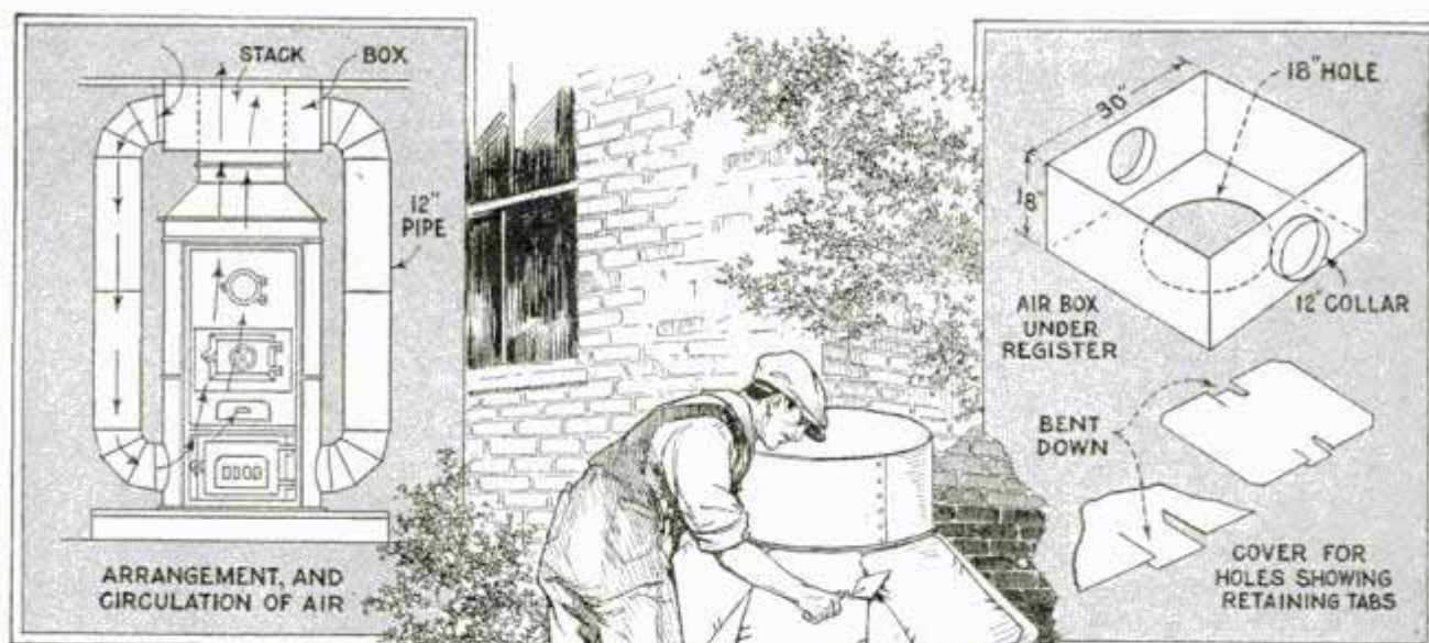
Old-Style Hot-Air Furnace Converted into an Efficient Pipeless Furnace, Which Heats the Entire House; the Cost of the Furnace Amounts to Only Fifty Dollars
