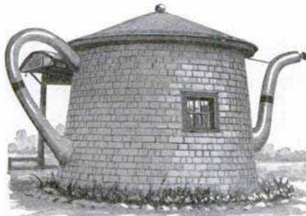
Teapot Service Station Attracts Attention and Proves Practical; the Spout Serves as Chimney
