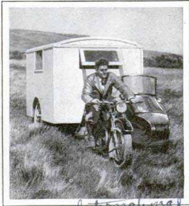
Trailer and Sidecar Fit This Motorcycle for Carrying the Camping Party and Equipment
