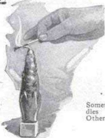
Safe and Clean. This Household Incinerator Has a Spark Arrester at the Peak of the Stack, Is Lighted from the Top and Burns Contents Thoroughly
