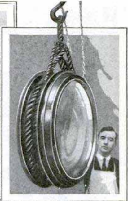
Twenty-Six and a Half Inch Object Lens for a Big Refracting Telescope, Ground and Mounted Ready to Be Installed; the Workman Gives a Comparison to Show the Size of the Big Glass
