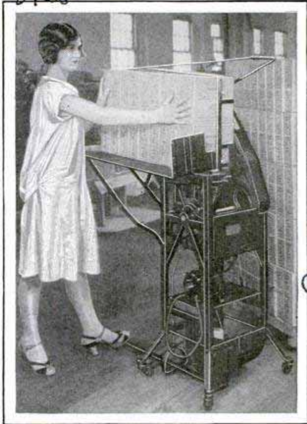
Package Tier in Operation; String Is Easily Passed over Entire Bundle and Machine Is Movable
