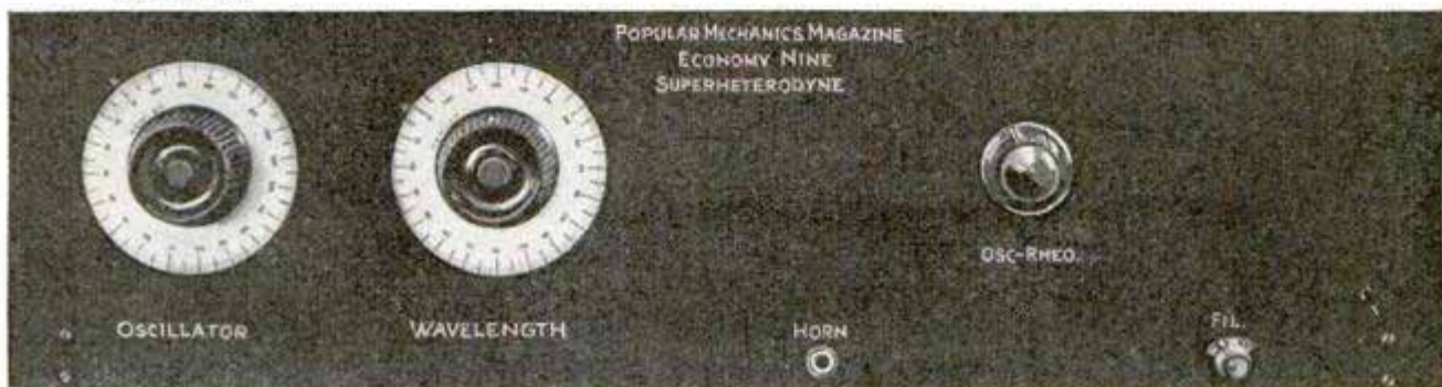
Above, Schematic Diagram; Below, Close-Up of Front Panel, Showing the Simple Controls, the Horn Jack and the Filament Switch
