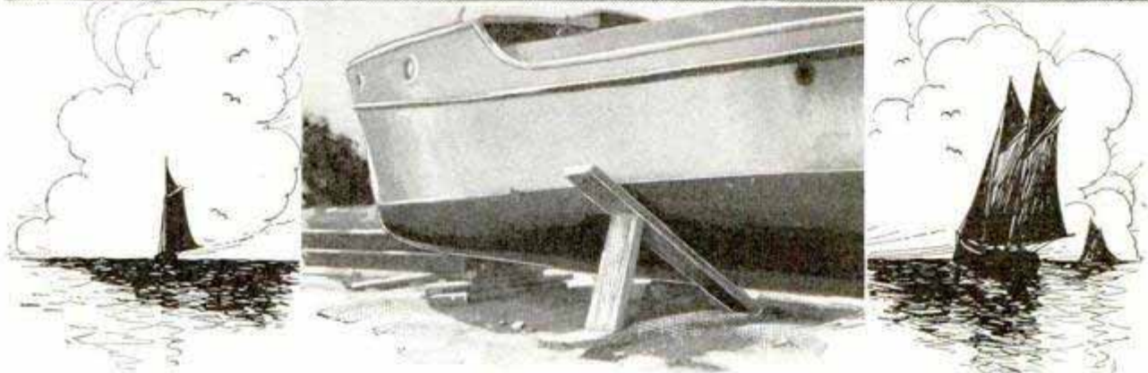
Top, Cradle on the Ways with Tackle Attached, Ready for Hauling When the Tide Rises; Center, Methods of Bracing Boats on Hard and on Sandy Ground; Bottom, a Good Method of Shoring on Firm Ground
