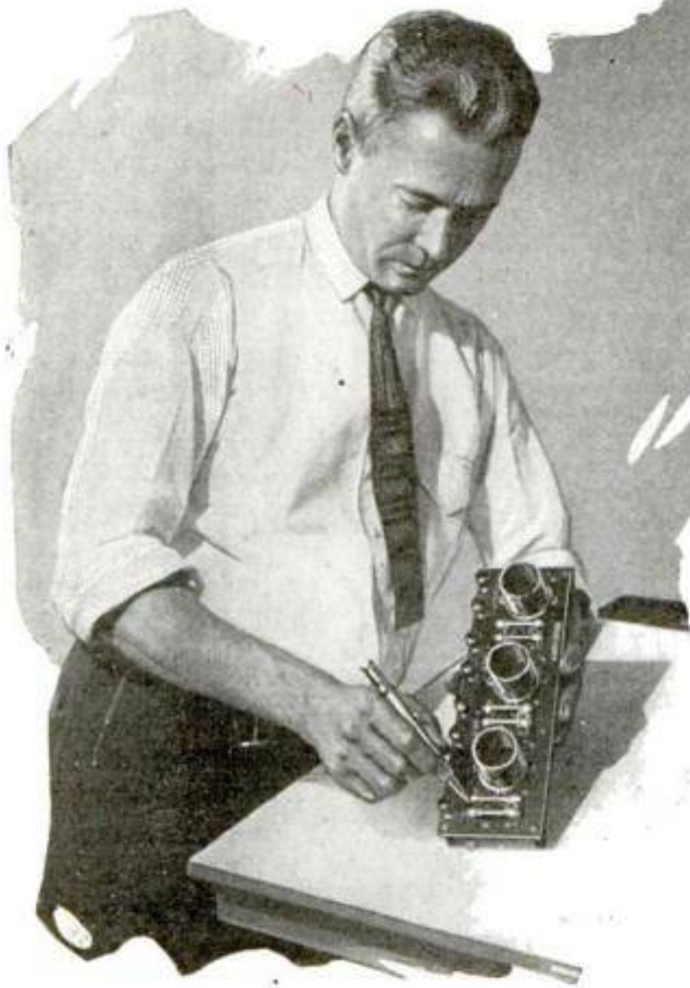
Above, Testing 45-Volt B-Battery Unit; Left, Pointing Out Resistor in Plate Circuit of Detector Tube
