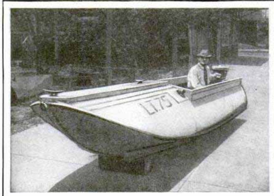
Pontoon of Flying Boat, Which Serves as Separate Craft
