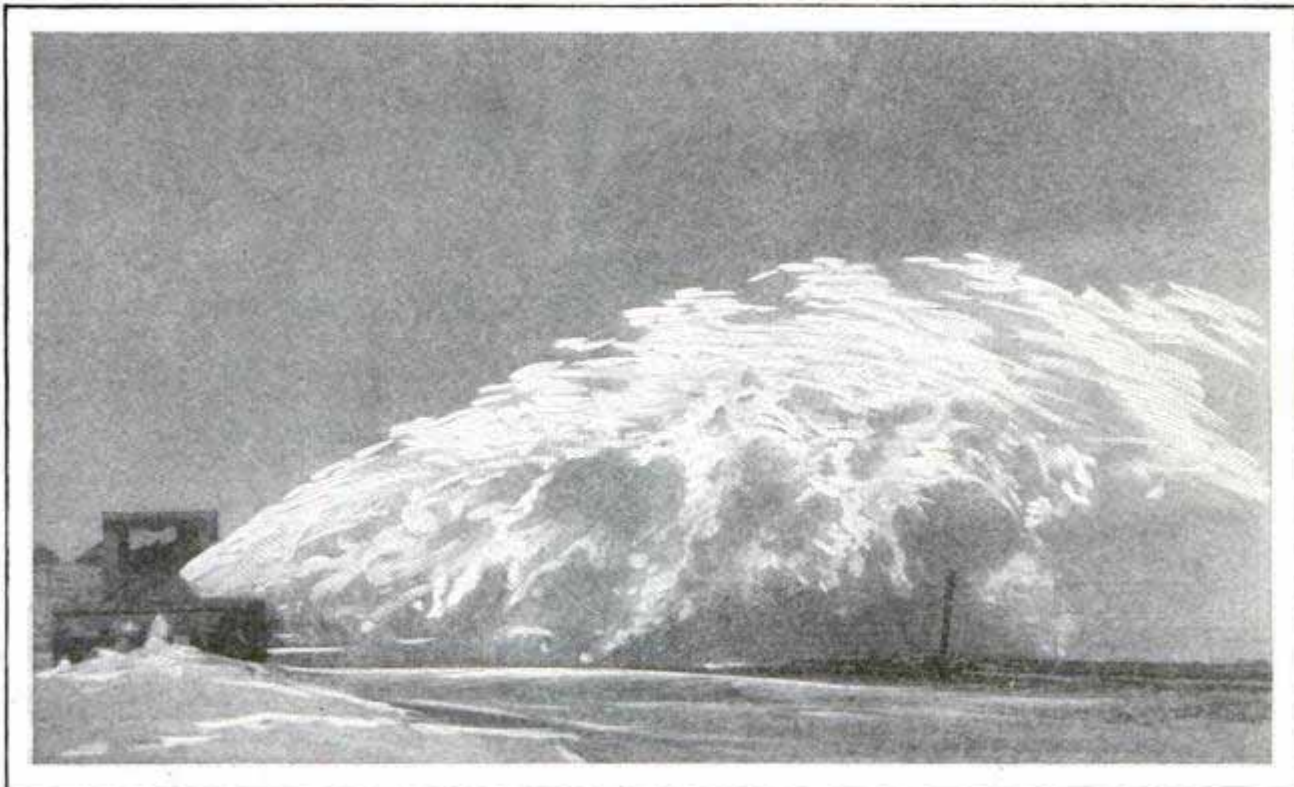
Boring through a Drift and Throwing the Snow over the Fence; the Machine in Action, Illustrating Its Powerful Blowing Force; It Is Said to Operate Effectively in All Kinds of Snow
