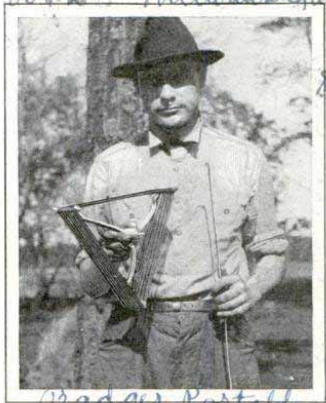
Reel Extended, Showing the Projecting Arms and Screw for Attaching It to Wall
