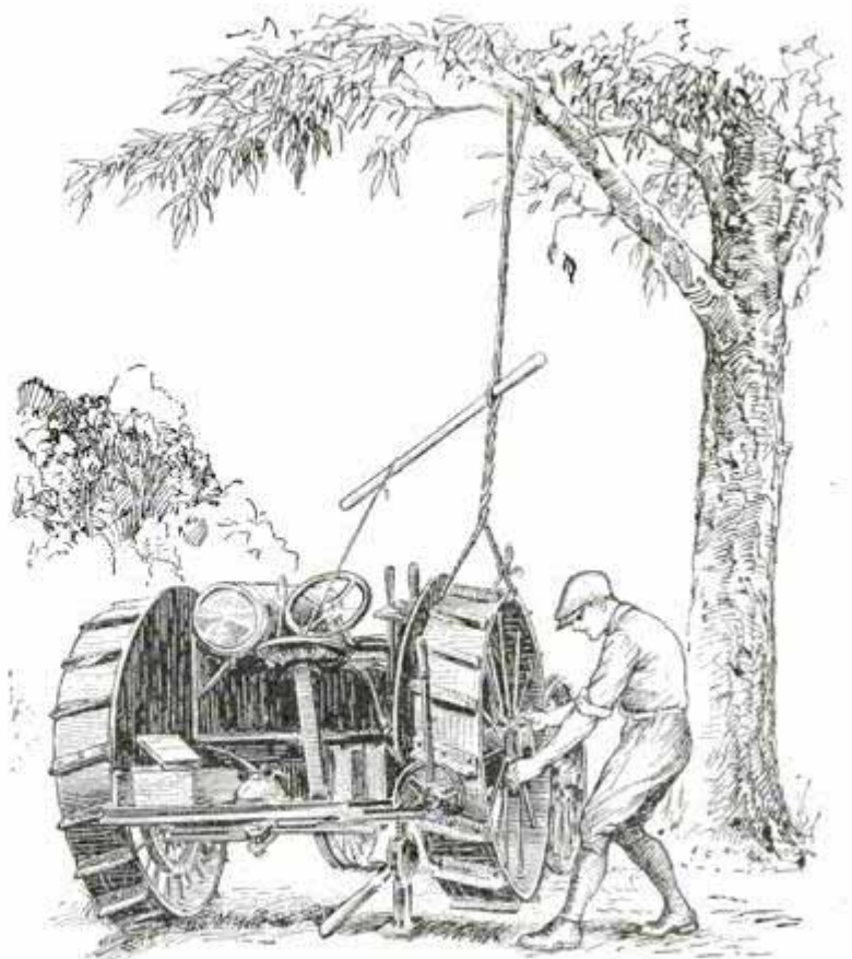
Heavy Wheel of Farm Tractor Can Be Removed Single-Handed with the Aid of This Sling
