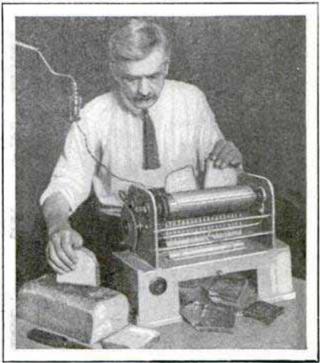
Toasting Bread in the Roller Unit; Speed and Even Browning Are Special Features of the Machine
