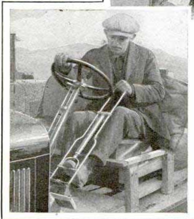
How Much Pressure Does It Take to Operate Your Clutch? The Testing Engineers Do Not Guess, But Use This Spring Scale to Get Accurate Figures
