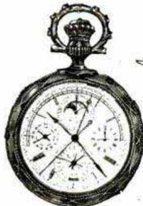
Weather Prophet, Watch and Compass, All in One; the Instrument Has 292 Parts
