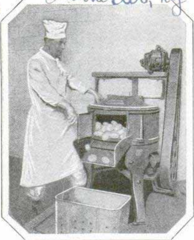
Robbing the Walnut Harvest of Its Most Unpleasant Feature, Removing the Hulls in Motor-Driven Machine
