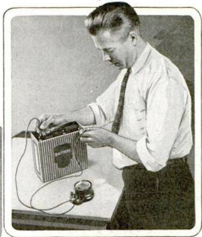
Above, Testing 45-Volt B-Battery Unit; Left, Pointing Out Resistor in Plate Circuit of Detector Tube
