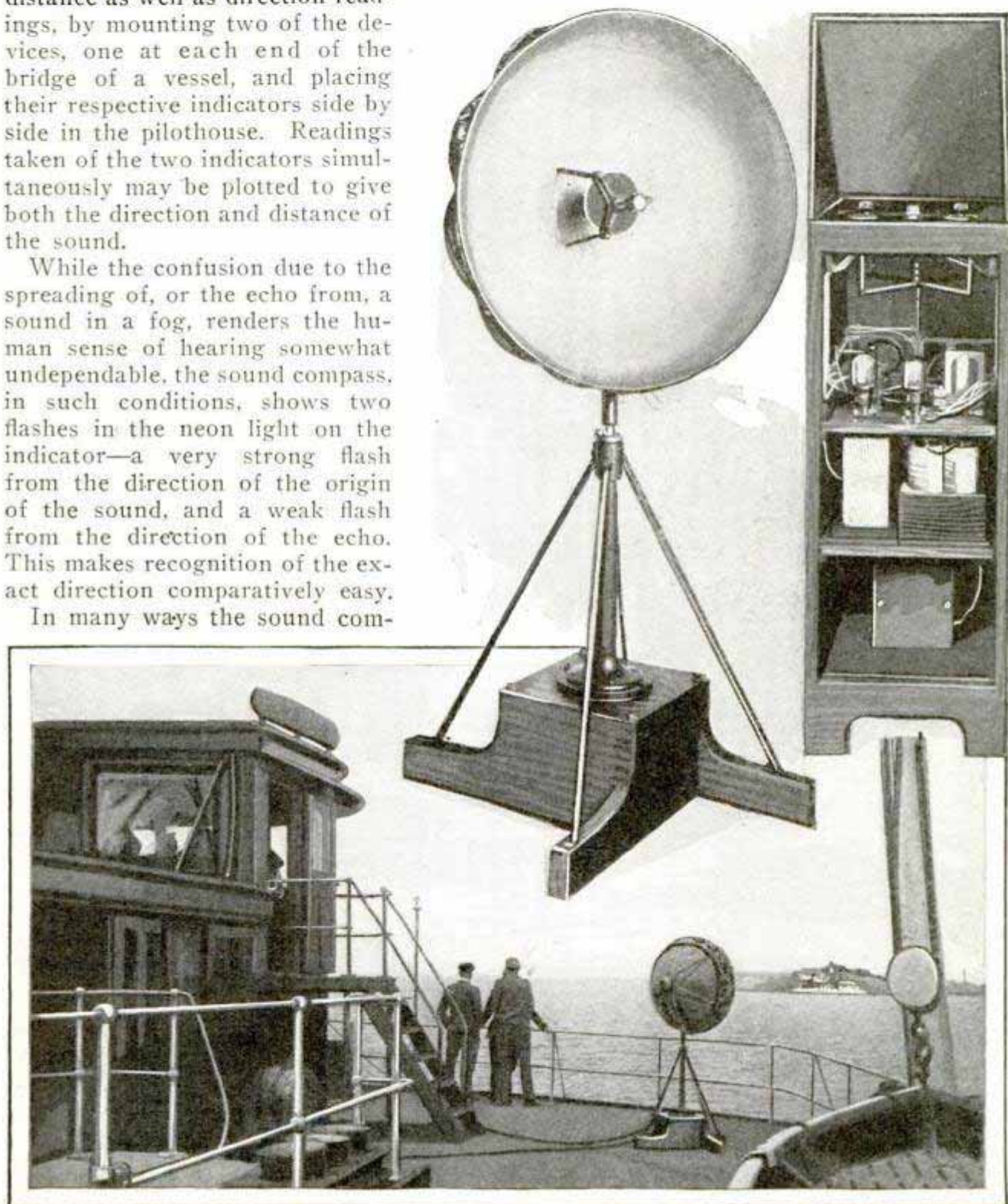
Receiver of the Sound Compass in Position at the Bow of a Frisco Bay Ferry, and, Above, the Front of the Receiver and the Recording Cabinet to Which It Is Connected
