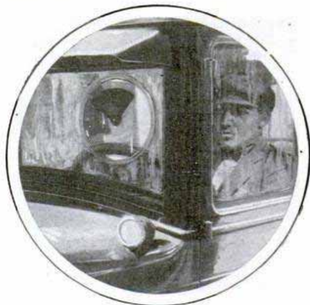
Circular Disk in Place on Windshield, Showing How It Clears a Wider Space for the Driver's Vision
