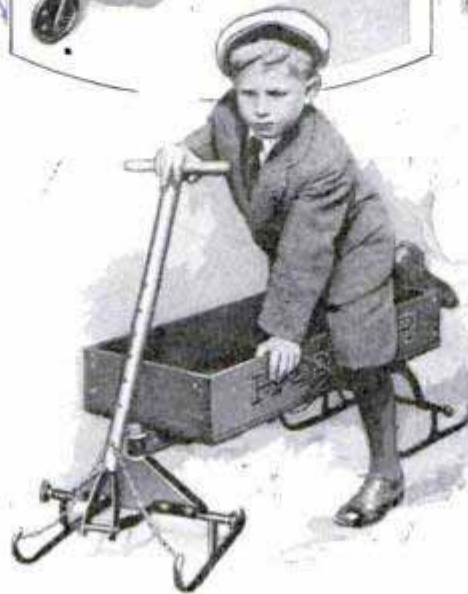
Four of the Vehicles Made from the Coaster Set; Parts Are Securely Held Together with Bolts Instead of Nails
