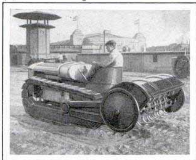
For Short Turns in Small Fields, This Tread-Drive Tractor Has Been Found Successful
