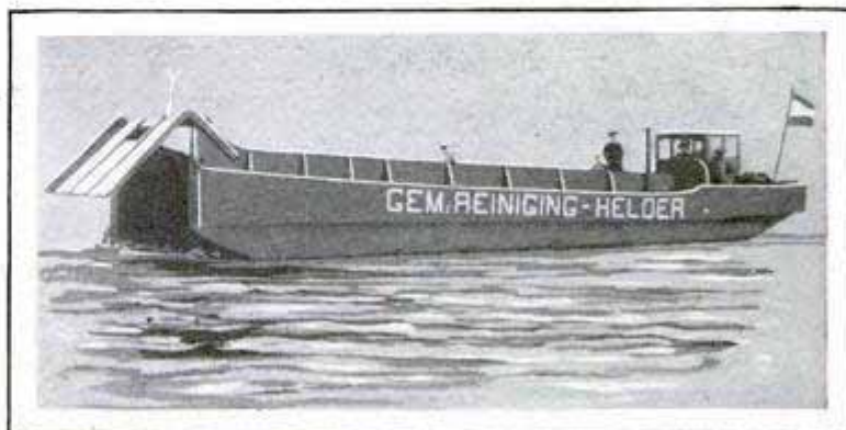
Hatch at Bow of Refuse Boat Raised to Permit Dumping; a Thirty-Ton Load Can Be Dropped in Eight Minutes
