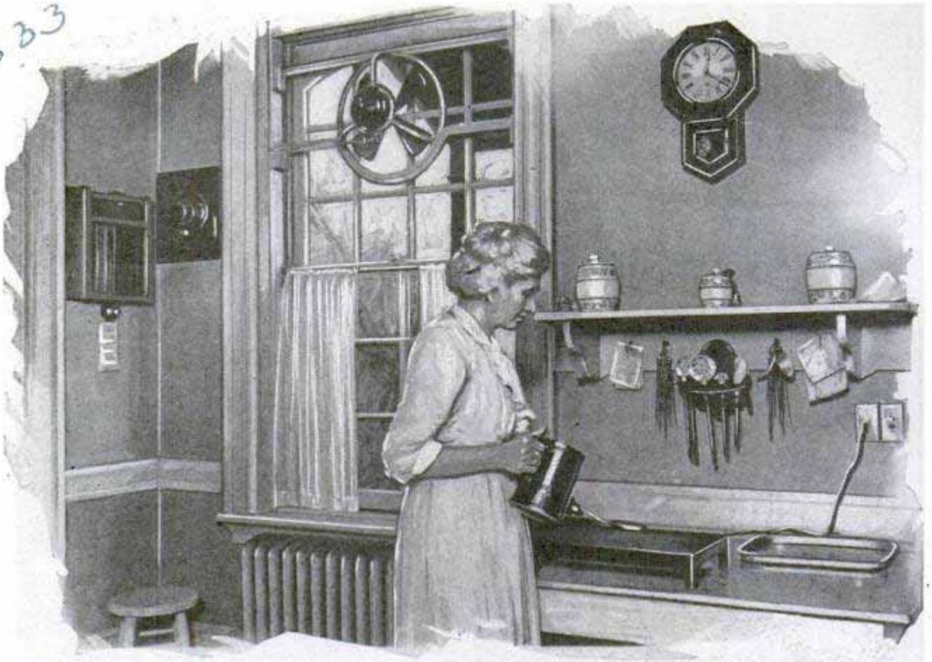
Mrs. Thomas A. Edison, Wife of the Famous Inventor, in Her Kitchen; Note the Electric Plate and the Ventilating Fan Mounted in the Window to Exhaust the Hot Air
