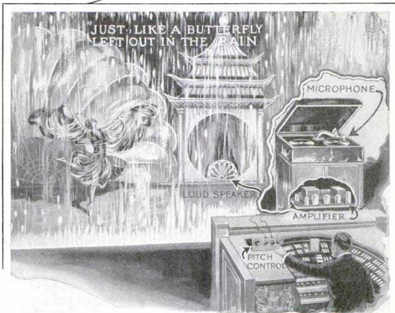
Artist's Drawing, Showing Arrangement of the Amplifying Phonograph, Position of the Loud Speaker and Pitch Control on Organ Console; Dancer and Setting Are Partly Concealed behind Curtain
