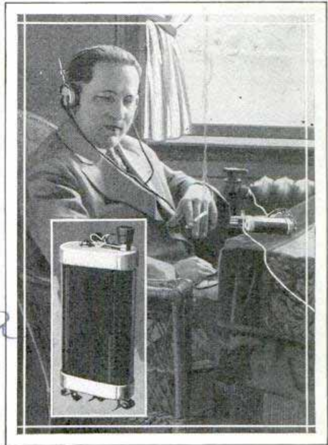
Vest-Pocket Set in Use, Showing Simple Connections; Insert Is About One-Fourth Actual Size
