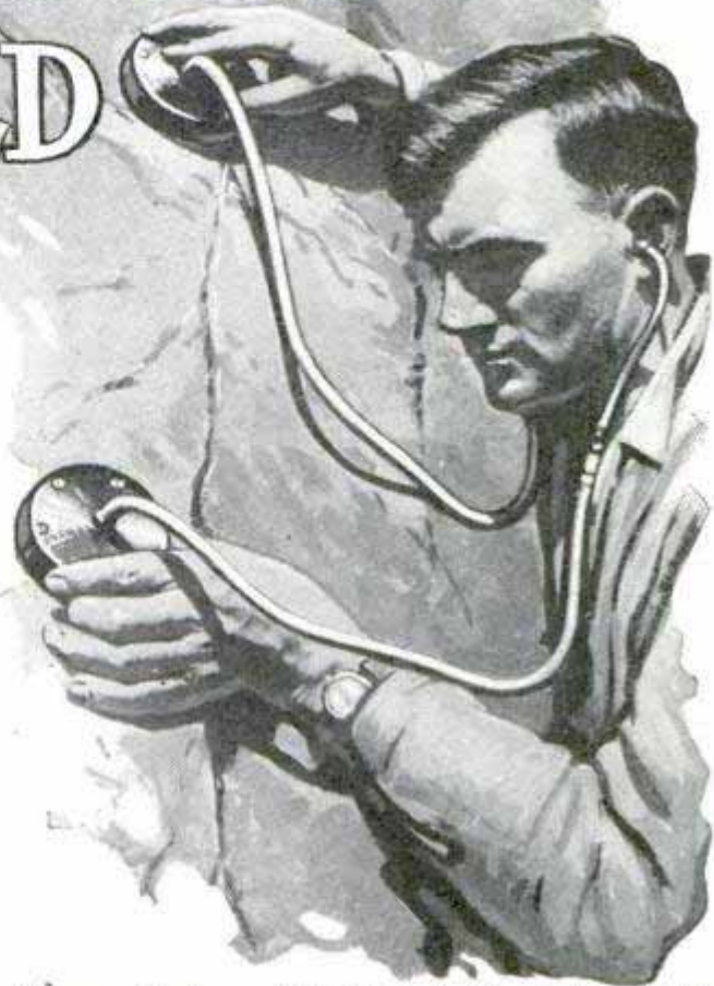
Using a Geophone, Which Detects Sound through the Rock, to Trace the Development of a Mine Fire
