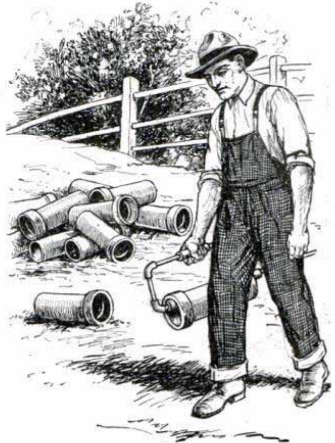
Handy Tile Carrier Made of Pipe and Fittings Eliminates the Necessity of Frequent Stooping
