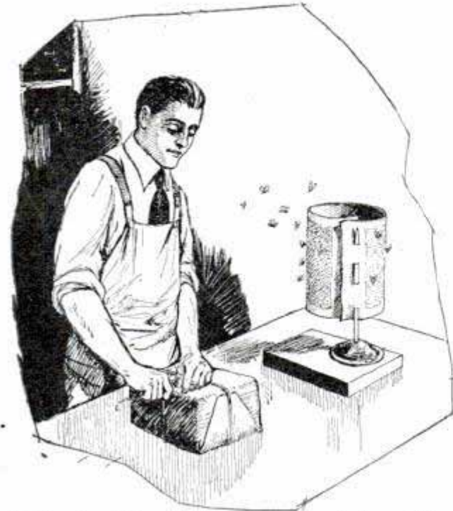
Holder for Sticky Flypaper Prevents It from Being Shifted by Breeze
