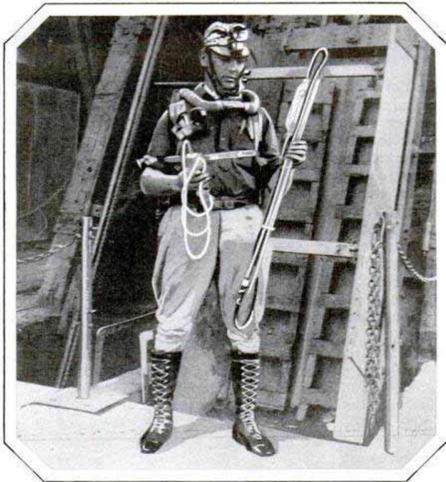
Bringing Up an Air Sample in a Sealed Glass Tube from a Burning California Mine, to Enable Expert Chemical Analysis to Be Made
