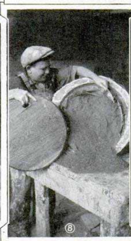
Applying First Plaster-of-Paris Coating by Throwing Motion of the Hand; the Entire Surface Is Coated in This Manner
