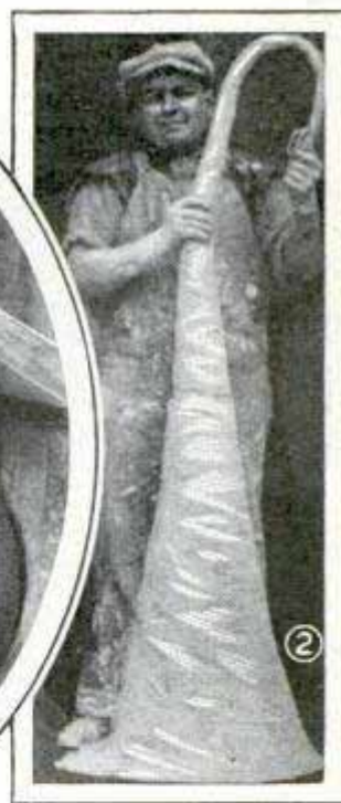
Sack Filled and Ready for Clay Covering; Left, How the Clay Coating Is Applied
