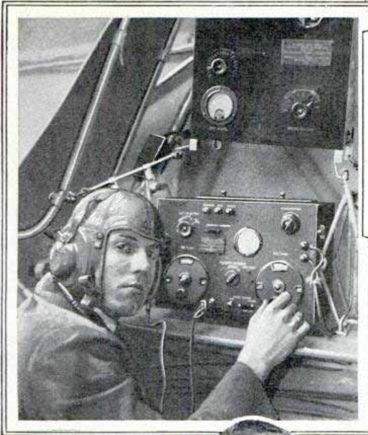
The Radio Set That Kept the "America" in Constant Touch with the World throughout Its Long Flight; the Operator Wears a Soundproof Helmet with Built-In Earphones to Eliminate the Roar of the Three Giant Engines
