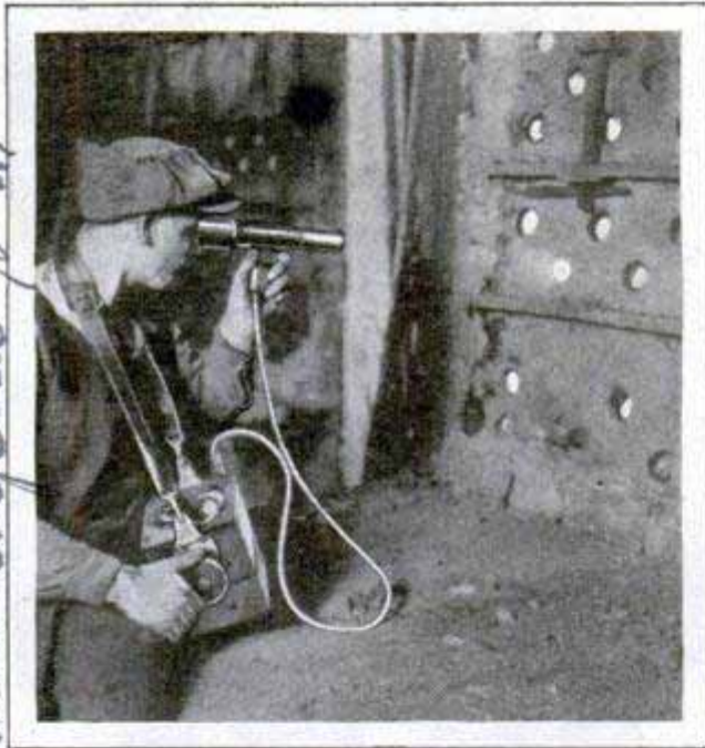
Testing the Temperature of the Furnace by Examining Color of Flames through Special Telescope
