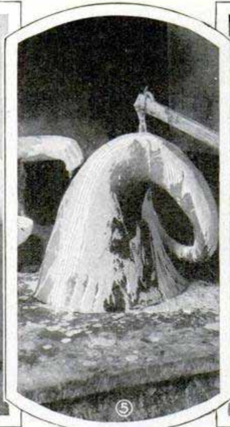
Applying First Plaster-of-Paris Coating by Throwing Motion of the Hand; the Entire Surface Is Coated in This Manner
