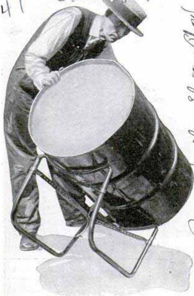
For Easier Pouring from a Barrel; the Tipping Rack in Operation; It Is Made of Metal
