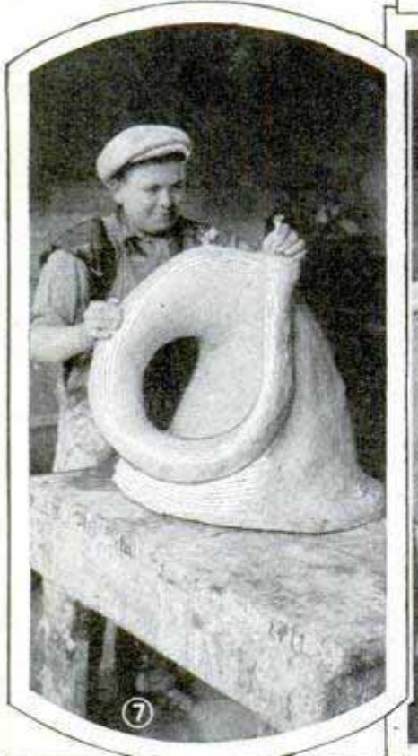
Completed Casting, Showing Small Coil Joined to Large Section; the Rope Extends beyond Mounting Point for the Loud-Speaker Unit
