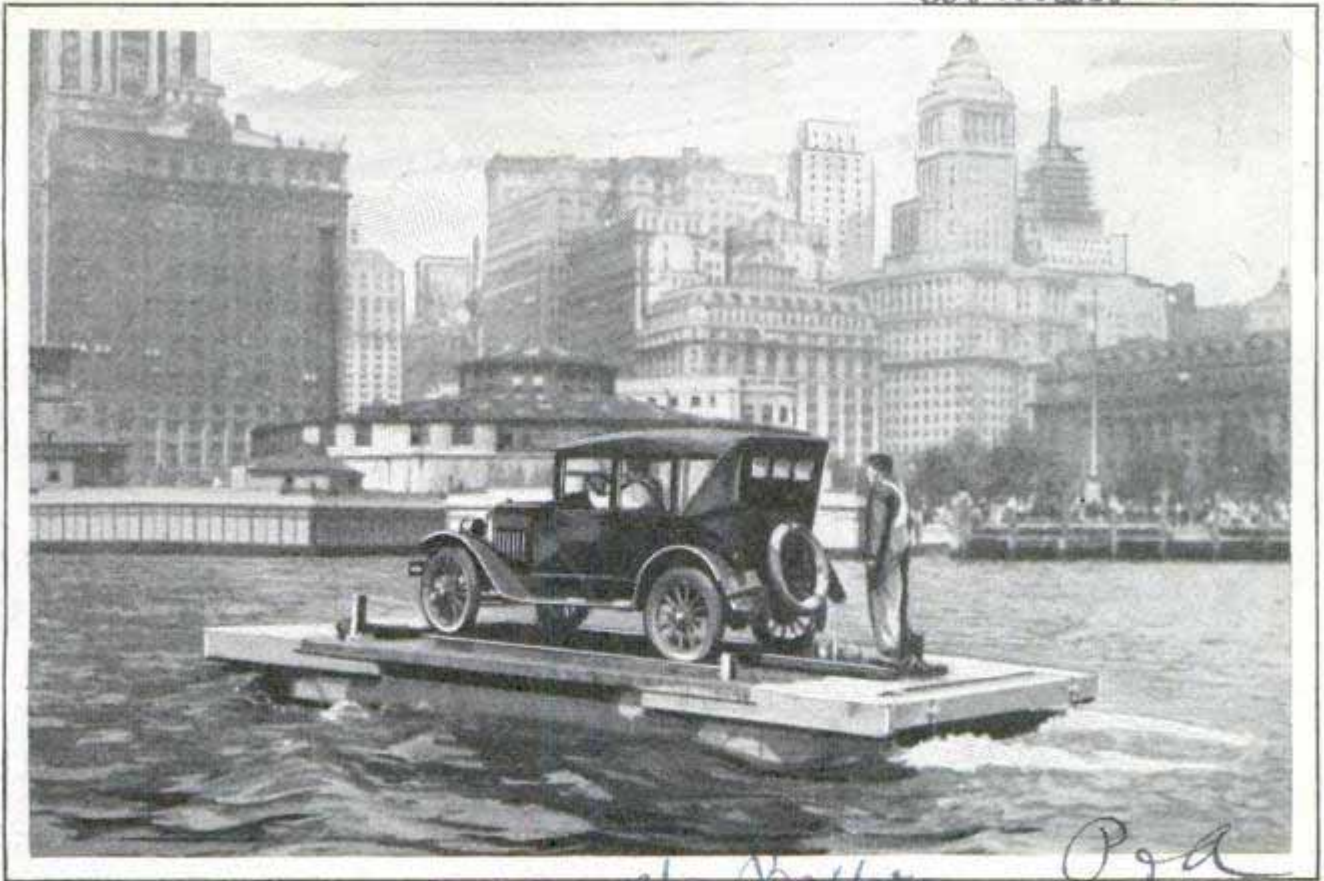
One-Car Ferry for Crossing the North River in New York; It Is Steered through the Automobile's Own Steering Gear and Requires Only One Man to Operate It besides the Car Driver
