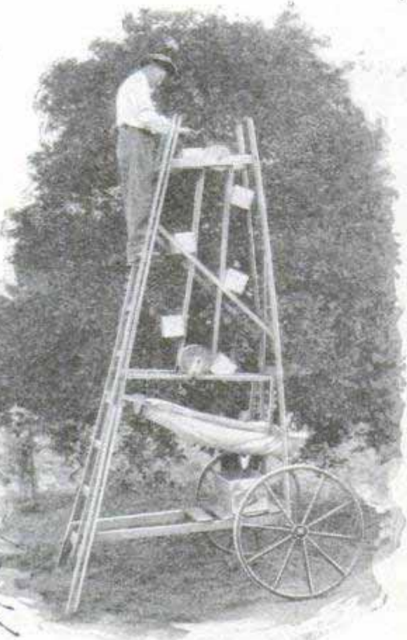
Tower in Operation; Fruit Is Placed in Small Baskets on Endless Belt and Dumped into Box Below
