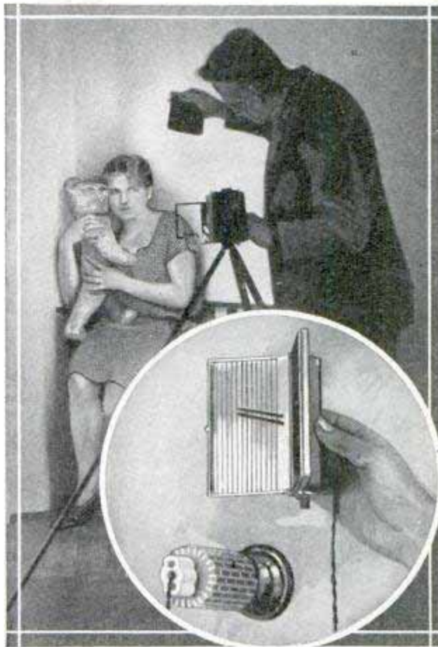
Using the Arc Light to Take a Picture, and Close View of Its Construction and Connections
