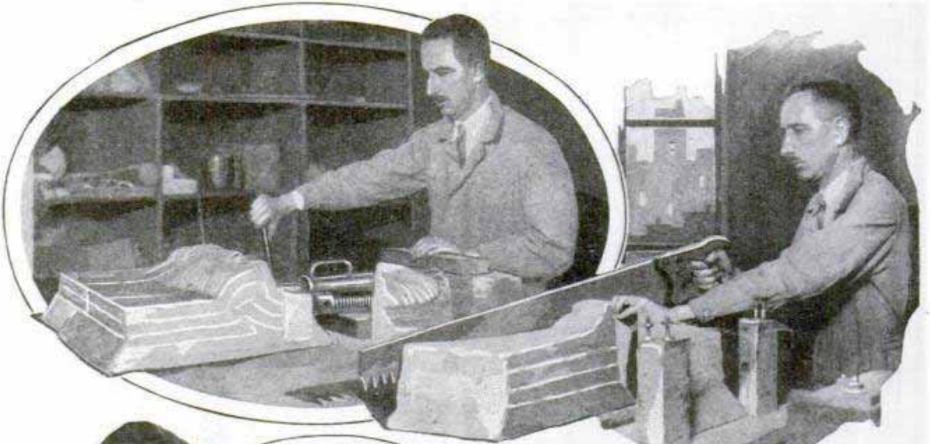
Dr. Link Applying Lateral Pressure to Model Mountains in Laboratory, to Illustrate How Appalachians Were Probably Formed; Right, Sawing a Block for Better Examination of the Strata
