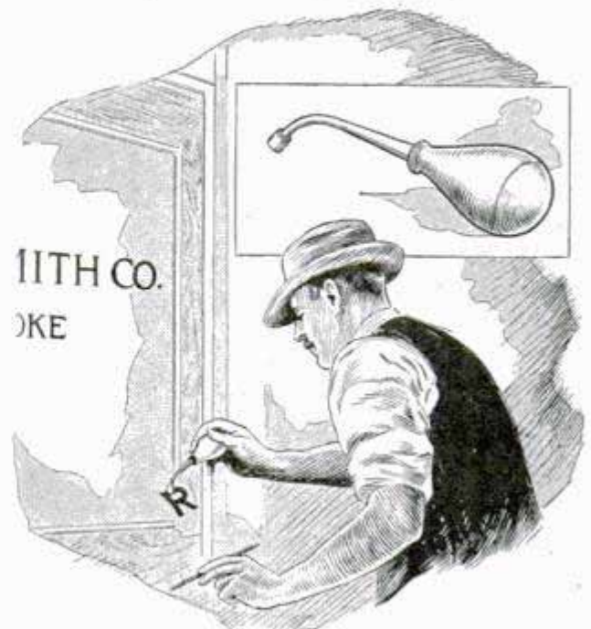
Holding Gold-Leaf Letters with a Small Air Syringe
