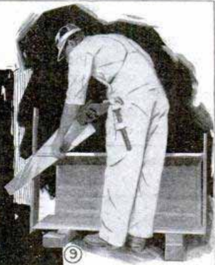
Fig. 9 Starting Cut for Lid; Fig. 10, Detail of the Corner Joint
