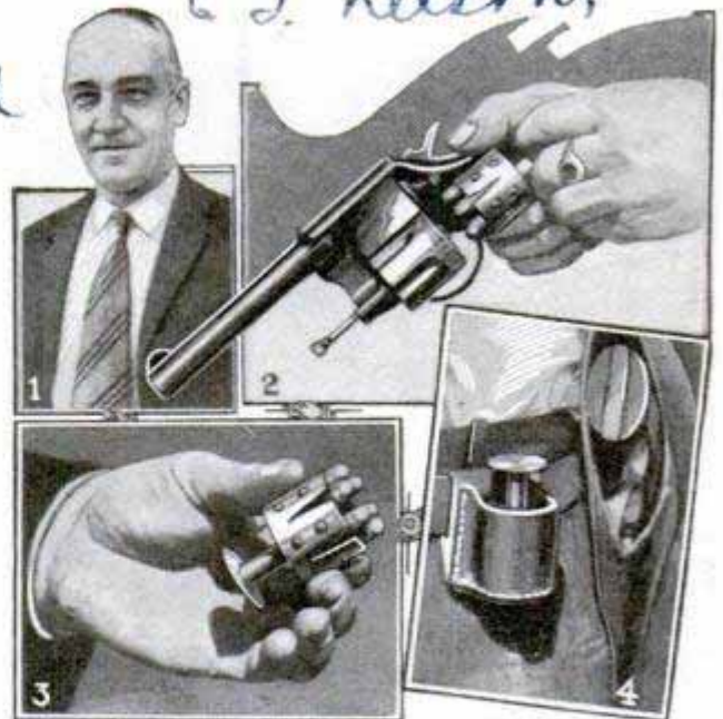
Inventor E. L. Nelson and Three Views of the Revolver Loader; Inserting It, Detached, and How It Is Worn
