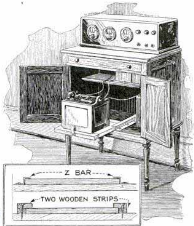
False Bottom in Console Holds Battery, and Slides Out to Facilitate Testing
