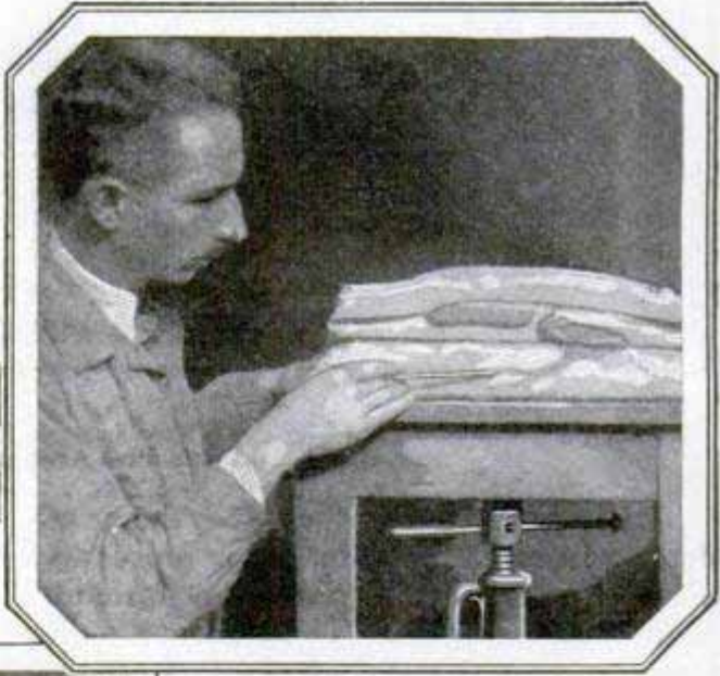
Grease as Lava, Forced between Layers of Concrete and Plaster, to Illustrate Ridge Formation
