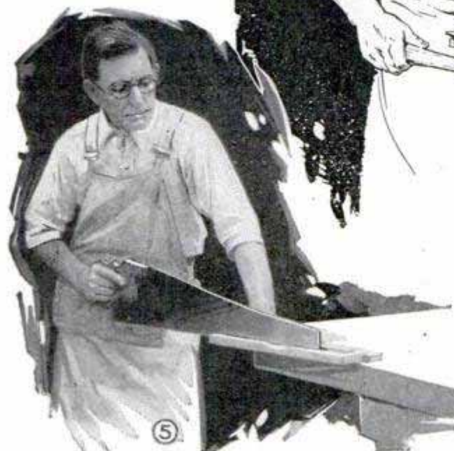
Fig. 2, Squaring across the Ends; Figs. 5 and 6, Cutting the Rabbits on the Endpieces
