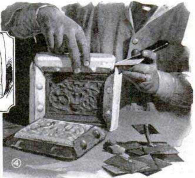
Fig. 4. Separating the Pieces of the Mold; Fig. 5. Tying Mold for Casting; Insert, Varnishing Mold Edges
