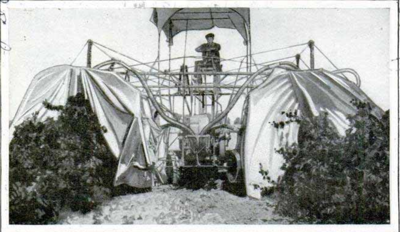
Killing Insects on Two Rows of Plants at Once, the "Spider" Fumigator in Operation; the Canvas Tents Keep the Dust from Blowing Away Too Soon and Help Expose the Branches
