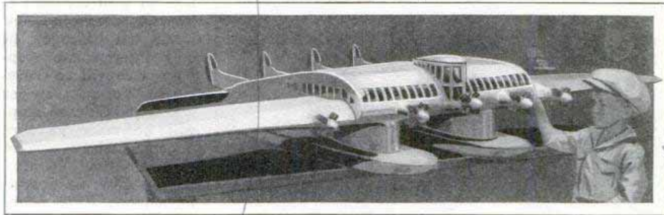
Model of the Aerial Yacht Which Is Planned to Carry Ten Persons at a Time from Los Angeles to Paris; It Will Have Five Motors of 300 Horsepower Each, Two to Be Kept in Reserve
