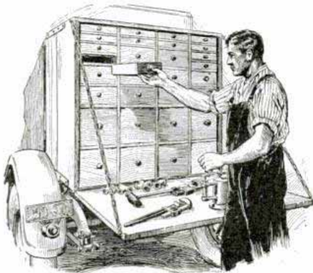
Plumber's Handy Tool Chest and Workbench Fitted at the Back of His Car
