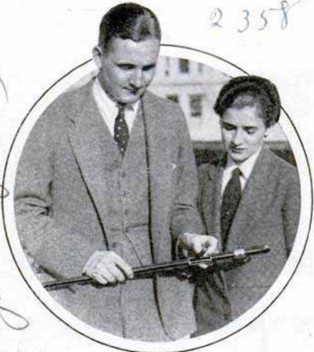
Handle of Cane Pulled Back to Expose the Gun; Weapon Is Quickly Made Ready for Firing
