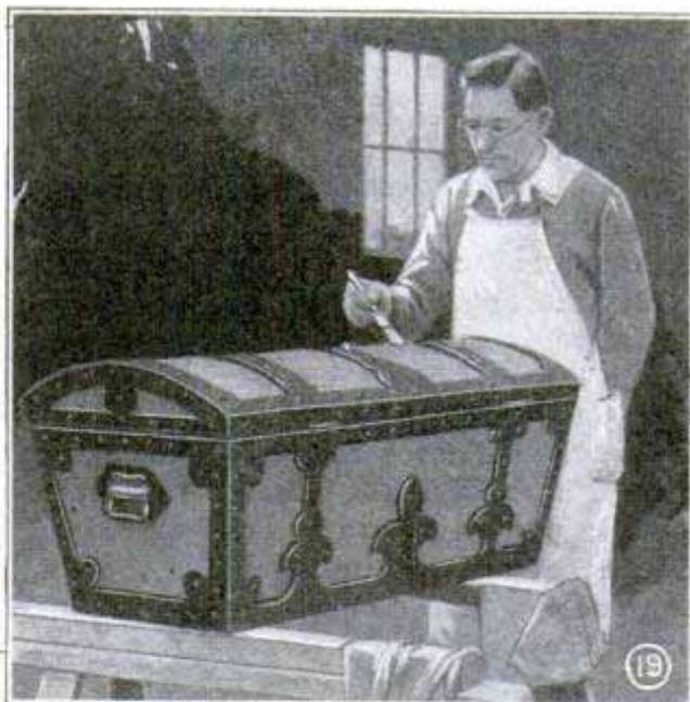
Fig. 17, "Peening" the Linoleum; Fig. 18, Mortising for the Hinges; Fig. 19, Staining the Finished Chest
