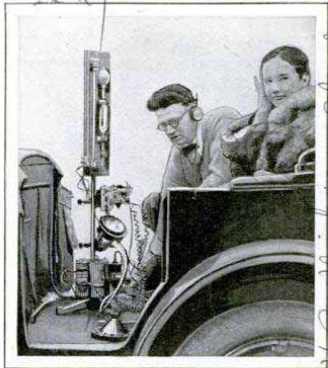
Measuring the Comfort of an Auto Seat with Instrument Devised by Bureau of Standards
