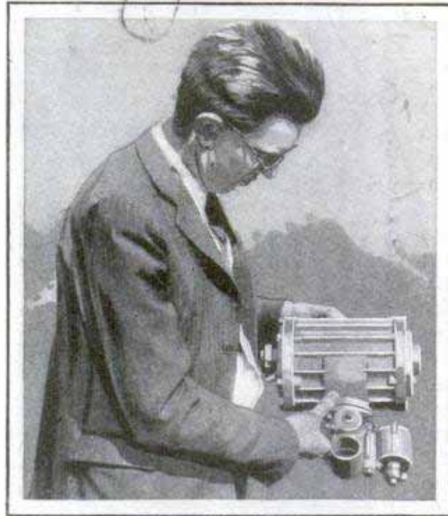
Examining a Supercharger Built for Passenger Cars, with Carburetor Attached
