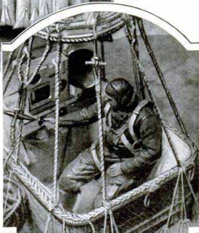
Capt. Gray Demonstrating the Usual Method of Dumping Sand Ballast; His New Sand Bags, Center, and at His Radio, Below
