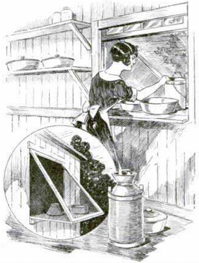
Screened Shelf Outside of the Window Permits Proper Airing of Dairy Utensils
