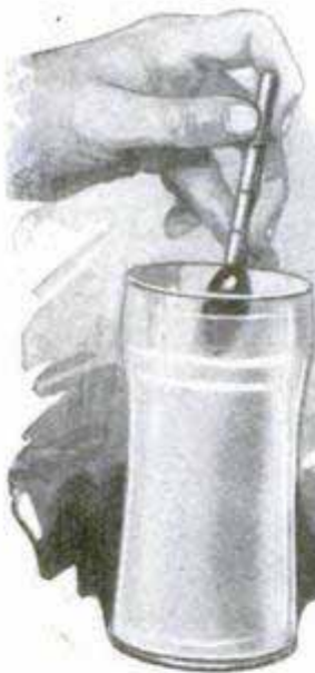
Metal Clamp Holds Dishcloth or a Cork for Scouring and Utilizes Last Bit of Steel Wool, Reducing Waste
