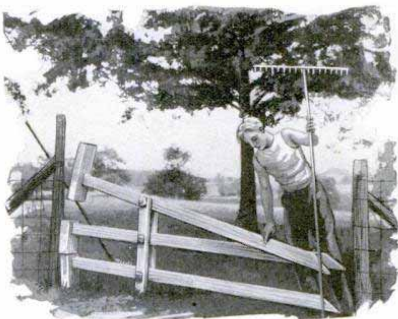
Novel Gate Permits Easy Passage of Persons and Drops Back into Position Automatically
