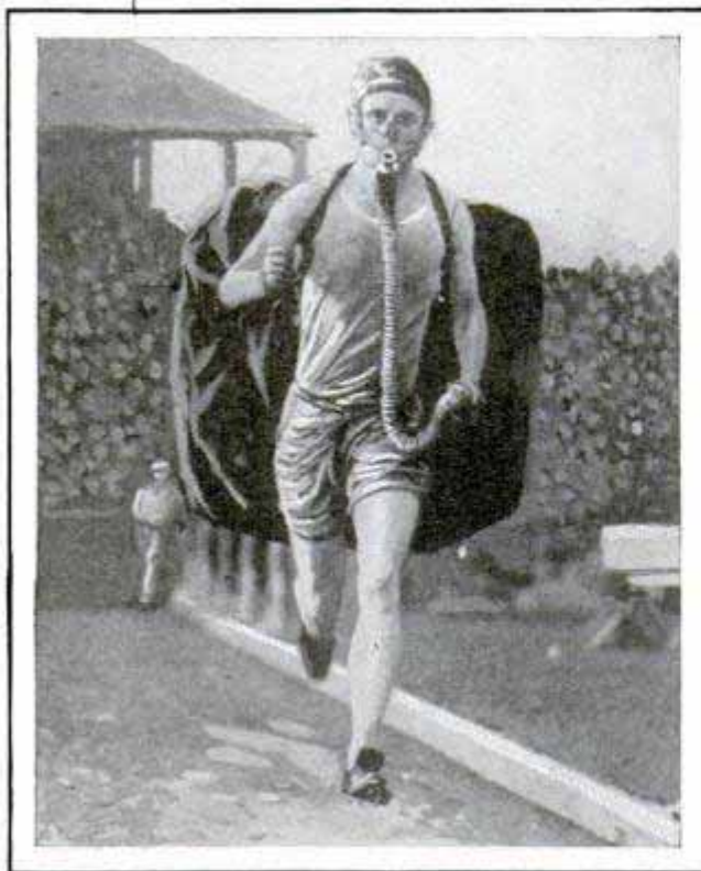
Racer Wearing Mask Which Collects Expired Air So That the Energy Expended Can Be Measured
