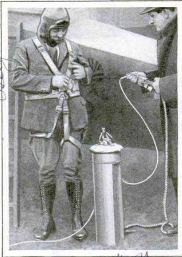
Parachute in Container; It Is Pulled Out When Pilot Leaps over Side, Saving Bother with Release Cord
