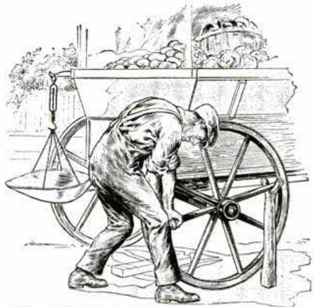
Lifting Wheel of Loaded Wagon by Using a Prop
