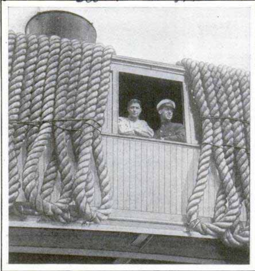
Protection from Chinese Bullets for Ships in Whangpoo River; the Rope Armor Is Draped on Vessel's Bridge
