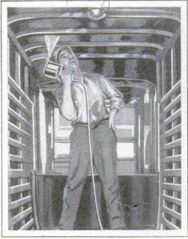
Illustrating How Paint-Spray Gun Is Adapted to Overhead Work and Reaching in Corners
