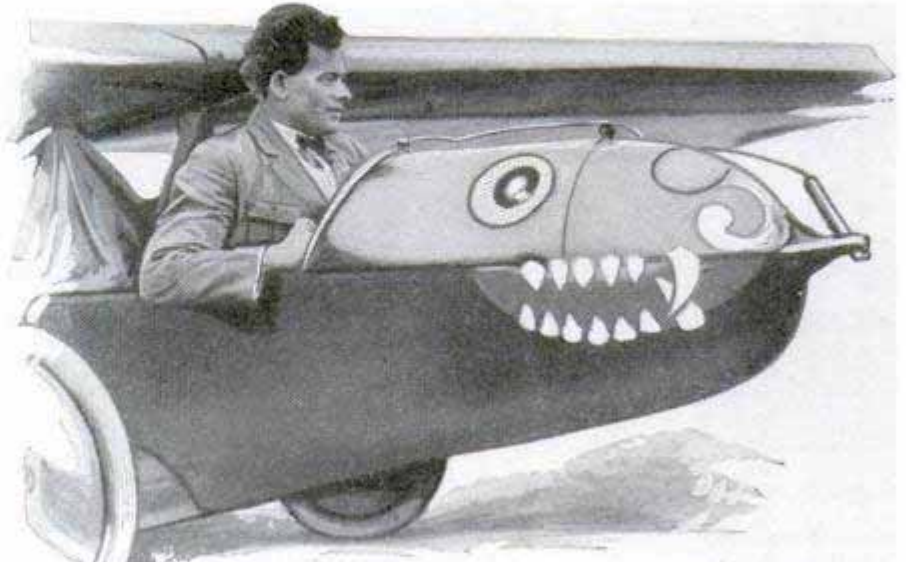
Glider Used as "Car" behind Airplane in Recent German Test; It Was Detached and Made an Independent Landing with Occupant
