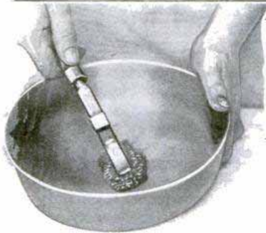
Metal Clamp Holds Dishcloth or a Cork for Scouring and Utilizes Last Bit of Steel Wool, Reducing Waste
