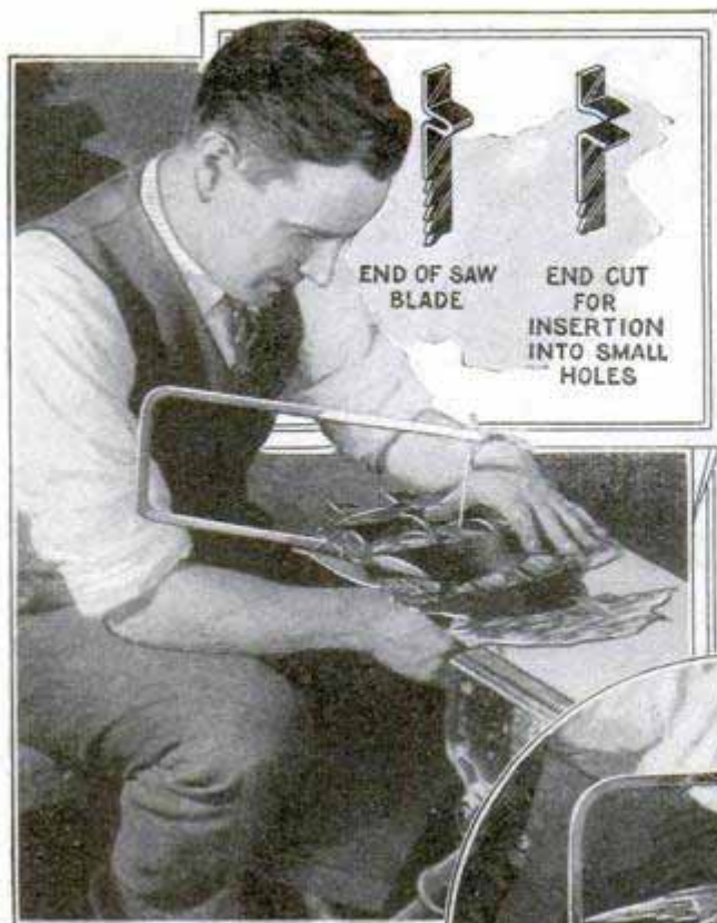
Above, Use of Bracket or Fret-saw in Cutting Out Ship; Below, Coping Saw Used for the Same Purpose
