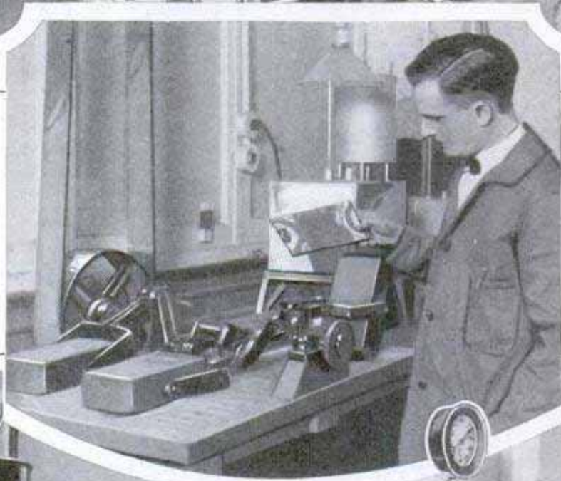
A Chicago Mail-Order Company Maintains a Laboratory to Test Samples of Everything It Sells. Above Is an Expert Testing Sugar, Essential Oils and Extracts, and Below Is a Light Test That Gives Suits and Other Cloth a Year's Exposure in Forty-Five Hours
