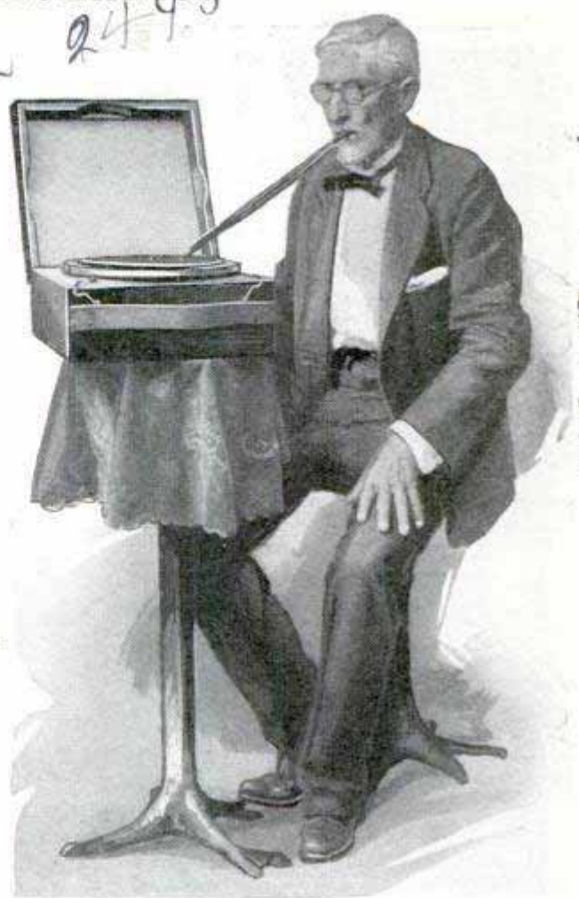
Demonstrating the "Wooden Ear"; Vibrations from Phonograph Record Carried to Teeth through Stick
