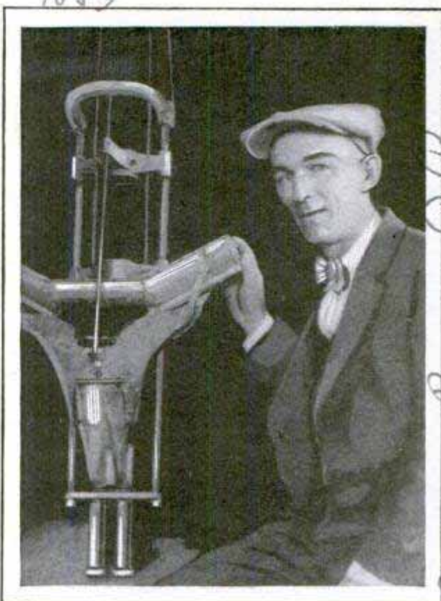
For Faster Work in Building Cars; the Double-Barreled Nail Driver Operated by Compressed Air
