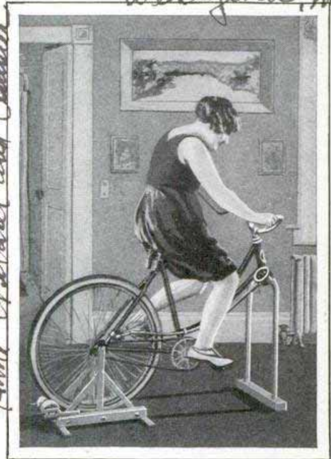
Stationary Bicycle Riding for Exercise and Reducing; a Speedometer under Handlebars Gives the Mileage
