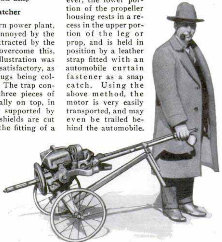
Light Rubber-Tired Cart Facilitates Hauling Outboard Motor Back and Forth, or May Be Attached to Auto as Trailer
