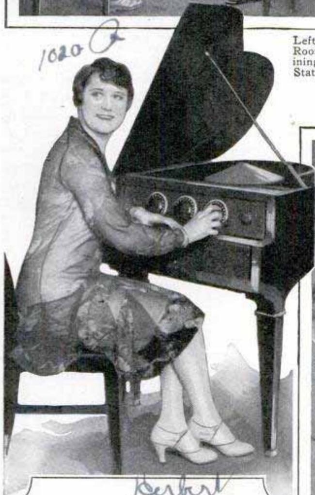
kerbert Above, Built into a Miniature Baby Grand Piano, This Six-Tube Home-made Set, with the Cone Mounted on the Sounding Board at the Rear, Makes an Attractive and Efficient Installation; Right, Recording Interference between Stations, to Obtain Data to Be Used by the New Radio Control Board in Allocating New Wavelengths
