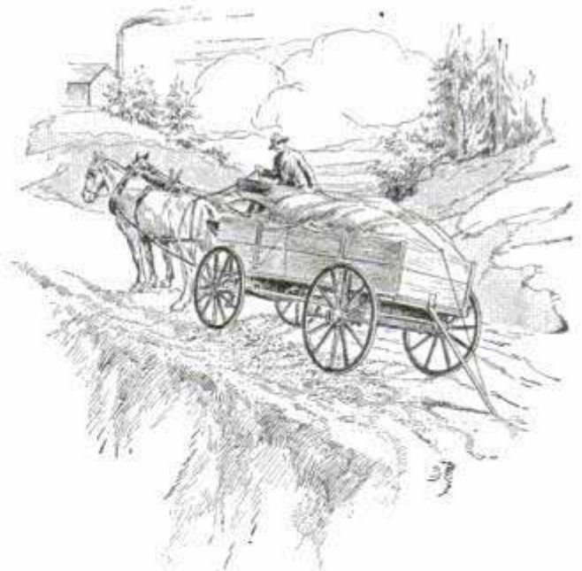
Brake on Wagon Relieves Horses of Heavy Load While Resting on Long Grade
