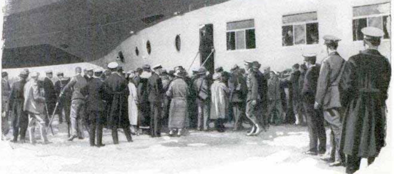
Friends Bidding Goodby to Passengers in the "Los Angeles"; the Round Portholes Are Windows in the Cook's Galley, and the Triple Windows Light the Pullman Staterooms
