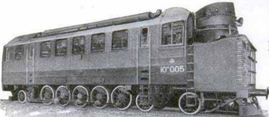
Completed Geared Diesel Engine, Showing the Cooling Radiator at Right, with Exhaust-Fan Duct above It
