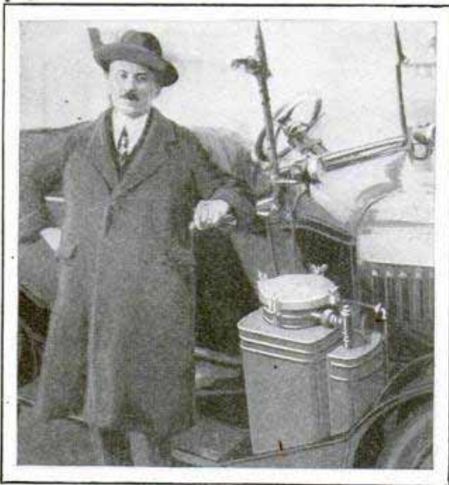
Acetylene-Gas Generator in Automobile; It Is Said to Reduce Expense of Running the Car
