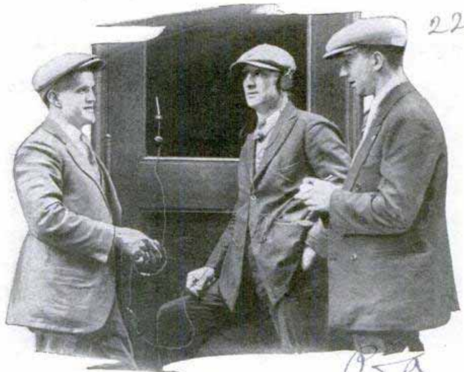
Testing the Sensitive Disk; It Is Attached to the Door and Is Relaying Sounds from the Other Side through Earphones
