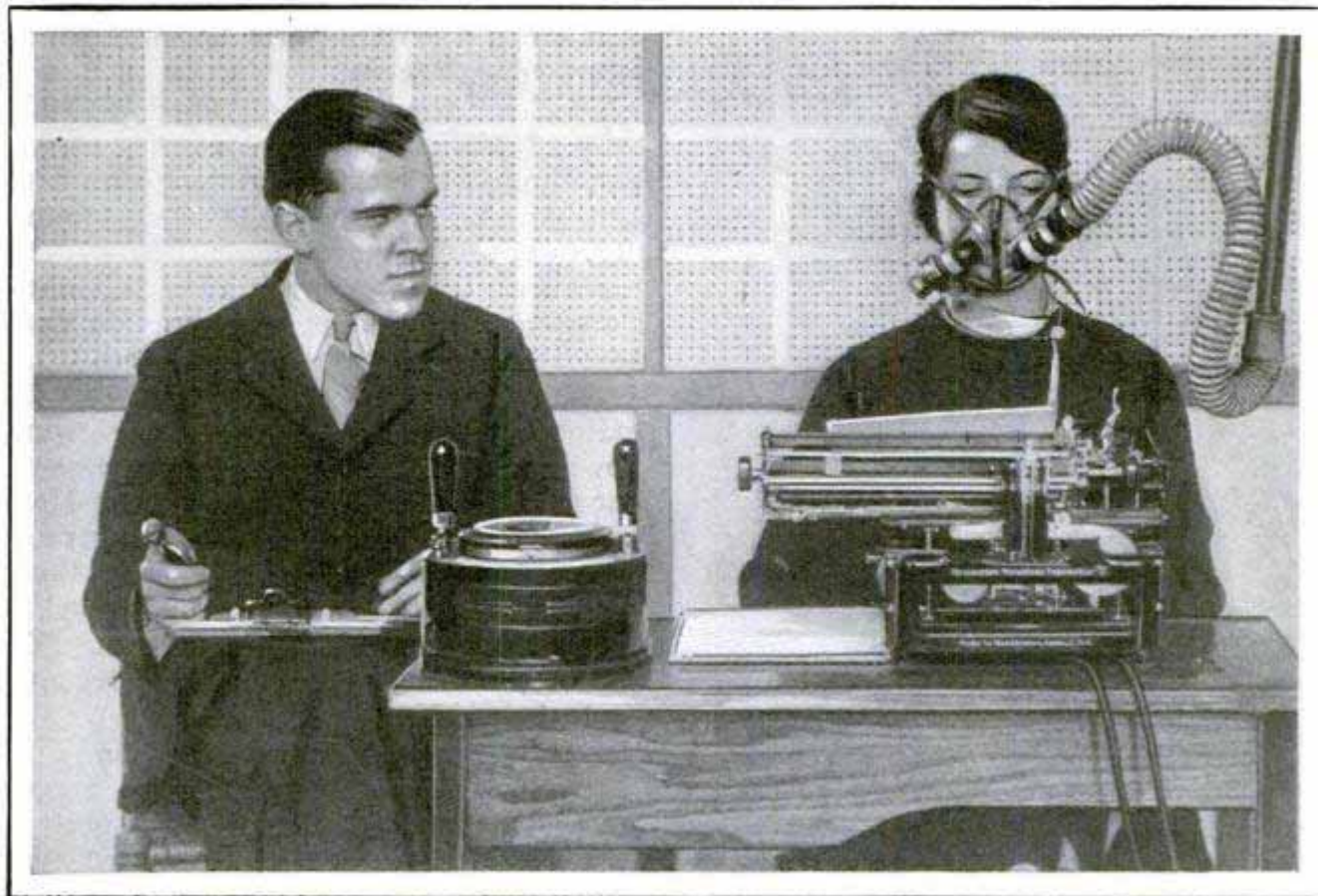
With Gas Mask to Collect the Breath, So That the Energy Consumed Can Be Measured, and an Observer with Stop Watch to Time the Output, the Typist Is Ready for a Noise Test
