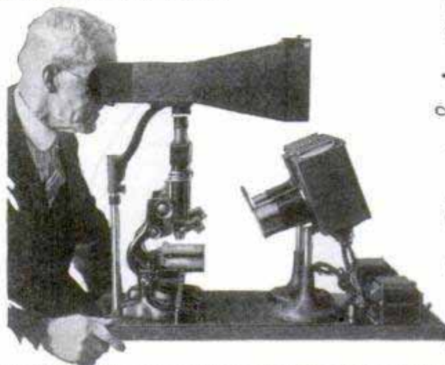
Outfit for Enlarging and Comparing Fingerprints; They Are Projected on a Screen for Close Analysis
