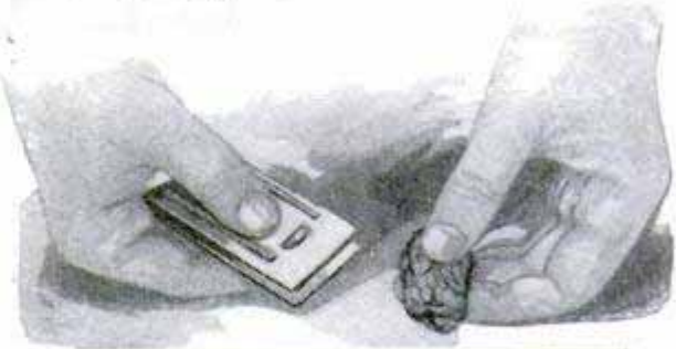
Both Sides of the Knife Are Sharpened at Once between Small Disks Rotated by Crank
