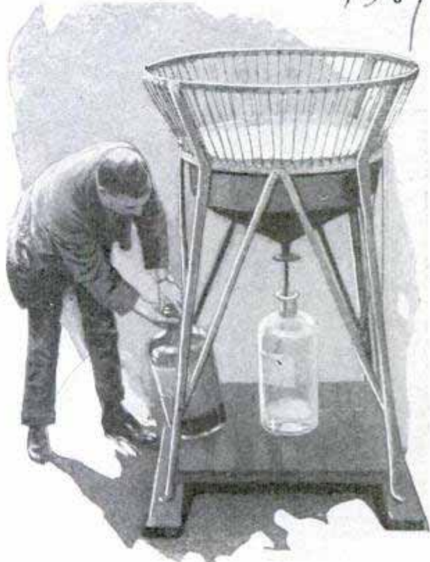
Soot Meter in Operation; Removing Bottle of Dirty Water for Analysis of Contents
