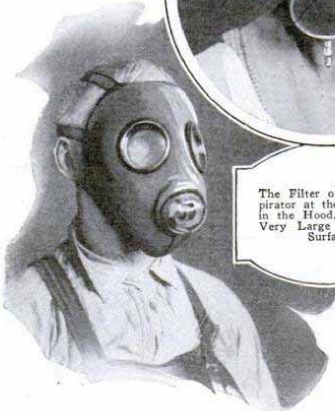
Despite Its Appearance, a Pig Was Not Used as the Model for the Mask Above, Which Uses Several Thicknesses of Woolen Felt to Protect the Wearer from Breathing Dangerous Dust While at Work
