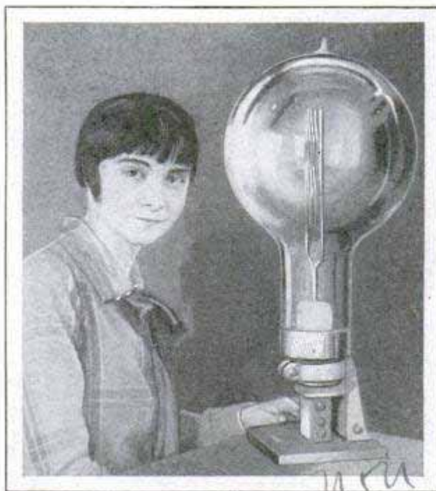
Bulb for Ten-Kilowatt Floodlight Used in Guiding the Air-Mail Pilots at Night
