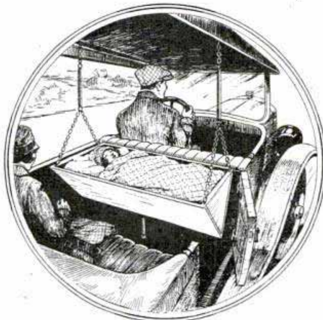
Simple Baby Carrier Hung behind Front Seat Is Safe and Comfortable
