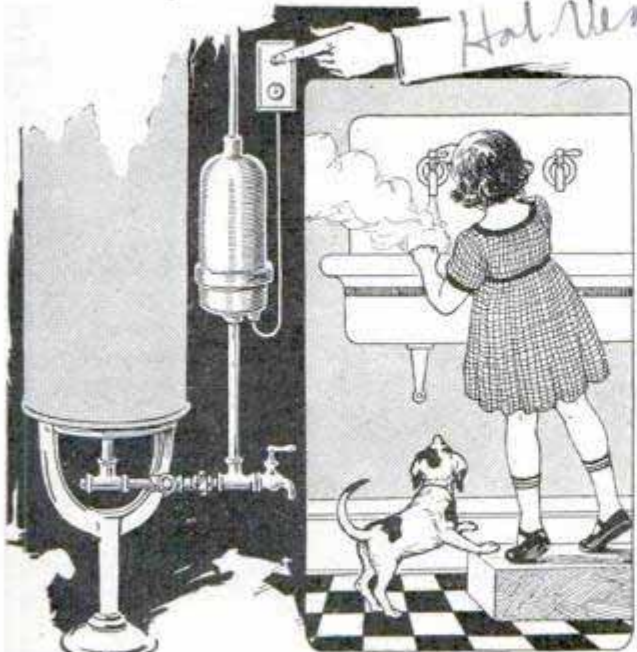
Electric Heater, Installed with Water-Supply Tank, and the Current Control Panel
