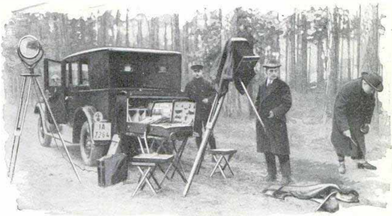
German Police Squad with Traveling Laboratory at the Scene of a Crime; besides the Camera, the Outfit Includes Chemicals for Making Analyses, Microscopes and Other Equipment
