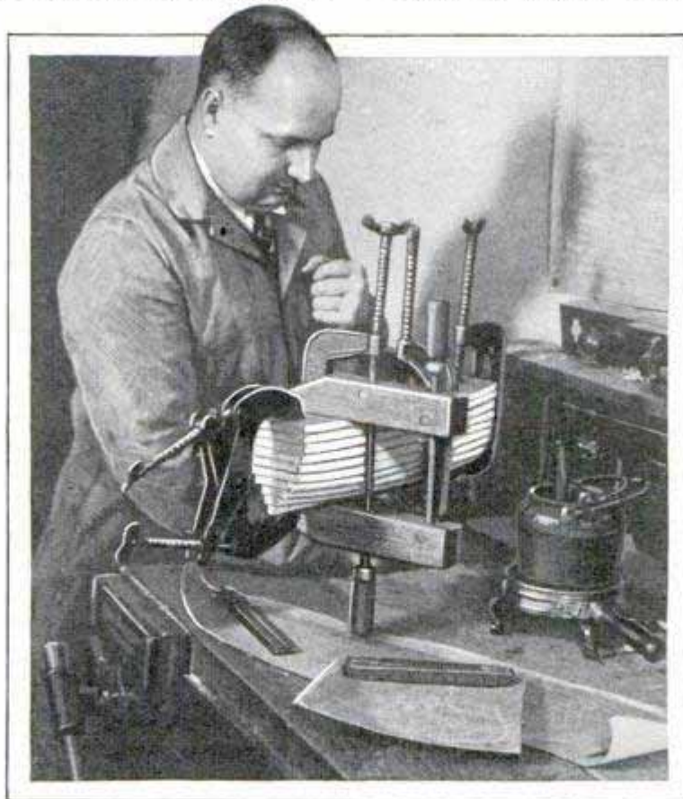
If the Model Maker Glues Up His Own Hulls, Several Large Clamps Are Essential
