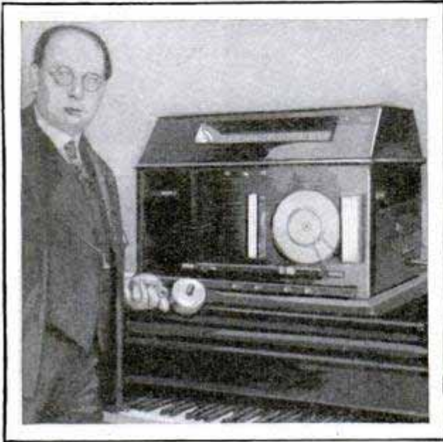
Giving the Orchestra Conductor Control of the Motion-Picture Film's Speed; the New Regulator Box
