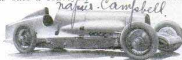
New Twelve-Cylinder Racing Car, Showing the Streamlined Side Bulges on the Hood
