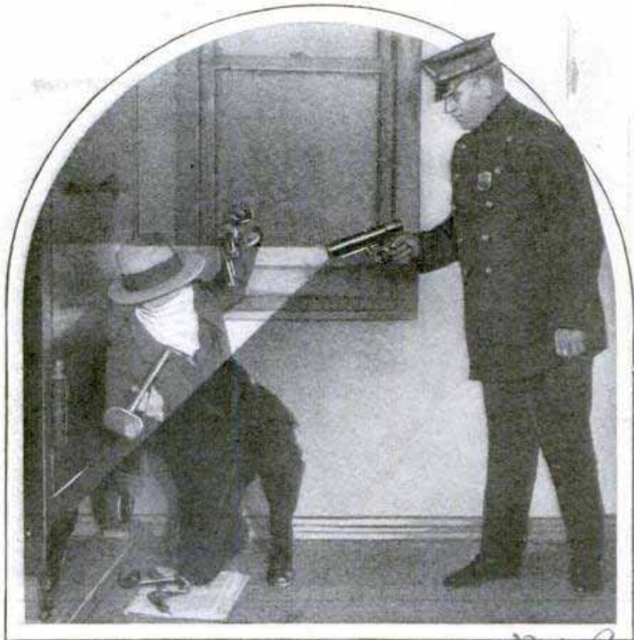
Double-Purpose Weapon for Police, the Combination Flashlight and Revolver, to Surprise Criminals and Aid in Firing
