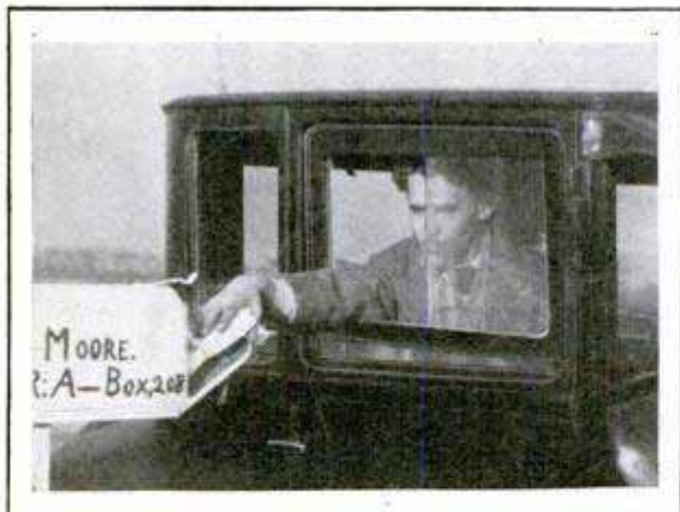
Mail Carriers Find the Sliding Panel Easier to Open than the Glass of the Auto Door
