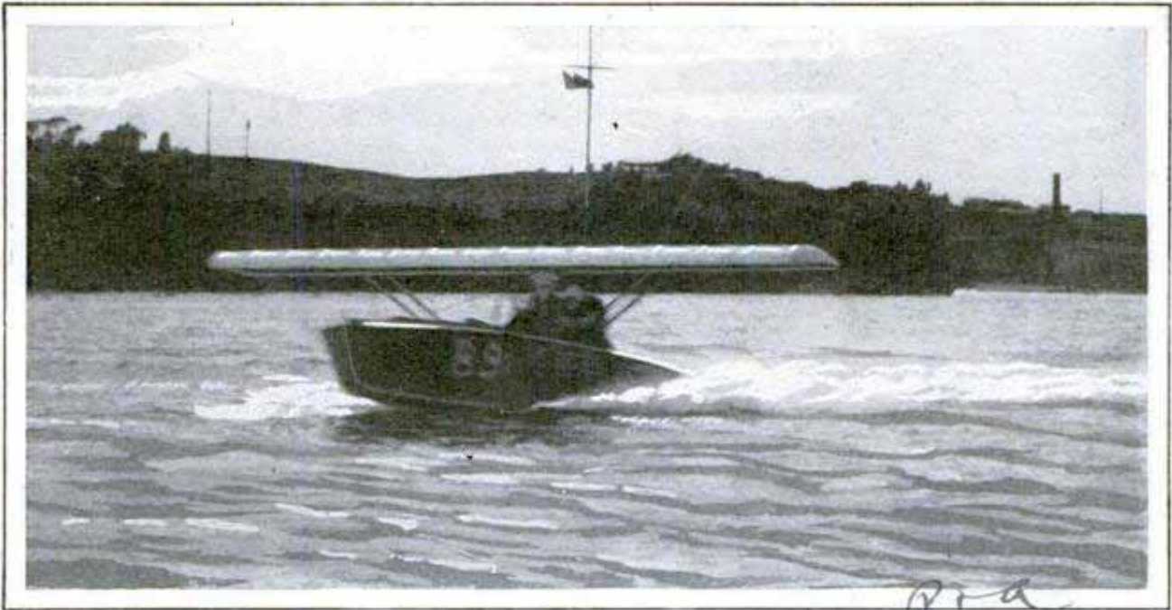
"Miss Spitfire V," with Airplane Wing Attached, Made Fifty-Eight Miles an Hour in a Recent Test; the Boat, without This Aid, Previously Sped at More than Forty-Seven Miles an Hour
