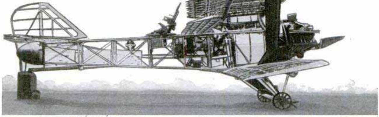
Courtesy The Sphere 11/13/26 Skeleton of Huge Fighting Plane Shows Rigid Bracing of Wings, Position of Fuel Tanks, Cockpit and Other Features; Exhibited at Madrid Exposition
