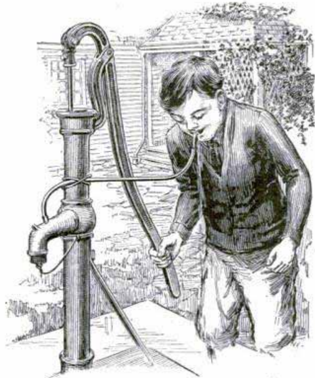
Ordinary Farm Pump Converted into a Sanitary Drinking Fountain
