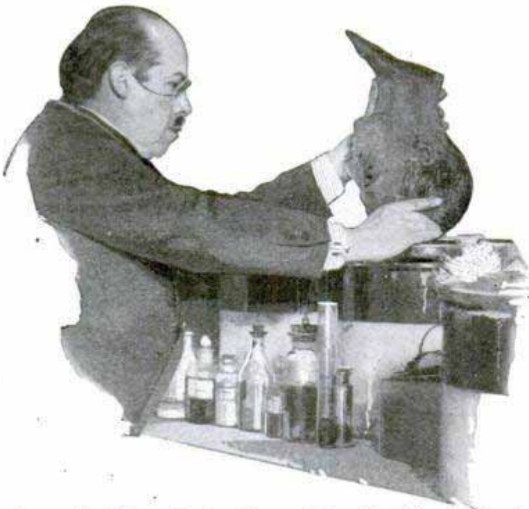
Bronze Head from Ancient Greece Being Placed in the Vat for Electrolytic Treatment to Restore the Original Metal
