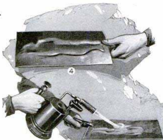
This Work Can Be Done at Home with a Ball-Peen Hammer, Woodworkers' Clamp, Vise and a Number of Nail Punches Ground to Suit the Work
