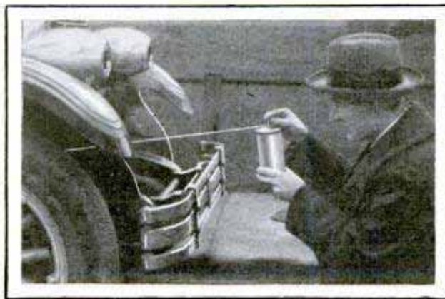
White Line Indicates a Stream of Oil Being Shot at Auto Spring
