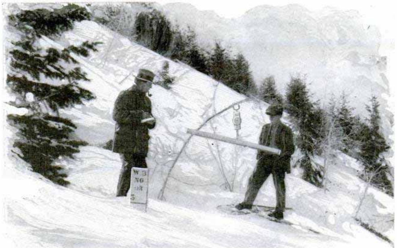
Forest Rangers Weighing a Sample from the Five-Foot Snowfall in Holy Cross National Forest, Colorado, in Order to Determine Its Density and Water Content
