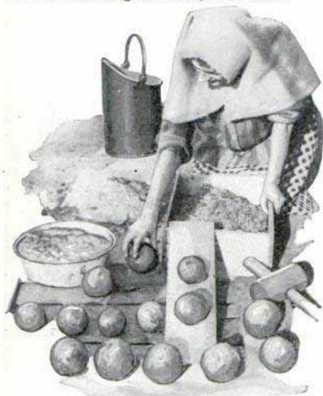
Molding the Coal-Dust Balls; They Are Coated with Sawdust to Prevent Stickiness.
