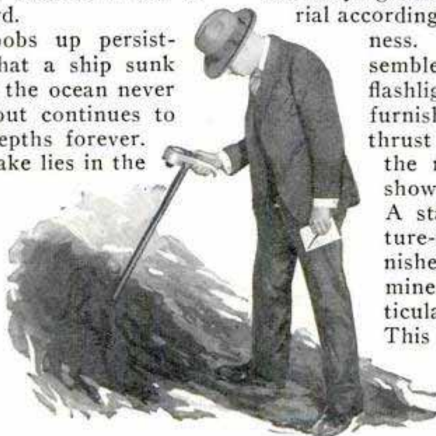
Moisture Meter in Use; End of Stick Is Stuck in Sand Pile and Reading Taken from Handle
