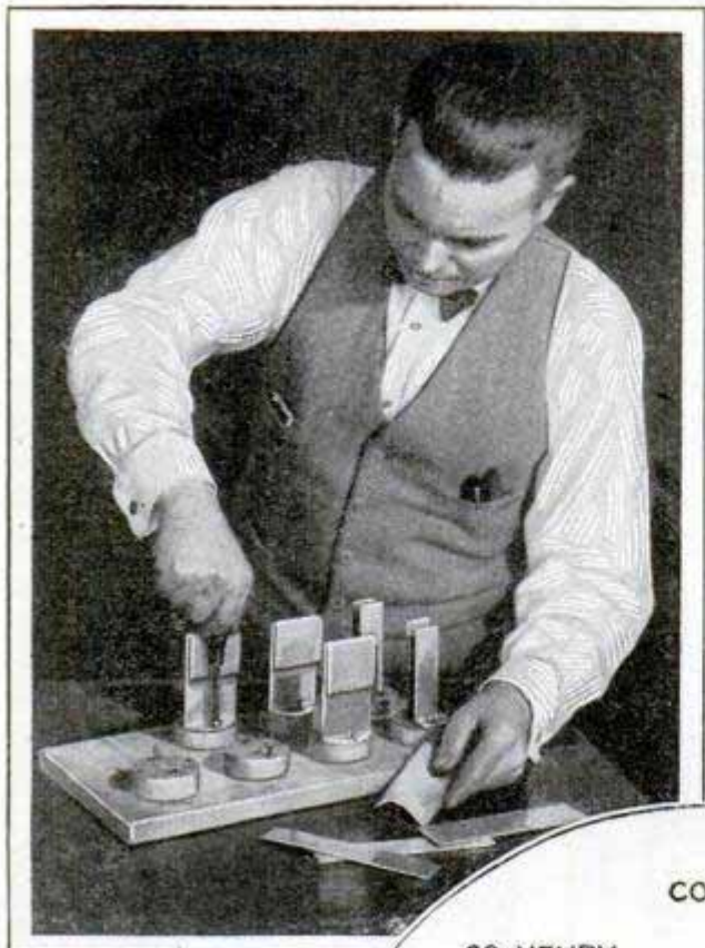
Above, Mounting Aluminum Condenser Plates; Center, Schematic Diagram of Circuit; Below, Pointing Out Taped or Insulated Portions of the Electrodes
