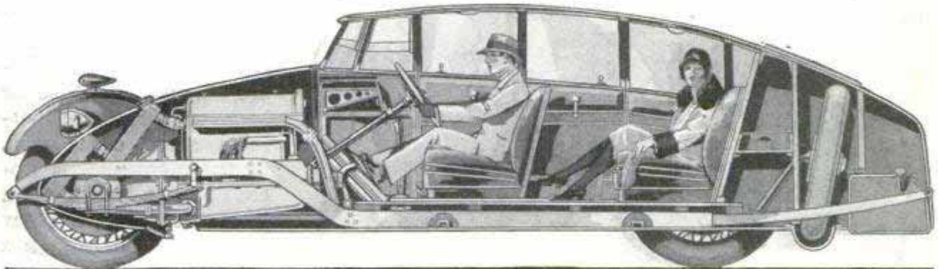
An English Idea for a Streamlined Body on a Front-Wheel-Drive Car; Notice How the Elimination of the Rear Axle Helps Bring the Body Down for a Low Center of Gravity
