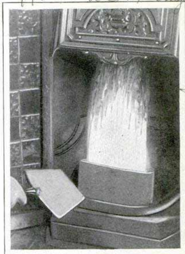
Kerosene Fire in Grate; the Box Is Filled with Absorbent Wool and Is Easily Removed
