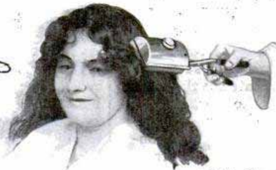
Hair Wayer, Showing the Chamber for Hot Water at the Top; Long Applications Are Possible
