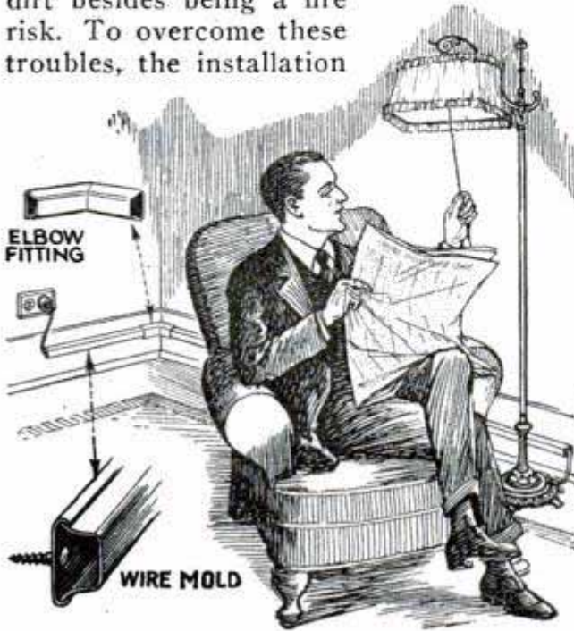
Lampcord Protected from Injury by Installing It in Metal Molding Screwed to Baseboard
