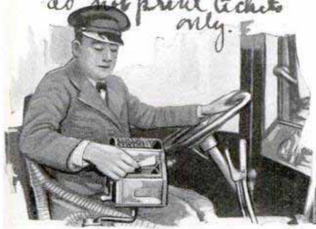
Issuing a Ticket from Register; Machine Keeps a Record of the Fare for Future Auditing
