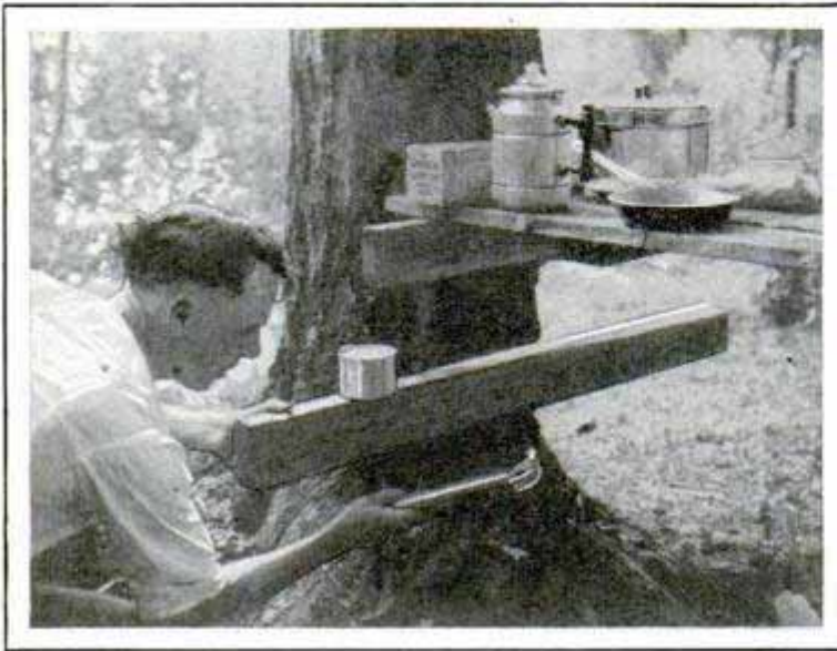
Tin Cup Filled with Water Makes a Serviceable Level for Campers in Making Furniture and for Other Purposes
