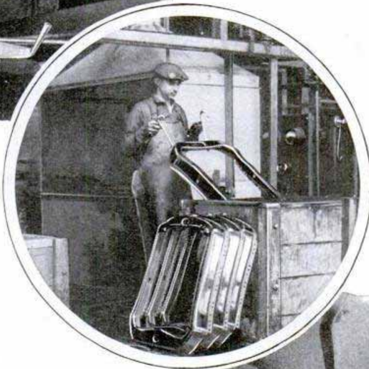
Courtesy Iron Age Golf Clubs and Metal Shafts Can Be Plated Either in a Bright or Satin Finish; Center Picture Shows Auto Radiators Being Plated; at Right, Scratching a Glass Plate with Pure Chromium
