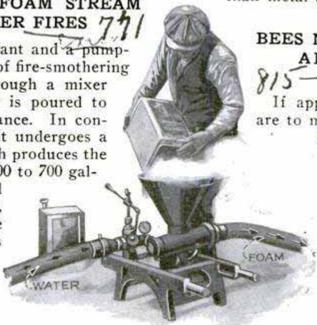
Pouring Foam Powder into the Mixer; the Smothering Stream Is Forced through Hose at Right
