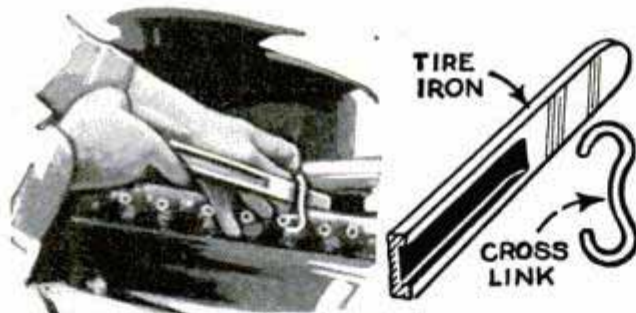
Tire Iron and Cross Link Facilitate Lifting Valve-Rocker Arms
