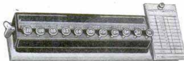
Tabulator to Simplify Making Up Payrolls; Pressing Keys Registers Number of Coins Needed
