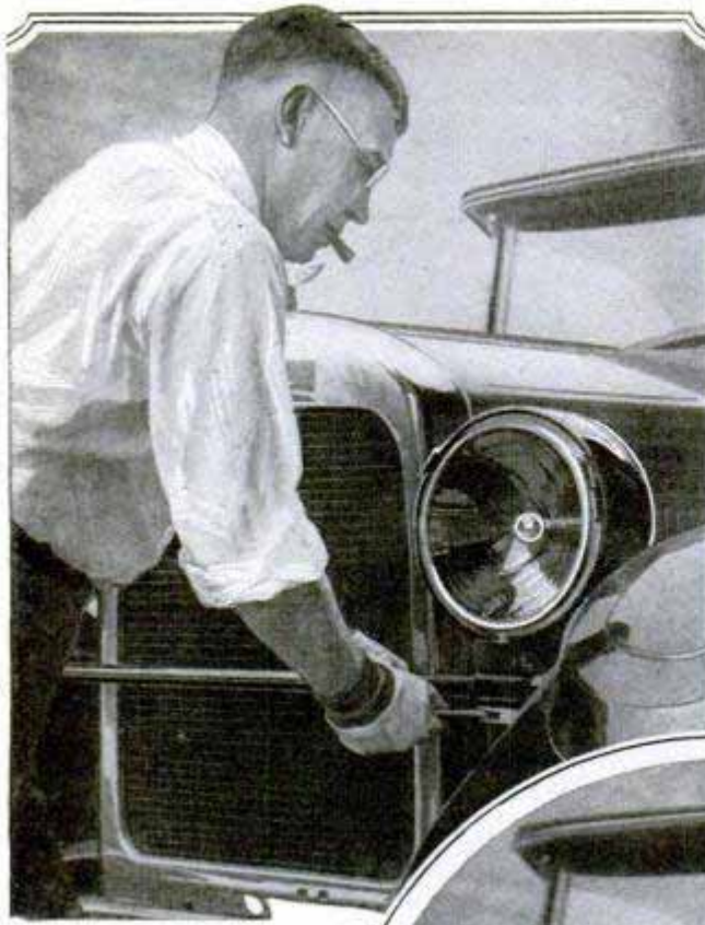
Top, Loosening the Lamp Adjustment; Center, Aiming Lamp; Below, Measuring Height of Lamp Center
