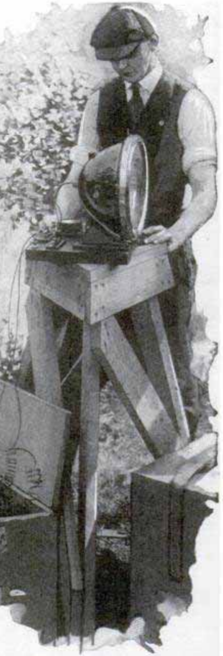
Fixing Your Location on the Map; Geodetic Engineers with Sun Reflectors and Telescopes; in the Center Is an Observation Tower, and at the Right, the Auto Light for Night Work
