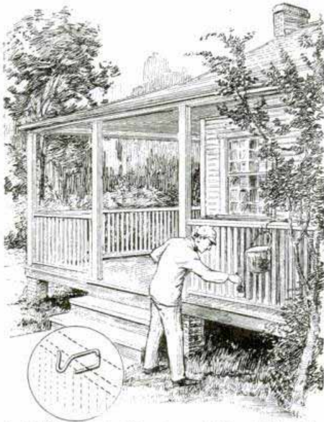
Small Wire Hook, Slipped over Railing, Holds Paint Pot in Handy Position
