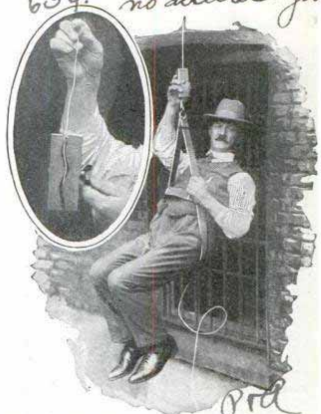
Descending the Wire Fire Escape; Inset Shows the Grooved Block and Speed Regulator
