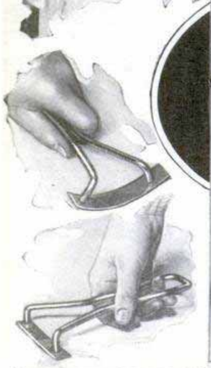
Two Scrapers in One: Squeezing Handles Bends Blade for Curved Surfaces
