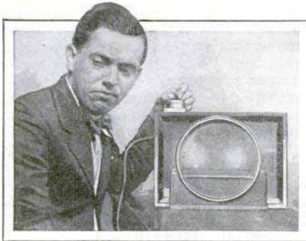
Illustrating the Fine Texture of Screen Used in Sifting Cement Materials; Sieve Holds Water
