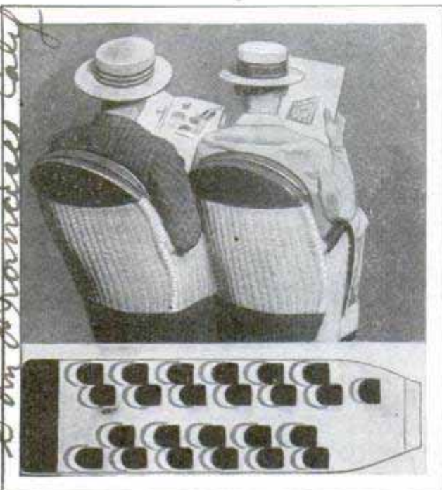
How the Staggered Seats Afford More Room for Passengers and Diagram of Bus Interior
