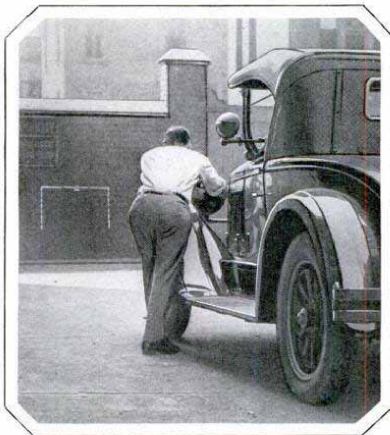
Adjusting the Lamps Sidewise So as to Center the Spots on the Marks Made on the Wall
