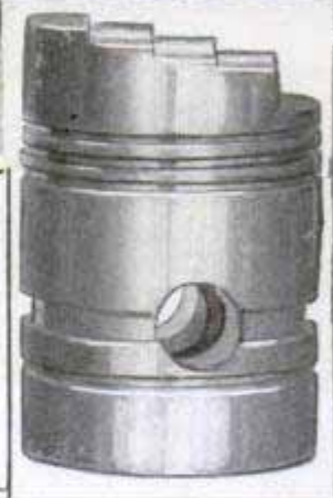
For Taking a Sun Bath or Sight-Seeing, the Convertible Touring Car, Above, with Its Transparent Top, Is Ideal; at the Right Is a Step-Top Piston, Designed to Eliminate Detonation at High Pressures
