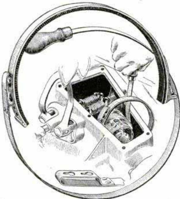
Handy Tool Made from Spring Steel Is Helpful in Inserting Transmission Bands
