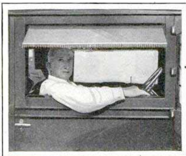
Automobile Awning in Place, Showing How It Provides Shade from the Sun for the Passengers
