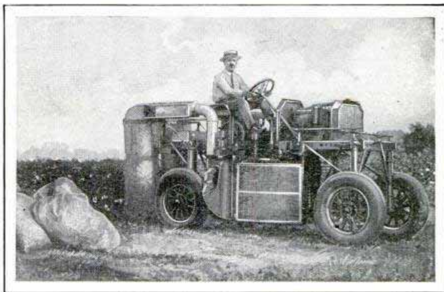
Picking Cotton by Auto; the Machine Straddles the Row and Is Said Not to Injure Plants or Unopened Bolls
