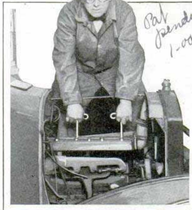
Lifting a Cylinder Head with Two Handles Which Screw into Any-Size Spark-Plug Opening
