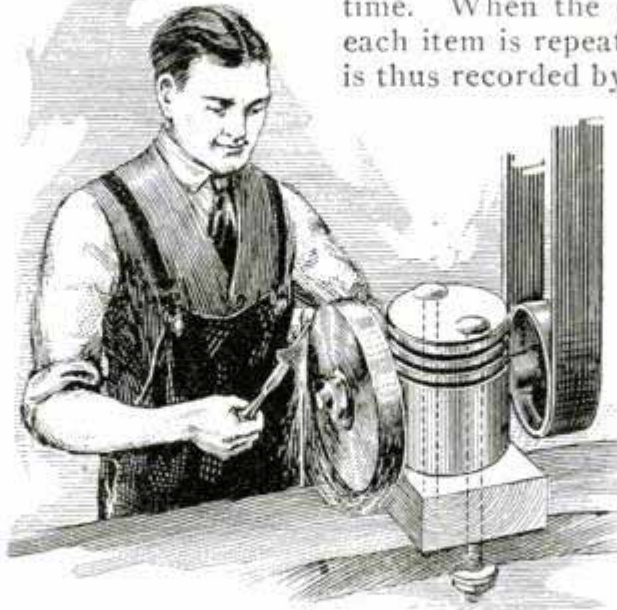
Serviceable Bench Stand for Emery Wheel Is Made from Old Piston
