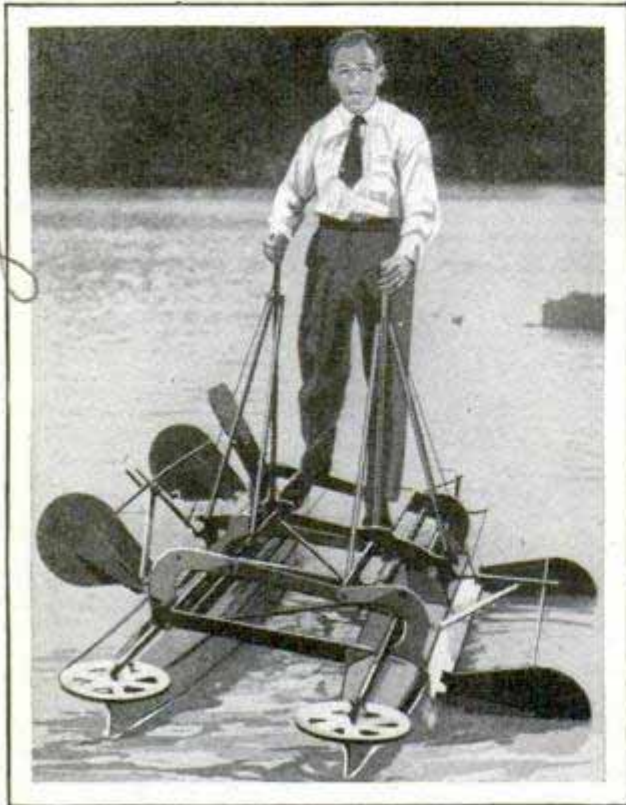
Operating the Paddle Foot Boats; Blades Are Moved Back and Forth by Levers
