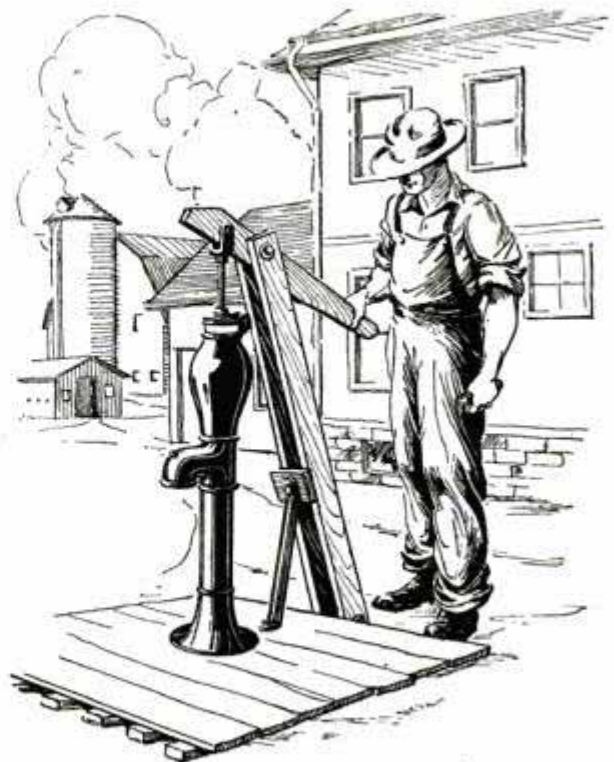
Wooden Pump Handle and Bracket Found Satisfactory in Emergency
