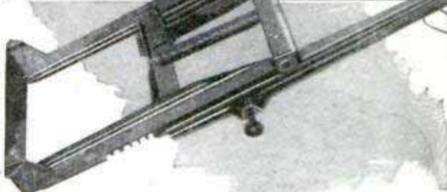
Seat Pulled Forward to Aid Passenger in Alighting, and Close View of the Sliding Rack
