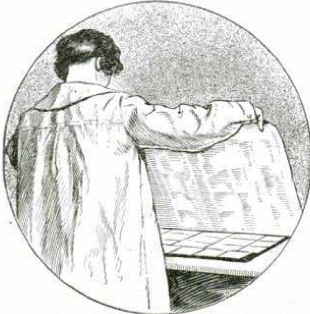
Large Piece of Oilcloth Absorbs Surplus Moisture from Ferrotyped Prints
