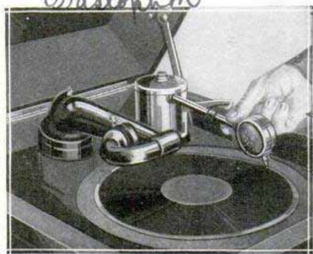
Electric Arm Adjusted to Ordinary Phonograph; Tones May Be Modulated and Installation Is Simple
