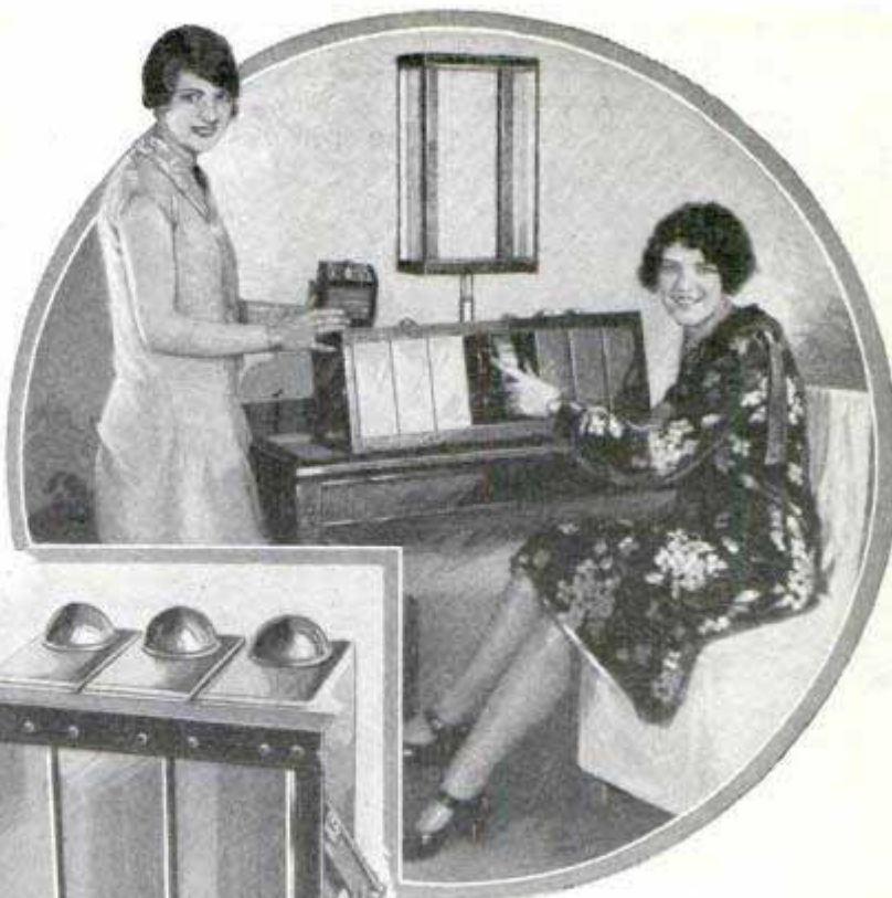
Left, Eight-Tube Neutrodyne, Showing Method of Shielding; Above, Comparison in Size and Type of Early Crystal Set with the Single-Control Receiver
