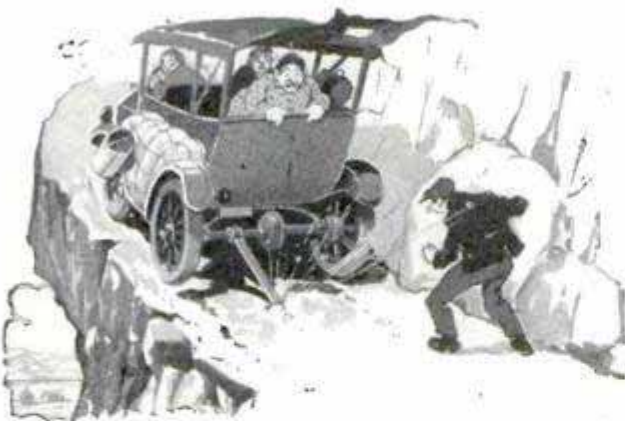
A Hinged Sprag Drags on the Road, But Digs In When the Car Stops and Holds It
