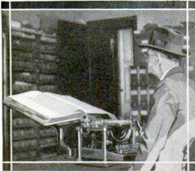
Adjusted on Holder near Typewriter, Big Book Is Easily Copied and Protected from Damage
