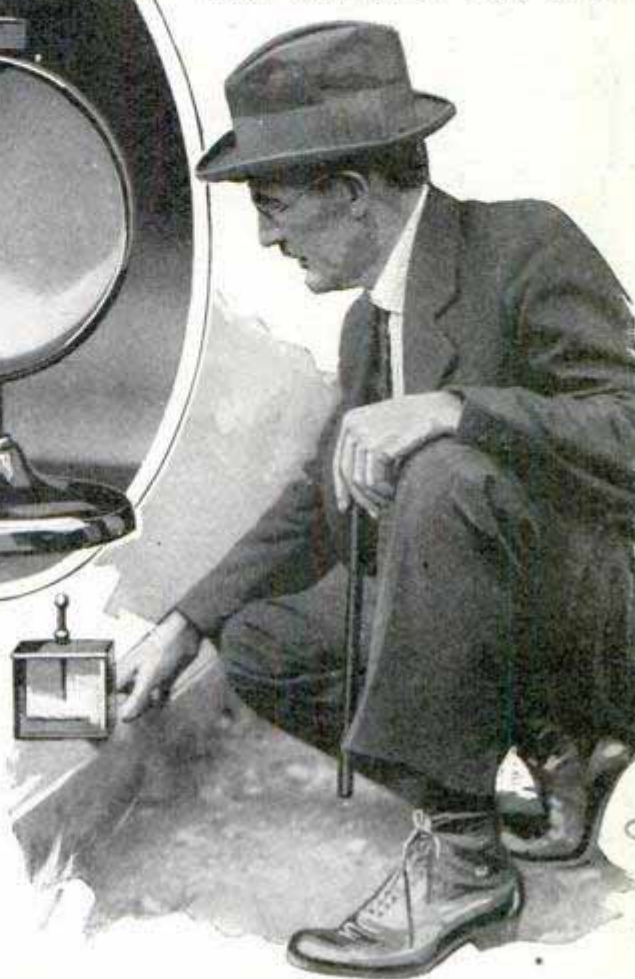
Electroscope in Use While Hunting for Lost Radium, and Closer View of Another Type
