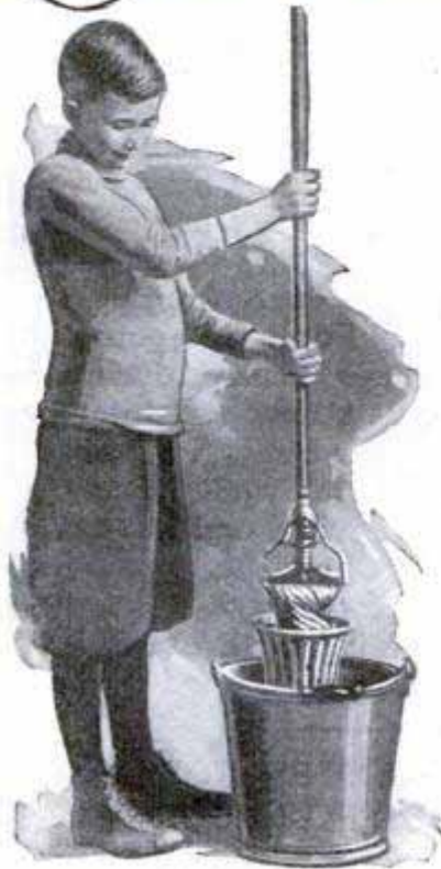
Wringing the Mop by Twirling It; End Fits into Corrugated Double Cone in Pail
