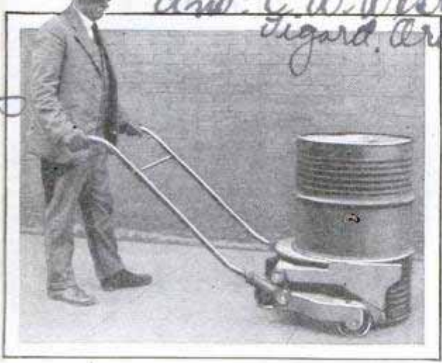
Truck for Hauling Drums of Oil or Other Liquids without Spilling; Movable Flanges Grip the Sides
