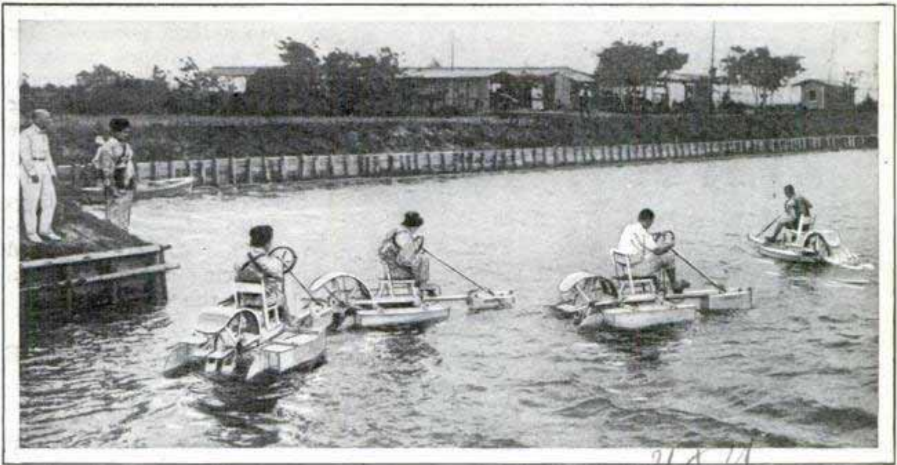
Japanese Men and Women in Race with Odd Paddle Cars; Steering Wheel Swings Rudder in Front for Guiding, and Power Is Applied to Rear Wheel through Pedals
