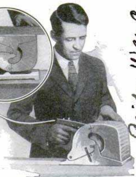
Novel Sander Operated Either by Hand, or Reversed, in Special Mount, to Become Table Type
