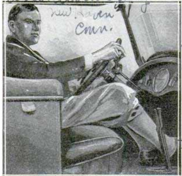
Gears Are Shifted by a Valve on the Steering Column of This Automobile
