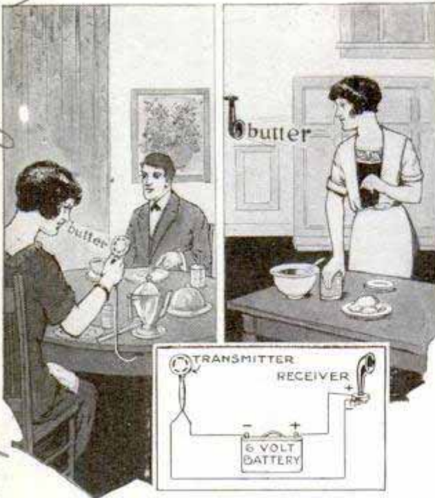
Drawing, Showing Housewife Using Microphone Installation to Call Maid, and Diagram of Circuit
