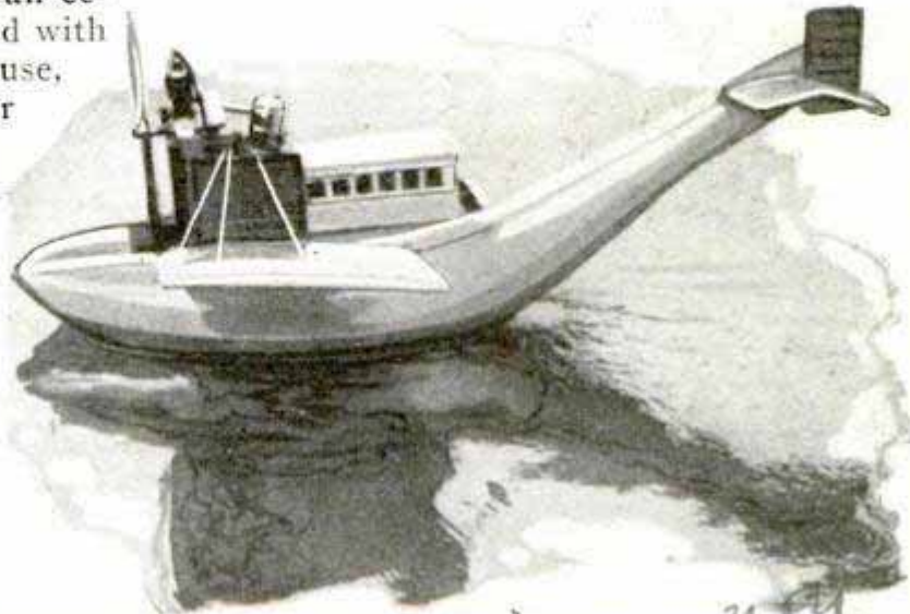
Elevating the Tail of This New Japanese Seaplane Insures the Rudder against Damage When Landing in the Water
