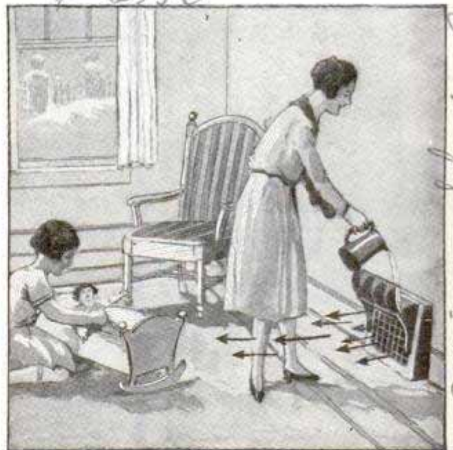
Water Chamber Built to Fit over Hot-Air Register to Maintain the Correct Humidity
