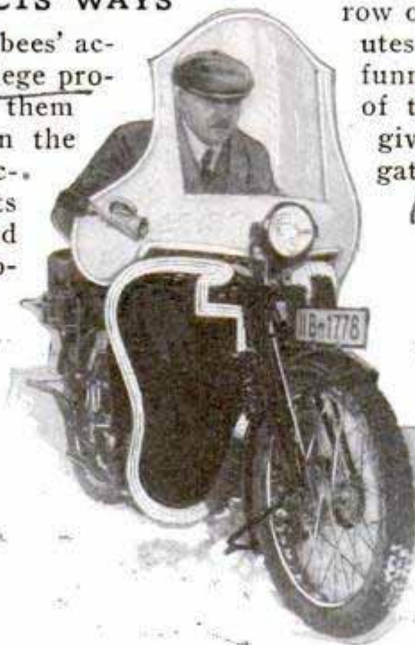
Motorcycle Shield Adjusted, Showing How It Protects Legs as Well as Face and Shoulders
