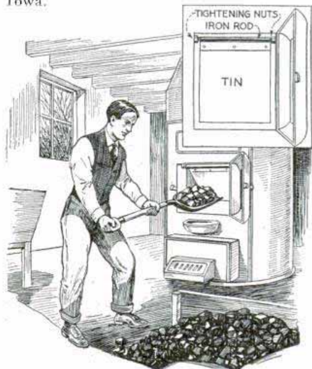
Heavy Sheet-Iron Swinging Door in Furnace Found Convenient
