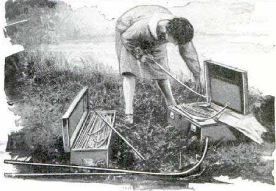
Packing the Folding Boat and Demonstrating Its Light Weight; a Canvas Covering Is Stretched over the Ribs
