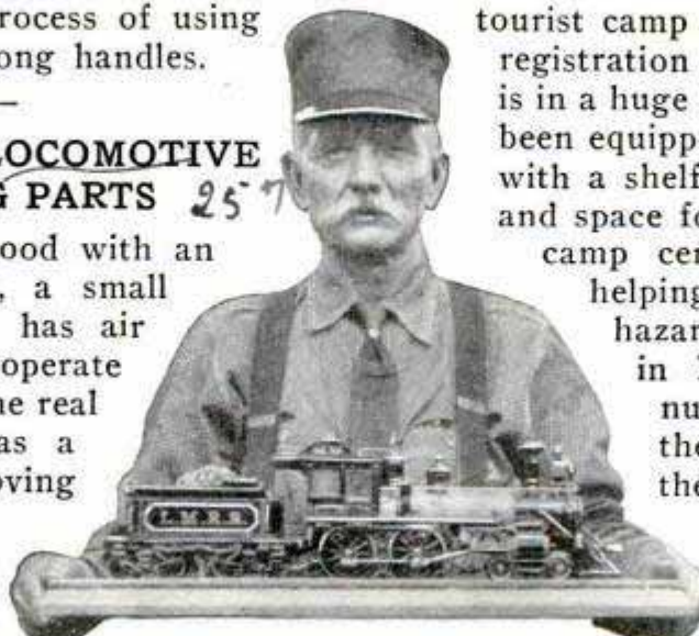
Whittled from Wood with Pocketknife, This Model Engine Has Metal Air Brakes That Work
