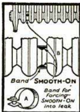
Leak at radiator joint stopped with Smooth-On
