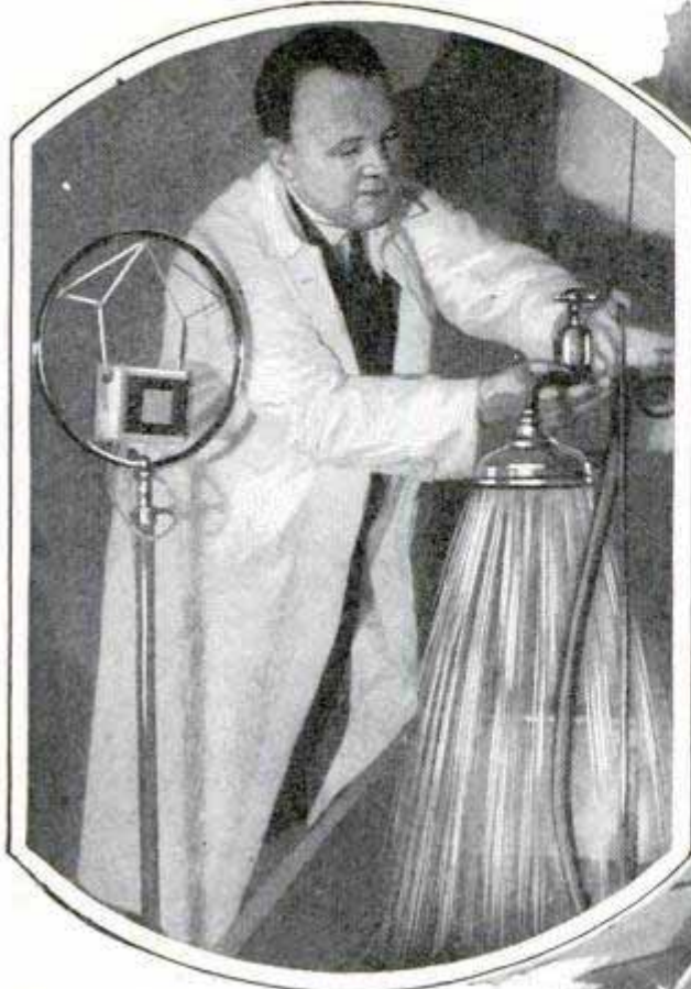
Above, Flowing-Water Arrangement for Imitating Rain, Falling Water and Dashing Waves; Right, Motor-Driven Device for Imitating the Noise of a Ship Propeller; Insert, Wind Machine Consisting of Cloth Stretched over a Wooden Drum; When Rotated, the Spokes on the Drum Brush against the Cloth Producing the Effect of Soft Breezes or High Winds
