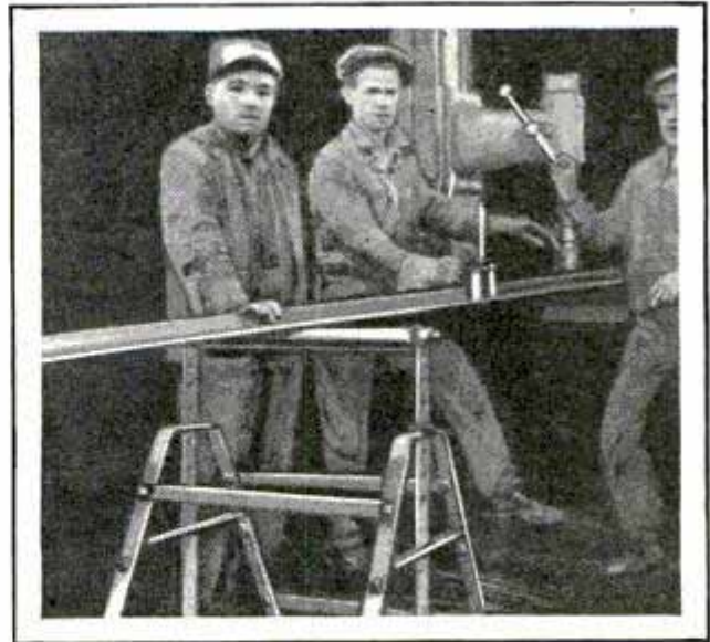
Adjustable Stand near Drill Press for Holding Long Work Reduces Labor
