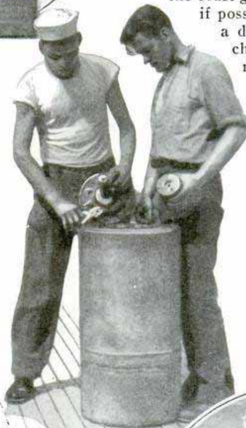
Preparing to Mine a Derelict; the Detonator, Top, Is Being Inserted in a 1,500-Pound Mine in the Center; Below Is the Cable and a Small Mine
