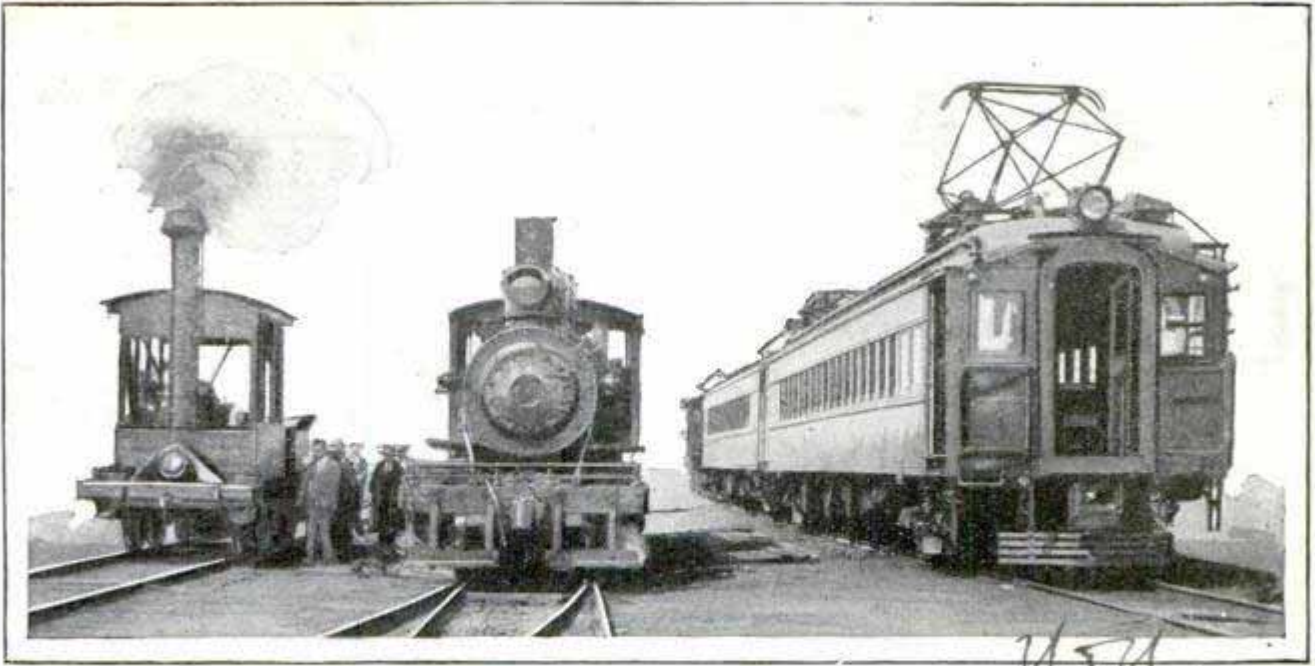
Three Scenes from Railway History Emphasizing the Changes of Less Than Fifty Years; Pioneer Wood-Burning Locomotive at Left, Coal-Fired Unit in Center and, at Right, Electric Train
