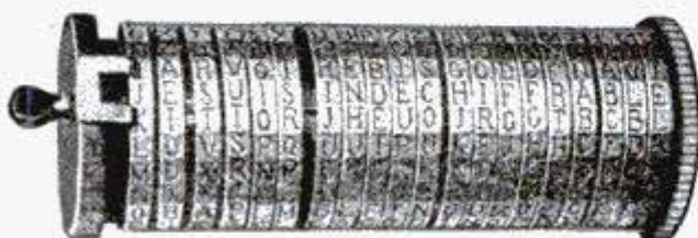
By Rotating the Different-Lettered Disks in This Device, Cipher Combinations Are Produced
