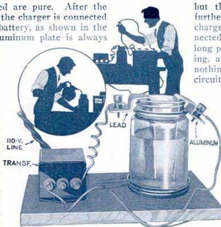
How Cell Is Connected across the Transformer for the Cell-Forming Process
