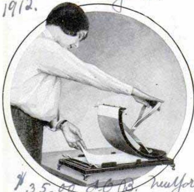
Duplicator in Service; It Is Rocked Back and Forth like a Desk Blotter
