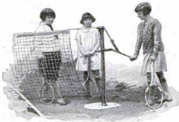
Pressing the Lever Raises the Tennis Net to the Correct Height and Keeps It There
