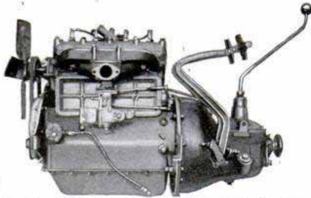
American Light-Car Engine of Only 131 Inches' Displacement, Which Gives Speeds of over Sixty Miles
