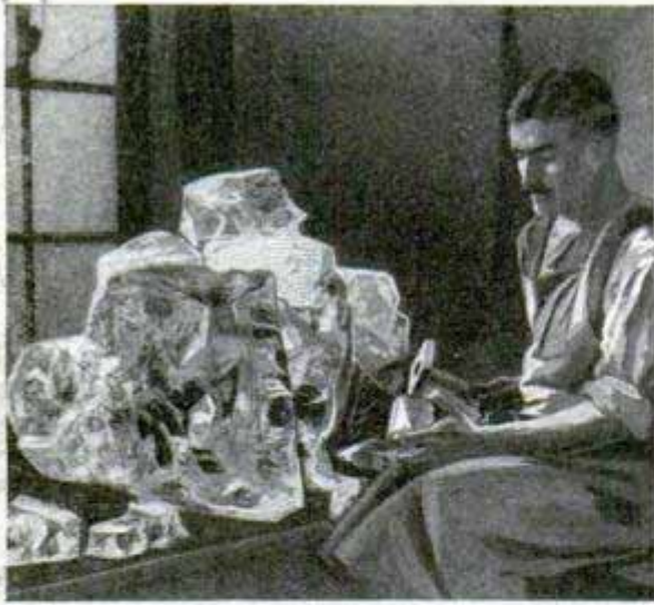
Fine Lenses in the Rough; Glass Nuggets Being Broken Up into Pieces Suited for Grinding
