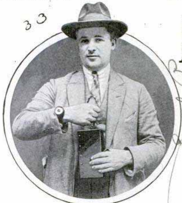
Battery and Shocker Exposed on Wearer's Wrist; It Is Intended to Stun an Assailant with Electric Charge
