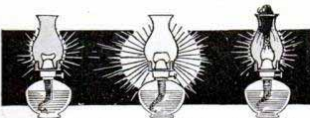
Illustrating Combustion in Cylinders, from Left to Right, Too Lean, Correct Mixture and Too Rich
