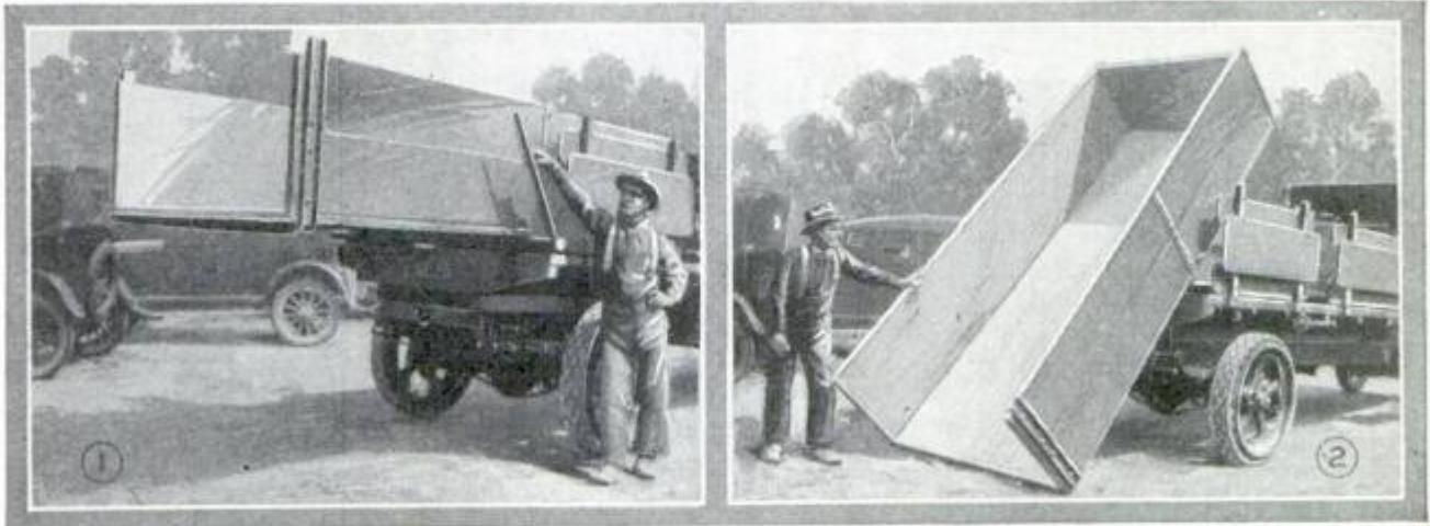
Special Body Built by a Wrecking Company for Hauling Brick; It Can Instantly Be Removed or Attached to Truck by One Man
