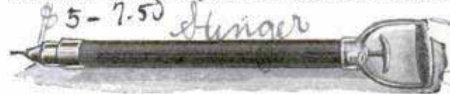
To Kill Weeds; the Poison "Needle" Injects Chemicals into Roots of Troublesome Plants
