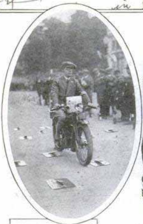
Tests of Steady Driving; in a German Contest, a Motorcycle Rider Guided His Machine between Traps That Fired Shots, if They Were Struck, and, at Upper Right, an Autoist Trying to Halt His Car Exactly at the Barrier Connected to a Horn Which Sounded if Board Was Pushed beyond the Mark
