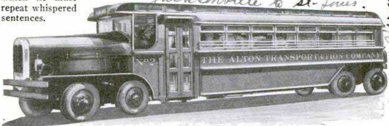
Railroad's Answer to Motor-Bus Competition; Huge Thirty-Five-Passenger Coach with Eight Wheels and Air Brakes Operated on Regular Schedules to Supplement Train Service
