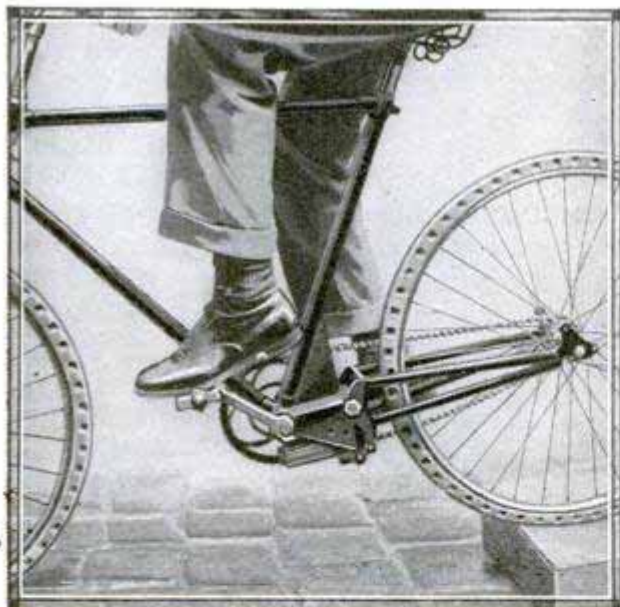
Spring in Socket Joint Keeps Bicycle Frame on Line While Going over Obstructions
