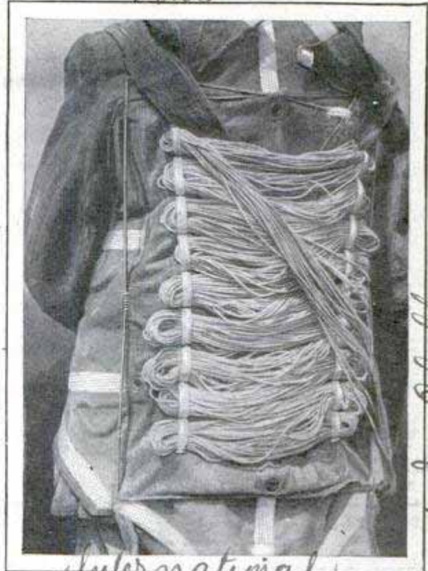
Rear View Showing Folded Cords of Parachute, Which Is Worn as a Coat
