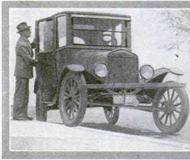
Put One Wheel on the Curb and Try Doors to See If They Bind; Also Inspect the Spark Plugs for the Uneven Formation of Carbon
