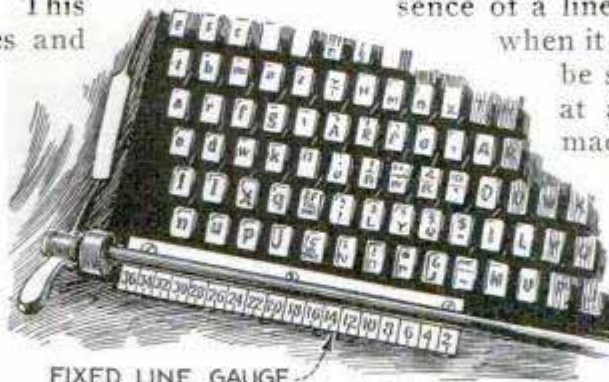
Line Gauge for the Linotype Operator Is Handier When Fixed on Keyboard
