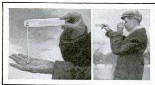
Using the Plumb-Line Attachment and Measuring Range of Distant Object with Gauge
