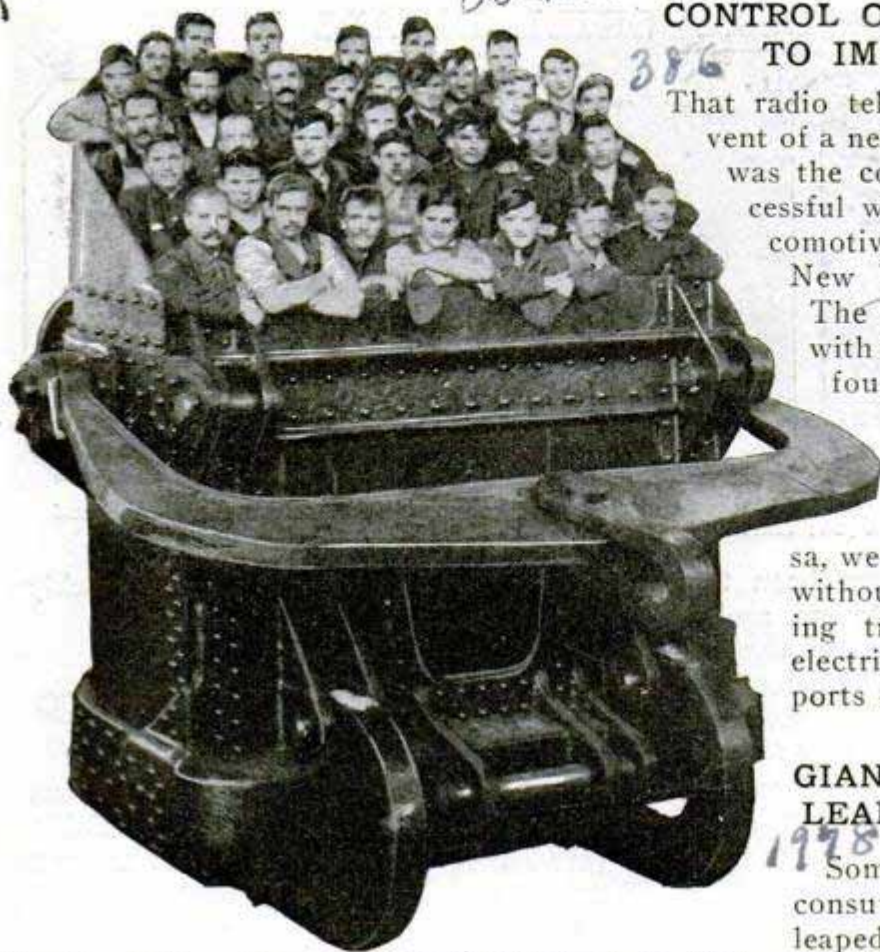
Capacity of Huge Steam-Shovel Bucket Illustrated by Men; Thirty-Four Stand Comfortably in It at Once
