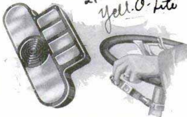
Light Signal and Switches Attached to the Steering Wheel within Easy Reach
