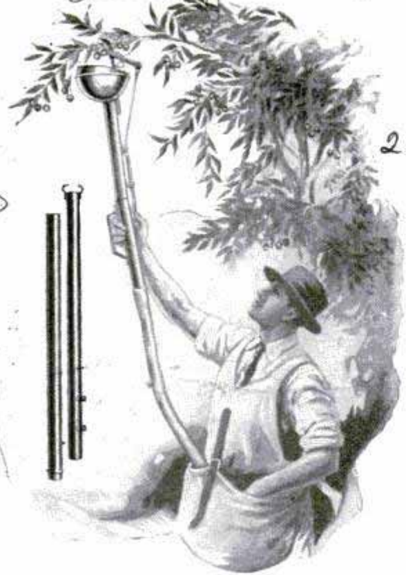
As Fruit Is Cut Off, It Slides down the Pipe into the Picker's Bag
