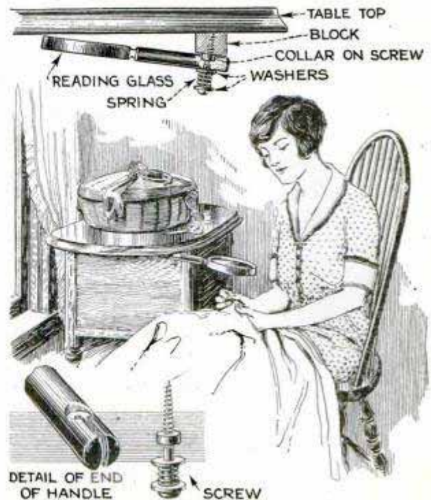
Magnifying Lens Mounted on Edge of Sewing Machine or Table Eliminates Eye Strain
