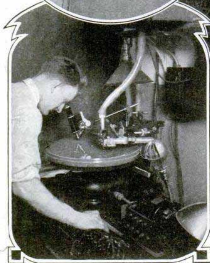
Soundproof Camera Booth, Special Microphones Above and Recording Apparatus Showing Wax Disks
