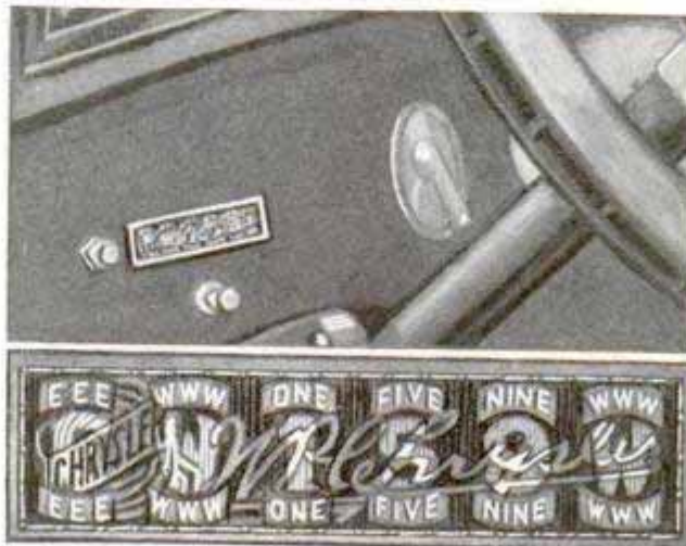
Auto Number Plate in Position on Dashboard, and Close View Showing How It Is Embossed
