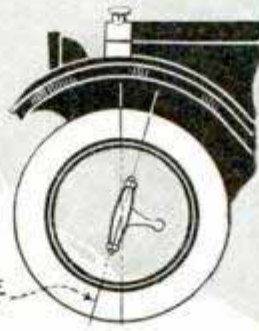
Above, Gauge That Automatically Registers "Pitch" of Axle; Below, Diagrams Explaining Caster Effect
