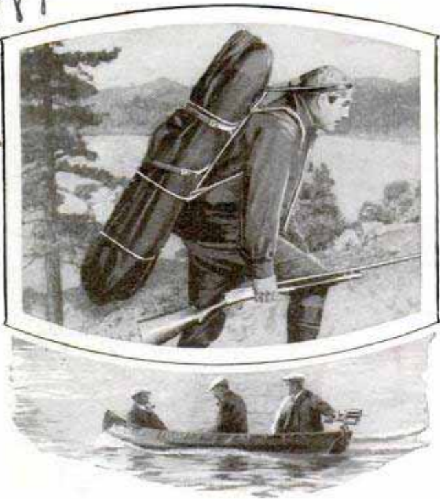
Canoe Folded into Pack and Collapsible Three-Passenger Boat in Use with Outboard Motor
