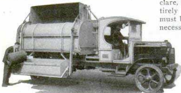
Filling the Lift Bucket on Refuse Truck Is Easy as It Is Lowered within Thirty Inches of the Ground
