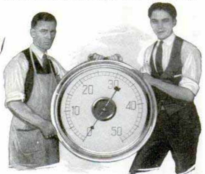
Huge Electric Meter to Save Steps in Substation, as It Can Be Read from Considerable Distances
