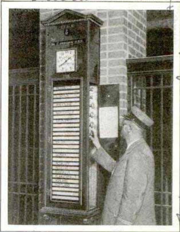
Setting the Train Indicator; a Turn of the Dials Exposes the Station Names
