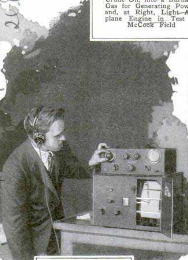
Sounder Measures Depth from Ship's Keel to the Bottom of the Ocean
