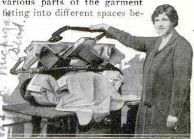
Shirt Ironer in Operation; It Presses Cuffs, Collar Bands and Yokes at a Great Saving in Time
