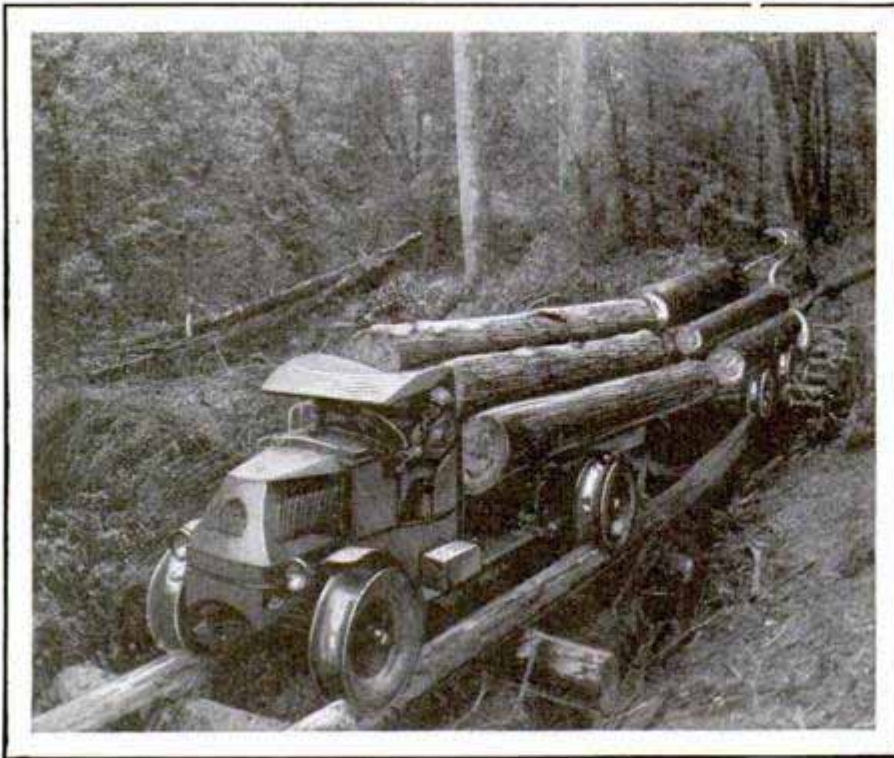
With Days of the Ox Team Almost Forgotten, Modern Loggers Adapt the Motor Truck to a Special Railroad for Hauling
