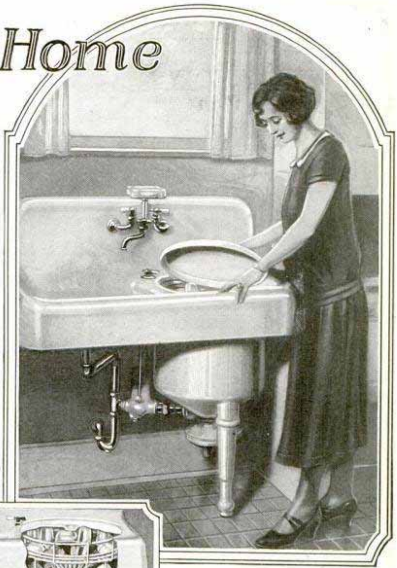
Electric Dishwasher, Built as Part of Sink, Cleans, Rinses and Dries; a Revolving Dasher Hurls Water to Every Part of the Stack and a Turn of the Handle Drains the Washer
