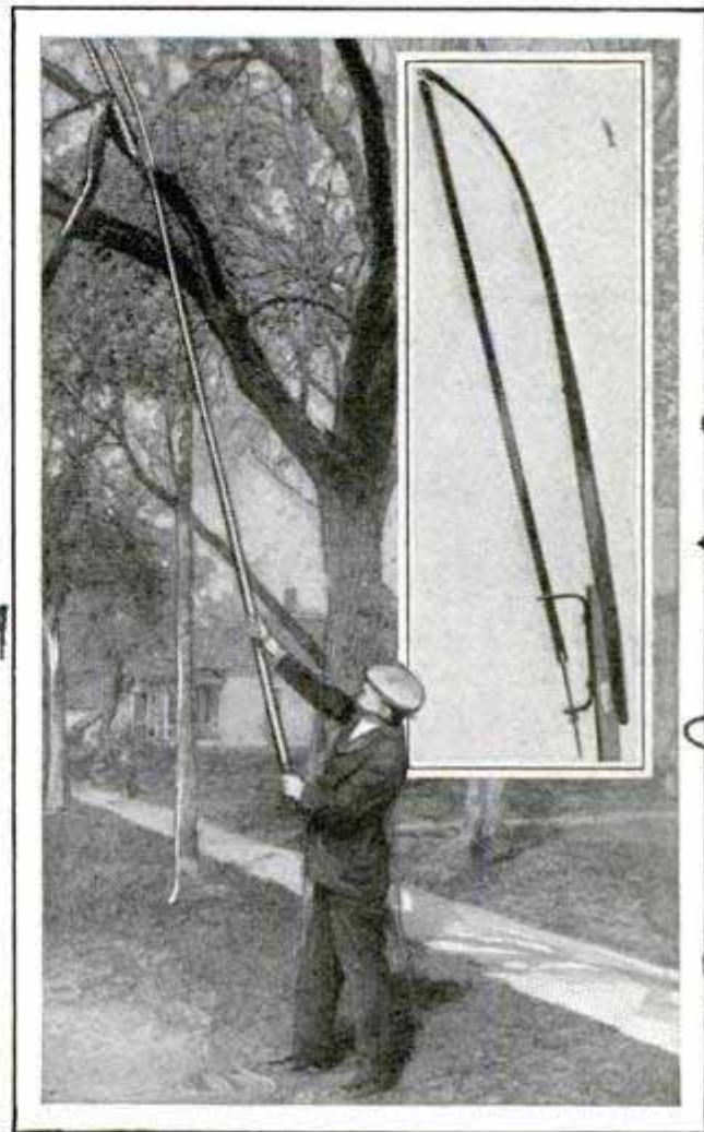
Trimmer in Use, and Inset Showing Its Narrow Saw Blade and Connection to Pole
