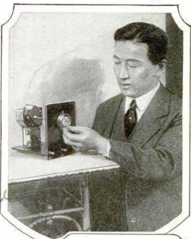
Above, Ushichiro Tokumi and His Radio Clock Switch That Can Be Set to Turn the Radio Set On or Off Automatically; Left, Complete Radio Set Built into a Table Which Harmonizes with the Other Furniture in the Room; the Loop Aerial Is Mounted on the Shelf under the Table, and a Cabinet Horn, Not Shown in the Photo, under the Instrument Panel or on the Table, as Desired
