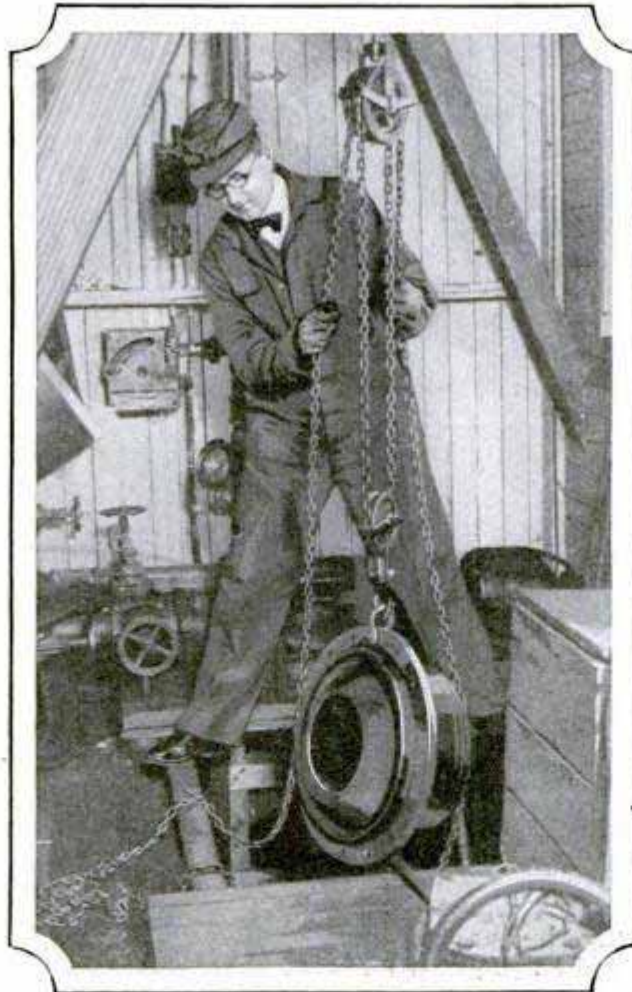
Receiving Instrument for Underwater Wireless with Which Conversations Have Been Carried On over a Distance of Two Miles
