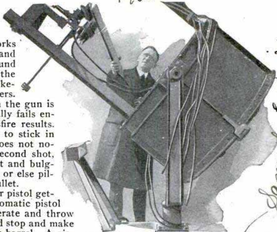
Holding Stick of Wood in Path of Rays from Huge Searchlight to Test Their Heat
