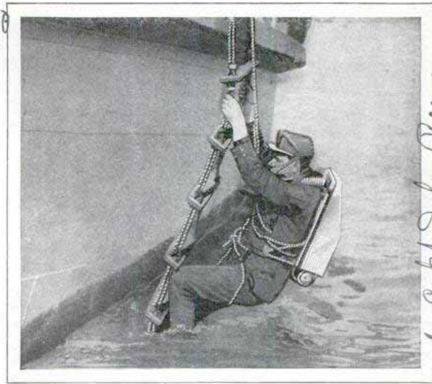
Using a Fireman's Smoke Helmet in Place of the Regular Suit, Diver Can Remain under Water Twenty Minutes
