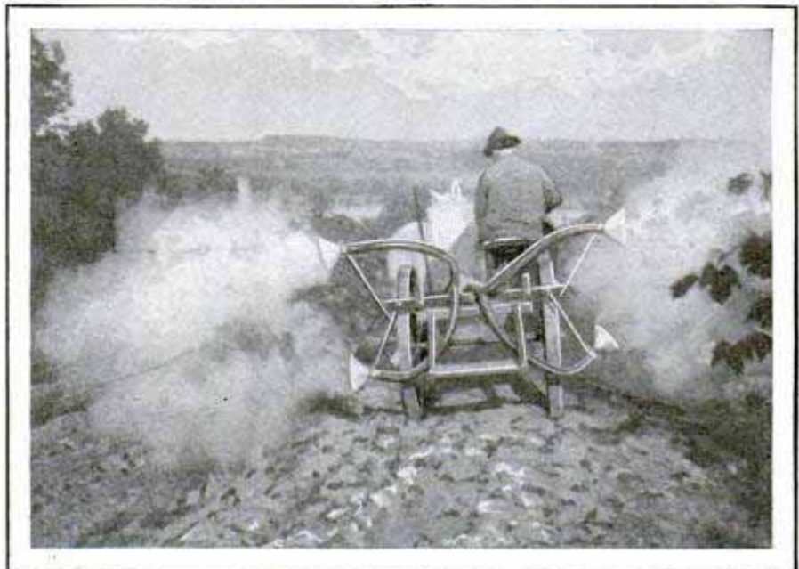
Dusting Two Rows at Once with the Motor Powder Spreader; Nozzles Reach Upper and Lower Parts of Plants
