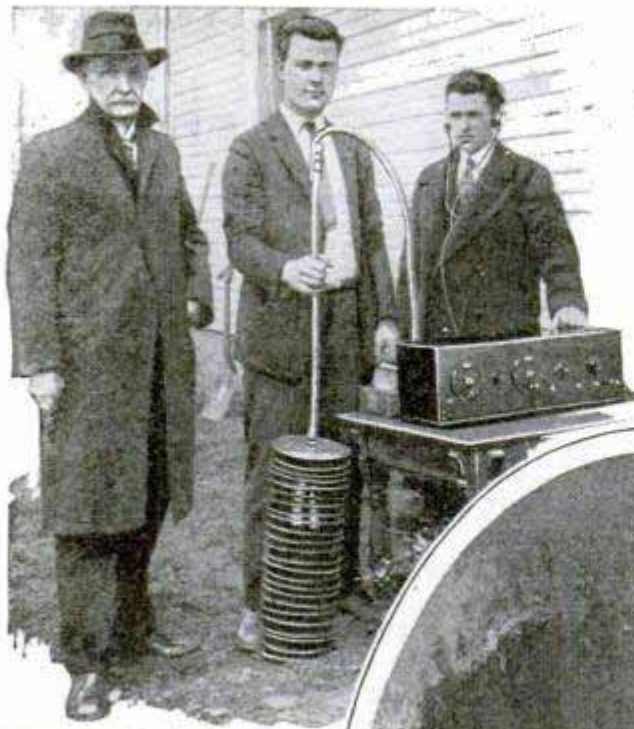
Left, J. Harris Rogers, Inventor of the Underground Aerial, and the Superheterodyne with Which It Was Used; Center, the Aerial in Its Water Pit, and Below, the Lead-In of a Buried Transmitting Antenna
