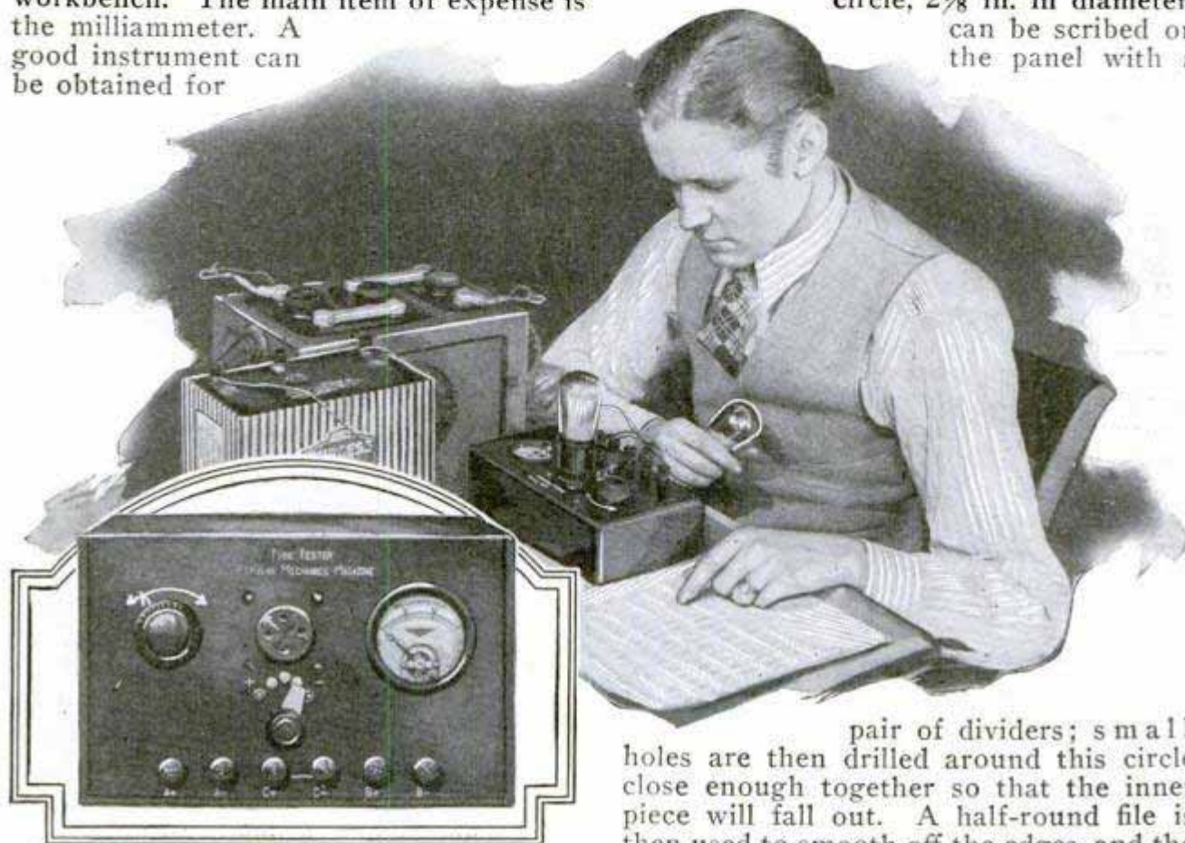
Tube Tester in Use; Detailed View of Front Panel Shown in Insert
