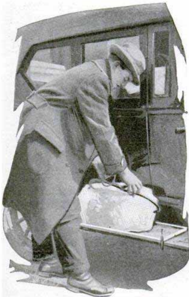
Shallow Pan on Running Board of Auto Carries Ice without the Need of Tying It
