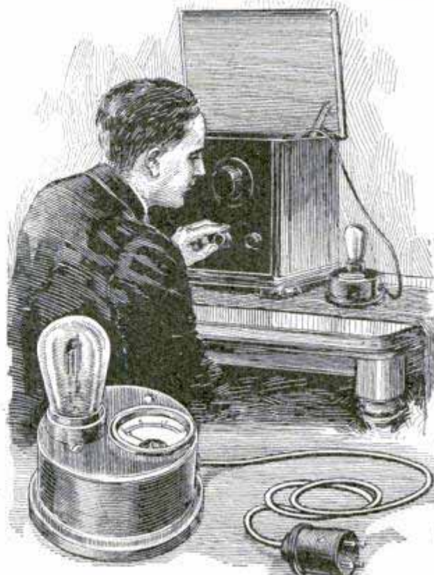
Tube Being Tested under Operating Conditions, Rheostat on Set Controlling Filament Supply
