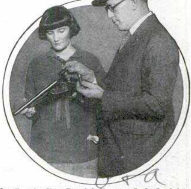
Loading the Short-Barreled Shotgun; It Is Carried in Shoulder Holster and Fired like a Revolver
