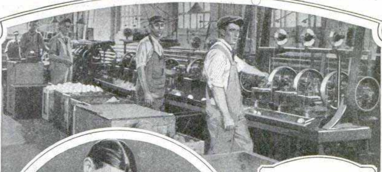
At the Automatic Winding Machines, Five Different Coverings Are Placed on the Cores to Give Uniformity of Size and Weight, Important Factors in a Baseball
