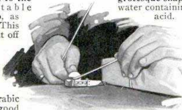
Can Opener Screwed to Top of Wrapping Table for Cutting Twine
