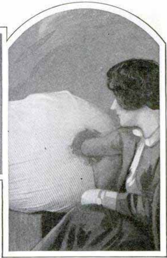
Learning Curve and Charts; Receiver in Hand of Deaf as "Listener," and Soundproof Bag in Which Subject Grasps Receiver While Undergoing Vibration-Interpretation Tests
