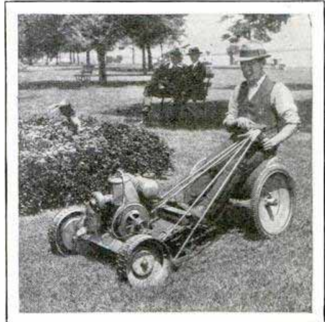
Motor Lawn Mower with Sulky Attached Saves Operator Work and Can Be Detached Quickly
