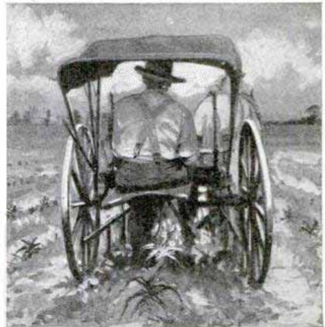
Old Buggy Top Makes a Good Shade on Cultivator and Provides Comfort for the Worker
