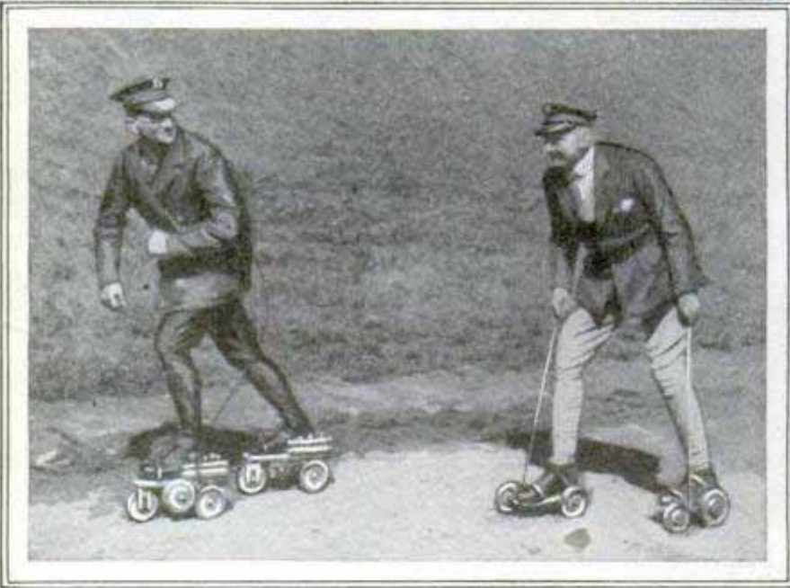
Roller Skates-like Tiny Individual Motor Cars Are Propelled by Acetylene Gas; Controls Manipulated by the Cords within Easy Reach While Both Grades and Rough Ground Are Traveled
