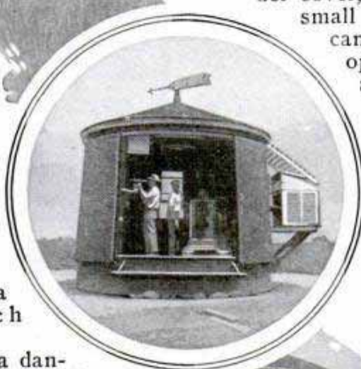
Above, Observer with Theodolite Prepared to Follow Ascent of Weather Balloon; Center, a Revolving Kite-Reel House, Where One Man Operates the Kite Reel and the Observer Charts Currents at Various Altitudes by the Kite's Movements; Below, Attaching the Recording Instruments to the Lead Kite
