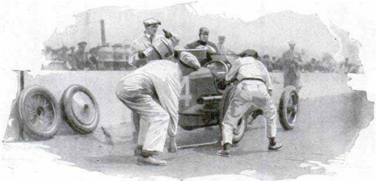
Changing a Tire and Refilling the Gasoline Tank Is Done in Twenty Seconds by a Trained Pit Crew, While the Pilot Has a Chance to Stretch His Cramped Muscles
