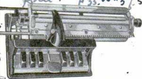
Typewriter on Which Blind Can Prepare Special Printing; It Has 220 Parts and Produces Fifty Symbols
