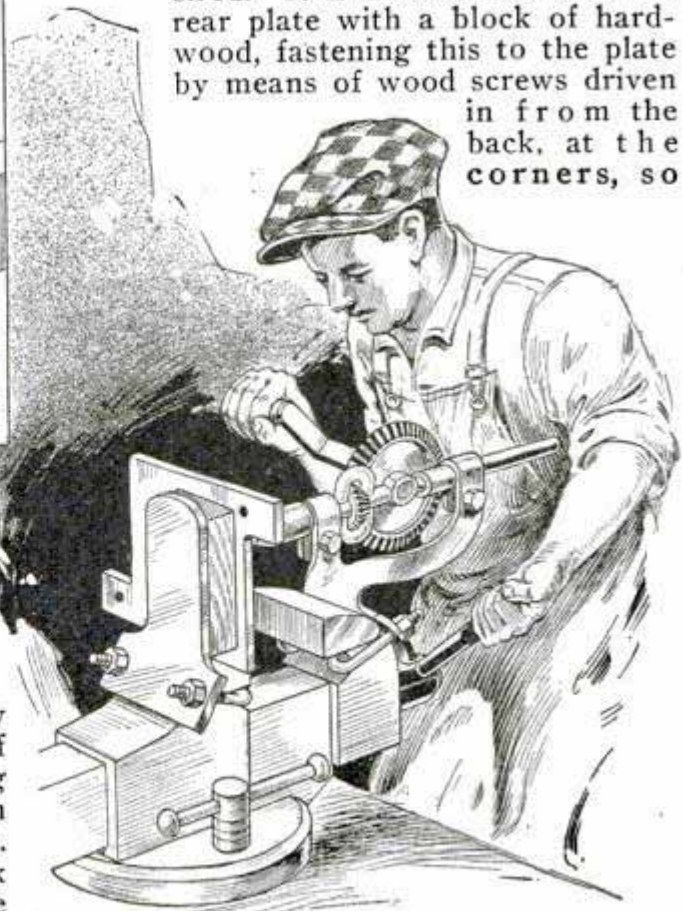
A Simple Attachment That Converts the Breast Drill into a Drill Press with a Positive Feed
