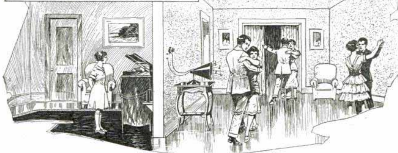
Relaying Phonograph to Another Room for Dancing by Means of an Improved Arrangement, Consisting of a Telephone Microphone, Dry Cells, Rheostat and Receiver, Fitted to a Tin Horn.
