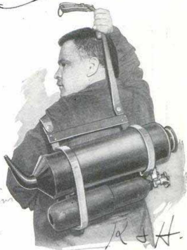
With Fire Extinguisher Slung on Back, Hands Are Free for Carrying Other Tools
