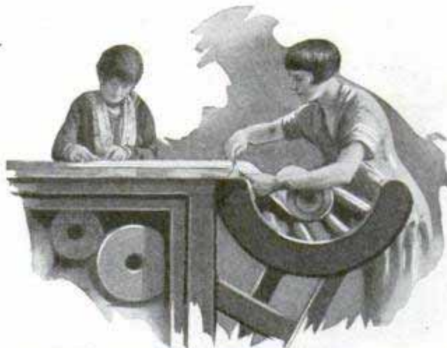
Cradle on End of Store Counter Facilitates Cutting Off Measured Lengths from Paper Rolls
