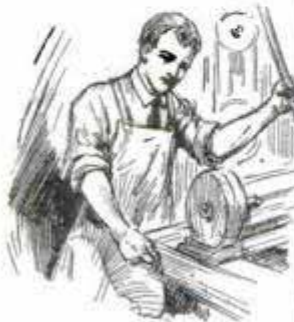
Upper Left, the Grinder Mounted on the Column for General Grinding; Right, Used to Grind Lathe Centers
