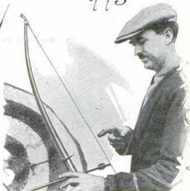
Sight in Middle of Bow Helps Archers in Aiming at Target on Long Shots
