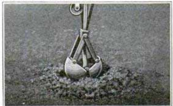
Improved Sand Bucket Works Like Clamshell, and with Its Use, Five or Six Loads Can Be Removed from a 100-Foot Well per Minute
