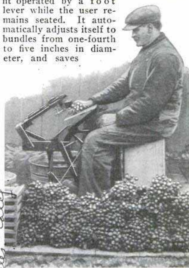
Harvesting Vegetables in Adjustable Press Which Binds Them Securely and Ties Knots
