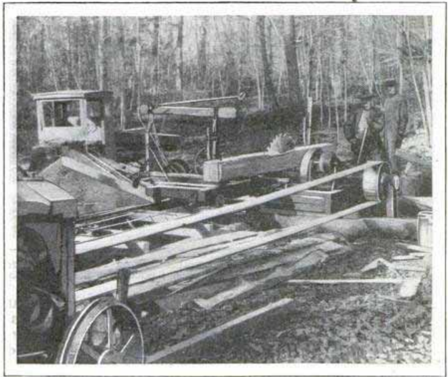
Running a Sawmill with Power from a Tractor; the Outfit Can Be Hauled Directly to the Timber
