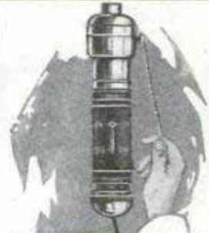
Plug with Pointer Tells When Current Is On
