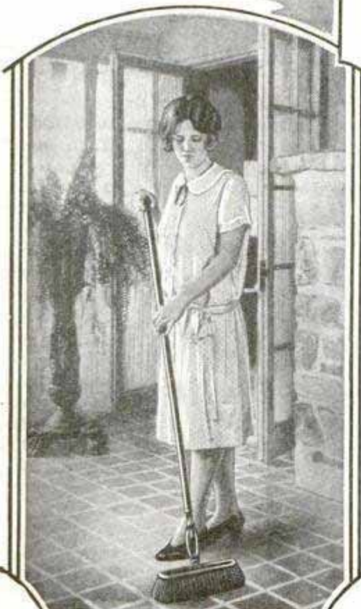
Push Broom Connected to Handle by Swivel Is Used in Three Positions for Difficult Places
