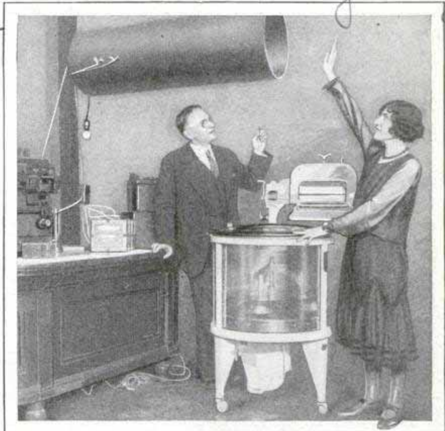
Waving the Hand in Front of the Cylinder Casts a Shadow Which Is Made to Close a Circuit and Start the Washer
