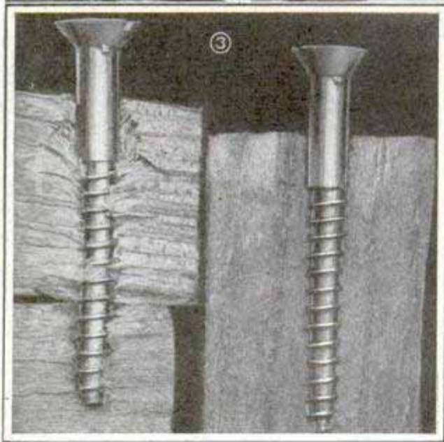
Left, Effect of Screw Binding in One Member; Right, Screw Driven in End Wood
