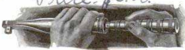
Wrench with Set of Different-Sized Sockets That Slip into the Handle
