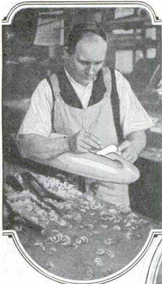
Workman, Above, Checking the Fair Lines as He Carves a Testing Model to Be Tried Before the Owner Orders His Full-Size Yacht Built; at Right Is a Model, Complete in Every Detail, of an Old-Time Frigate; Center, Rigging a Model of the Cup Defender "Resolute," Which Defeated the "Shamrock IV" for the America Cup in 1920; Many of These Boats Are Sold in Parts for the Owner to Build at Home
