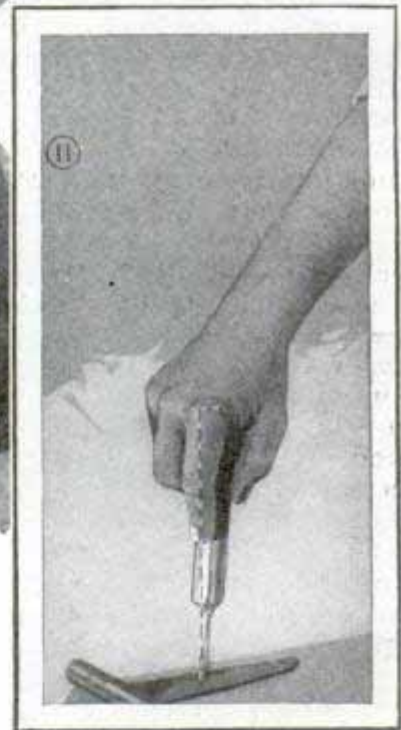
Fig. 10, Effect of Using Long Screwdriver; Note Lever Arm Indicated by Dotted Lines; Fig. 11, Short Lever Arm Formed by Short Screwdriver
