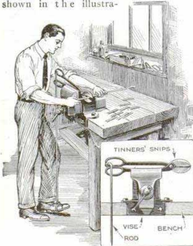
Cutting Heavy Work with Ordinary Tinnners' Snips by Foot Power
