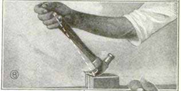
Fig. 6, Starting to Draw Nail; Fig. 8, Use of Block When Nail Is Partly Drawn
