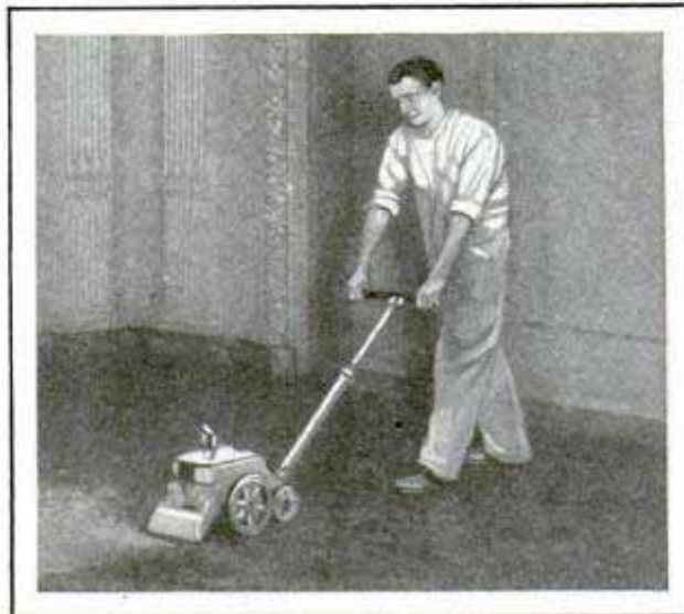
Combination Floor Scraper and Sander, Run by Spring Motor and Steered by User
