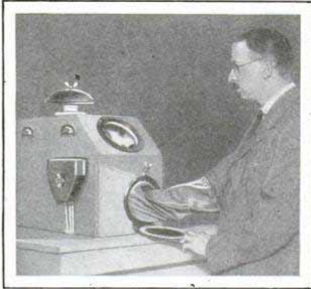
Waterproof Wireless Transmitter for Lifeboats, and How Operator Employs Protecting Sleeve
