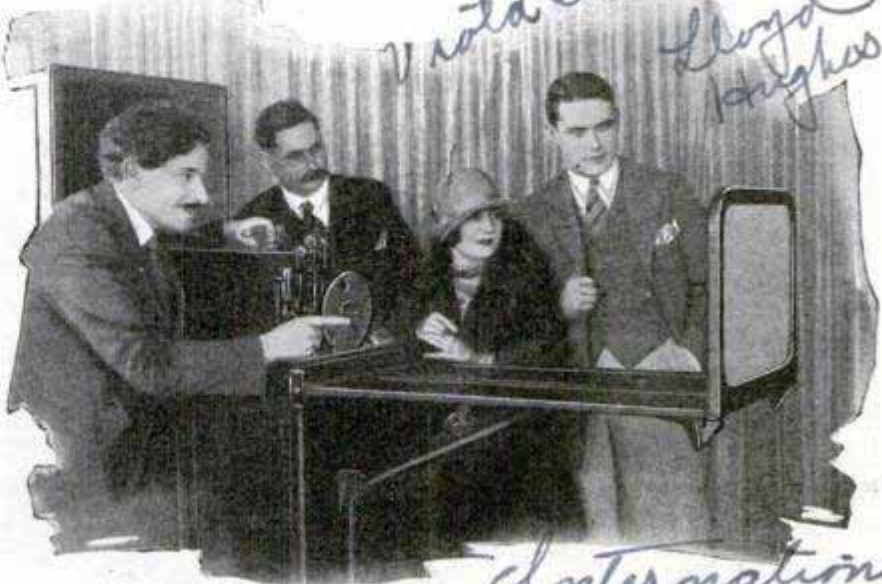
Movies from the Phonograph; Projector Attached to Motor in Cabinet Throws Pictures on Transparent Screen in Front
