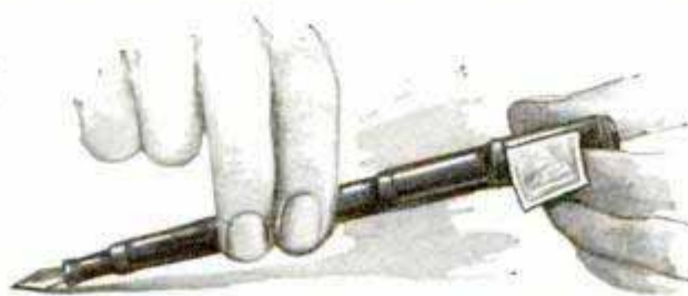
Unrolling Stamp through Slot in Side of Pen-Holder Barrel by Twisting
