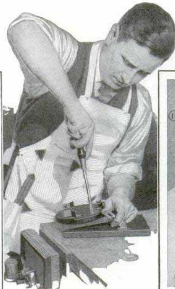
Fig. 10, Effect of Using Long Screwdriver; Note Lever Arm Indicated by Dotted Lines; Fig. 11, Short Lever Arm Formed by Short Screwdriver
