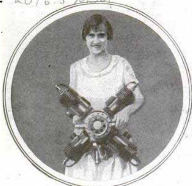
Illustrating Light Weight of Motor for Small Airplanes; It Registers Sixty-Four Pounds
