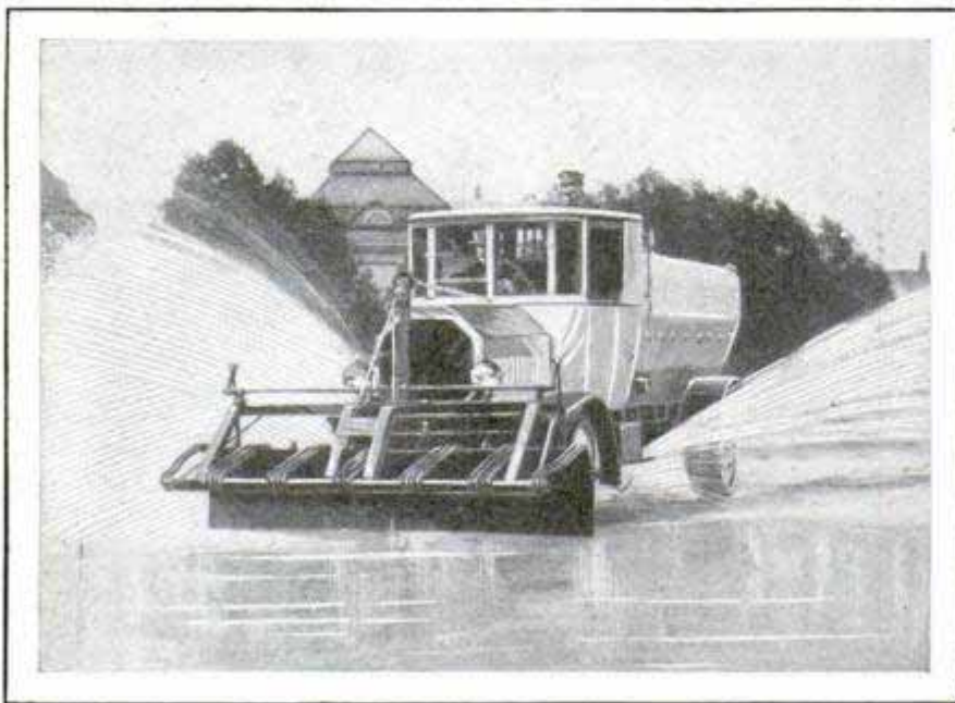
Combination Truck in Action; Plow for Scraping Snow or Dirt in Front, Street Flushers at Sides, Operated by Powerful Pumps
