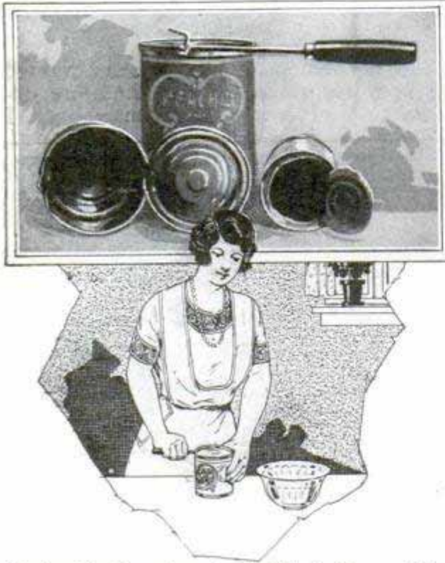
Cutting Tin Cans through the Side Is Easy and Permits All the Food to Be Removed
