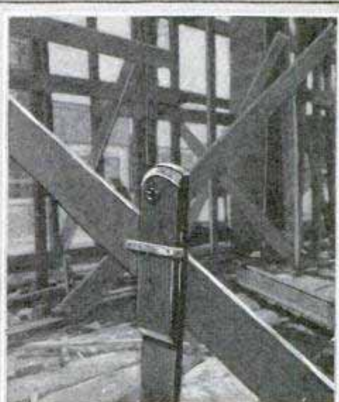
Simple Wood Vise Attached to Strut for Filing Circular Saws
