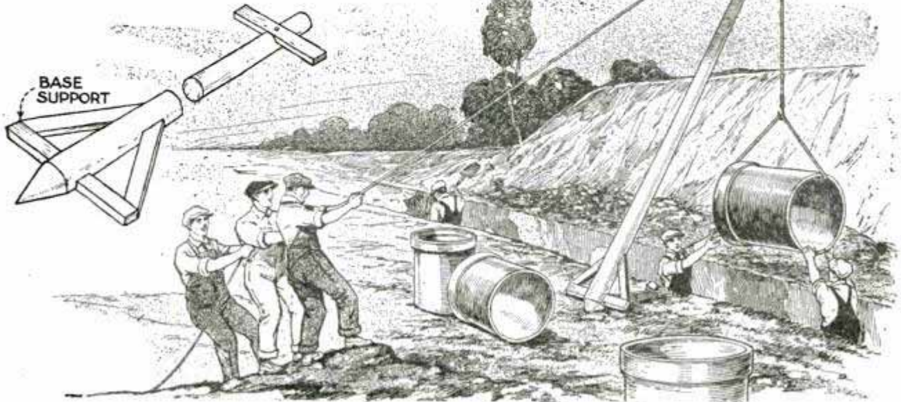
Simple Improved Derrick for Farm Use Which Makes It Possible to Lift Objects of Considerable Weight
