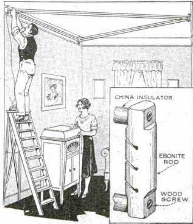
Simple Indoor Aerial Supported by Ebonite Rods; Lower Right, Detail of Construction
