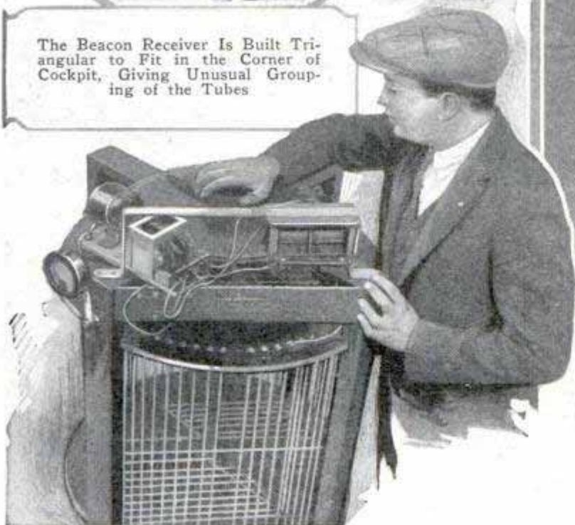
With the Goniometer, at the Left, It Is Possible to Direct the Radio Beacon to Any Point Desired by Merely Shifting the Revolving Pointer; the Queer Apparatus in the Foreground, Driven by the Small Motor, Carries Notched Disks Which Automatically Send Out at Five-Second Intervals the Dots and Dashes Which Interlock to Guide the Plane; Above Is a Big Rectifier, Which Changes Alternating Current to Direct Current
