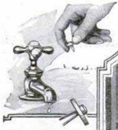
Faucets Can Be Mended without Tools by Using This Split-Pin Washer That Is Pushed in Place
