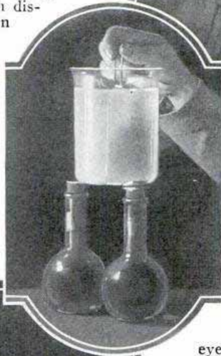
Mercury Lamp in Quartz Globe and Black Glass, Which Passes Only Ultraviolet Rays, Above; Water with a Small Amount of Esculin, at Bottom, Remains Clear as Crystal, but Becomes Fluorescent under the Rays, Center
