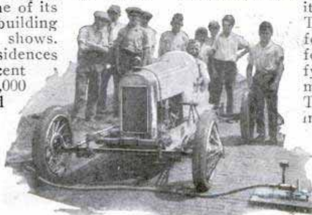
When Auto Runs over Hose, Plunger Starts or Halts Stop Watch on Stand
