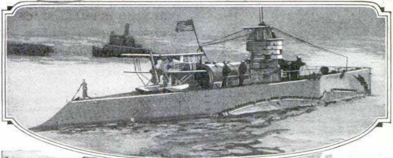
Seaplane on Submarine Deck Ready for Flight, and View of Storage Tank with End Removed to Show Nose of Plane Tucked Away After Wings Were Taken Off
