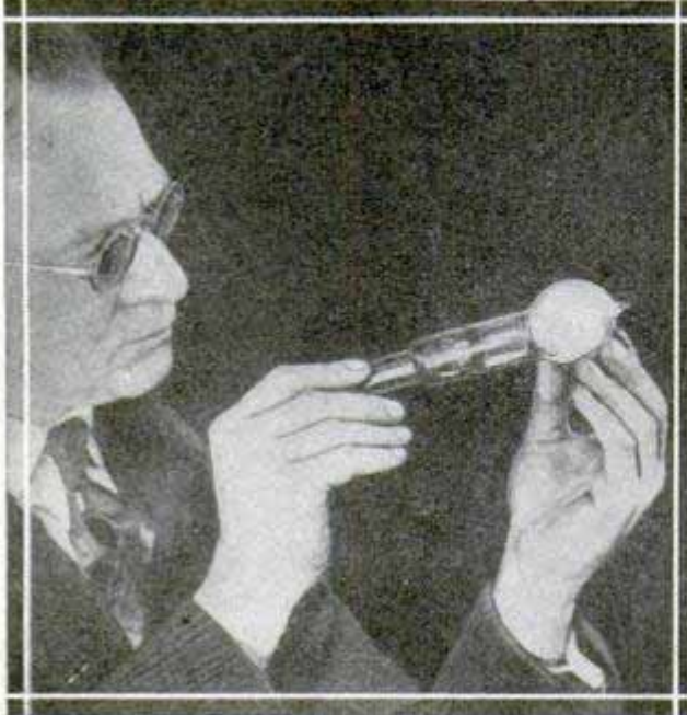
Sensitive Tube to Help Radio Movies; It Emits Electric Impulses When Light Strikes It
