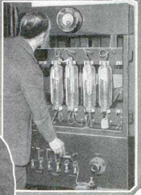
With the Goniometer, at the Left, It Is Possible to Direct the Radio Beacon to Any Point Desired by Merely Shifting the Revolving Pointer; the Queer Apparatus in the Foreground, Driven by the Small Motor, Carries Notched Disks Which Automatically Send Out at Five-Second Intervals the Dots and Dashes Which Interlock to Guide the Plane; Above Is a Big Rectifier, Which Changes Alternating Current to Direct Current
