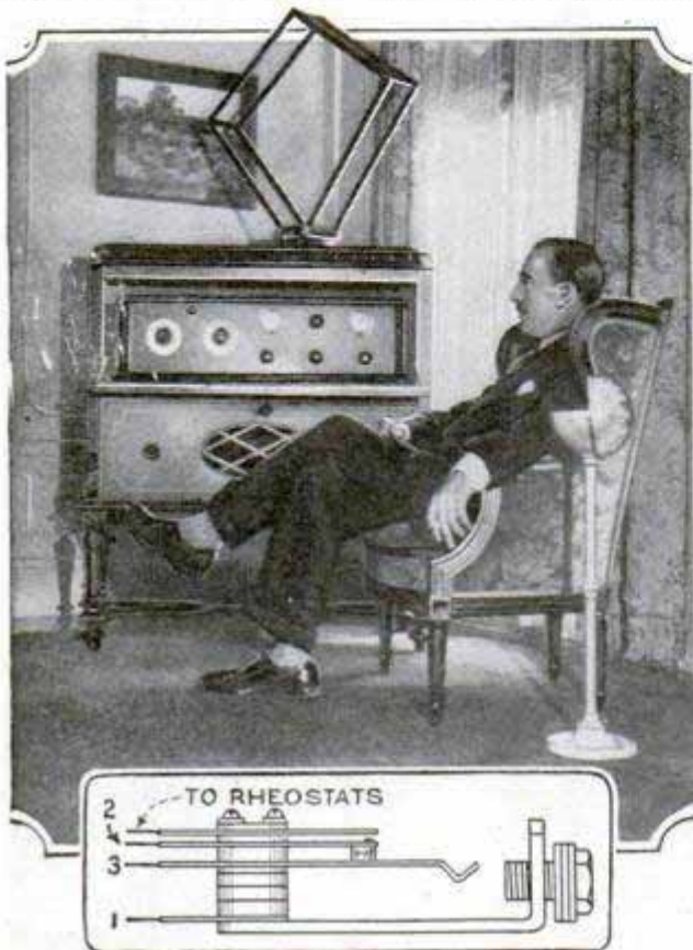
Side View of Jack, with Springs Numbered to Correspond to Diagram
