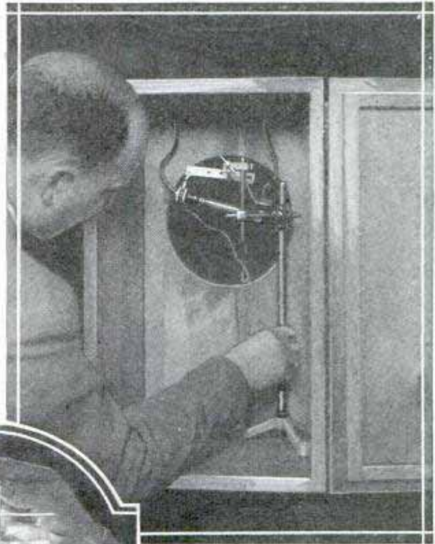
Mercury Lamp in Quartz Globe and Black Glass, Which Passes Only Ultraviolet Rays, Above; Water with a Small Amount of Esculin, at Bottom, Remains Clear as Crystal, but Becomes Fluorescent under the Rays, Center
