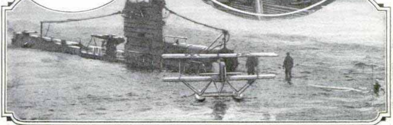
Tackle for Lifting Plane So That Wings May Be Attached or Unfastened for Storing, and Ship on the Water; to Launch It, Submarine Simply Ducks and Leaves It Floating
