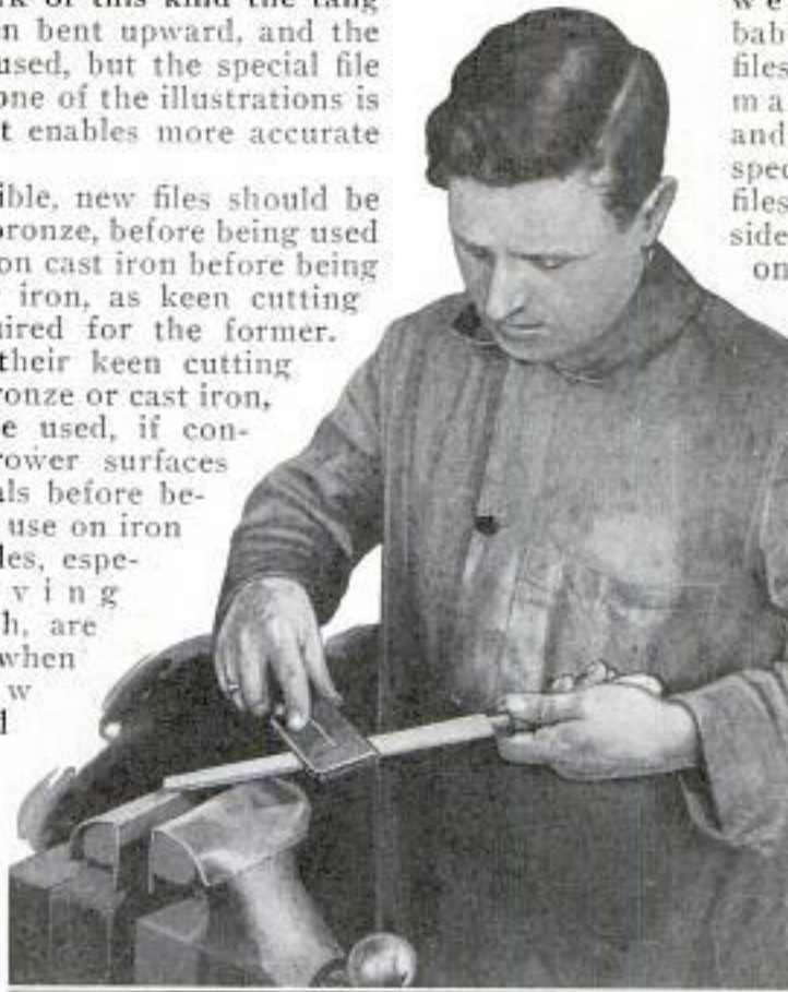
Fig. 12. Cleaning Teeth of File with Card File, to Prevent Scratching Work
