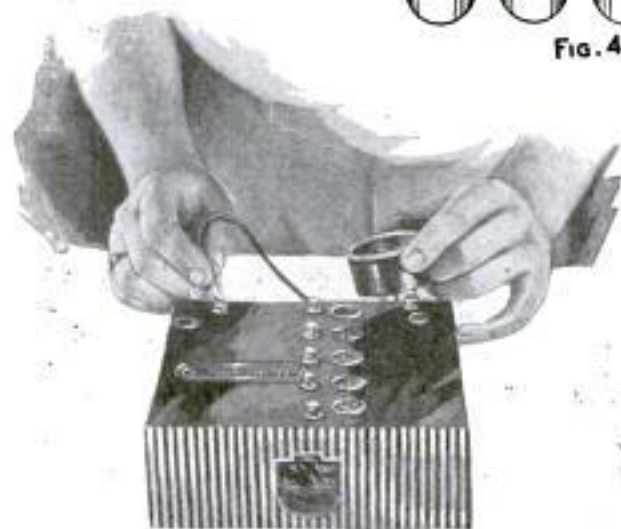
Testing B-Battery with Voltmeter; Diagrams Showing the Various Methods of Combining Dry-Cell Units for Radio Sets Employing One Up to Eight Tubes, and Above, Proper Manner of Making the Connections
