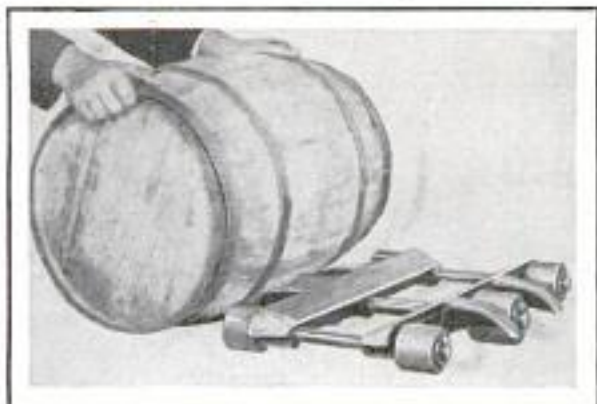
Barrels Are Loaded On Easily from the Side without Danger of the Truck Slipping
