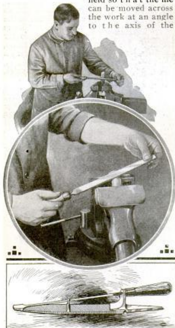
Figs. 8-11. Upper Left, Filing Convex Surface; Lower Left, File Holder for Broad Surfaces; Upper Right, Convenient File Rack; Lower Right, Chalking a File
