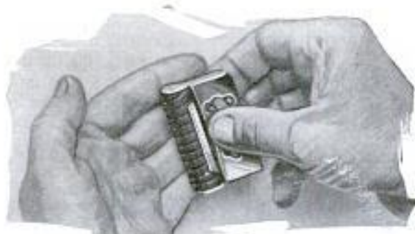
Sharpening Safety-Razor Blade in Stropper That Is Rolled over Palm of Hand
