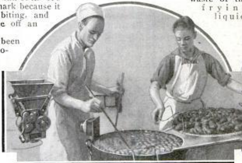
Electric Heater Clamped to Doughnut Kettle below Chef’s Right Hand; Keeps the Frying Liquid at Cooking Temperature
