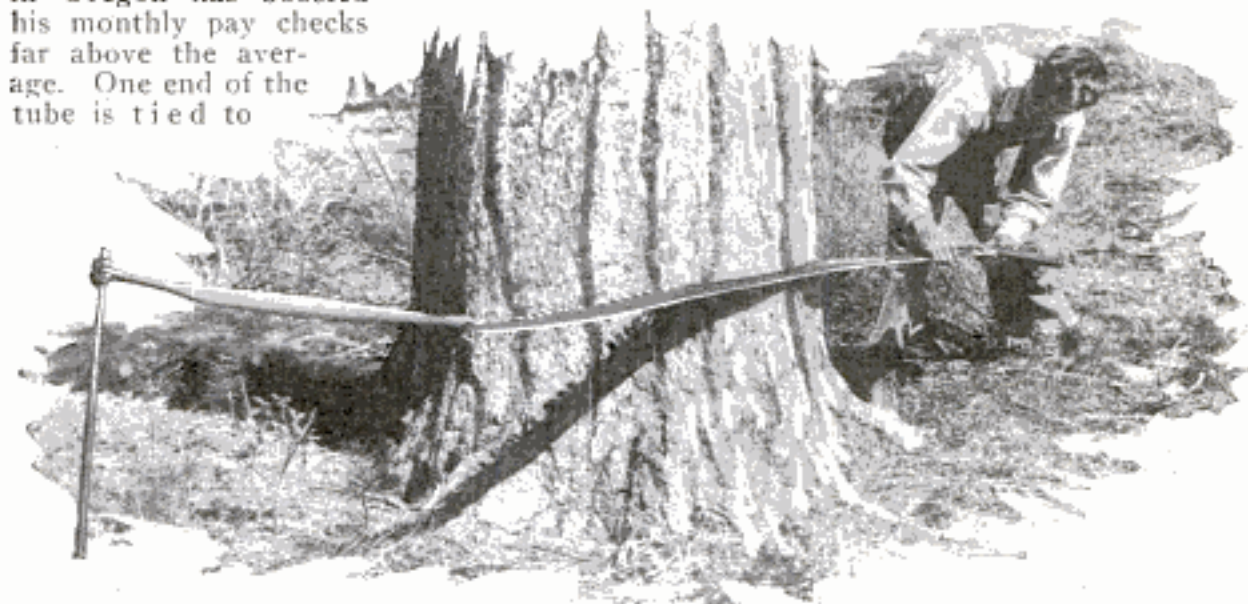
Use of an Old Inner Tube Eliminates One Man on a Two-Man Crosscut Saw in Felling Trees in Oregon Logging Camp, Boosting the Ingenious Inventor's Pay Check
