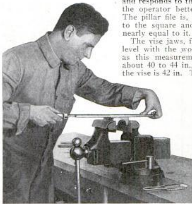
Fig. 1. Position for Filing in Vise; Note That Vise Jaws Are at Height of Elbows
