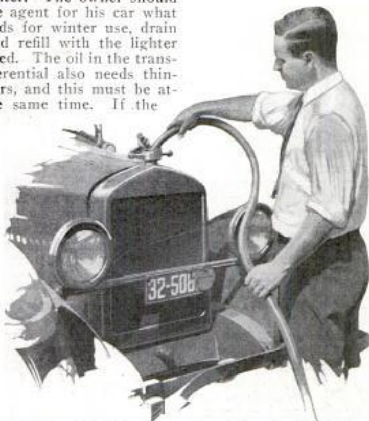
Flush Out the Radiator Thoroughly to Clean It of Rust before Filling with the Anti-Freeze Solution
