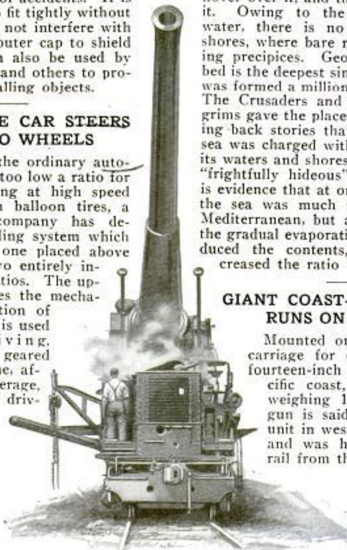
Monster Coast-Defense Gun Mounted on Railway Carriage
