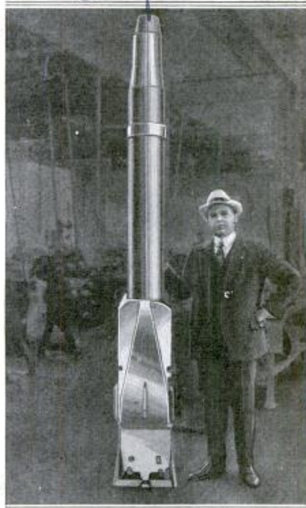
Inventor with Huge Four-Bladed Bit to Save Time in Oil-Well Drilling
