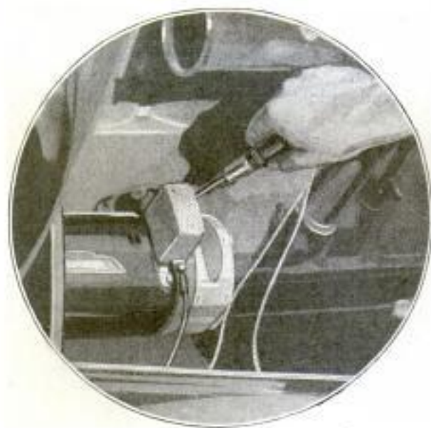
Above, Left, Kinks in the Gas Piping Should Be Fixed; Right, Various Points in the Fuel Lines Where Sediment May Collect; Below, Removing Generator-Brush Cover, and at Left, Removing the Strainer from the Carburetor
