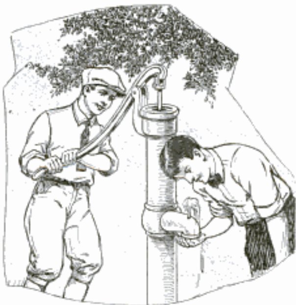
Converting the Ordinary Pump into a Sanitary Drinking Fountain
