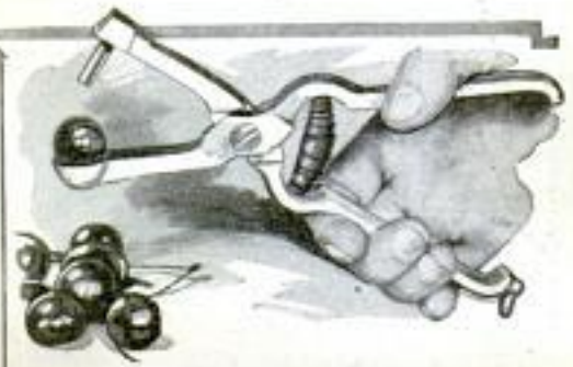
Cherry Stoner Works Like Punch, Pushing Pit through Hole in Cup
