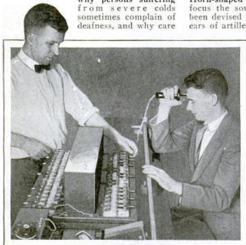
An Ear Test by Radio; Dr. Kranz, at Left, Changing Tone's Intensity While Subject Alters Pitch with Sliding Bar
