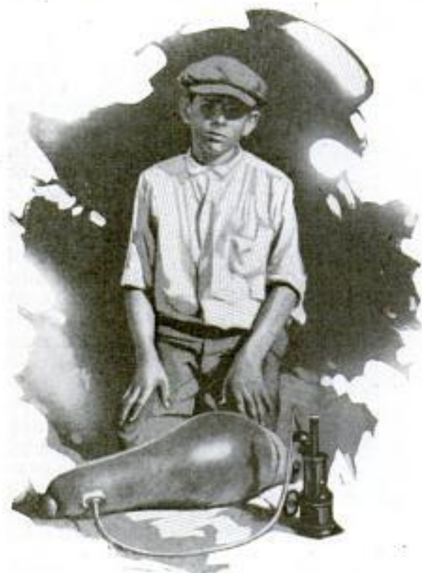
Old Inner Tube Used as an Air-Pressure Tank for Running Miniature Steam Engine
