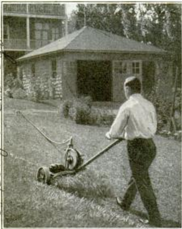
Electric Lawn Mower in Use; Current Cable Attached to Light Socket near House
