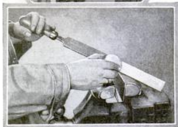
Figs. 8-11. Upper Left, Filing Convex Surface; Lower Left, File Holder for Broad Surfaces; Upper Right, Convenient File Rack; Lower Right, Chalking a File
