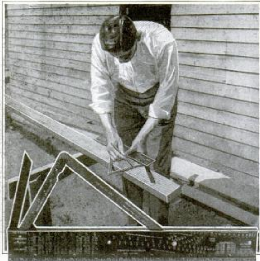
Side View of Miter Gauge, Showing Folding Rule, Tables and Holes, and Using Instrument to Mark Rafter
