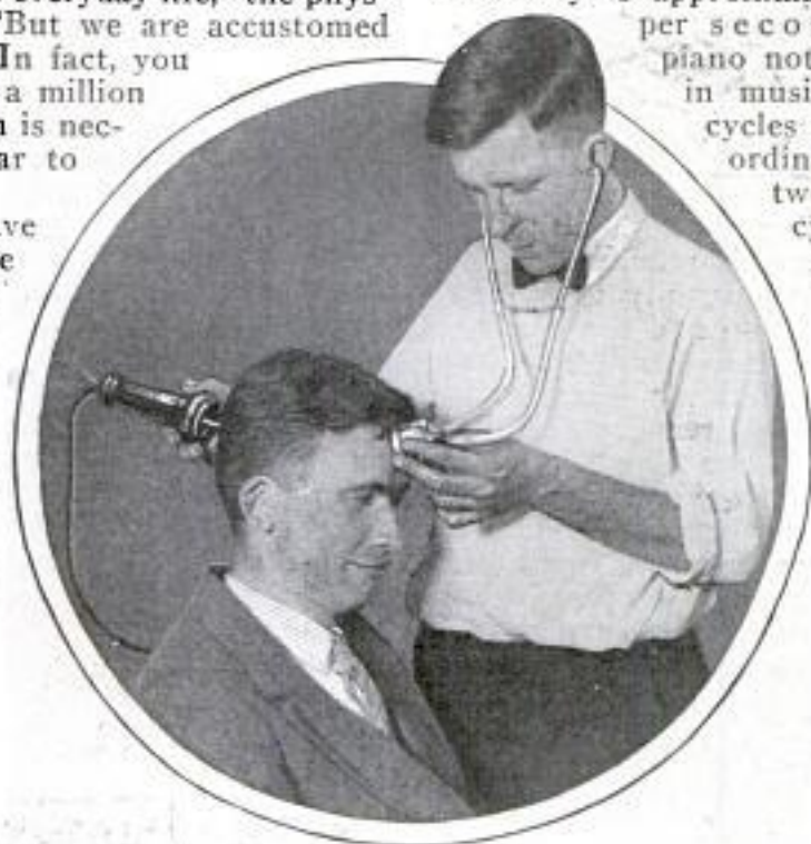
Testing a Doctor's Stethoscope by Listening to Sound Vibrations as They Pass through Subject's Head from Special Receiver
