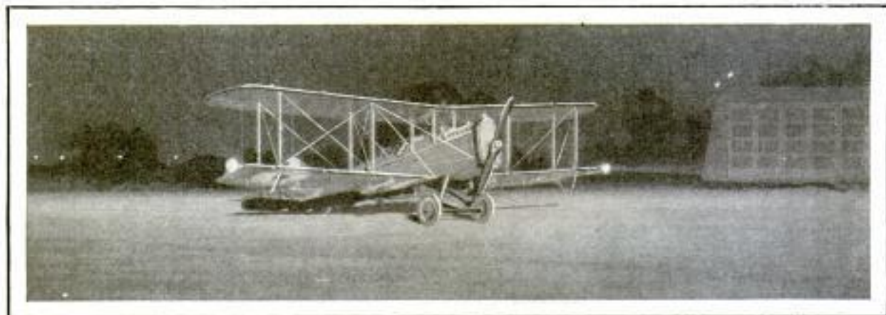
An Airplane Making a Safe Landing Guided by Its Own Wing-Tip Flares, Which Enable the Pilot to Determine the Smoothness of the Field and Level Out at the Correct Height above It
