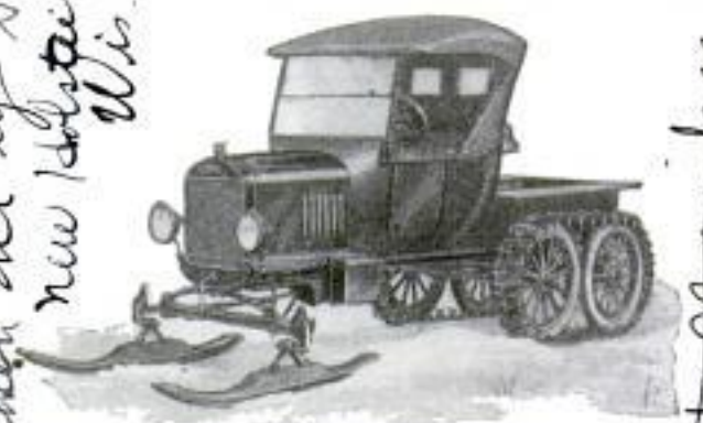
Ready for Winter Trips, Auto Fitted with Caterpillar Tread Behind and Runners in Front
