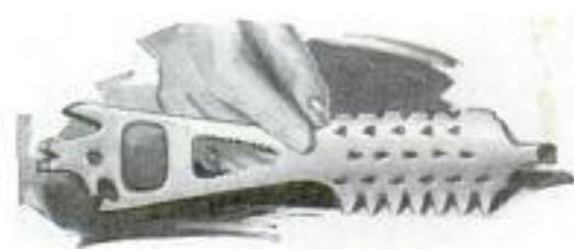
Stove Lifter, Tack Puller, Hammer, Fish Sealer and Screwdriver are Combined in This Single Tool
