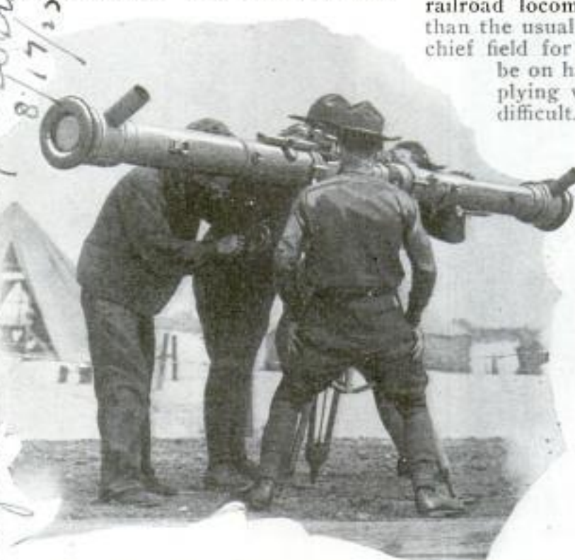
Soldiers Using Special Finder to Gauge Height of Moving Airplane Targets during Tests with Anti-Aircraft Guns
