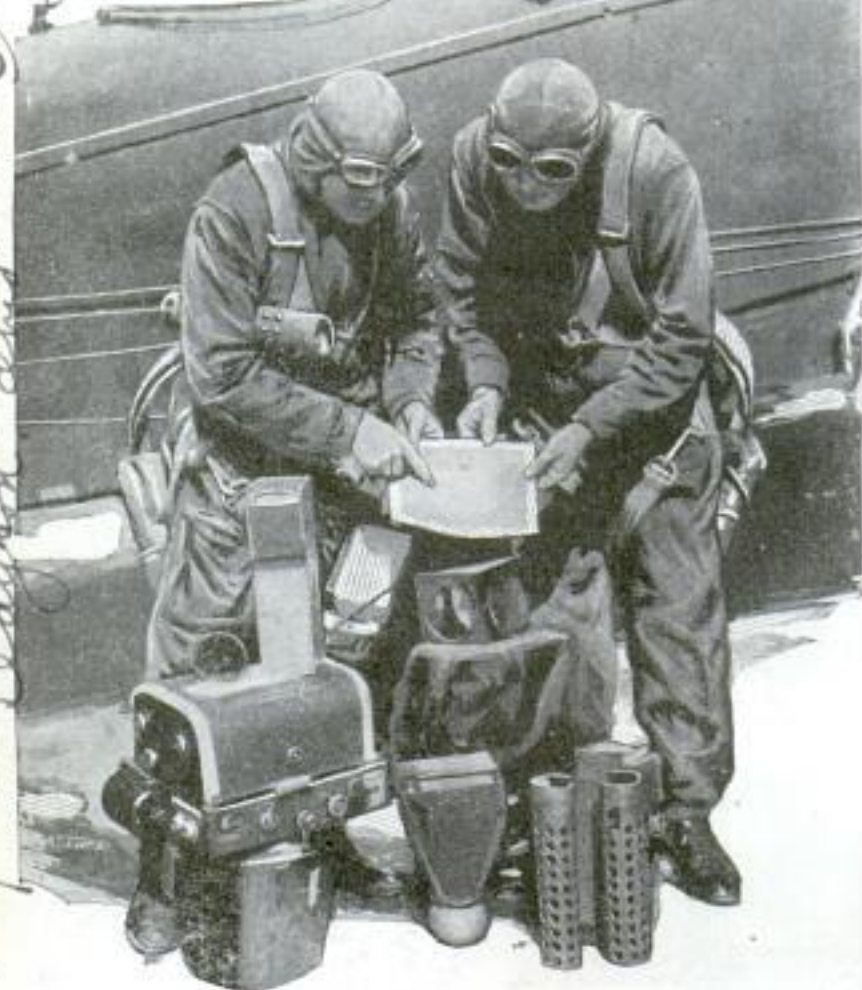
Aviators Examining Print of Exposure Developed in Seven Minutes on Airplane; Two of the Cylinder Carriers in Foreground.
