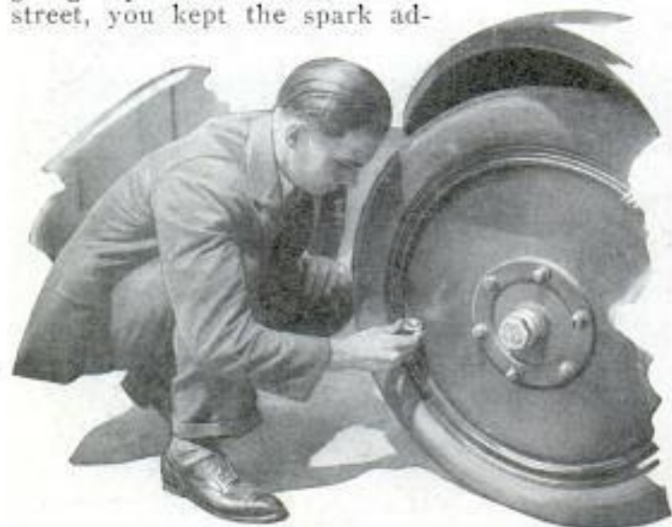
Keep the Tires Inflated to the Proper Pressure to Reduce "Rolling Resistance"
