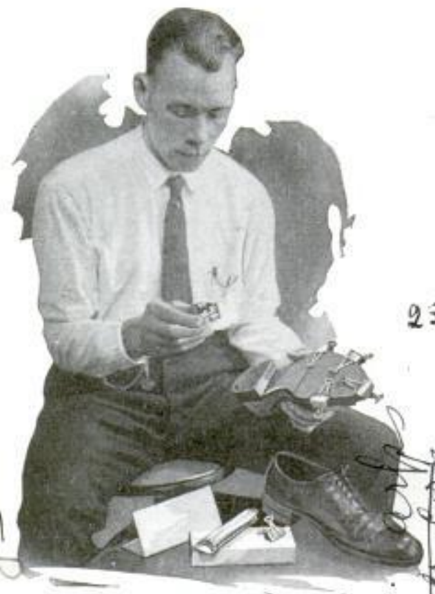
Home Shoe-Repair Outfit with Sole Glued On, and Held by Special Clamps
