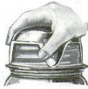
Toothbrushes Collect Germs if Left Exposed; This is Avoided in Metal Holder Attached to Wall or Cabinet with Shelf for Drinking Glass to Be Turned Upside Down over Them; Above, Fruit-Jar Sealer Straightens Caps, Insuring Air-Tight Fit
