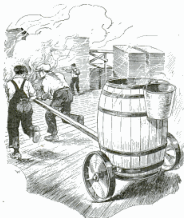
Wheeled Trucks for Water Barrels in Lumber Yard Help to Prevent Large Fires
