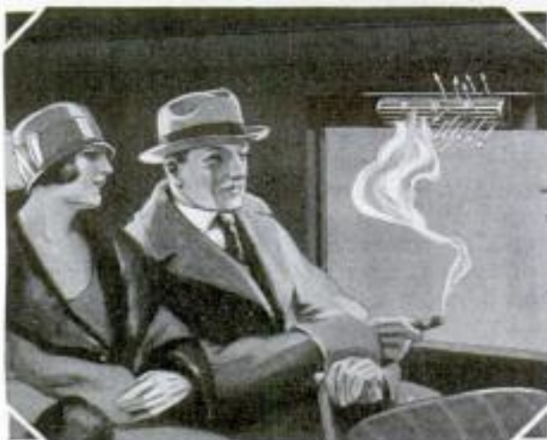
Ventilator Installed: Arrows Indicate Incoming Air; Smoke Pours through Other Apertures
