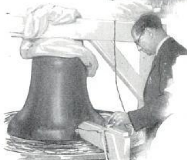
Recording Turns on Pulley Tester; Dutch Windmill for Grinding Feed, and Studying Bell's Vibrations in Mercury
