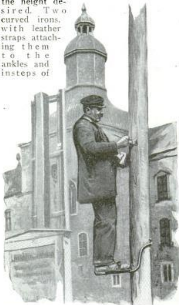
Climbing Irons Which Become Standing Platform When the Wearer Stops to Do Work on Pole
