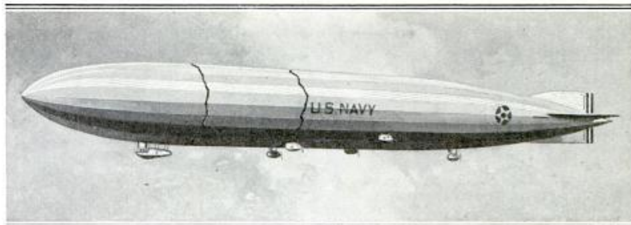
The Three Parts into Which the "Shenandoah" Broke When the Great Airship Was Torn Apart by a Terrific "Line" Squall While Flying over Ohio on Her Ill-Fated Western Trip
