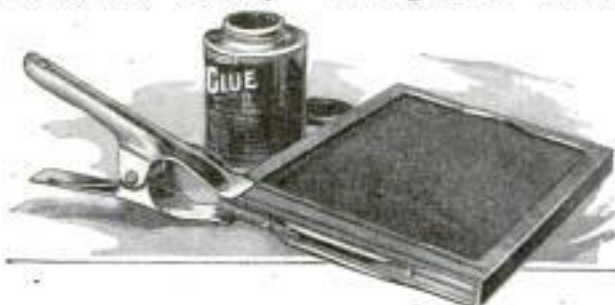
Mending Photograph Plate Holders Is Simplified by Using Clamp Plier to Keep Edges Together
