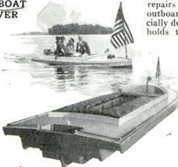
Boat Carrying Party of Four, and View of Stern Showing Arrangement of Air Chambers
