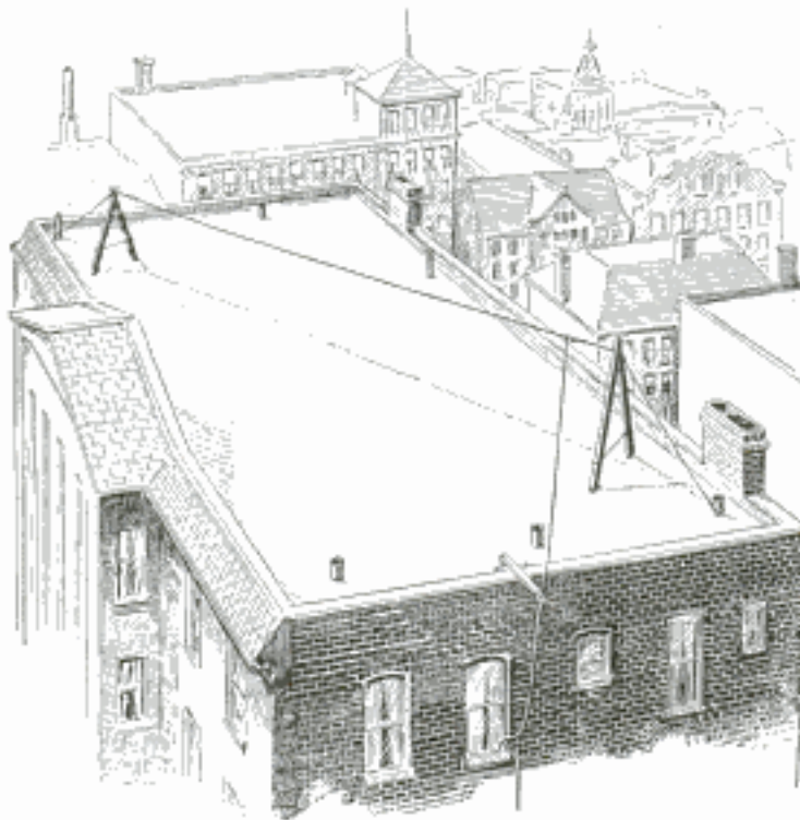
Simple Method of Erecting Single-Wire Antenna on Apartment-House Roof
