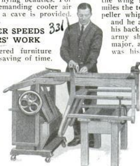
Web Stretcher Places Upholstery Straps in Minimum Time and Maintains Constant Tension
