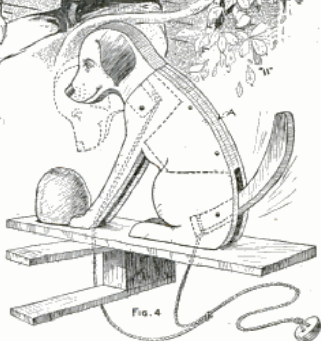
Assembly of the Parts of the Nodding Doggie. Showing How the Cords Are Attached to the Head and Tail and Led through the Platform
