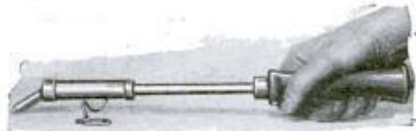
Iron with Swivel Point That Simplifies Soldering in Corners and Other Spots Hard to Reach
