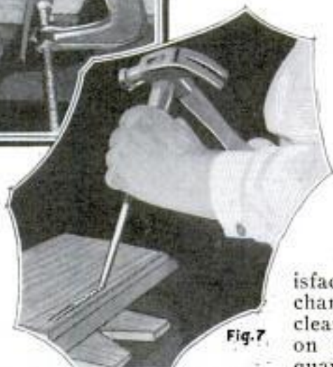
Fig. 5. Using One Side as Template for Other; Fig. 6, Clamping Box; Figs. 7 and 8, Cutting Grooves in Box for Housing Side and End
