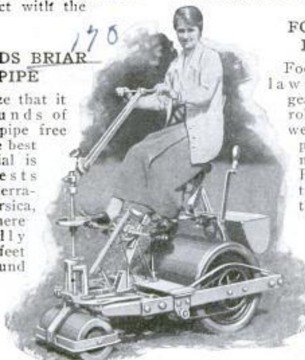
Special Gears on Mower Make Pedaling Easy
