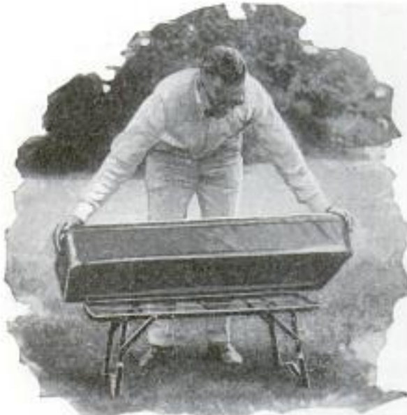
Collapsible Frame Used to Support Auto Seat and Convert It into Table for Picnics
