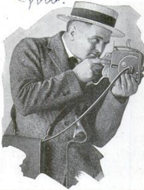
Spring Motor Concealed in Bag Cranks Small Motion-Picture Camera through Flexible Shaft
