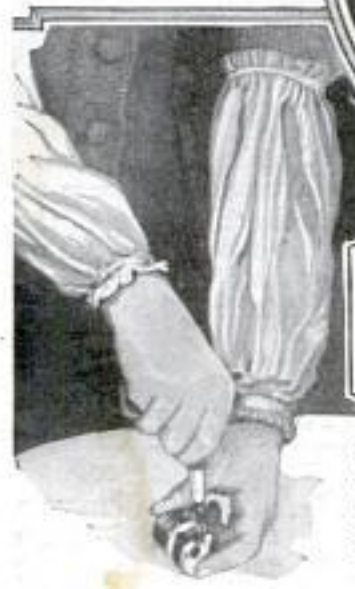
Right, Easily Operated Can Opener Removes Tops from Square as Well as Round or Oval Containers by Turning the Finger Screw
