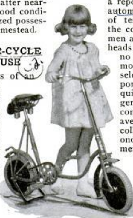
Scooter and Bicycle in One Can Be Used on Sidewalks and Has Rubber Tires.
