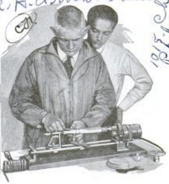
Versatile Tool in Operation, Doing Drilling, Buffing and Wood-Turning; the Motor Is Connected to a Lighting Socket and May Be Detached to Form a Portable Electric Drill
