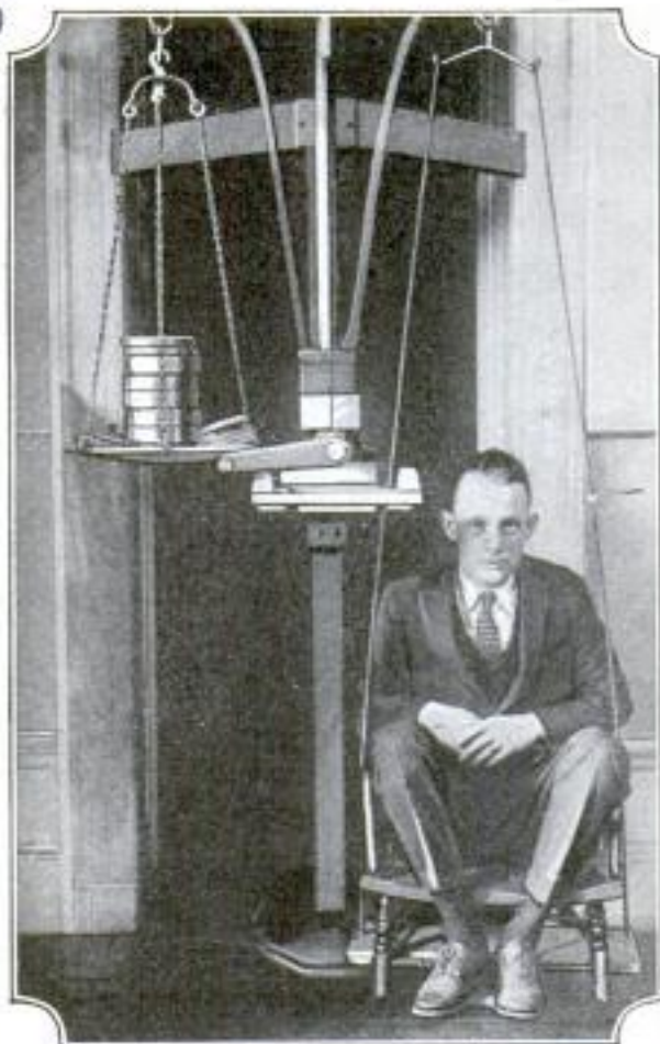
Weight Lost during Sleeping Hours Is Measured Accurately by These Delicately Adjusted Scales
