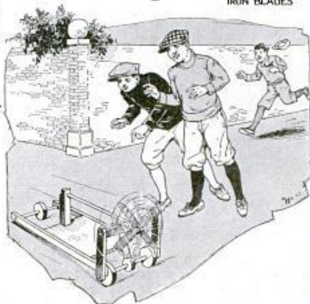
Self-Propelling Wind Wagon That Any Boy Can Build; It Consists of a Light Wooden Frame and Has a Sheet-Metal Propeller Which Drives It against the Wind with Surprising Speed
