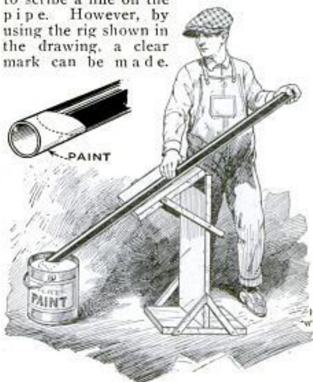
Time-Saving Method of Marking Pipe for Cutting at an Angle
