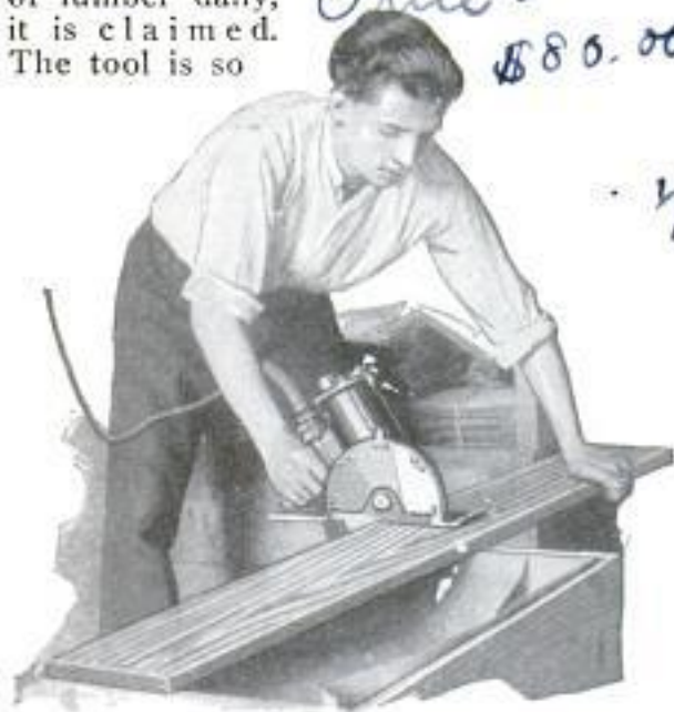
Lightweight Electric Circular Saw Cuts Variety of Materials and Is Operated with One Hand
