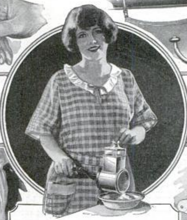
Food Grater with Sanitary Glass-Topped Hopper Prevents Injury to Fingers and Keeps Material Pressed against Blades, Saving Time and Labor
