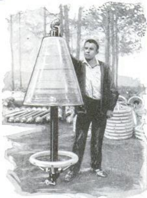
Insulators for the Sending Apparatus of Transatlantic Radio Stations Are Taller Than a Man
