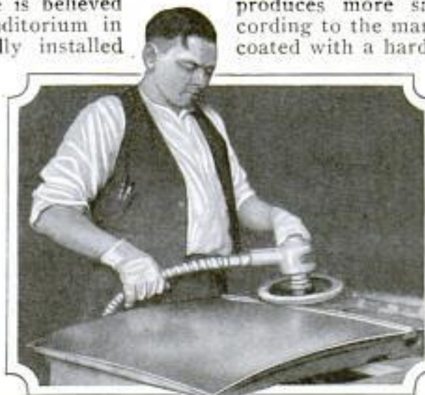
Buffing Surface with Portable Finisher Showing How It Is Adjusted for Beading
