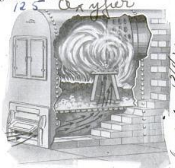
Drawing Illustrating Preheater in Operation. Air Passing under Grate, through Pot and Igniting Gases
