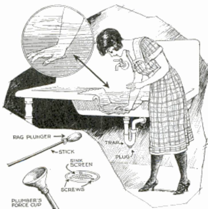
Above, Cleaning a Stopped-Up Sink, Using the Hand as a Force Cup; Left, the Plumbers' Force Cup and an Improvised Plunger
