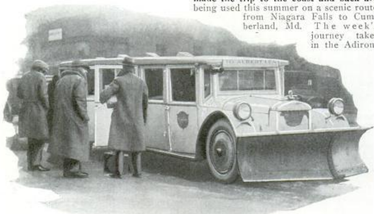
High-Powered Busses Push Their Own Snowplows over the Hard Roads of Minnesota in Winter
