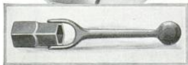
Spark-Plug Wrench in Use and Close View Showing Attachment of Swivel Handle
