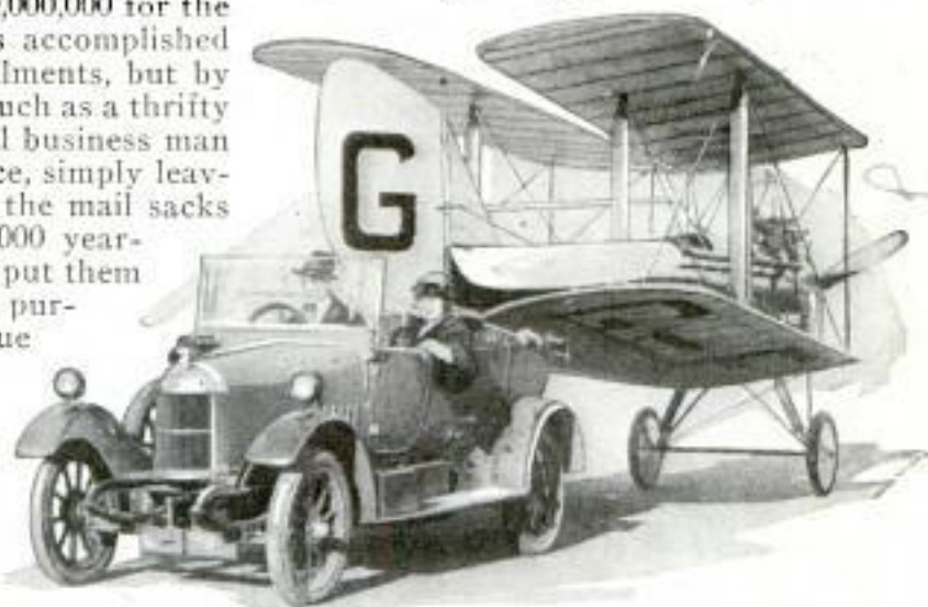
Courtesy De Havilland With Its Wings Folded at the Side, Tiny Two-Seater Airplane Is Easily Towed by Automobile
