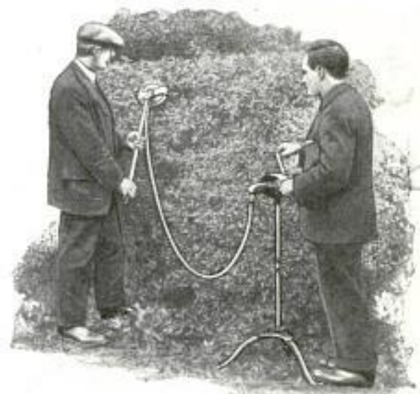
Trimming Hedge with Portable Clipper That Does Rapid Work and Reaches Difficult Places
