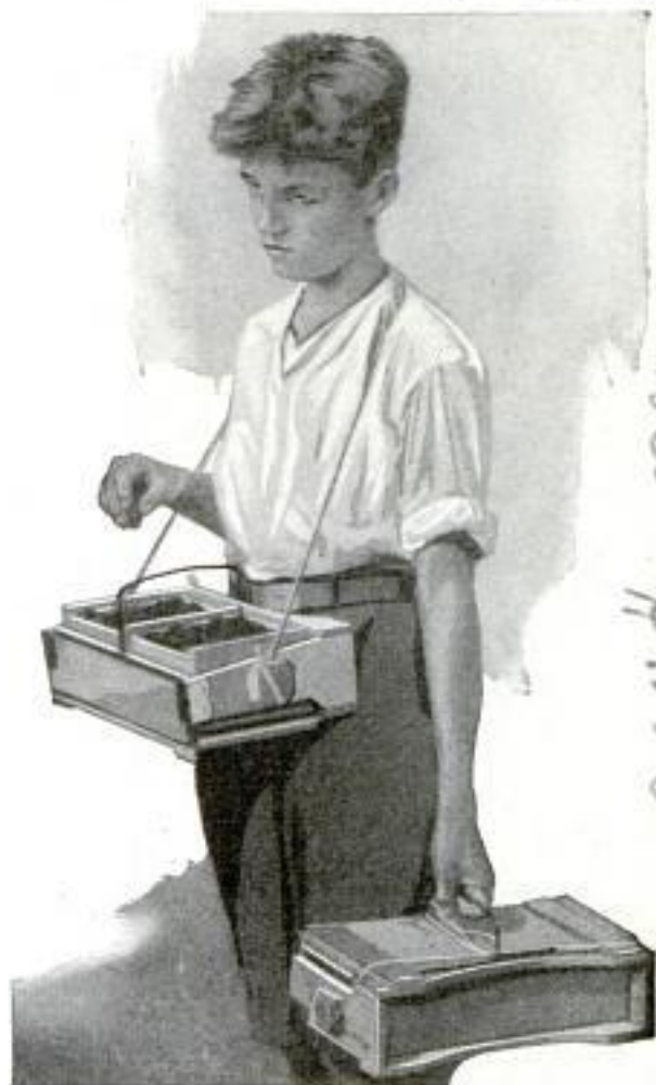
Berry Box Holder in Working Position and Turned Edgewise to Show Curve That Fits Body
