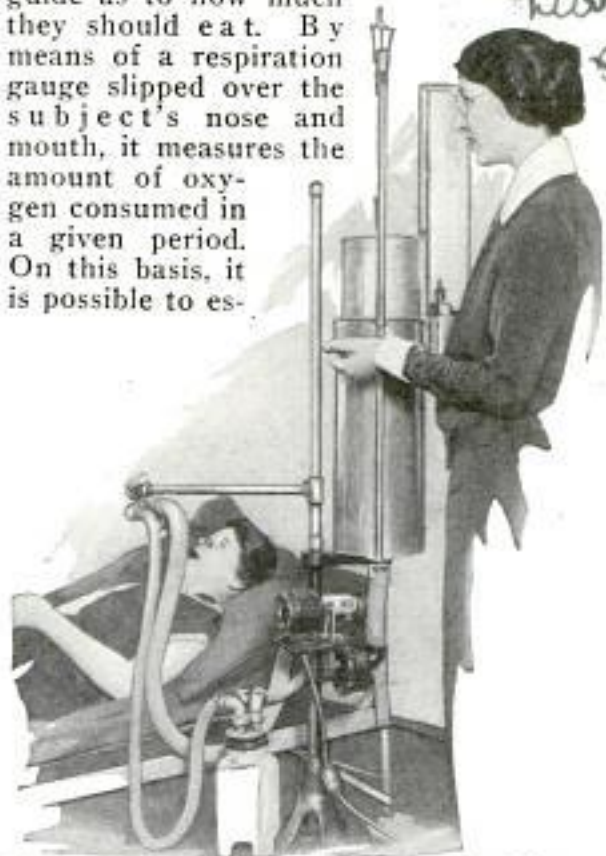
Measuring Oxygen Used by Subject in Breathing, as Basis for Estimating Correct Diet
