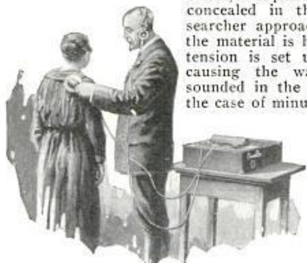
Searching for Concealed Metal Objects in Subject's Clothing with a Magnetic Finder
