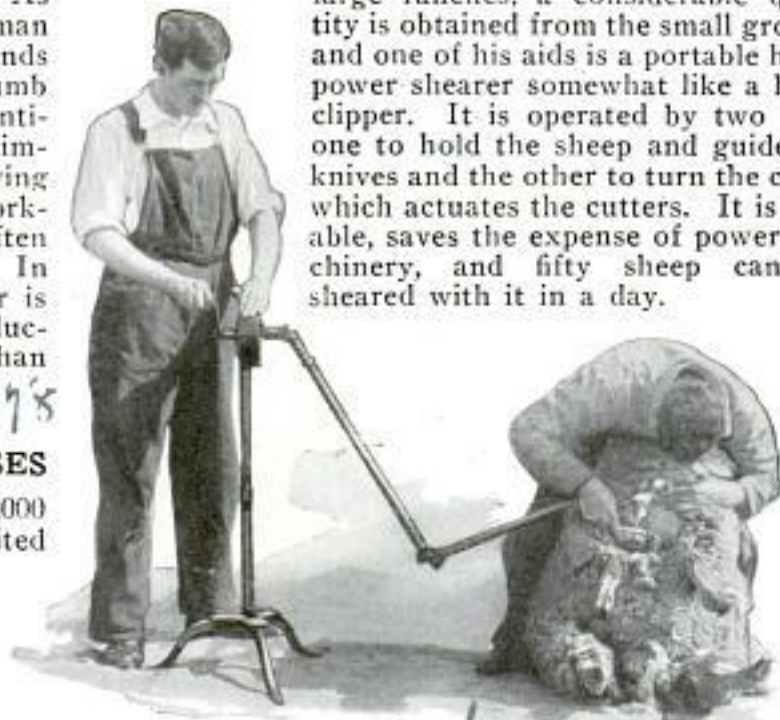
Shearing Sheep with Hand-Crank Clipper; Elbow Arm of Shaft Permits Free Movements and Whole Outfit Is Easily Carried
