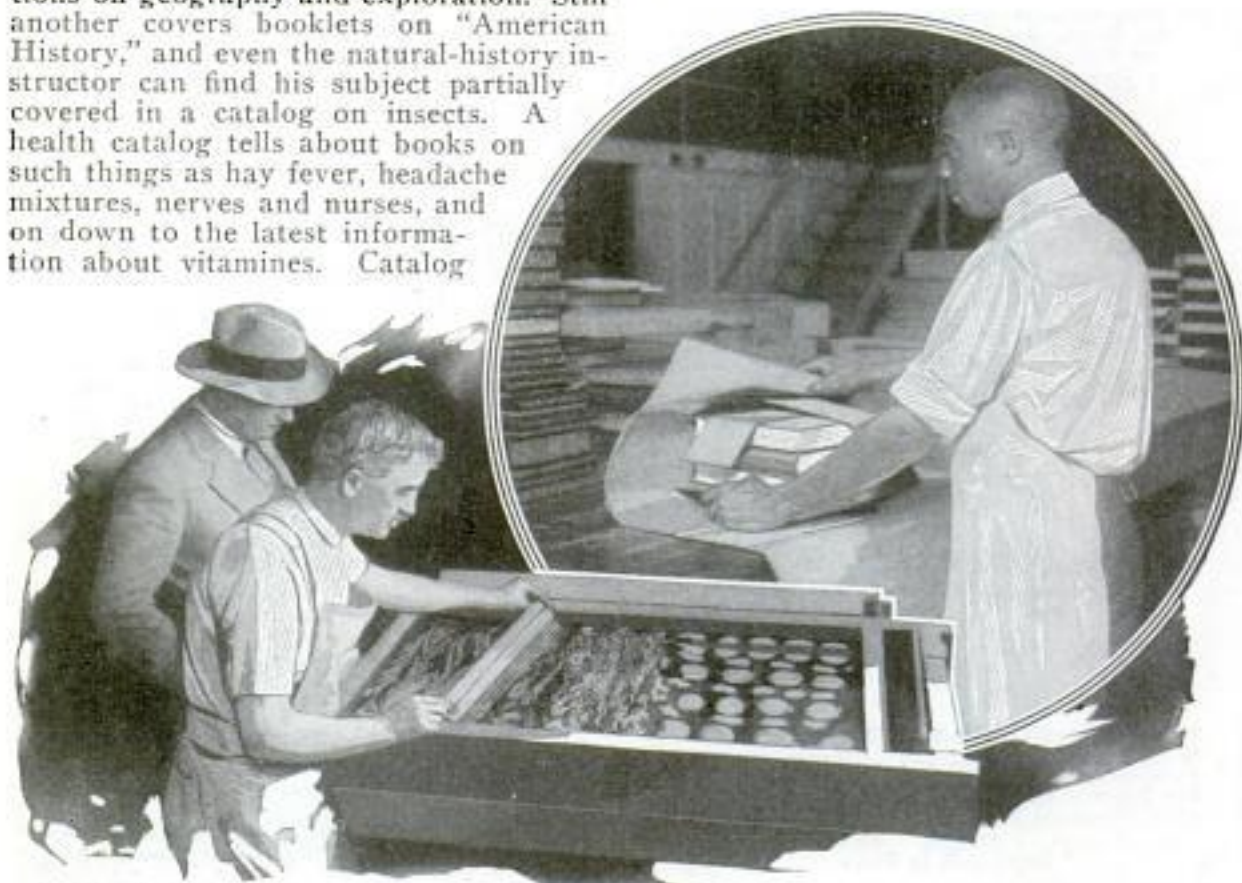
Book Marbler "Combing" a Tank of Floating Water Colors into an Intricate Design, and the Shipping Department Where Government Books Are Mailed to You
