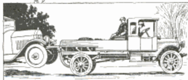
Convenient Towing Rig on Service Car Replaces Expensive Hoist and Can Be Made by Anyone
