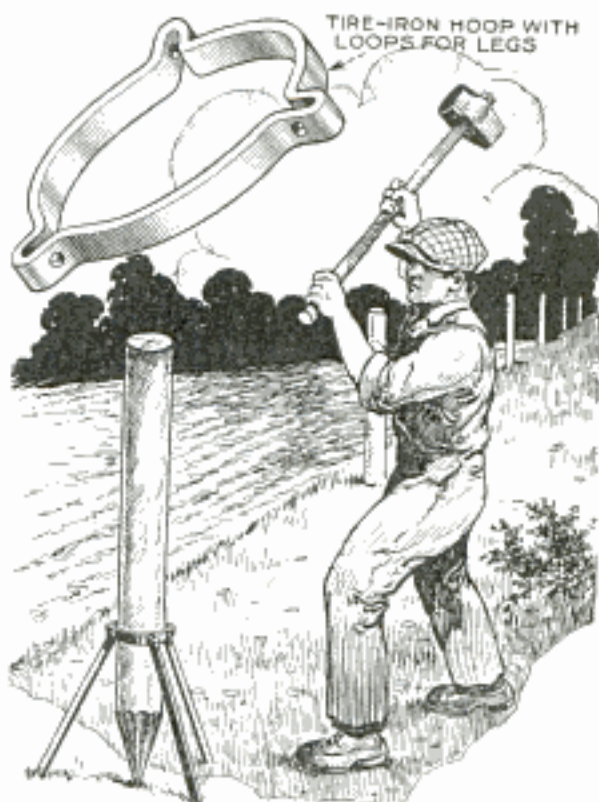
Tripod Holder for Fence Posts Enables One Man to Drive Them In
