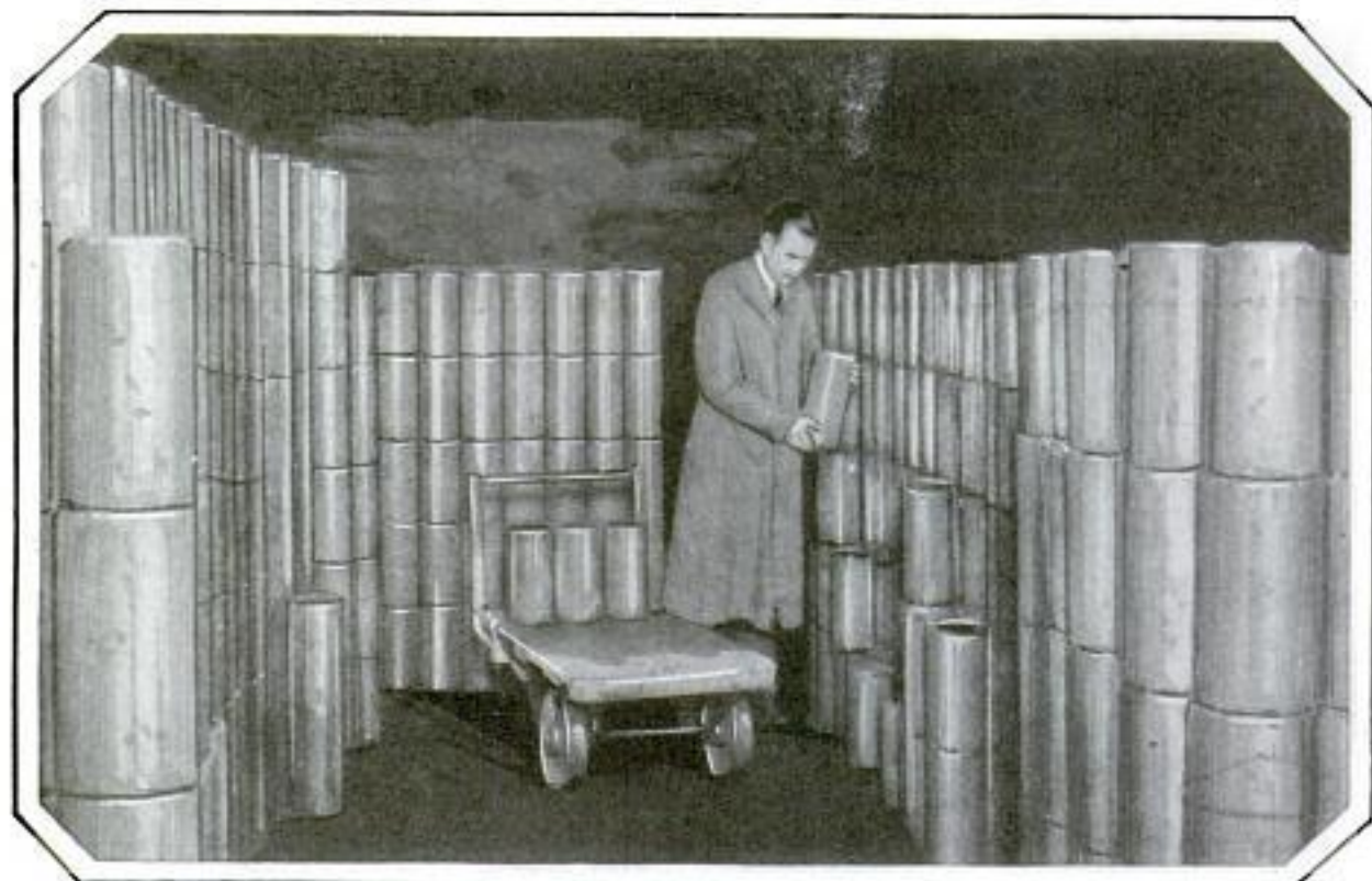
Cylinders of Cement Are Filled with Water and Stacked Away; After Hours of Soaking, They Are Carefully Examined to See How Much Moisture Has Leaked Through
