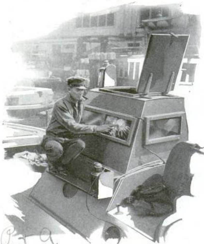
Pointing to Window on Rum-Runner's Pilot House That Cracked but Did Not Break When Bullet Struck It
