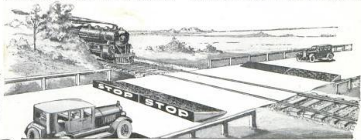
Sketch of Proposed Crossing-Guard Stops in Operation; Weight of Approaching Train Has Raised Barricades from Road Level; When It Passes, They Will Resume Normal Position
