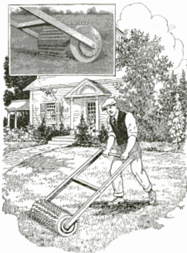
Simple Spiked Roller for Pruning Old Lawns Improves Their Appearance
