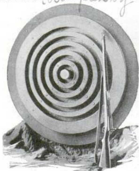
Bullets Striking the Steel Rings of This Target, Cause Them to Register Hits on Electric Indicator
