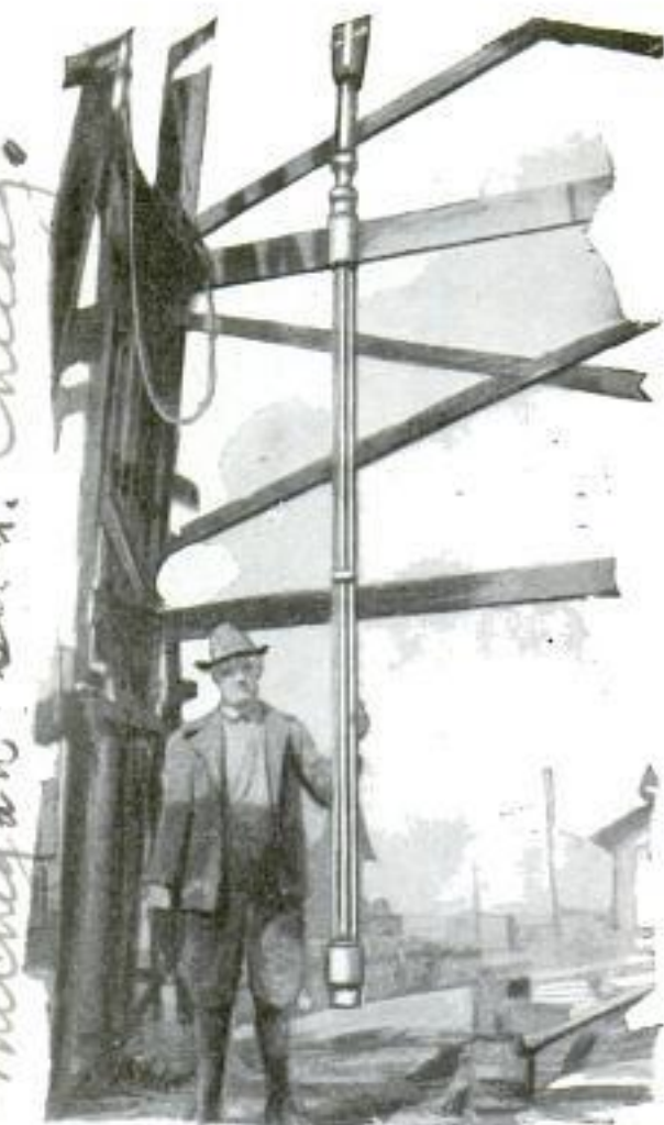
Electric-Heater Rod Which Is Lowered into Oil Well to Melt Accumulated Wax
