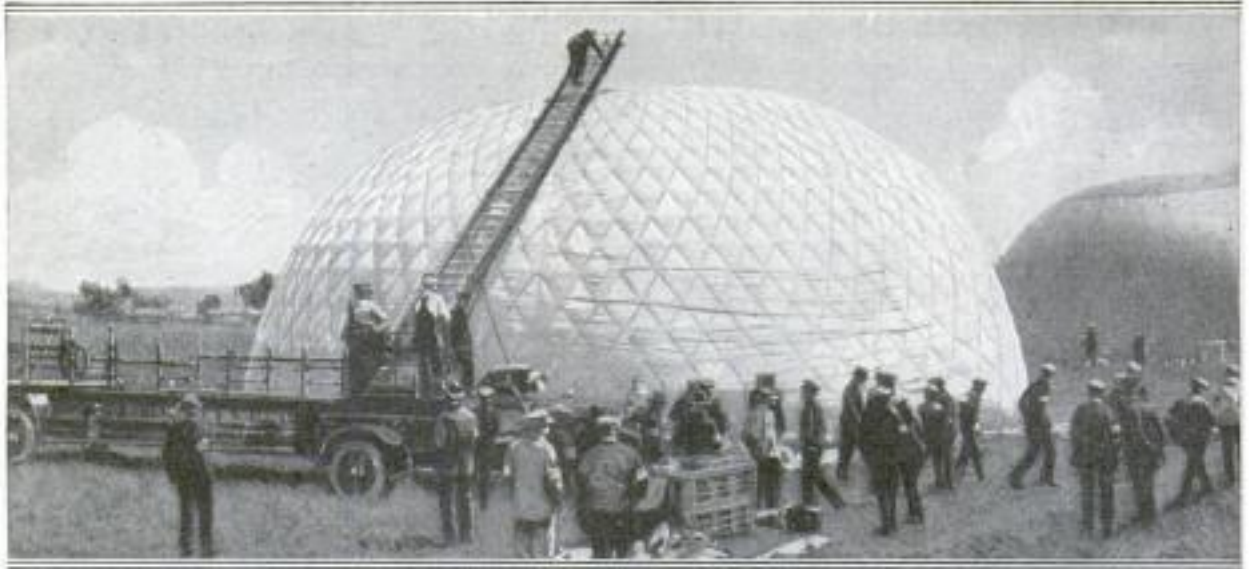
Using a Fire-Truck Ladder to Reach the Top of the Half-Filled Balloon "Detroit," to Repair Broken Netting before Start of National Race
