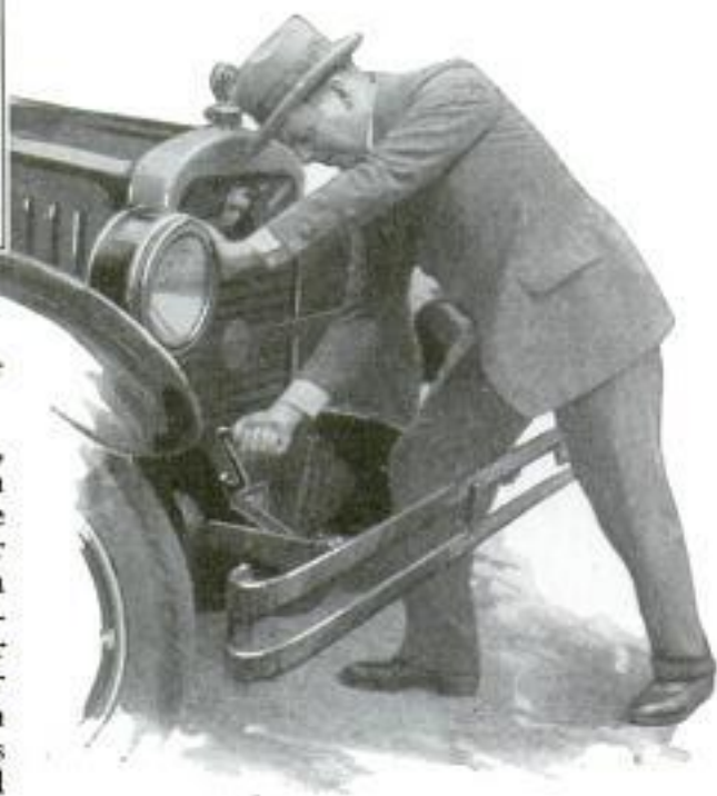
Above, Filling the Battery; Below, Turning the Motor Over with the Crank before Starting
