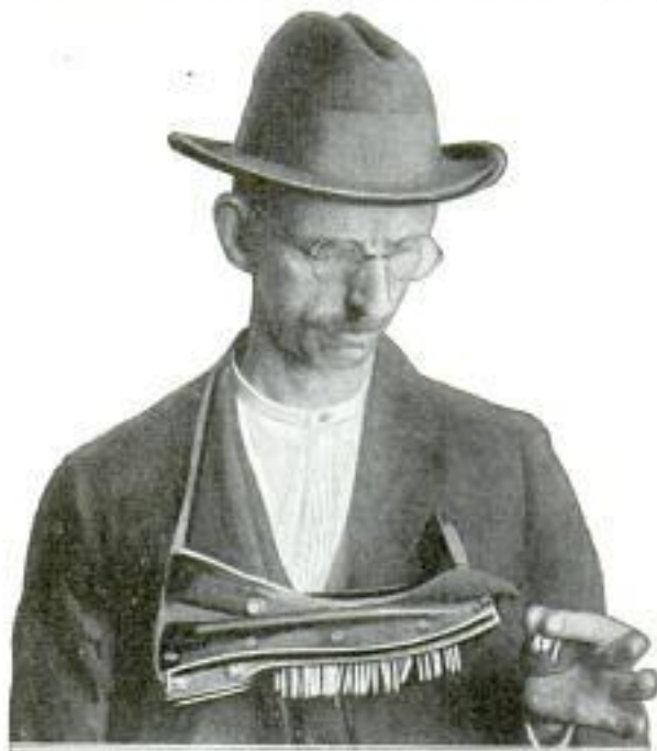
Picking Nails from Handy Sorter Worn by Neck Strap in Convenient Position
