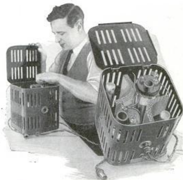
The Pull-Apart Plug on the Front of the Charger, and the Fahnestock Clips on the Rectifying-Jar Electrodes Are Non-Reversible
