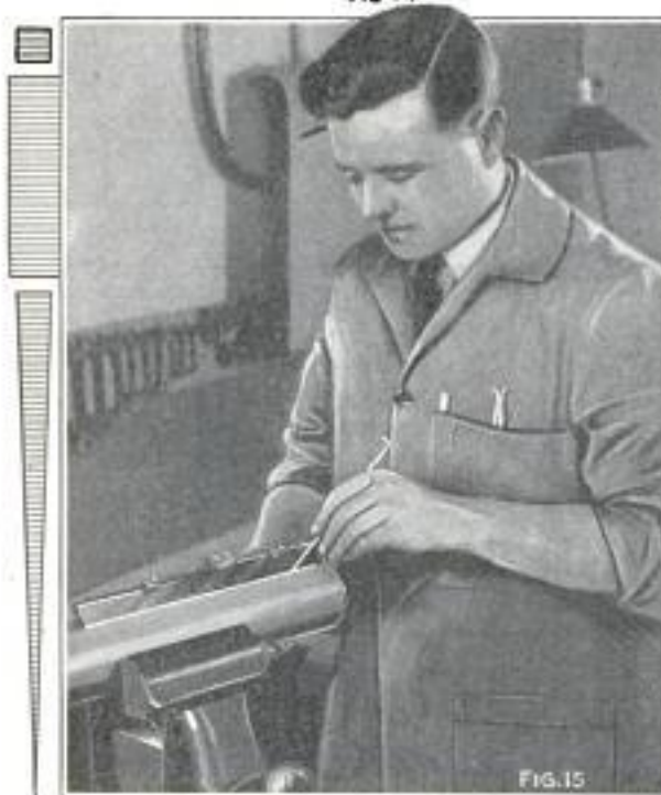
Fig. 14, Chipping a Broad Surface; Figs. 15 and 16, Laying Out and Cutting Keyseat on Shaft; Fig. 17, Holding Pulley for Keyseating and Fig. 18, Keyseat Square
