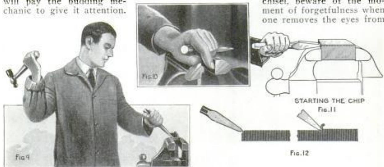
Left, End of Swing; Fig. 10, How the Chisel Is Grasped; Upper Right, Taking the Chip, and Lower Right, the Cape or Crosscut Chisel
