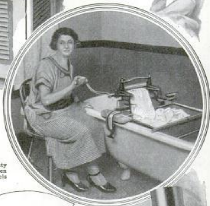
Clamps Fit the Clothes Wringer to the Bath-tub, Saving Stooping; Below, Tea Caddy That Shakes Out One Spoonful at a Time
