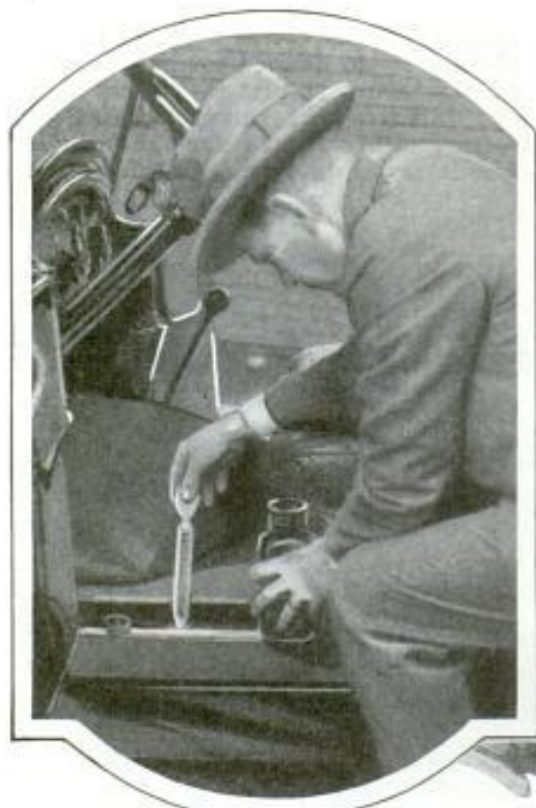
Above, Filling the Battery; Below, Turning the Motor Over with the Crank before Starting
