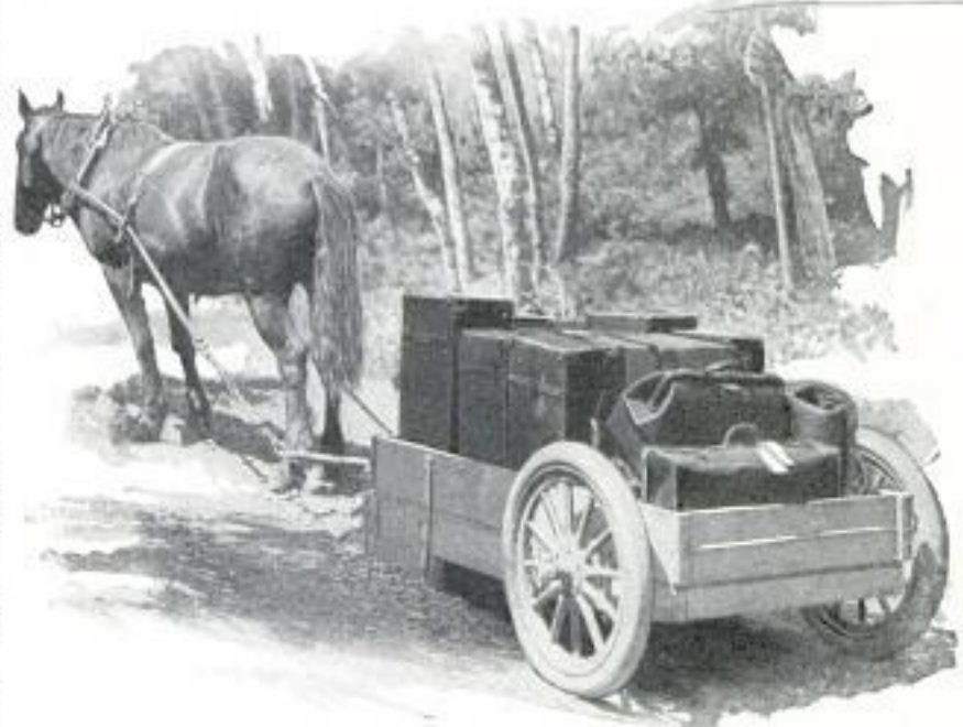
Baggage-Laden Cart Ready for Rough Paths; Runners Keep the Load to the Ground and Wheels Ease the Horse's Burden
