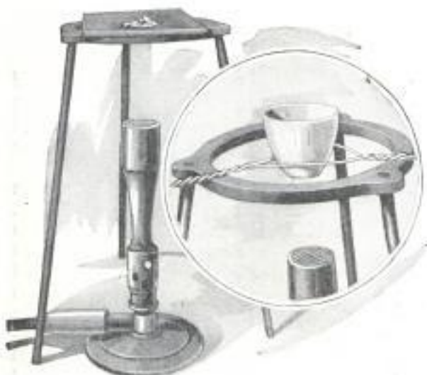
Methods of Melting Lead and Sulphur on Iron Plate and in Crucible for Making Synthetic Crystals
