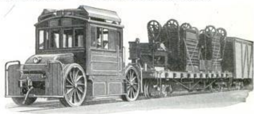
Rubber-Tired Electric Tractor Hauling Freight Train through City Street Barred to Steam Locomotives
