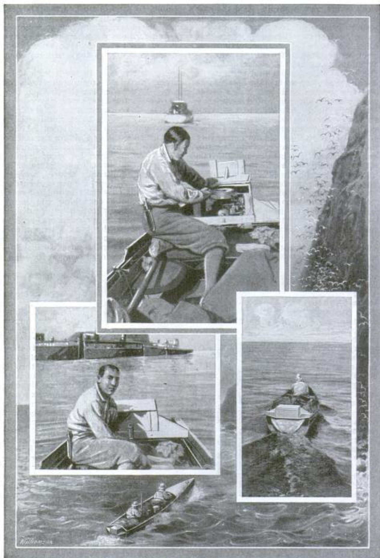
Above, the Motor Housing Is Opened to Start the Engine; the Housing Is Removed Merely by Releasing a Few Hooks; Left, Cruising with the Housing Closed, and Right, View over the Stern, Showing the Canvas "Petticoat"
