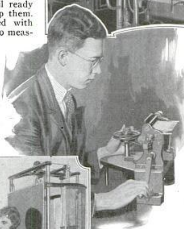
Machine for Cutting Tiny Radium-Filled Tubes Used in Internal Treatments
