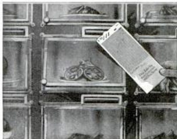
Food Compartments and Slotted Card That Is Stamped with Price as It Unlocks Them
