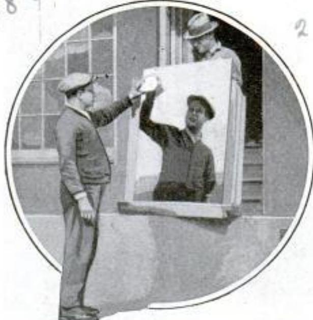
Polishing Metal Mirror before Shipment; Reflection of Workman Seen as Clearly as in Glass
