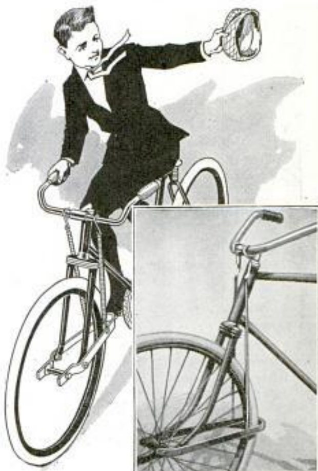
Extra Fork and Springs on Bicycle Reduce Vibration of Handlebar and Make Riding More Comfortable
