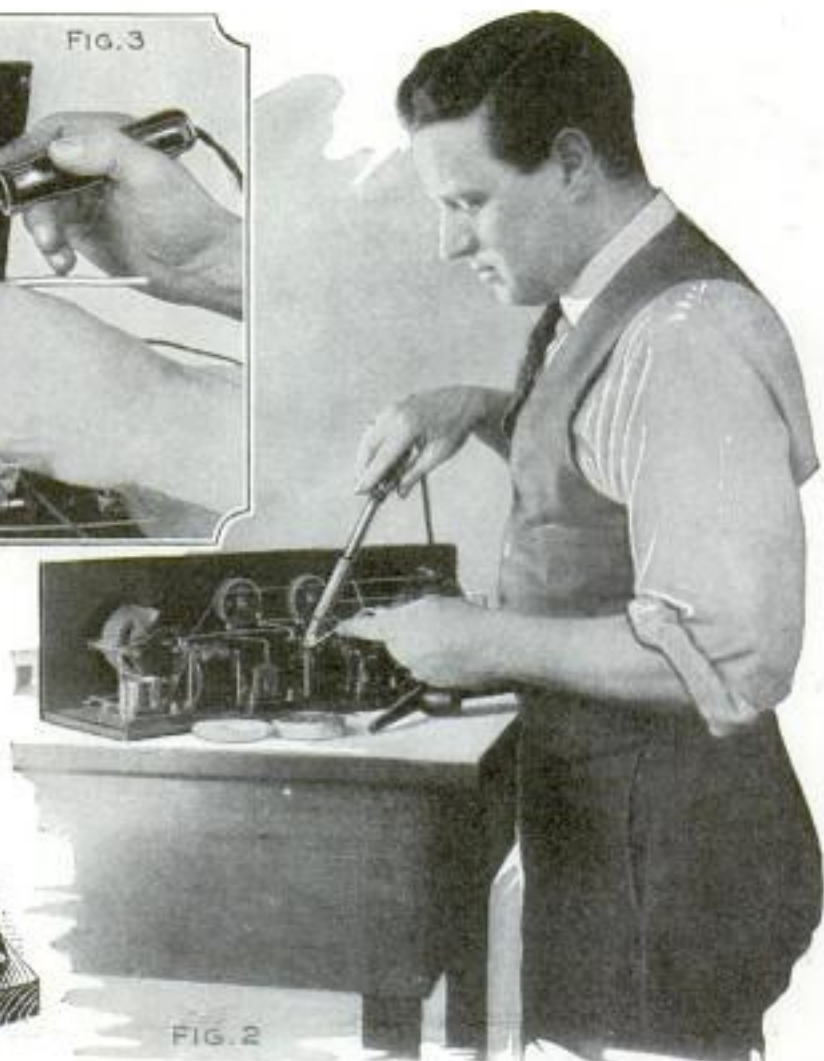
Two Types of Electric Soldering Iron, Showing How Each Is Used; Below, Method of Heating Plain Iron, and Simple Stand
