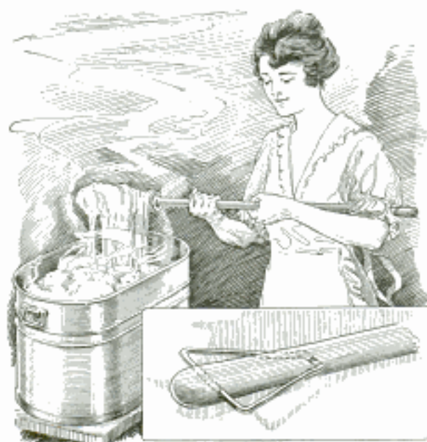
Wire Attachment on End of Stick Facilitates Removing Clothes from Boiler
