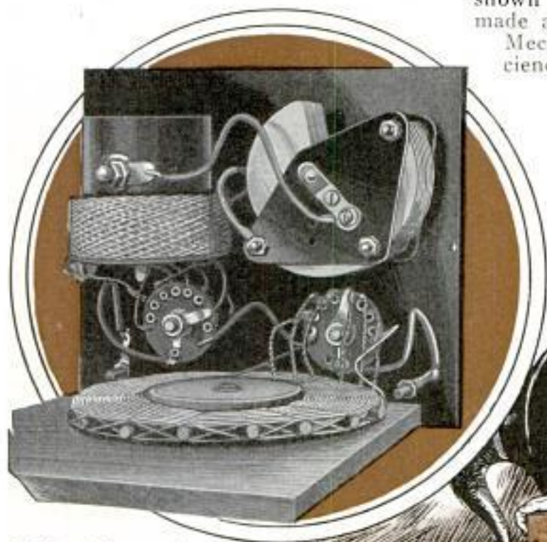
A Wave Trap of Merit, Which Adds to the Enjoyment of a Small Tube Receiving Set as It Eliminates Undesired Signals of Near-By Stations
