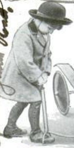
© Henry Miller When His Car Is Out of "Fuel," This Young Driver Charges the Compressed-Air Tank with a Foot Pump and Drives On
