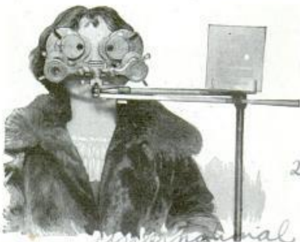
2574 Vision-Tester Employed to Determine Fitness of Auto Drivers to Operate Cars
