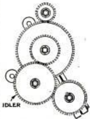
COMPOUND GEARING ON LATHE: WITH INTERMEDIATE OR IDLER GEAR
