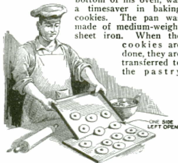
Three-Sided Pan Aids Baker in Transferring Cookies from Oven to Pastry Board
