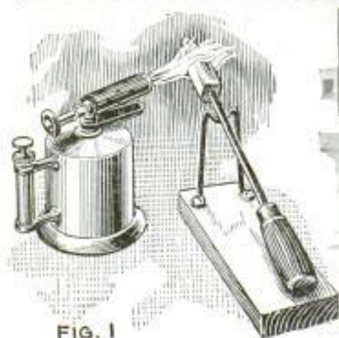
Two Types of Electric Soldering Iron, Showing How Each Is Used; Below, Method of Heating Plain Iron, and Simple Stand
