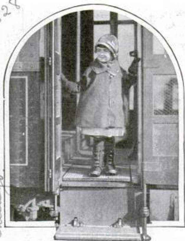
Street-Car Safety Exit Which Is Automatically Opened by Passenger's Weight as Car Stops
