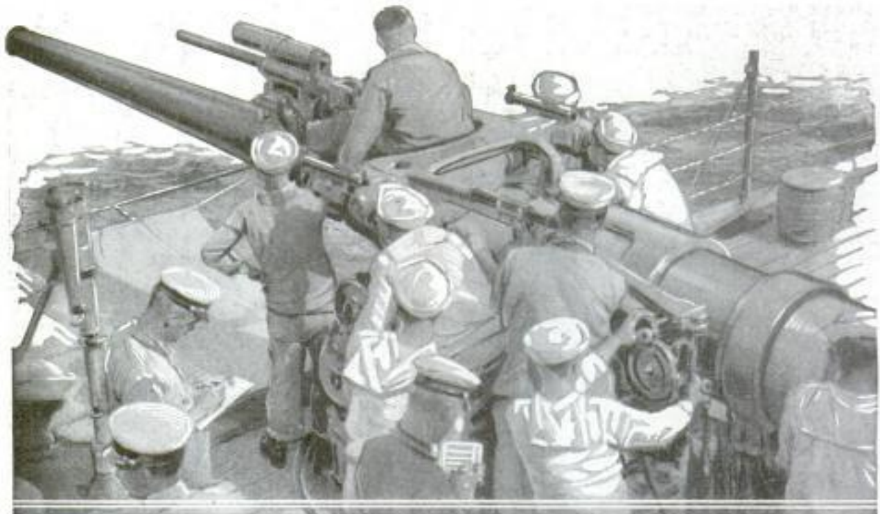
Gunner Sitting Astraddle the Big-Gun Barrel Loads the One-Pound Gun Which Is Pointed by Aiming the Five-Inch Rifle on Which It Is Mounted
