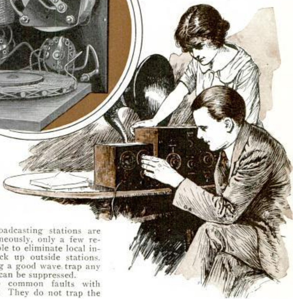
A Wave Trap of Merit, Which Adds to the Enjoyment of a Small Tube Receiving Set as It Eliminates Undesired Signals of Near-By Stations
