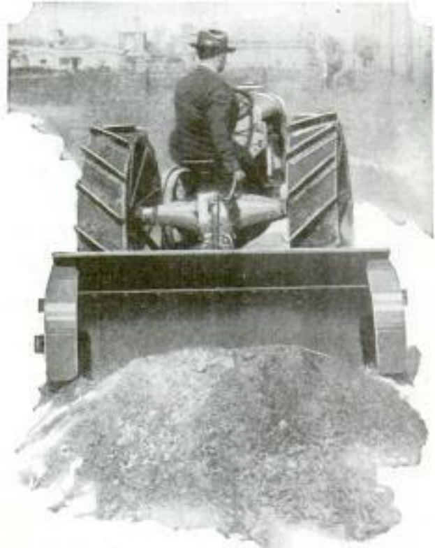
Rear View of Tractor Scraper, Showing How Control Is Managed from Driver's Seat
