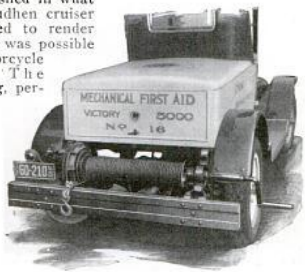
Rear of First-Aid Truck with Windlass, Tow Rope and Tool Box in Body
