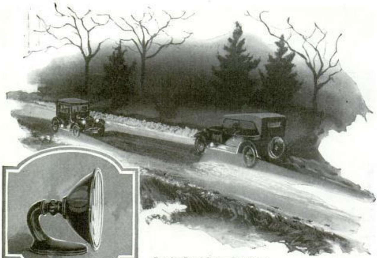
Running-Board Lamps Installed, a Headlight on Right and the Left One Casting Glow to Rear; Inset Gives Close View of Lamp
