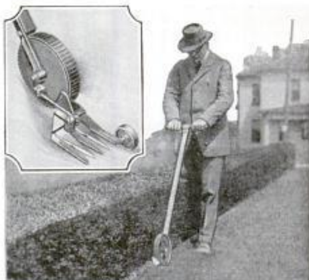
Trimmer in Operation Showing Clean Edge It Leaves; Close View in Inset
