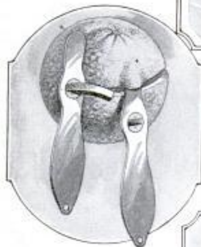
Peeling an Orange or Similar Fruit without Breaking It and Losing Juice Can Be Done with This Cutter, Shown in Position for Grooving the Skin and for Prying It Off
