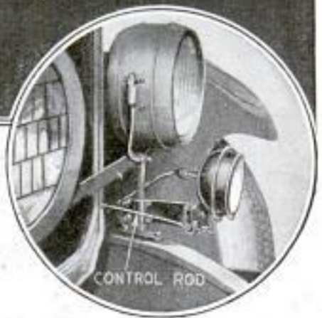
Spotlight Worked from Steering Post of Auto, Casting Rays to Avoid Blinding Oncoming Driver; Left, Construction of Control Lever on Post, and Right, How Light Is Placed at Front of Car
