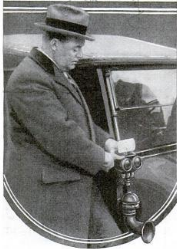
Automatic Horn and Lights That Tell When Car Exceeds the Lawful Speed Rate
