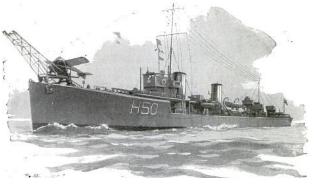
Experimenting with Pilotless Aircraft: When Catapult Is Released, the Plane, with Motor Running, Shoots Sharply Upward; from Then On, Radio from the Boat Is Its Unseen Guide
