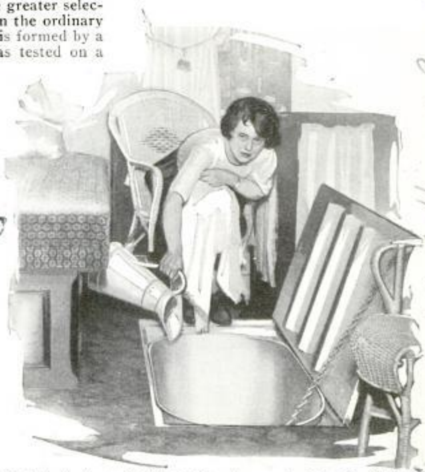
Ready for Service at the End of a Dusty Journey, the Motor-Bus Bathtub Is Concealed in the Floor
