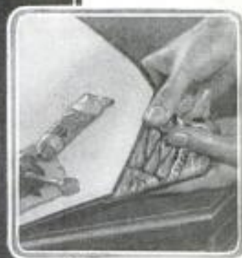
When the Glue Has Set Until It Is Partly Dry, the Ribbon Is Pressed Down into Place with the Fingers; the Selvage of the Ribbon Eliminates the Need of Folding
