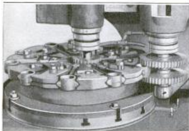
The Work Is Mounted on the Table and Both Ends Are Faced at Once
