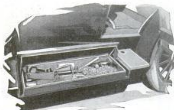
Automobile Tool Box Installed under Step Which Locks with Closing of Car Door
