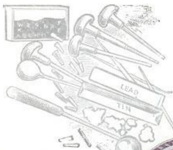
Punches, Ladle and Metal Used by Hunter in Making Type
