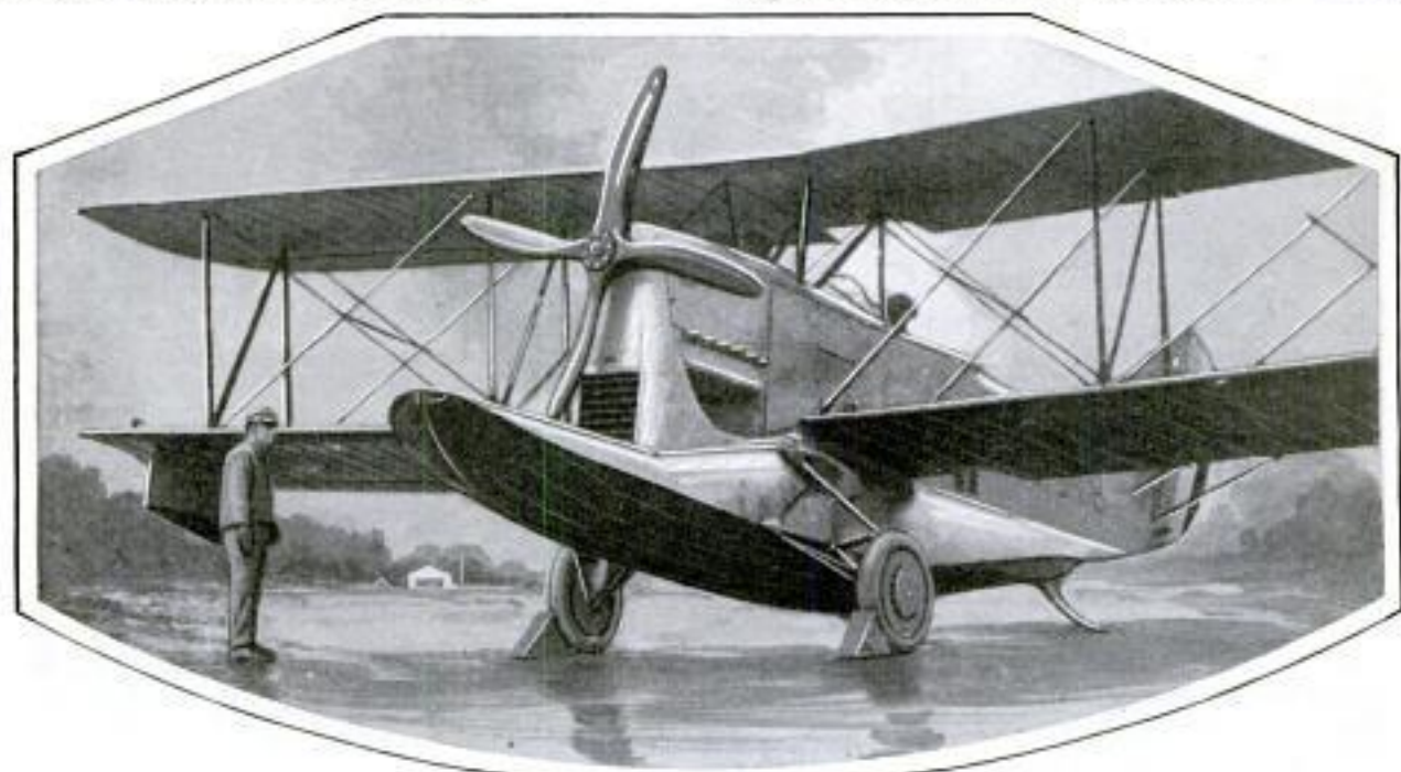
Metal Seaplane with Wheels Attached to Boatlike Hull, for Use in Ground Landings, Which Carries a Crew of Three and Fuel for a 700-Mile Non-Stop Flight
