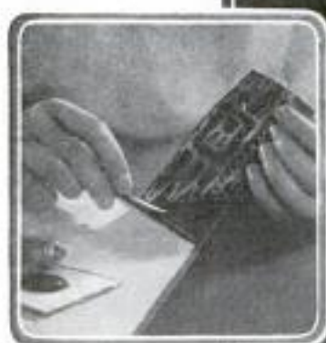
The Glue Is Spread over the Surface of the Desk-Pad Corners, and Allowed to Set Until It Is "Tacky," or Almost Dry; the Ribbon Is Held Firmly as Shown
