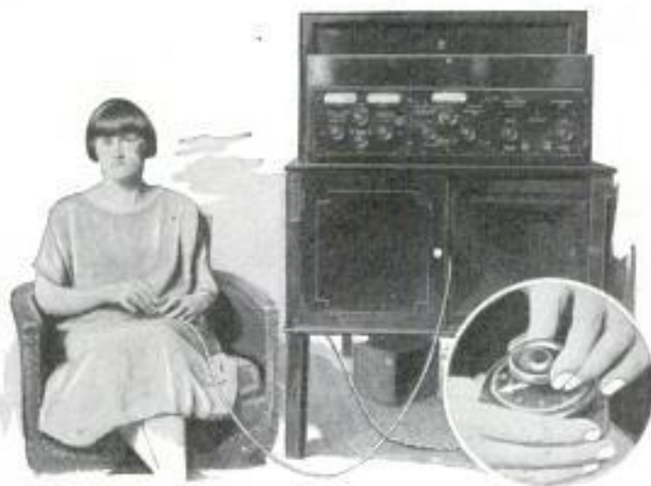
Remote Control Permits Adjustments from Any Part of Room; Insert, Control Unit
