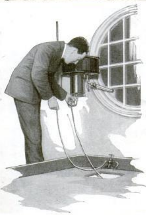
Fog Gauge in Operation, Air from Outdoors Being Drawn In Through Window Tube
