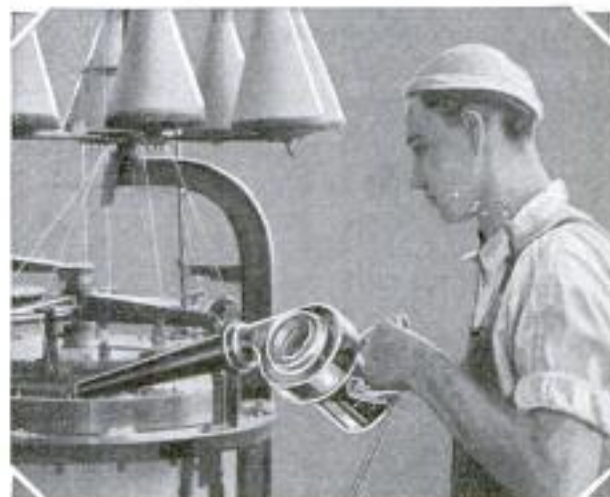
Removing Waste and Dangerous Dust from Spinning Machine with Portable Electric Blower
