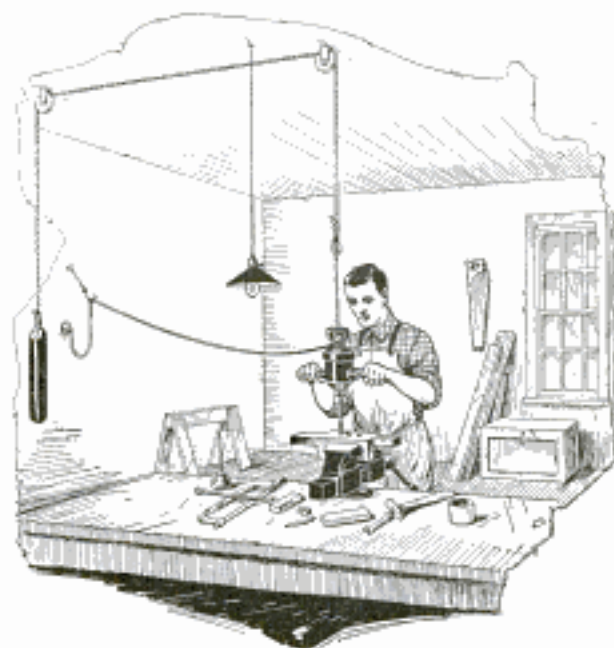
Counterweight for Electric Hand Drill Facilitates Handling It
