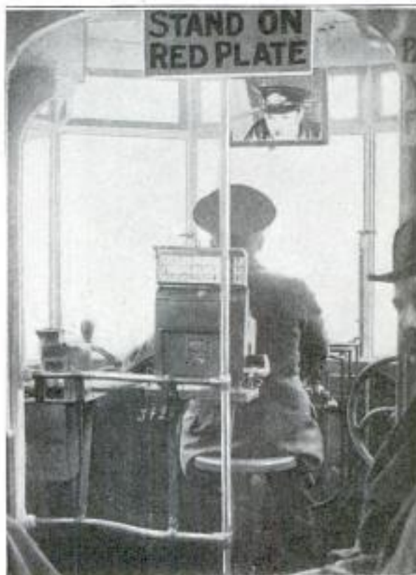
Front of One-Man Street Car with Mirror above the Motorman's Head
