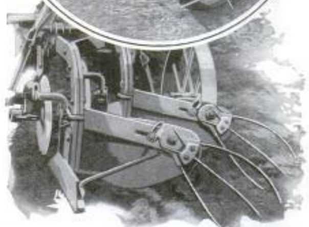
Three-Fingered Knives as They Are Attached at the Rear of the Plowshare
