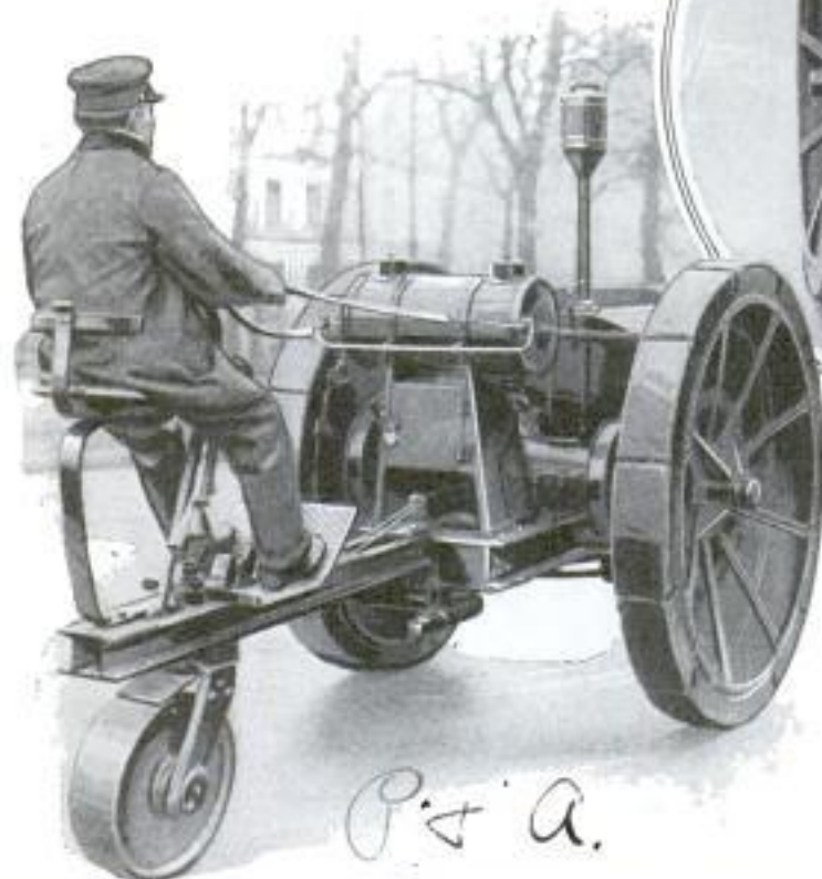
Front and Rear Views of Tricycle Tractor, Showing Reins by Which Driving Wheels Are Regulated
