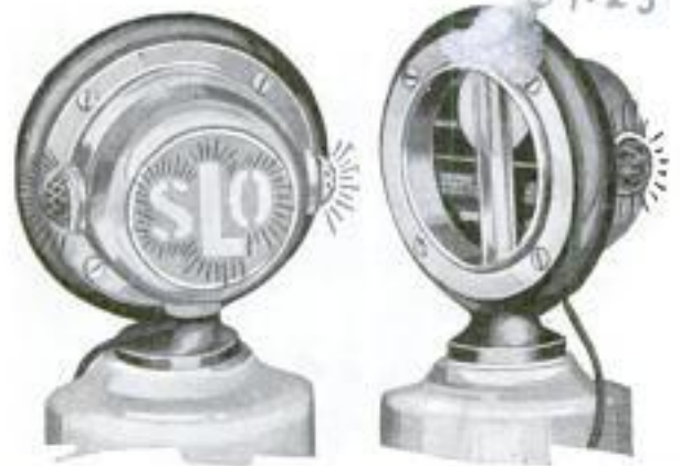
Front Light with Side Signals as Seen by Approaching Motorist and from Driver's Seat
