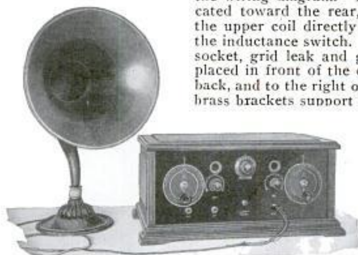
View of Front of Finished Two-Step Cockaday Receiver, Showing Arrangement of Panel
