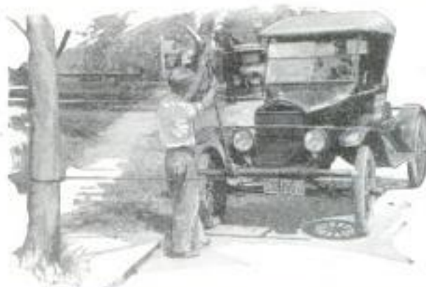
How Combination Auto Bumper and Winch Can Be Utilized to Relieve a Stalled Car
