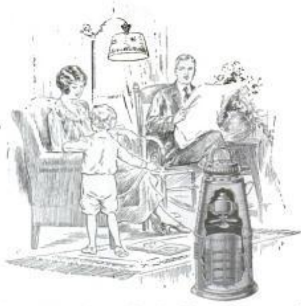
Cross-Section Diagram Showing Heating Elements and Fan That Keeps Air in Circulation
