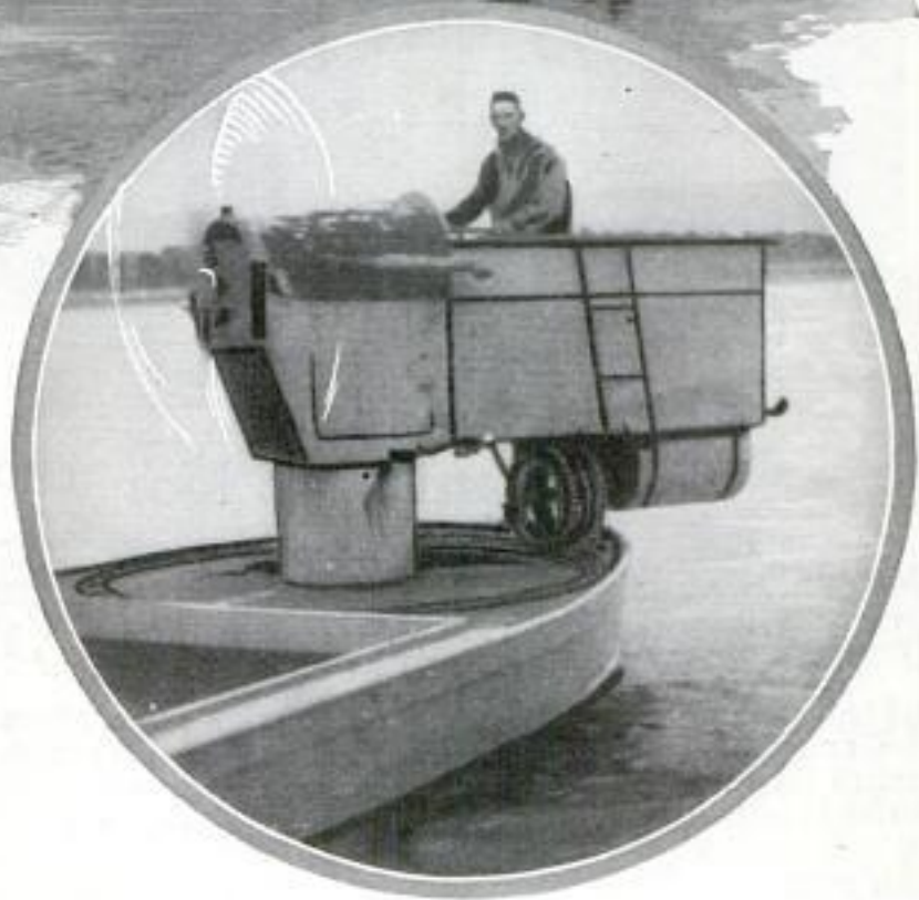
Harnessed to Barge, Airship Motor Speeds Craft Upstream and Pilot Steers by Turning Fuselage and Propeller on Revolving Carriage
