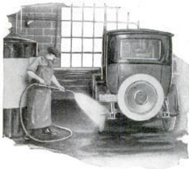
Through Long Hose and Nozzle, Spray from Pressure Tank Reaches All Parts of Car
