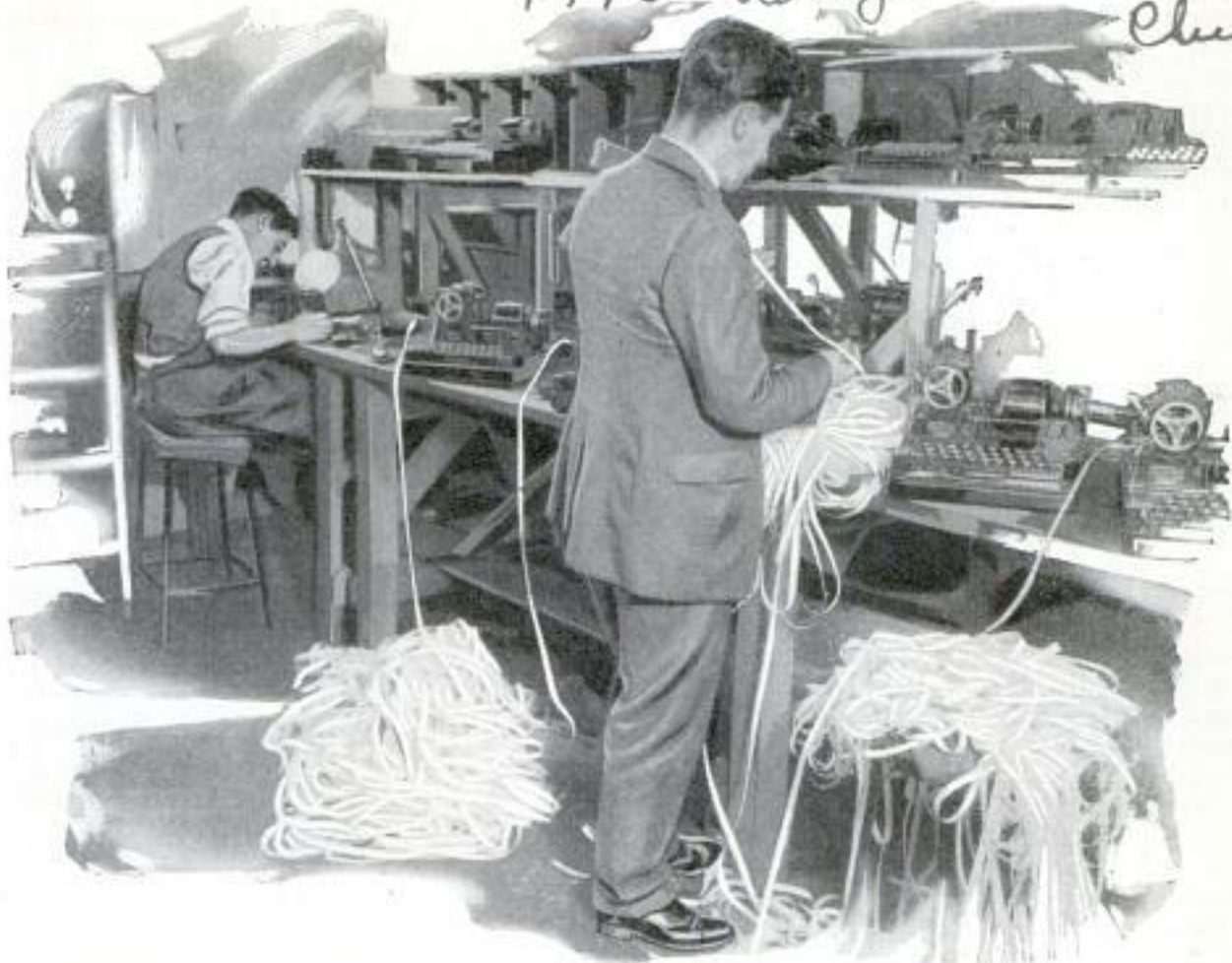
Testing Teletype Printers, with the Entire Battery Writing a Sample Sentence Sent Over and Over Again All Day Long from One Sending Machine
