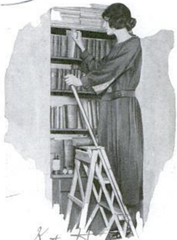
Keeping Balance on High Ladder Is Easy with Handrail Securely Fixed in Sockets
