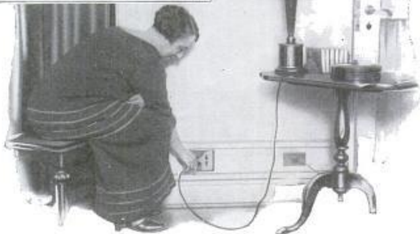
Battery of Radio Sets on Upper Floor; Programs Are Received in Apartments by Connecting the Loud Speaker to a Wall Socket
