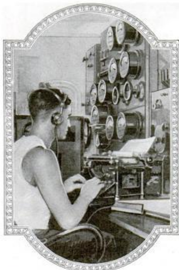
Radio and Depth-Finder Equipment of the U. S. S. "Hannibal," Used in Sounding the Ocean
