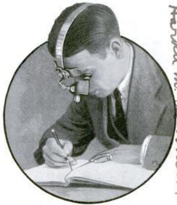
Telescope Magnifier Attached to Head Clip, for Use by Weak-Sighted Person in Reading
