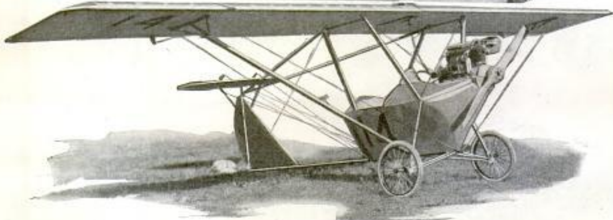
Sidecar and Motorcycle Engine as They Appeared Transformed into Speedy Monoplane That Flew Twenty-Five Miles on Half Gallon of Gasoline, and Start of 150-Mile Flight
