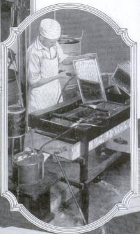
Left, Honey Tanks and Extractors, Turned Out in Large Quantities by Factories, Make Bottled Honey Possible; Below, a Steam-Heated Knife, Connected by Tubing to Boiler on the Stove, Slices Beeswax Caps off Honey Frames Before They Go into the Revolving Extractor
