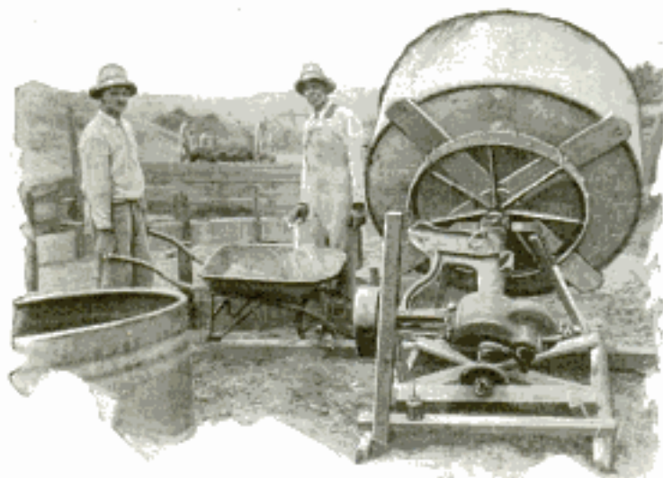
Novel Concrete Mixer Made from Mower and Circular Water Tank
