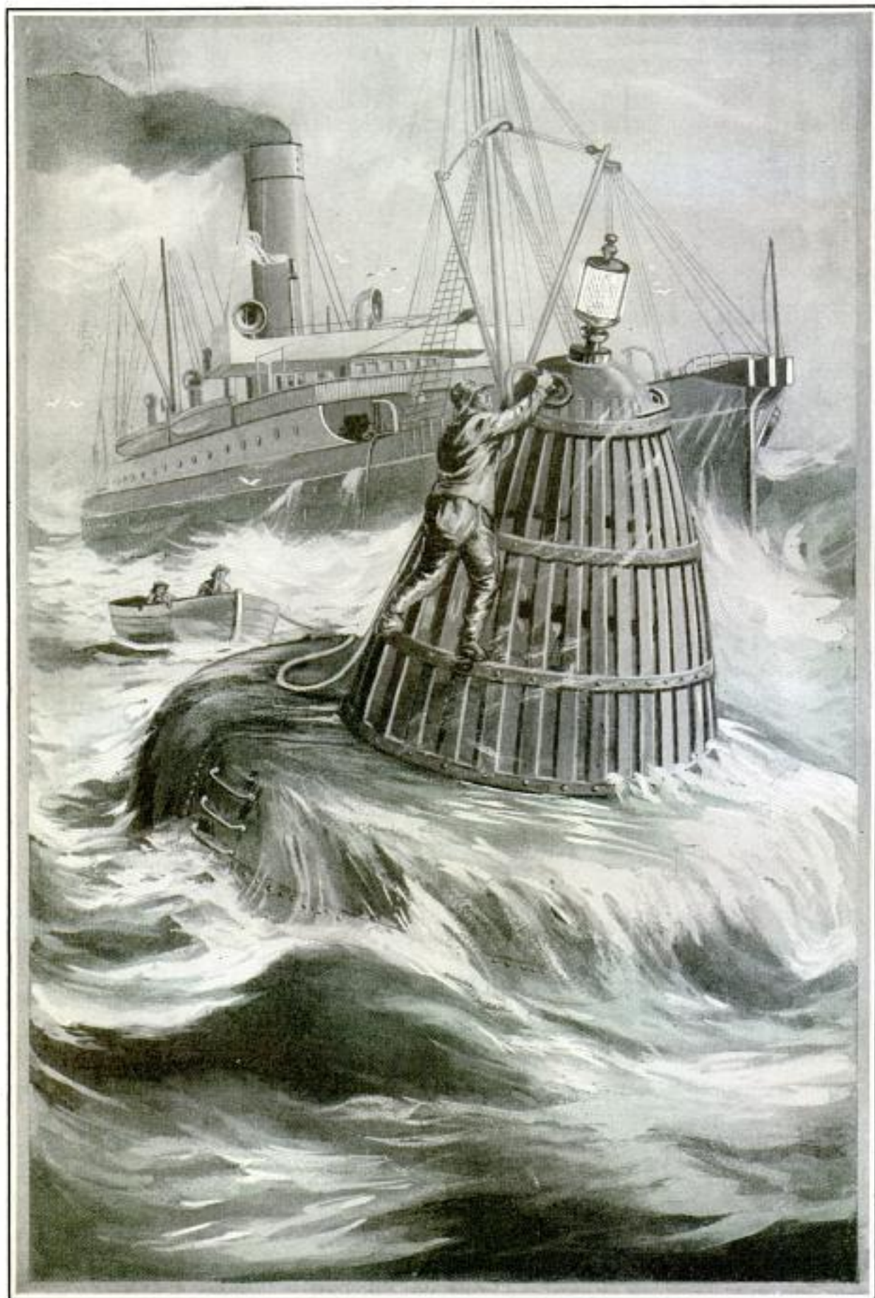
Loading the Gas and Air Chambers of a Light and Whistle Buoy That Operates for Three Months on Single Charges from a Tender Ship Which Carries Generating Plants
