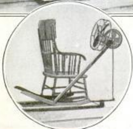
Fan That Operates by Power Provided by Motion of Rocking-Chair
