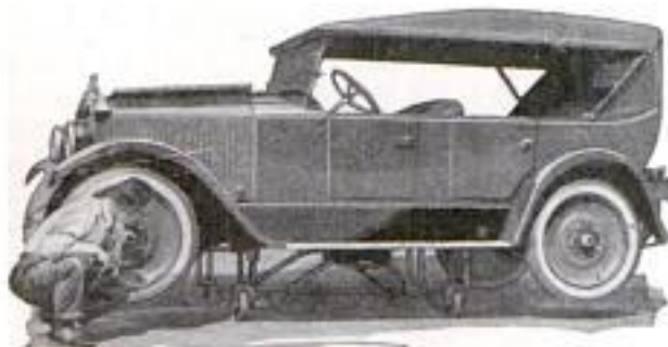
Automobile Raised by Rolling Hoist Attachment Which Allows Car to Be Moved Sideways
