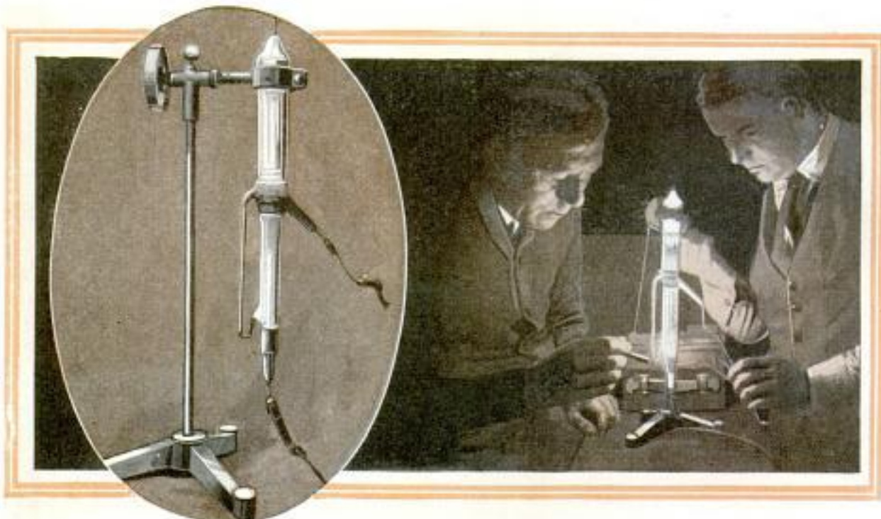
Testing the Return Speed of the Condensed Mercury Passing through the Siphon Tube to the Boiling Level; Insert, Close-Up of a Desk-Type Lamp and Bracket
