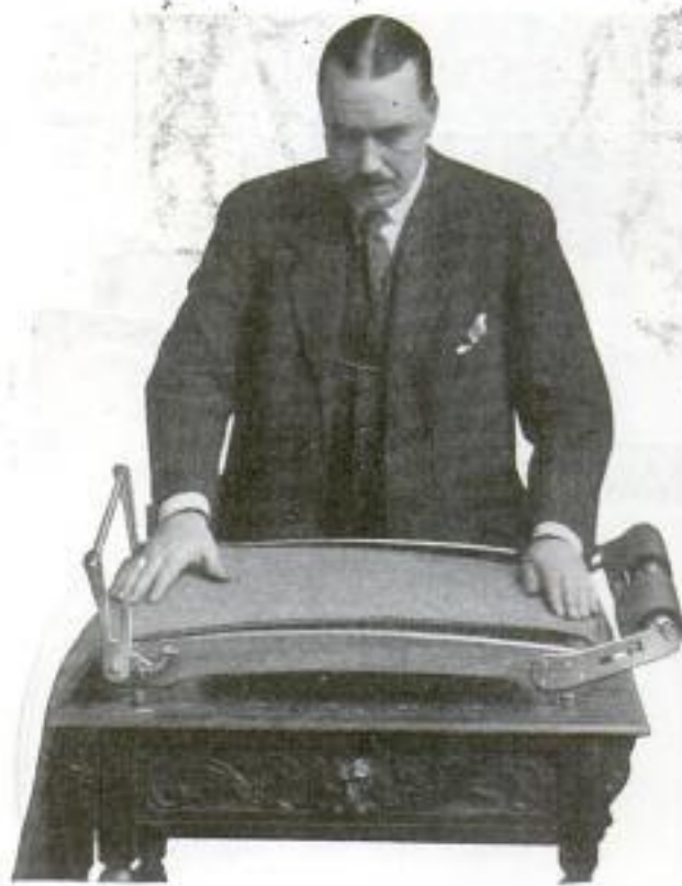
Smoothing Trousers Before Webbing Strips at Right Are Clamped across to Other Side
