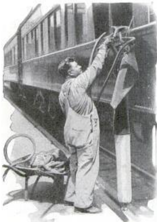
In Almost Any Coach Yard, the Car Cleaner with His Vacuum Outfit and Dust-Trap Bag, That Catches the Dirt Removed by Powerful Suction, Is a Familiar Sight
