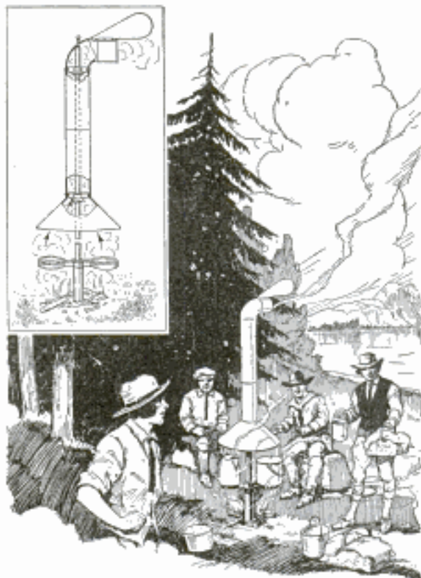
Outdoor Fireplace Eliminates Annoyance from Smoke and Provides Grate over the Fire
