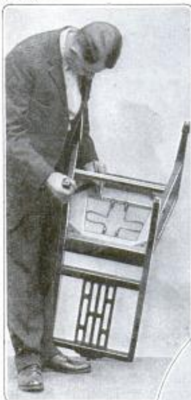
Spring Brace under Chair Seat for Rais- ing Sunken Bottom
