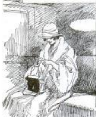
Handy Matchbox Holder for the Autoist; It Is Attached to the Steering Column at a Convenient Height
