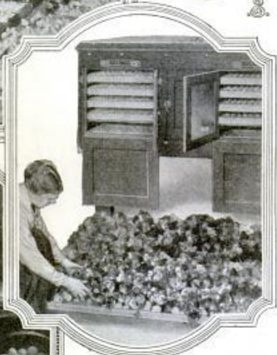
Transferring the Baby Chickens from an Electric "Hen" That Holds 2,400 Eggs; Youngsters Can Be Removed without Disturbing Other Hatches
