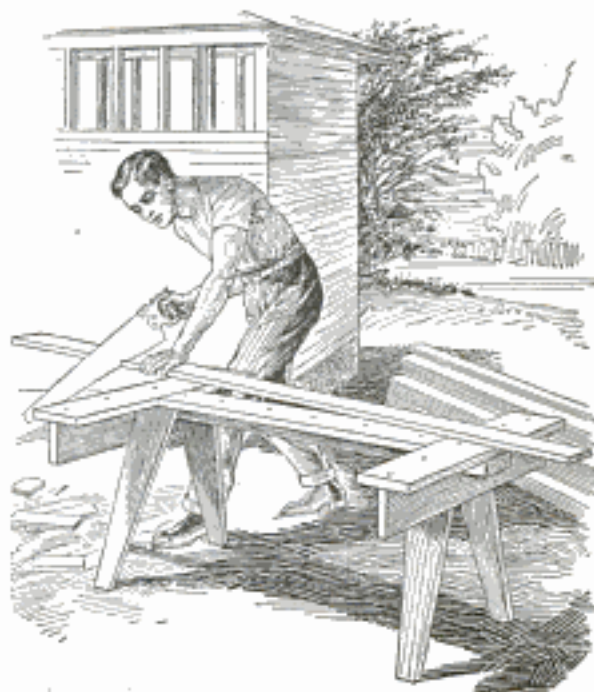
Crosspieces Make Single Sawhorse Give Service of Two
