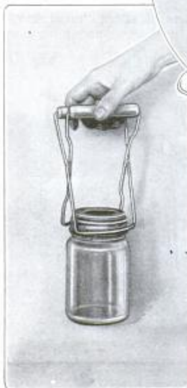
Grip for Lifting Fruit Jars Saves Burning Fingers and Will Not Slip
