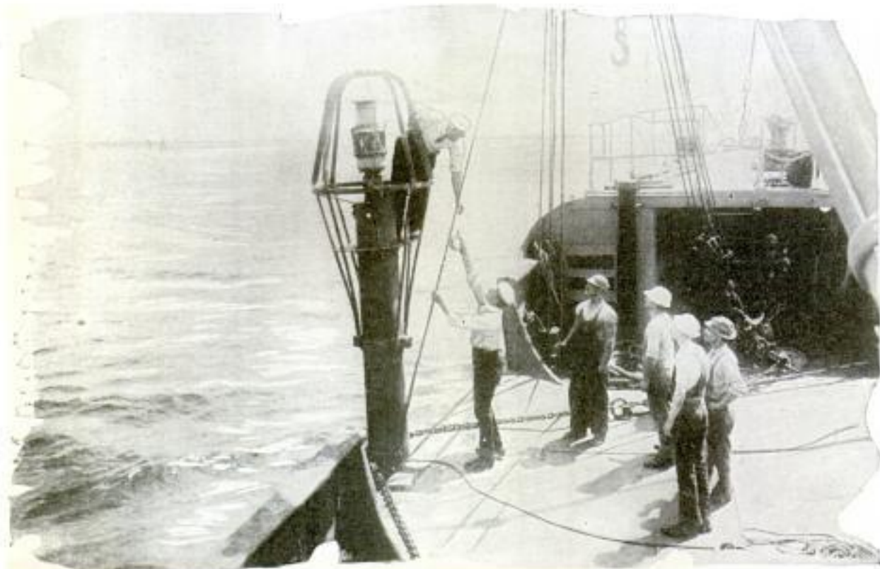
How Gas Buoys Are "Captured" and Moored to a Vessel by the Attending Crew, Who Test the Supply of Fuel with a Gauge They Apply to the Valve of the Lamp's Reservoirs
