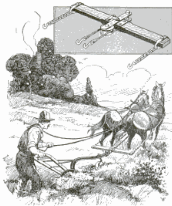
Two-Horse Evener Which Requires About Half as Much Space as the Ordinary Evener
