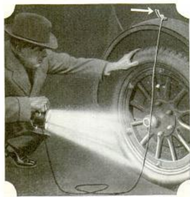
Inspecting Automobile with Fender Light That Can Be Carried to Any Part of Machine
