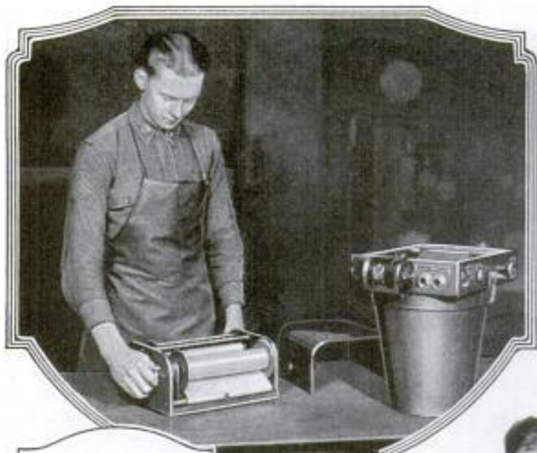
Films Fifty, Seventy-Five or One Hundred Feet in Length Are Placed in the Aerial Cameras and the End Threaded onto the Motor-Driven Winding Spool; the Motor Which Turns the Film as the Pictures Are Automatically Taken Is Shown at the Left Corner of the Camera
