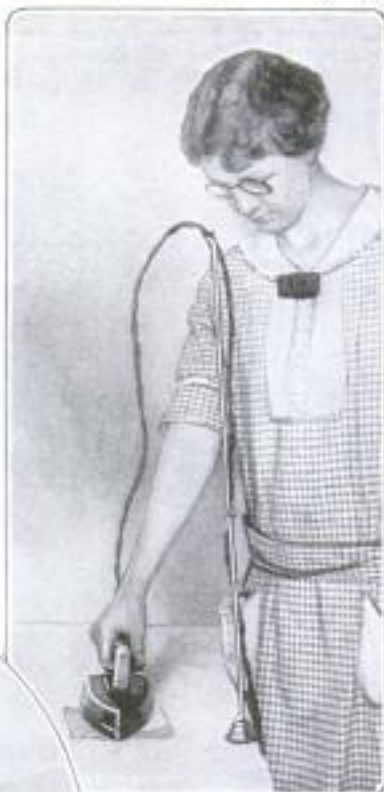
Electric-Iron Cord Carrier Prevents Kinks and Twists
