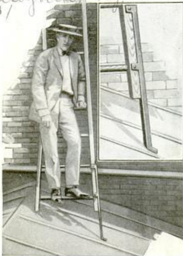
How Extension Ladder Works on Sloping Roof, and Close View of Attachment
