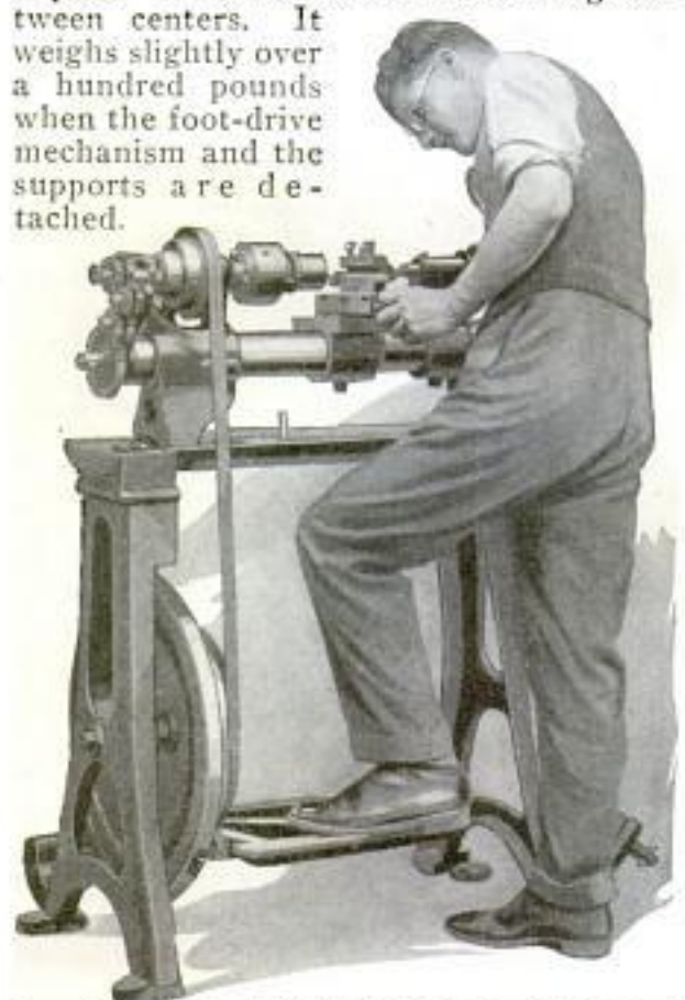
Foot-Power Lathe with Cylindrical Bed in Which Lead Screw Runs and Is Protected
