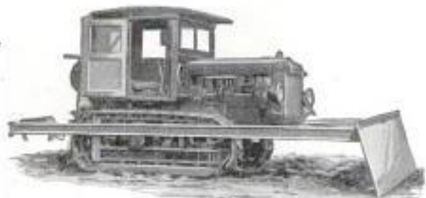
Tractor with Dirt-Pushing Attachment in Place, Ready to Batter Down Piles of Rubbish
