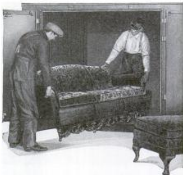
Removing Large Divan from Vault Where It Has Been Fumigated for Twelve Hours
