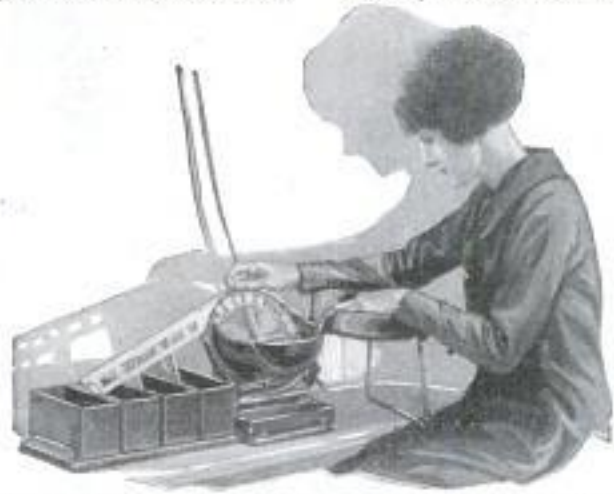
Coins Passing down Slotted Trough and Falling into Proper Compartments from Hopper and Disk
