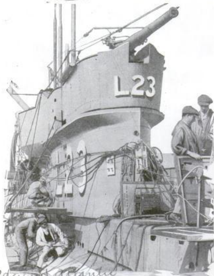
Product Atlantic Rifle Turret of Submarine Shaped to Protect Gunners from Wash of the Sea When Craft Is Traveling Partly Submerged
