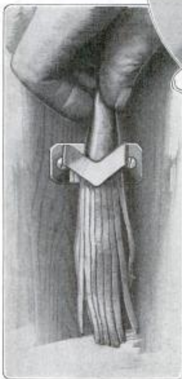
Slicer Cuts Beans and Other Vegetables into Narrow Strips
