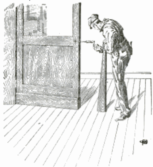
Support for Brace Aids in Drilling Holes in Doors
