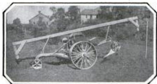
Automatic Tractor Plow in Action, Showing Reversing Beam and Suspended Share near Fence
