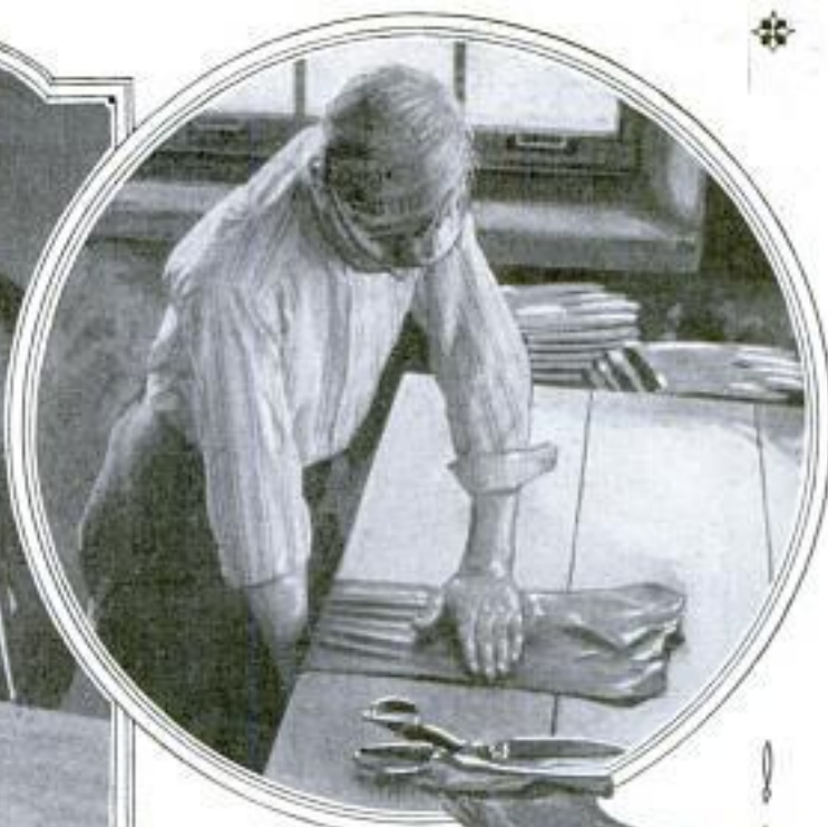
Stretching and Working Leather to Make Grain Even and Reveal Unde- sirable Blemishes
