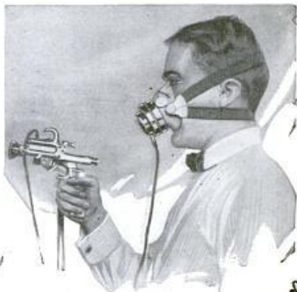
Painter Demonstrating a Lead-Poisoning Preventive the Air-Filter Mask Connected to Spray Gun
