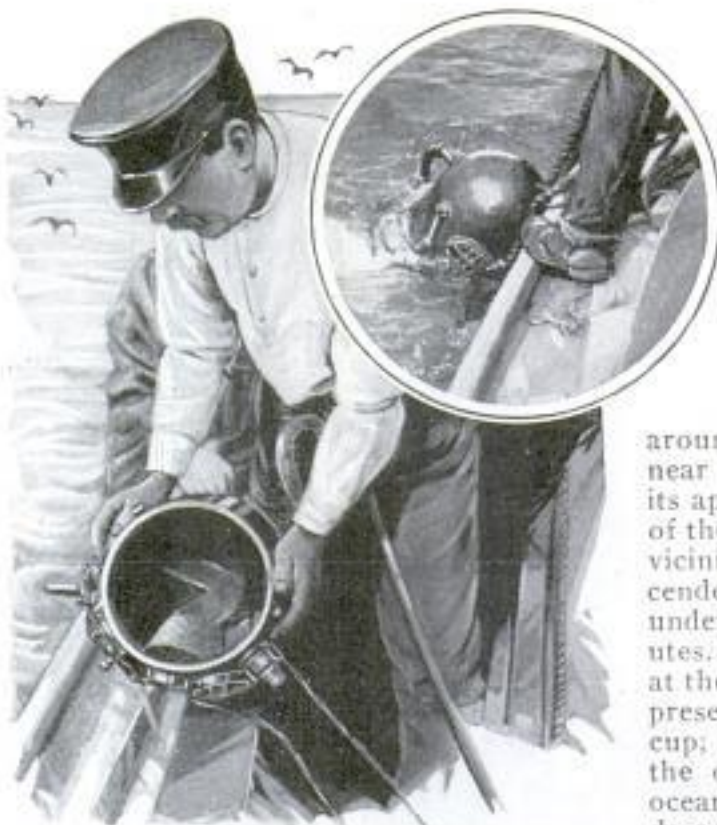
The Microphone inside the Helmet, Protected by Sponges; Insert, "Coming Up"
