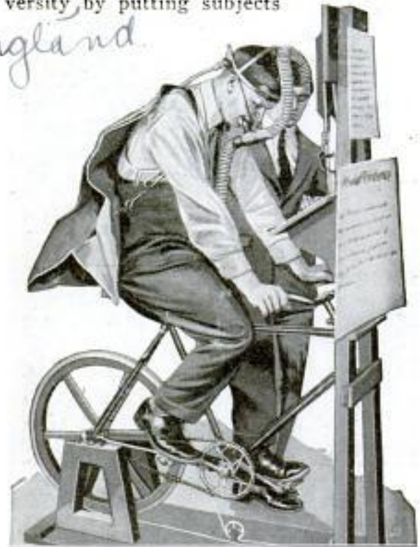
Rider Taking Bicycle Test for Muscular Efficiency; Breath Is Exhaled into Mask Device
