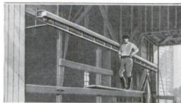
Sections of Conveyor Track Cut and Hinged on End to Permit Passage of Loaded Rack
