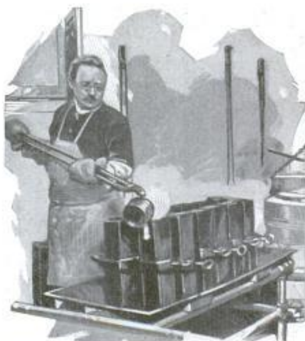
Casting Large Ingots of Gold in Molds for Storage in the Treasury Vaults
