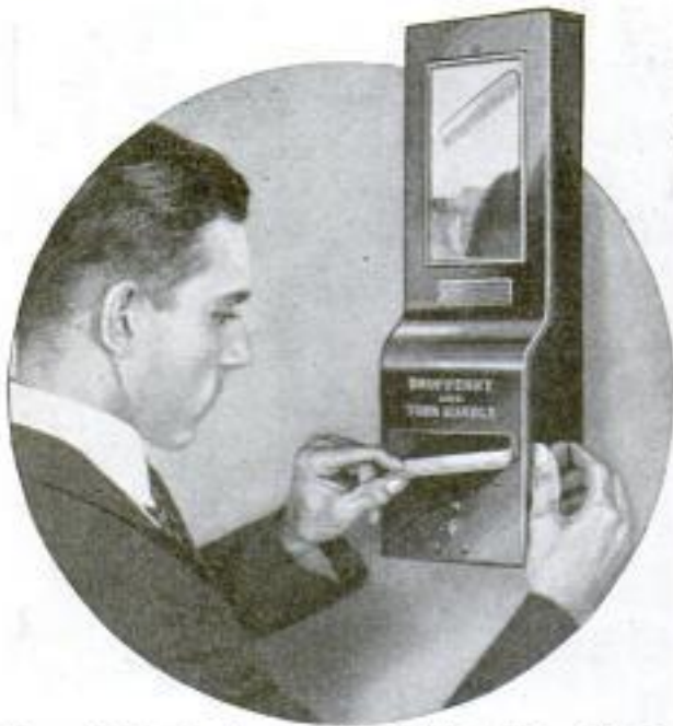
Penny-in-Slot Vending Machine Which Delivers Comb When Penny Is Dropped in Opening
