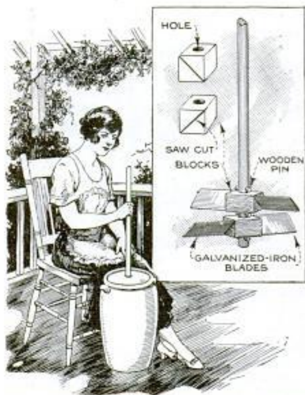
Churn Plunger with Two Revolving Blades Lightens Task of Butter Making
