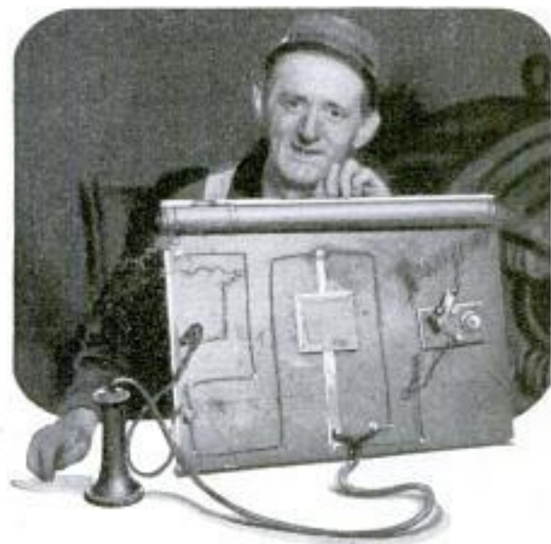
Receiving Set Built at Cost of Thirty Cents and Using Ordinary Telephone Receiver
