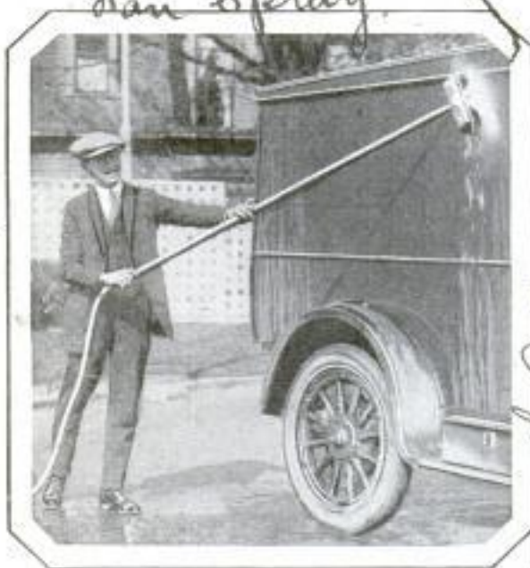
Brush Holder and Spray Which Gets Water Supply through Hollow Handle Attached to Garden Hose
