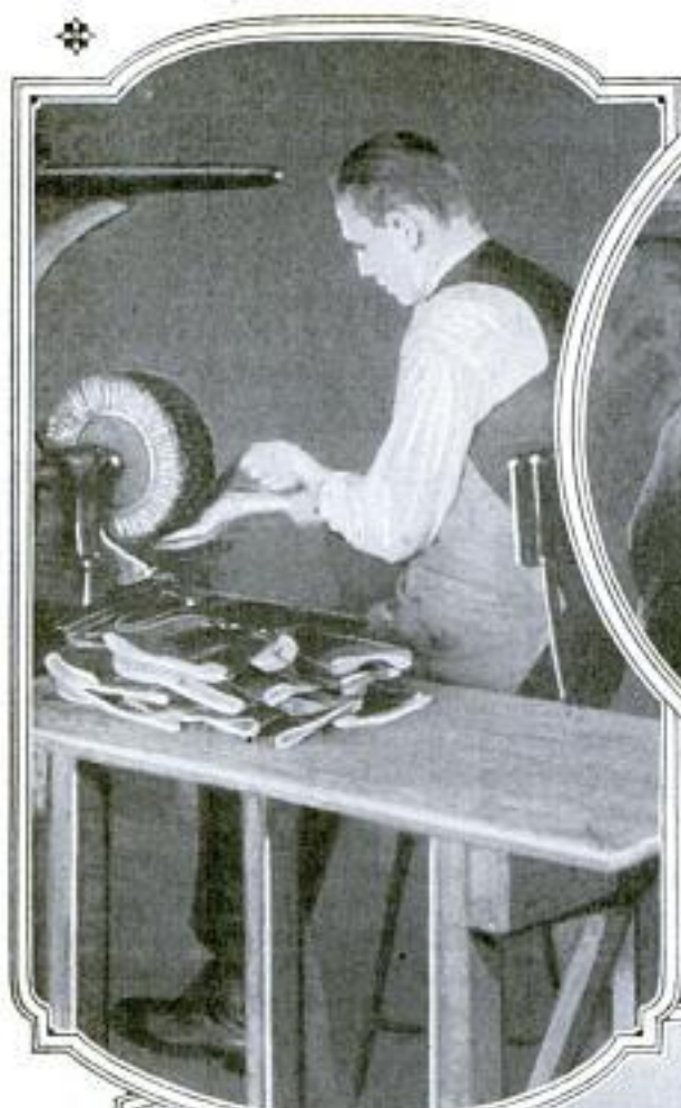
Above, Polishing Gloves against a Whirling Buffing Wheel Made of Silk; Below, Turn- ing Inseam Models Right Side Out
