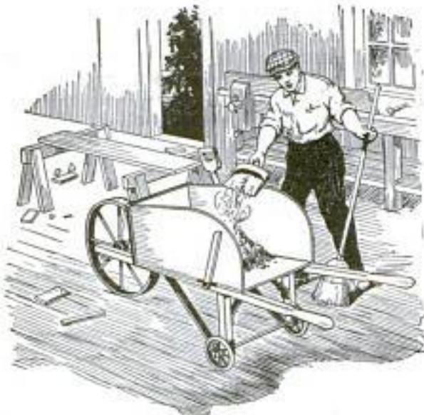
Small Auxiliary Wheels Added to the Barrow Lighten the Labor of Sweeping the Shop
