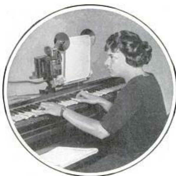
Copyright, Keystone View Co. Music Typewriter with Its Portable Piano Keyboard
