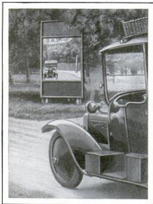
As Car Nears Curve, the Big Signboard Mirror Warns the Driver That Another Is Approaching
