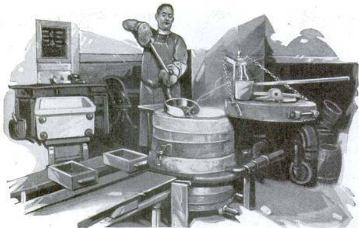
One of the Huge Melting Pots in the Assay Office Where Foreign Coins Are "Naturalized" for American Mints by Extracting the Various Alloys from the Metals
