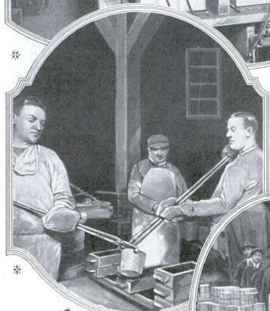
Above, the Gold-Refining Room of the U. S. Assay Office; Center, Pouring Molten Metal into Bar Molds for Storage in Vaults; Below, Overseas Shipment of Gold Being Delivered to Bank, in Boxes of One-Inch Lumber and No Larger than Those Used for Cigars; Left, Testing and Stamping Blocks of the Precious Metal
