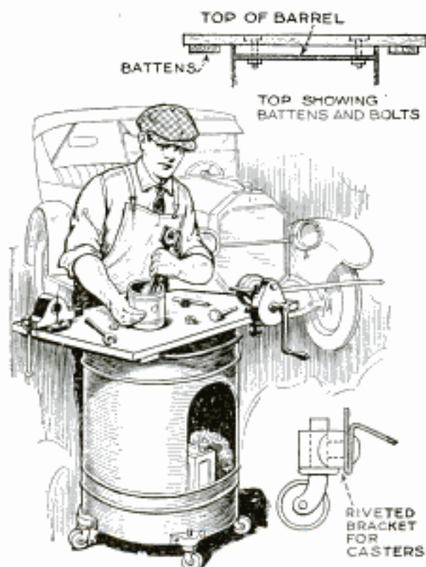
Sturdy Workbench Made from Oil Drum and Mounted on Casters
