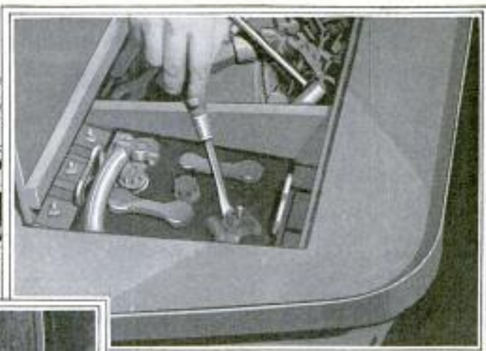
A Nail Driven between Connector and Post Tightens Battery Connection
