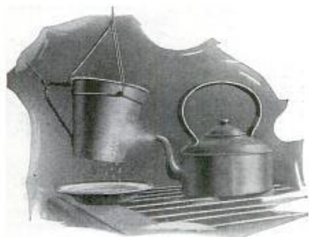
Distilling Water by Directing Steam of Kettle against Cooled Vessel
