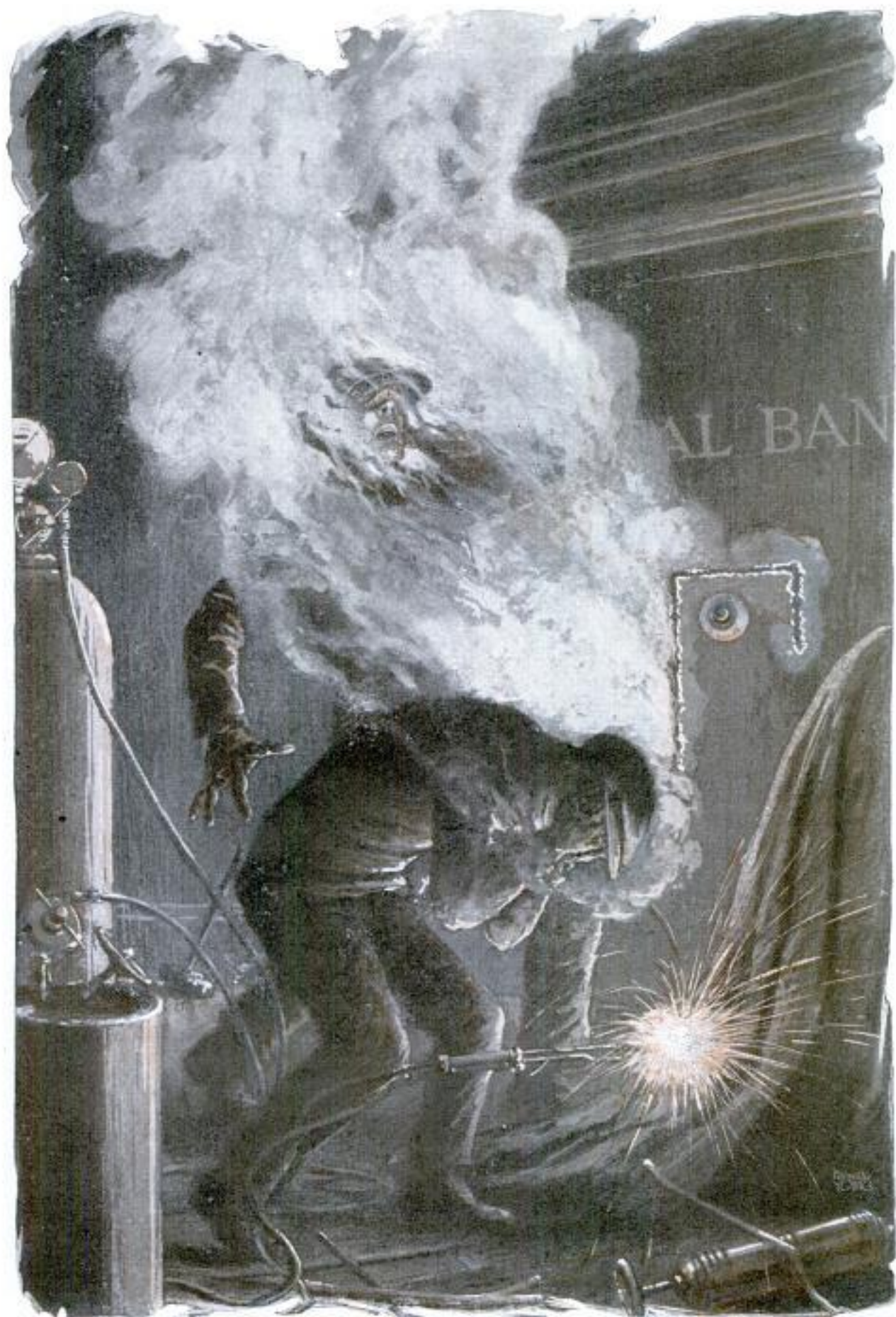
Set Off by Acetylene Torch Which Has Cut through Steel Door, a Tear-Gas Bomb, Placed Inside, Explodes, Compelling Cracksmen to Flee
