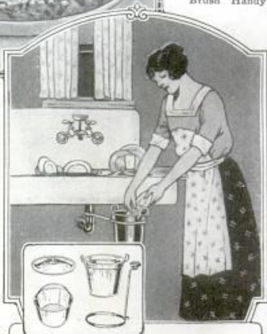
Catch Basin Fitted to Drain Pipe Keeps Refuse from Clogging the Sink
