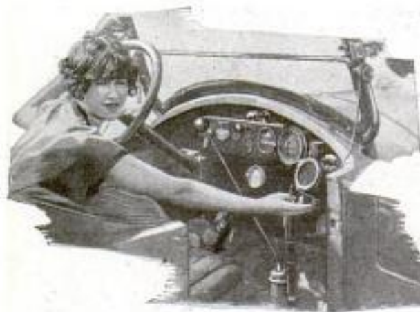
Instrument Board of the "Pathfinder" Automobile, Showing Compass, Altimeter and Other Devices
