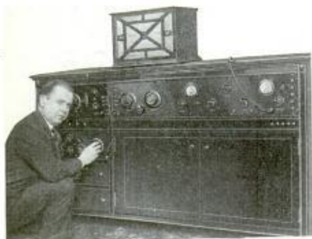
A Giant Set. Using a Combination of Either Eight, Nine, Eleven or Fourteen Tubes
