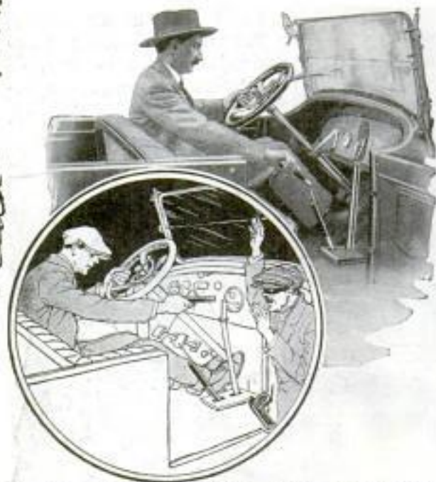
Inserting Pistol in Gear-Shift Lever, and Diagram Illustrating How It Could Be Used
