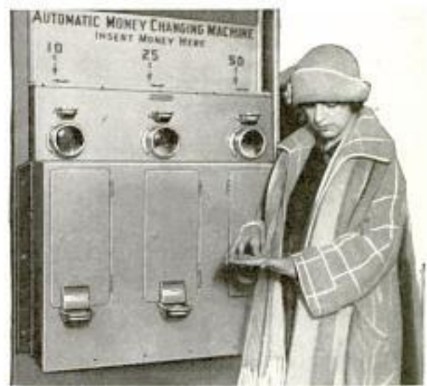
Machine That Automatically Changes Ten, Twenty-Five and Fifty-Cent Pieces into Smaller Denominations
