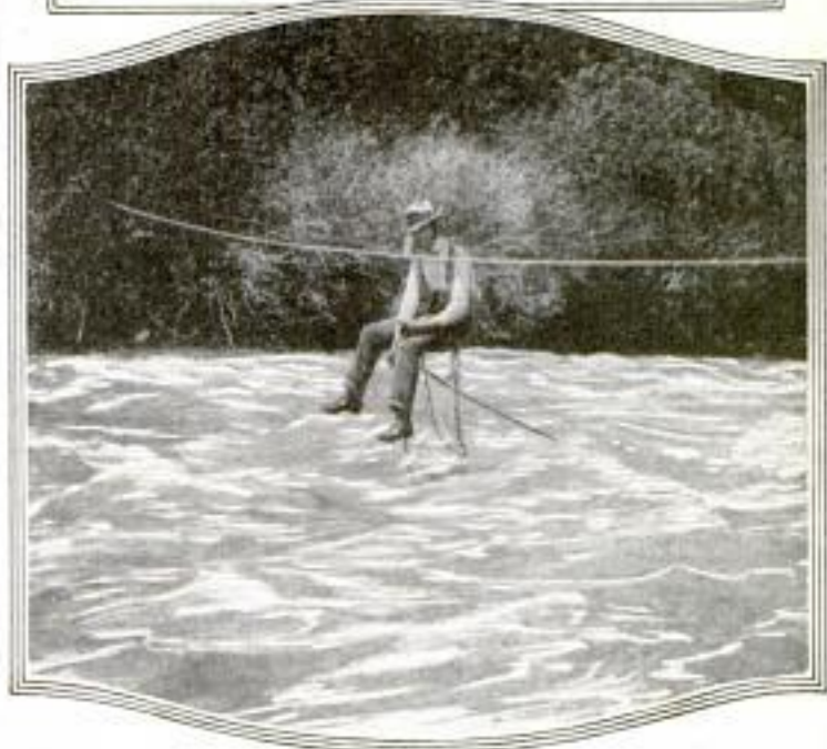
Water-Power Surveyor Seated in a Traveling Chair, Swinging above a Swollen River, While He Takes Soundings of Its Depths and Gauges Its Velocity; Similar Apparatus Are Installed at Hundreds of Points throughout the Country and Are Regularly Read by Inspectors
