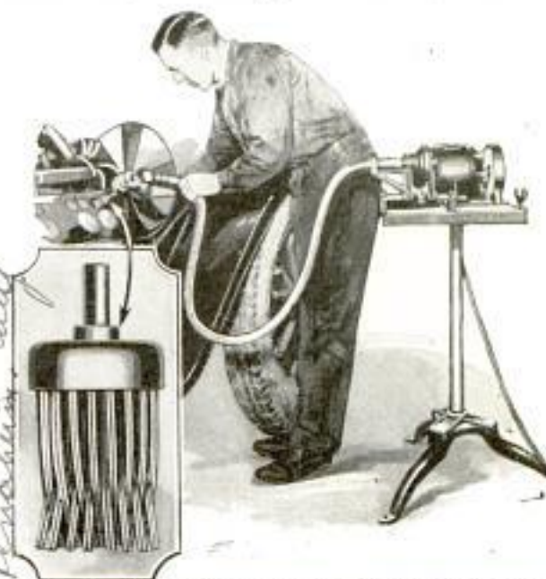
Removing Carbon Deposits from Cylinder Head with Stiff Wire Brush Operated by Electricity
