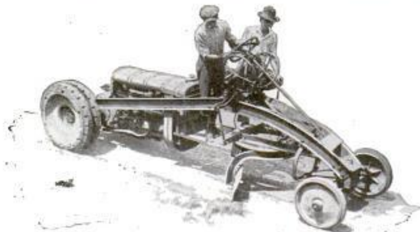
Copyright, Underwood & Underwood Compact One-Man Road Grader That Is Pushed Along by Tractor Engine and Heavy Wheels
