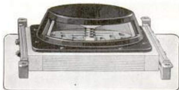
Ventilator in Roof of Auto Which Keeps Air Circulating on Interior When Car Travels
