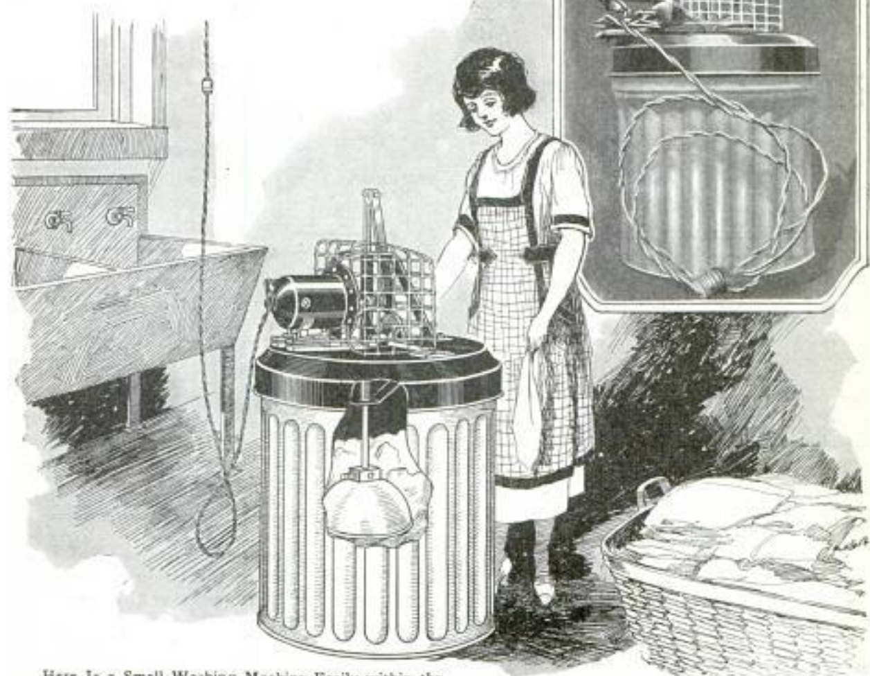
Here Is a Small Washing Machine Easily within the Ability of the Amateur Mechanic to Build, and That Will Wash Articles Up to Bath-Towel Size
