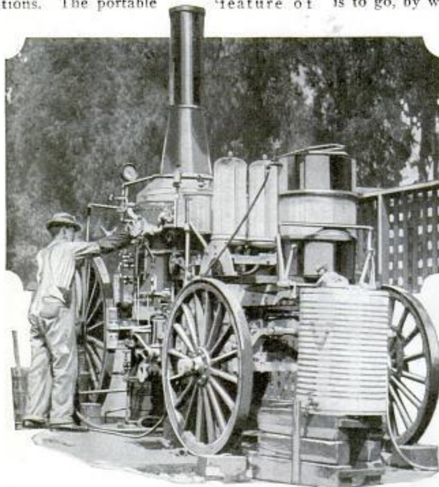
Discarded for Motor-Driven Equipment, Gallant Old Horse-Drawn Fire Engine Remodeled, on Duty as Oil-Refining Plant
