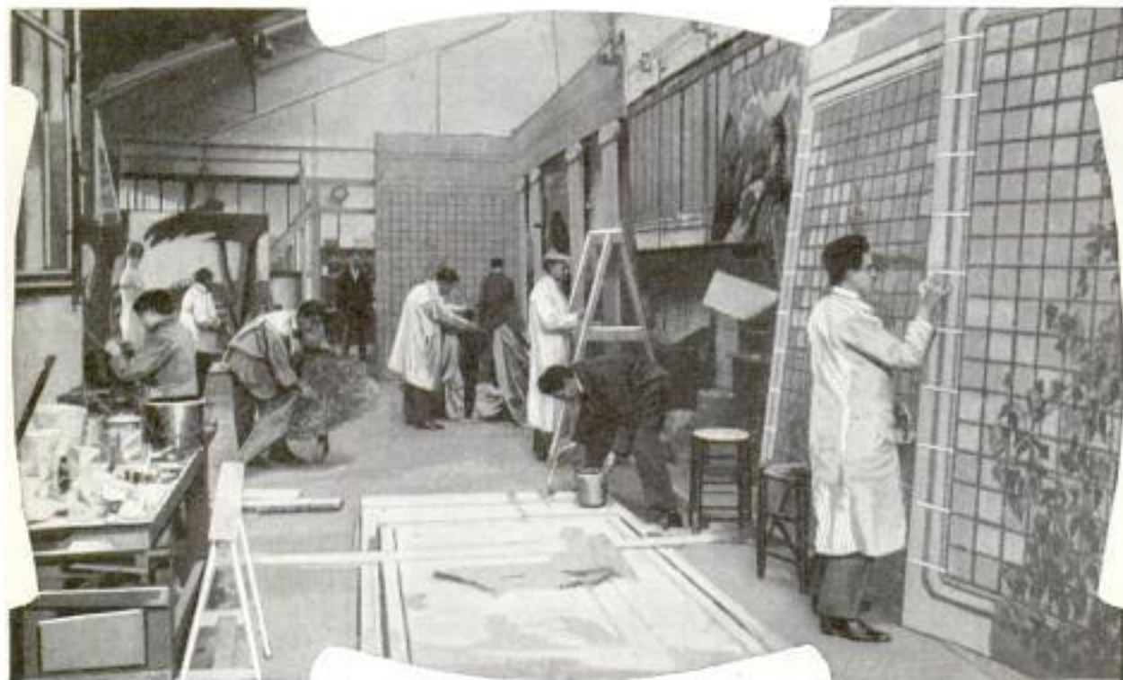
Studio Where Manikins and Ornamental Display Material Are Cut from Thin Wood to Replace Wax and Clay Models Used in Shop Windows and Show-Room Exhibitions
