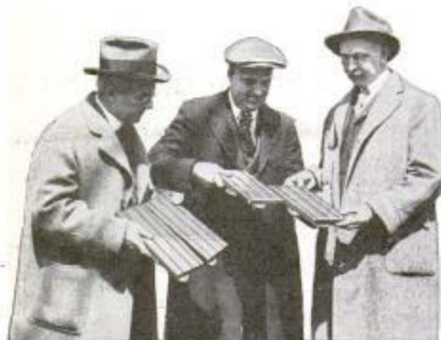
Inspecting Rubber Paving "Stones," with Which Much of Traffic Noise May Be Silenced
