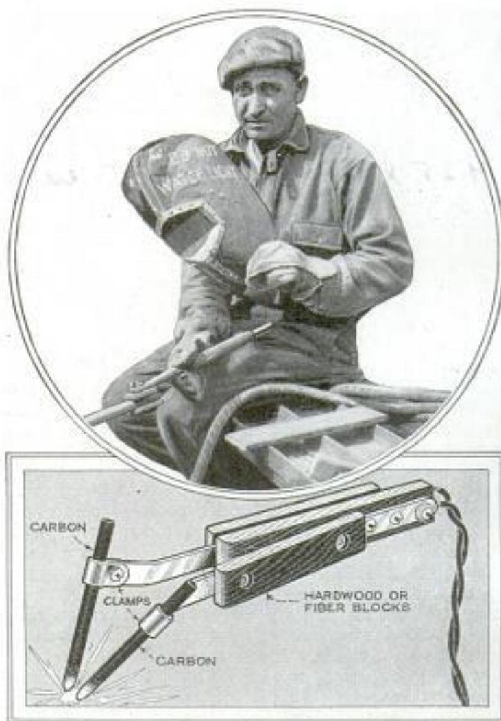
Fig. 1—Assembly View of the Portable Electric Welder. This Is an Easily Made Tool and One of Considerable Usefulness
